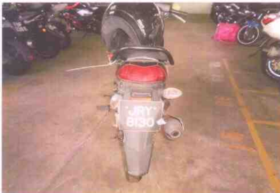
Photo 3 shows a general view of the rear body of the Motorcycle at the time of our inspection. The Motorcycle was observed to sustained minor damage at the rear left signal lamp at time of inspection.
