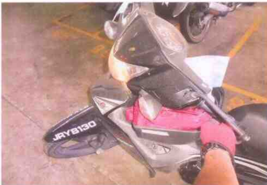
Photo 12 shows the steering system was observed to be in a serviceable condition. It was able to be steered to the full left at time of our inspection.
