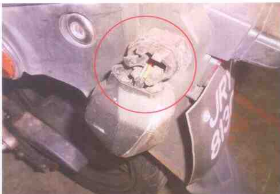
Photo 5 shows a closer view of the rear left signal lamp of the Motorcycle at the time of our inspection. It was observed to be damage likely due to the accident. (Circled)
