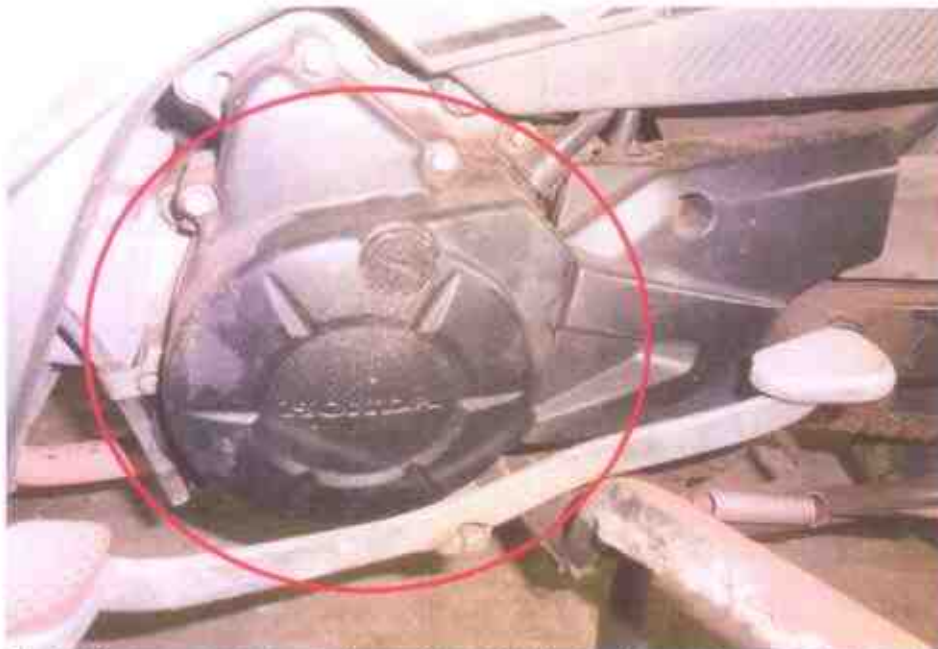
Photo 8 shows sign(s) or indication(s) of fluid leak observed around the left side of the engine area of the Motorcycle.
