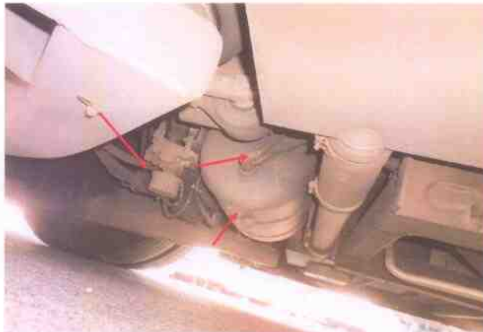
Photo 20 shows a general view of the air tank, valves, pipes and hoses, which are some of the components for the air-assisted braking system of the Motor Bus. This was at the underside of the Motor Bus's body. There were no damages observed at time of our inspection.
