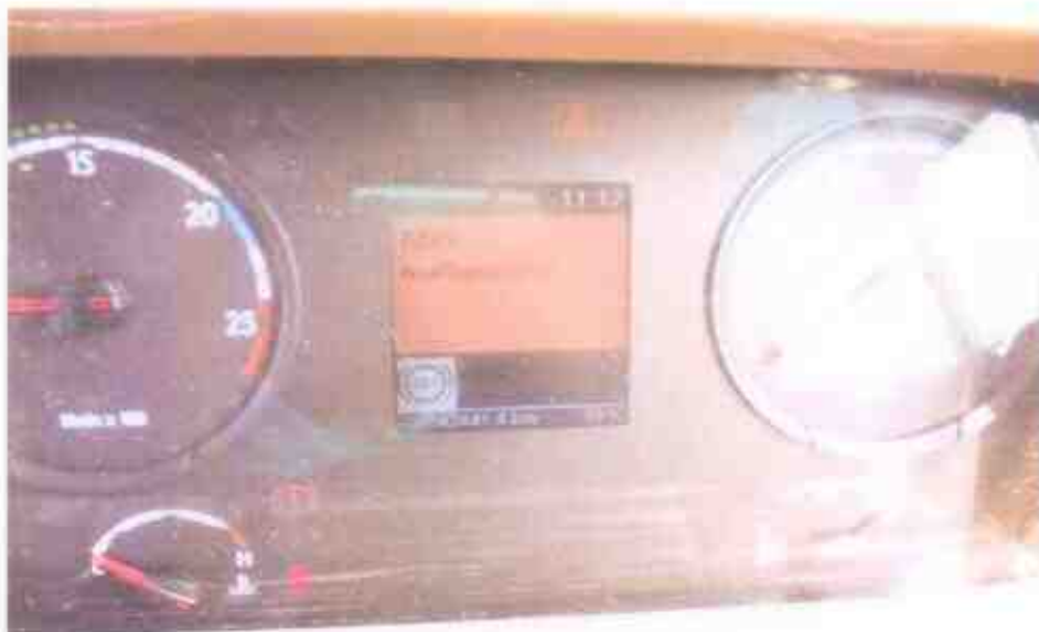
Photo 23 shows the warning lights for the various electronic operating systems of the Motor Bus appearing on its instrument panel during the self-test when the engine was cranked. However, only the Anti-Locking Braking System (ABS) stayed lighted up amongst others.
