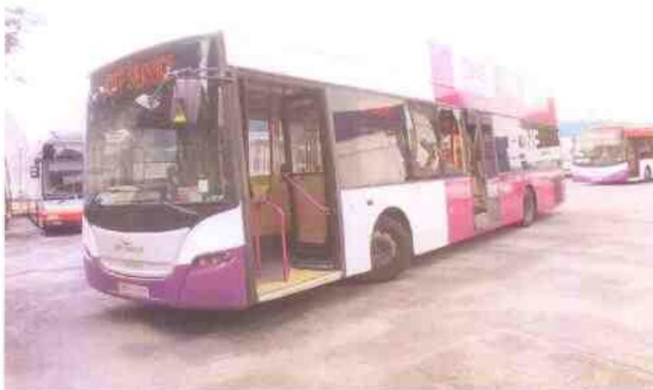
Photo 4 shows a general view of the Motor Bus front left portion that was observed with damages not consistent to the accident's case fact. Window glass & rear passenger door found to be damaged at time of our inspection. Refer to paragraph 6 for details.
