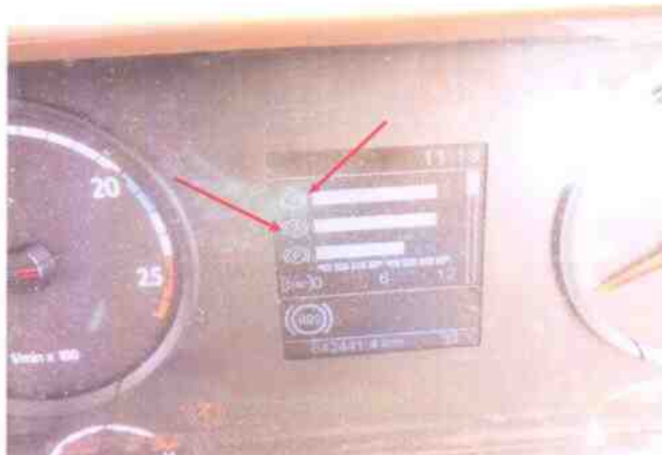
Photo 19 shows pressure tank 1 & tank 2 were observed to be pressurised up to 10bars after the engine start-up. No drop in the pressure after a few minutes which means there's no air leakage from the air-braking system.
