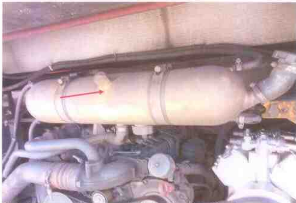
Photo 14 shows the engine coolant cylinder of the Motor Bus. It was observed to be of sufficient level without any contamination at time of our inspection.
