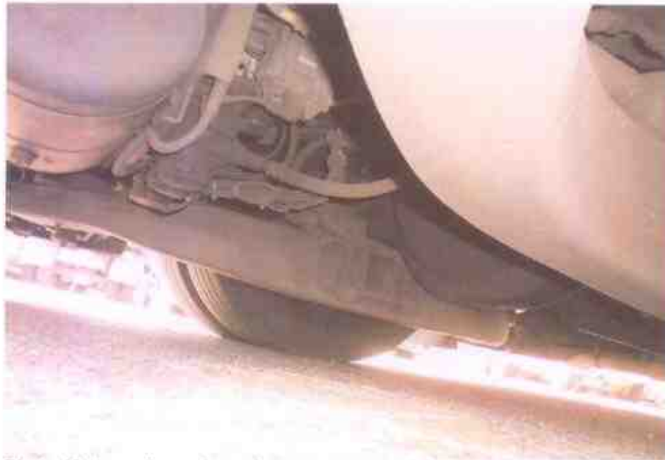
Photo 18 shows the undercarriage components at the rear steering system of the Motor Bus. The various undercarriage components of the Motor Bus were all observed to be intact and without any visible damage. This had included the transmission system of the Motor Bus, which were observed to be securely attached to the rear wheels.
