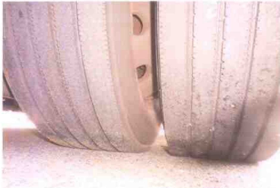
Photo 10 shows the condition of the rear left tyres of the Motor Bus, which were observed to be in serviceable condition with remaining tread depth of approximately 8mm. The tyres, which were wrapped around standard alloy wheel rims, were also observed to be sufficiently inflated for vehicular operation.
