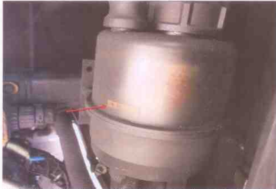
Photo 13 shows the steering fluid of the Motor Bus. It was observed to be of sufficient level without any contamination at time of our inspection.
