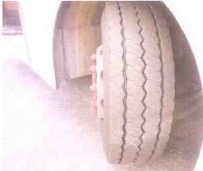
Photo 8 shows the condition of the front left tyre of the Motor Bus, which was observed to be in serviceable condition with remaining tread depth of approximately 9mm. The tyre was also observed to be sufficiently inflated for vehicular operation.
