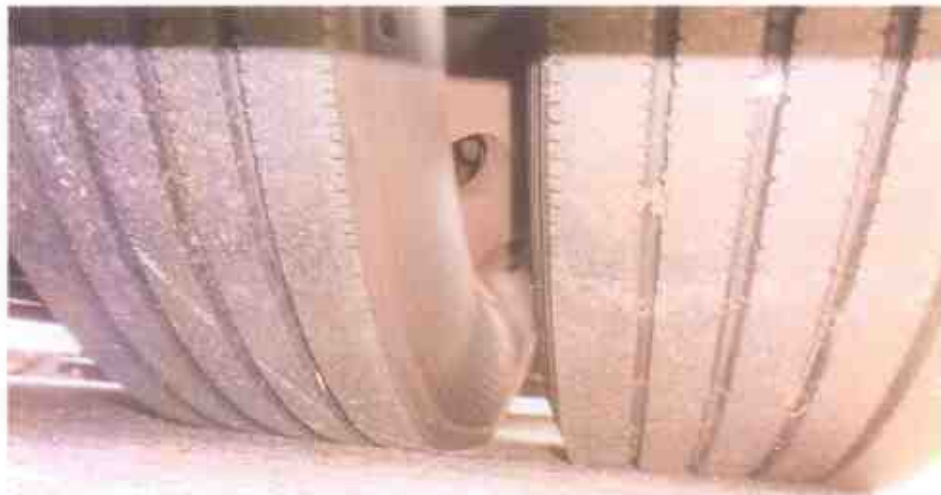
Photo 8 shows the condition of the front left tyre of the Motor Bus, which was observed to be in serviceable condition with remaining tread depth of approximately 9mm. The tyre was also observed to be sufficiently inflated for vehicular operation.
