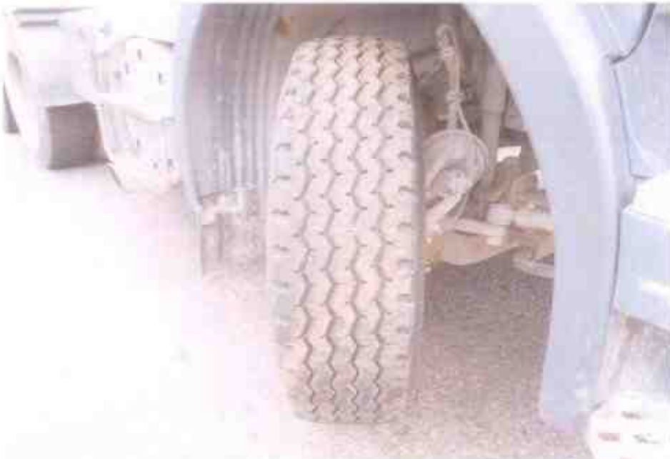
Photo 9 shows the condition of the front right tyre of the Motor Trailer, which was observed to be in serviceable condition with remaining tread depth of approximately 9mm.
