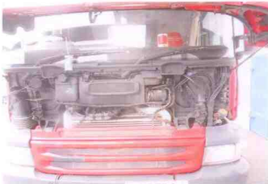
Photo 18 shows a general view of the engine compartment area from the front bonnet of the Motor Trailer. It was observed to be intact and unaffected by the collision. There was also no sign(s) or indication(s) of fluid leak and/or fluid stain found.
