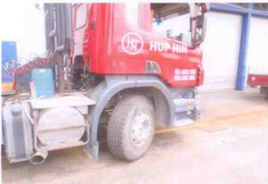
Photo 25 shows that we did not experience any abnormal free play and/or other resistance when turning the steering wheel left and right to full lock positions.
