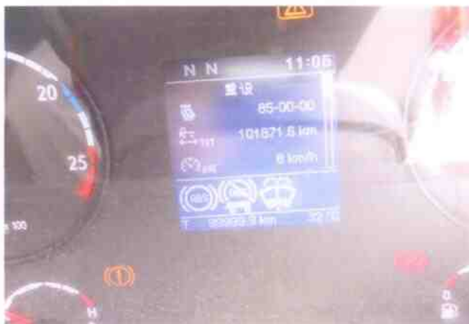
Photo 1 shows the mileage of the Motor Trailer at the time of our inspection was recorded at 101871.6 km.
