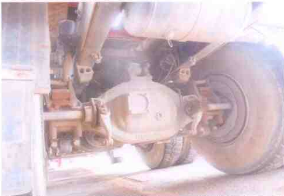
Photo 29 shows the brake hoses leading to the rear left wheel and rear right wheel of the Motor Trailer. At the time of our inspection, the various mechanical components of the air-assisted hydraulic braking system of the Motor Trailer were all found to be in good general condition and securely fitted.
