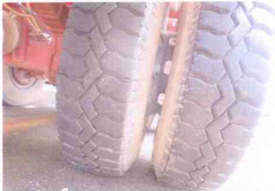
Photo 17 shows the condition of the rear right tyres of the Motor Trailer, which were observed to be in serviceable condition with remaining tread depth of approximately 8mm. The tyres, which were wrapped around standard alloy wheel rims, were also observed to be sufficiently inflated for vehicular operation.
