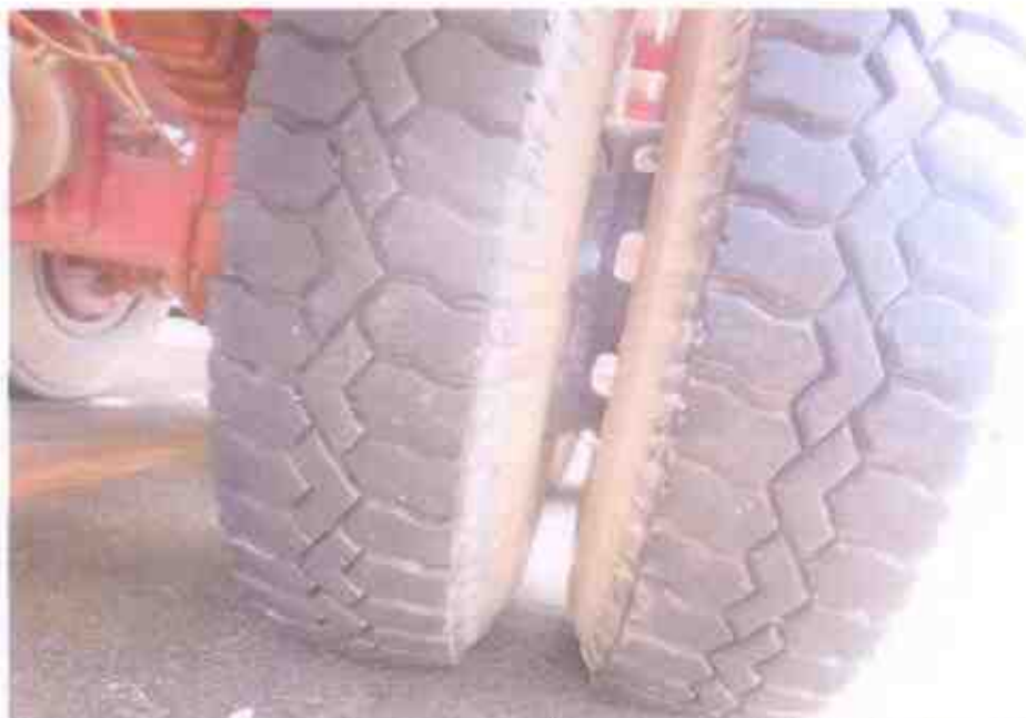
Photo 12 shows the condition of the left 4 th row tyres of the Motor Trailer, which were observed to be in serviceable condition with remaining tread depth of approximately 5mm. The tyres were also observed to be sufficiently inflated for vehicular operation.
