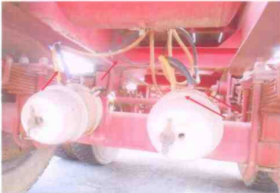
Photo 28 shows the valves, brake hoses and pipes, which are some of the components for the air-assisted braking system of the Motor Trailer. These components were observed to be unaffected by the accident. Our visual examination of these parts revealed all to be in good general condition and securely fitted.
