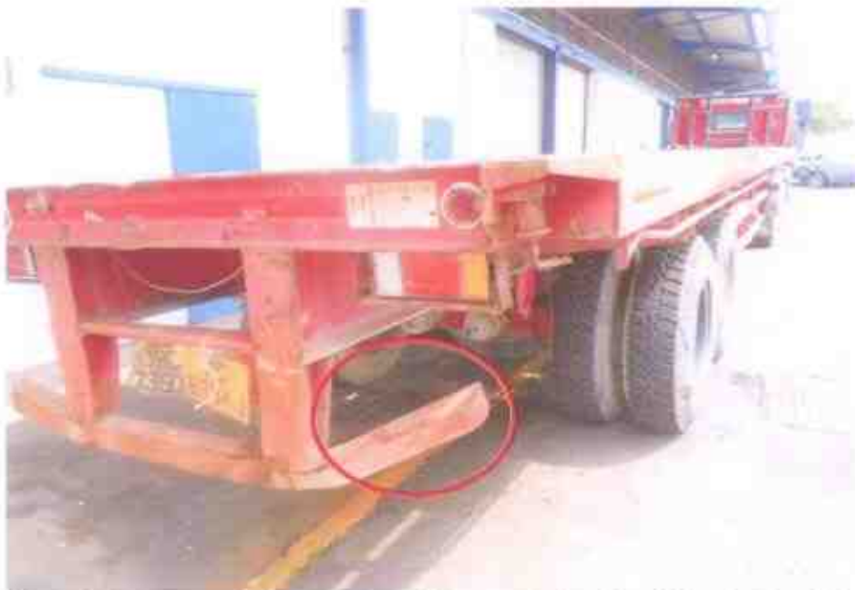
Photo 6 shows a semi-close-up view of the rear body of the Motor Trailer at the time of our inspection. It was observed to have sustained minor damages on the rear right crash bar due to the accident's impact collision.
