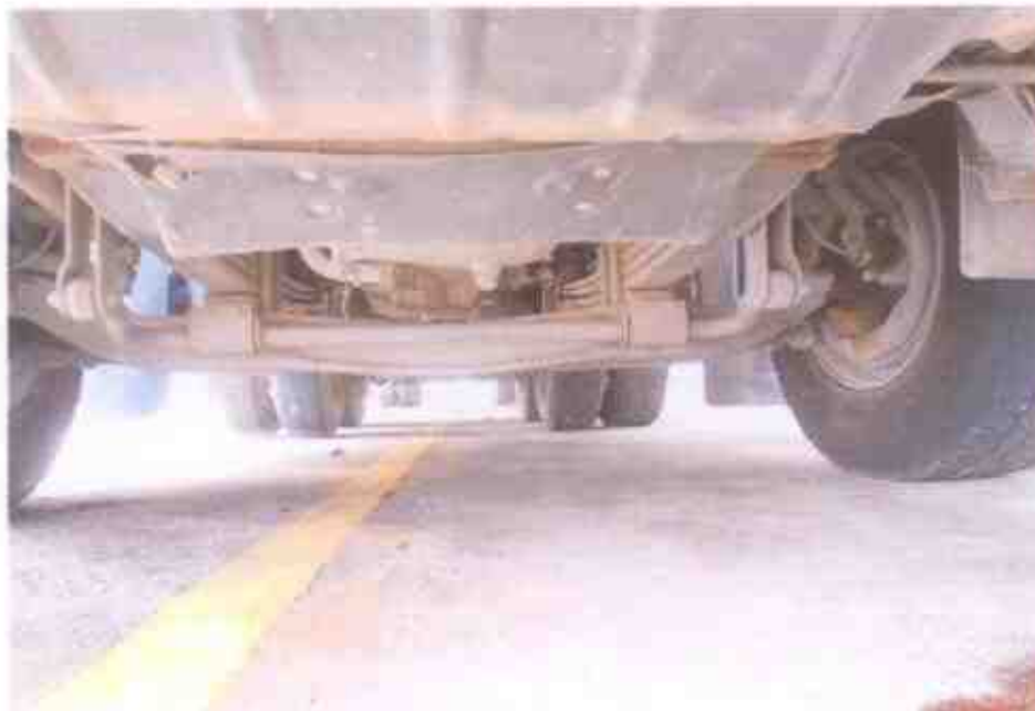
Photo 20 shows a general view of the engine area from the underside of the Motor Trailer. The engine assembly and transmission assembly of the Motor Trailer were both observed to be intact and unaffected by the collision. There was also no sign(s) or indication(s) of fluid leak and/or fluid stain found.
