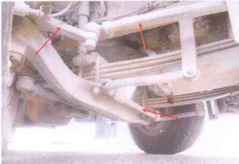
Photo 22 shows some of the mechanical components (arrowed) of the Motor Trailer's steering system. Our visual checks on the various mechanical components of the steering system revealed all to be intact and in good condition. The steering system of the Motor Trailer is hence likely to be in serviceable condition at the time of accident.
