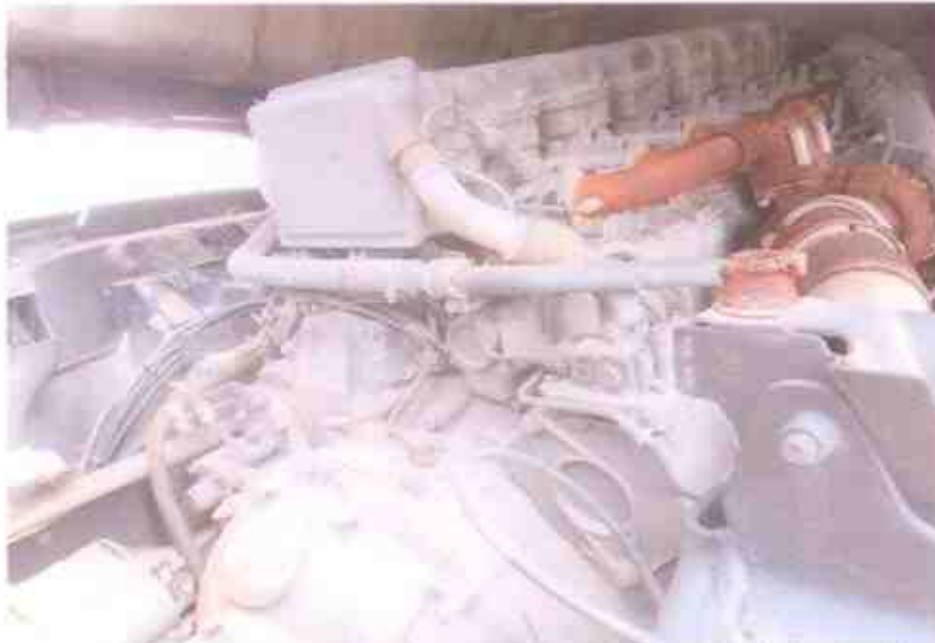
Photo 19 shows a general view of the engine area from under the front cabin of the Motor Trailer. The engine assembly and transmission assembly of the Motor Trailer were both observed to be intact and unaffected by the collision. There was also no sign(s) or indication(s) of fluid leak and/or fluid stain found.
