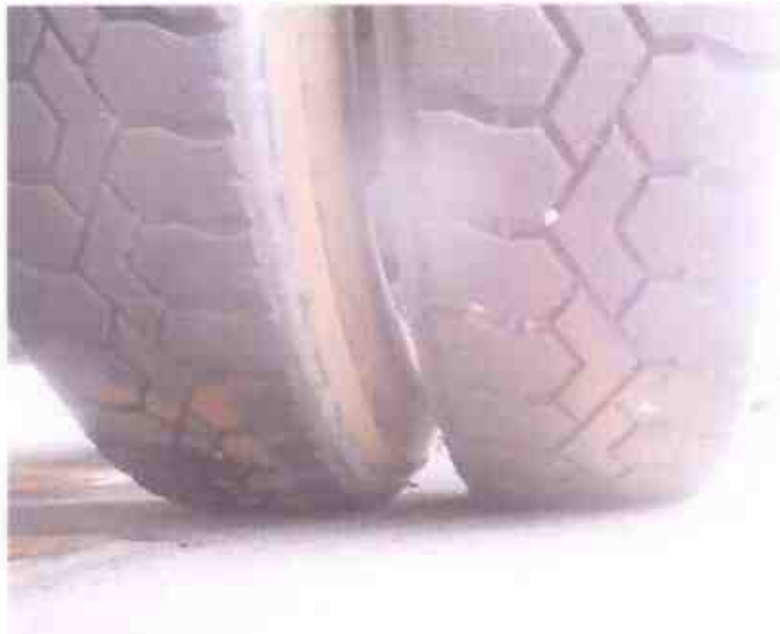
Photo 14 shows the condition of the right 2 nd row tyres of the Motor Trailer, which were observed to be in serviceable condition with remaining tread depth of approximately 7mm. The tyres were also observed to be sufficiently inflated for vehicular operation.
