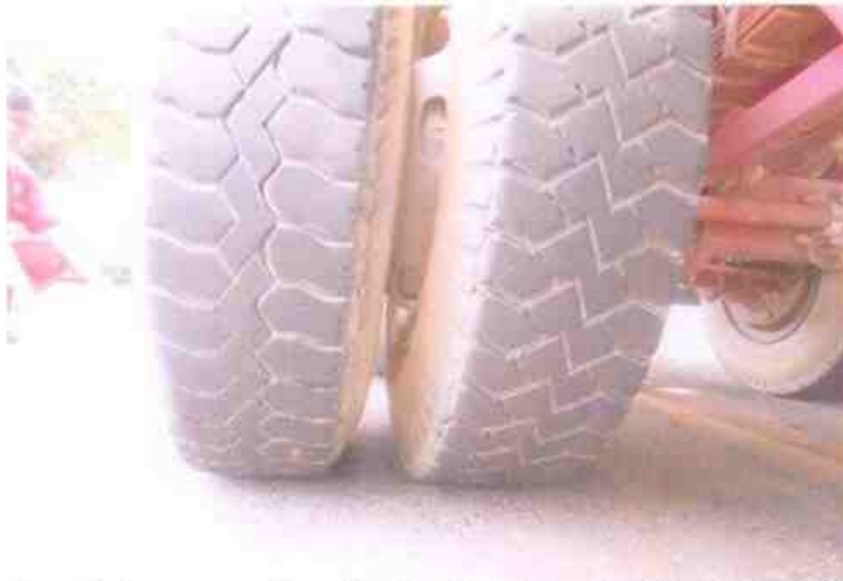
Photo 16 shows the condition of the right 4 th row tyres of the Motor Trailer, which were observed to be in serviceable condition with remaining tread depth of approximately 5mm. The tyres were also observed to be sufficiently inflated for vehicular operation.
