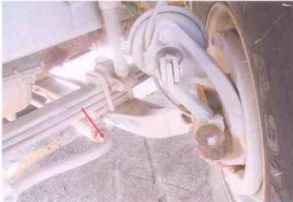
Photo 24 shows the undercarriage components at the front left wheel of the Motor Trailer. The various undercarriage components of the Motor Trailer were all observed to be intact and without any visible damage. This had included the steering rack (arrowed) of the Motor Trailer, which was observed to be securely attached to the front left wheel and front right wheel.
