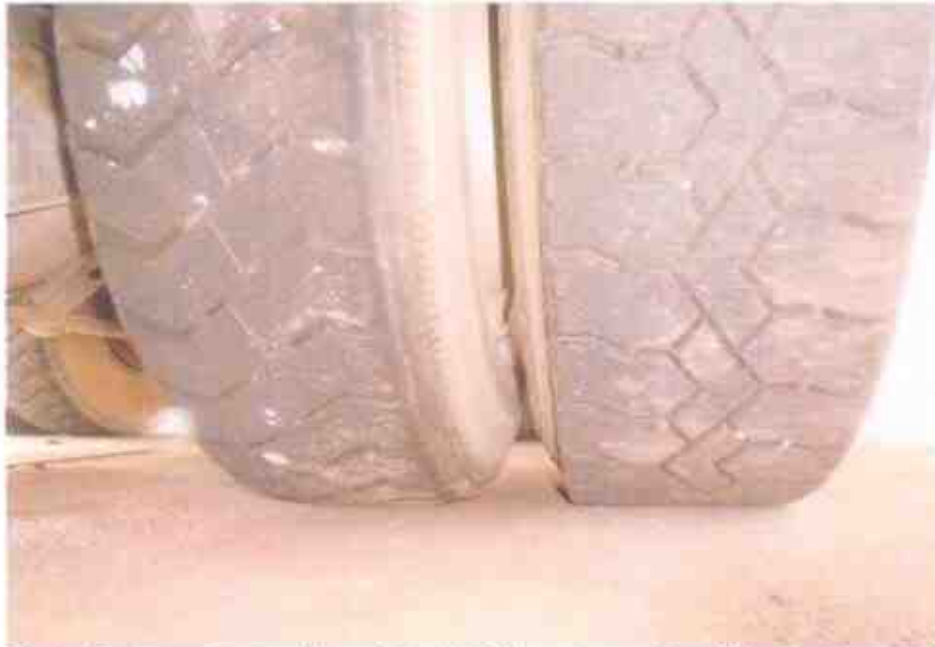
Photo 10 shows the condition of the left 2 nd row tyres of the Motor Trailer, which were observed to be in serviceable condition with remaining tread depth of approximately 6mm. The tyres were also observed to be sufficiently inflated for vehicular operation.
