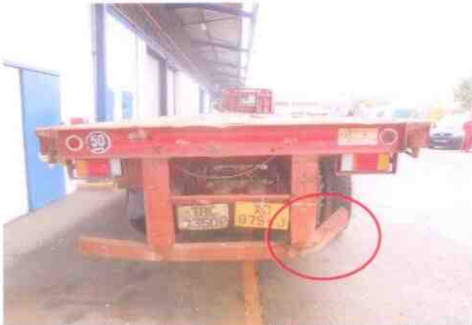
Photo 5 shows a general view of the rear body of the Motor Trailer at the time of our inspection. It was observed to have sustained minor damages on the rear right crash bar due to the accident's impact collision.
