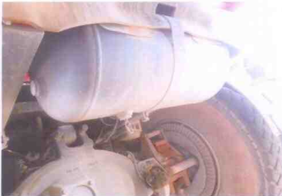
Photo 27 shows the air tanks, valves, pipes and hoses, which are some of the components for the full air-assisted braking system of the Motor Trailer. These components were mainly located at the underside of the Motor Trailer and were unaffected by the accident.
