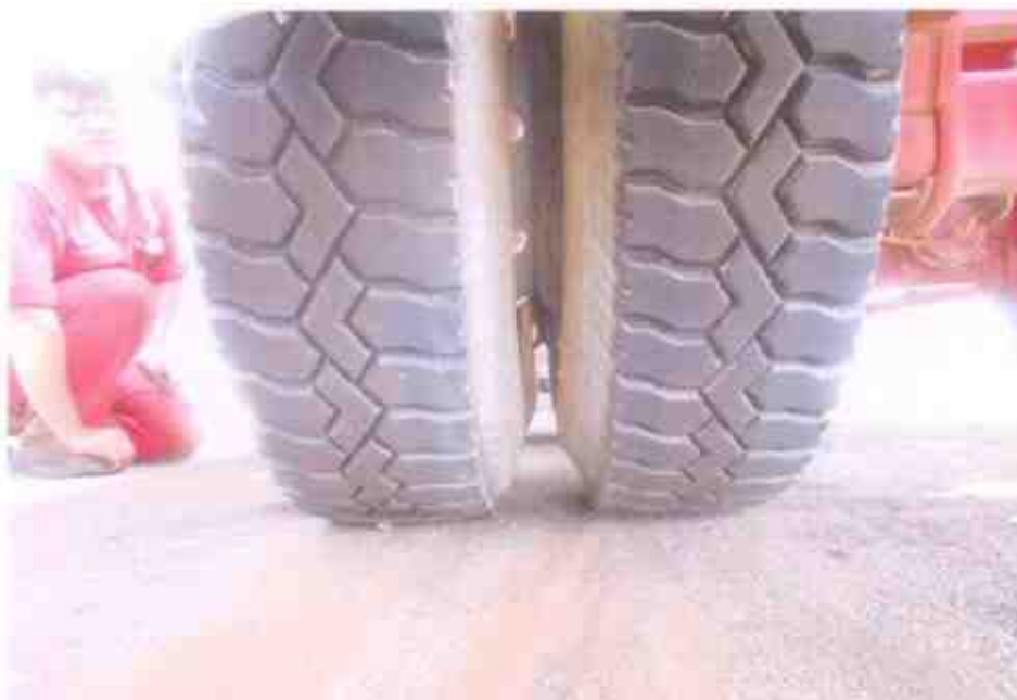
Photo 13 shows the condition of the rear left tyres of the Motor Trailer, which were observed to be in serviceable condition with remaining tread depth of approximately 8mm. The tyres, which were wrapped around standard alloy wheel rims, were also observed to be sufficiently inflated for vehicular operation.
