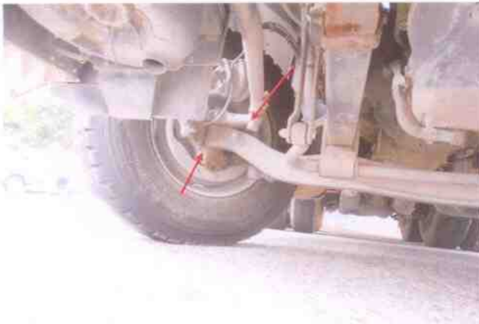
Photo 23 shows the undercarriage components at the front right wheel of the Motor Trailer. The various undercarriage components of the Motor Trailer were all observed to be intact and without any visible damage. This had included the steering rack and steering linkages (arrowed) of the Motor Trailer.
