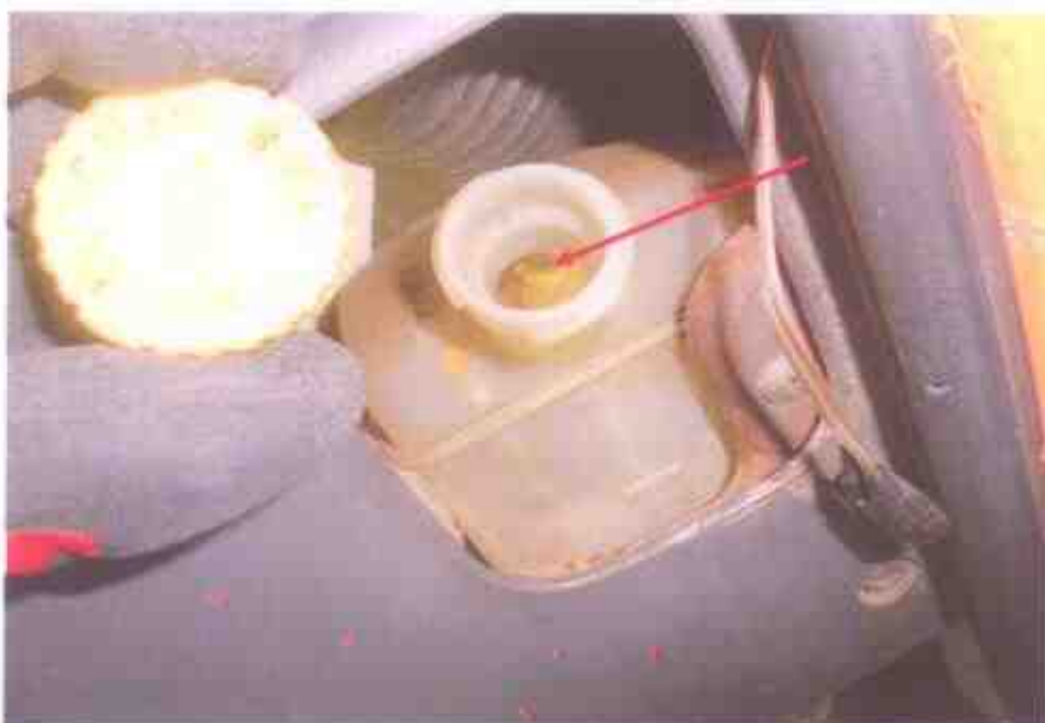
Photo 13 shows the brake fluid reservoir of the Motor Lorry at the time of our inspection. The brake fluid was observed to be of sufficient level and without any visible contamination (arrowed).
