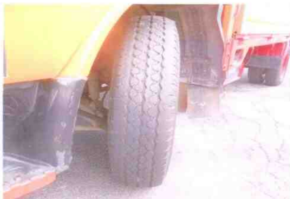
Photo 8 shows the condition of the front left tyre of the Motor Lorry, which was observed to be in serviceable condition with remaining tread depth of approximately 6mm. The tyre, which was wrapped around standard alloy wheel rim, was also observed to be sufficiently inflated for vehicular operation.
