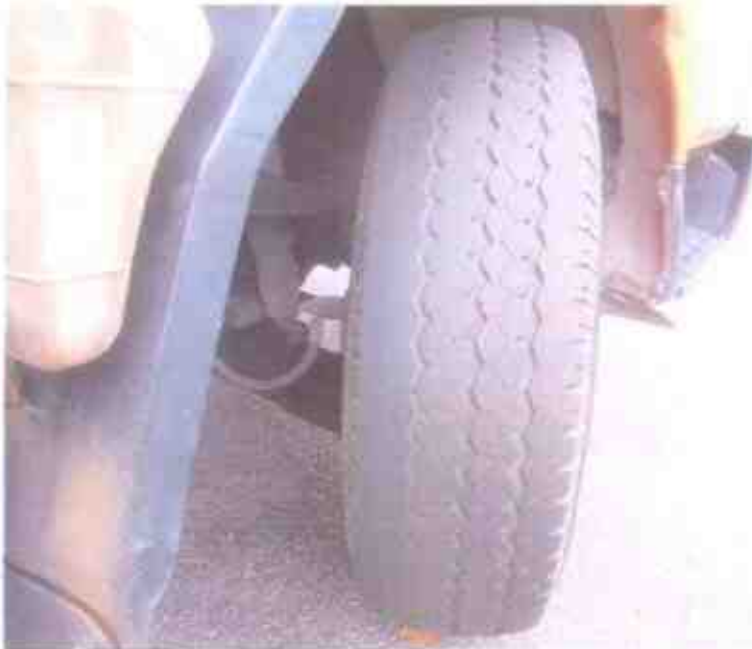
Photo 9 shows the condition of the front right tyre of the Motor Lorry, which was observed to be in serviceable condition with remaining tread depth of approximately 5mm. The tyre, which was wrapped around standard alloy wheel rim, was also observed to be sufficiently inflated for vehicular operation.
