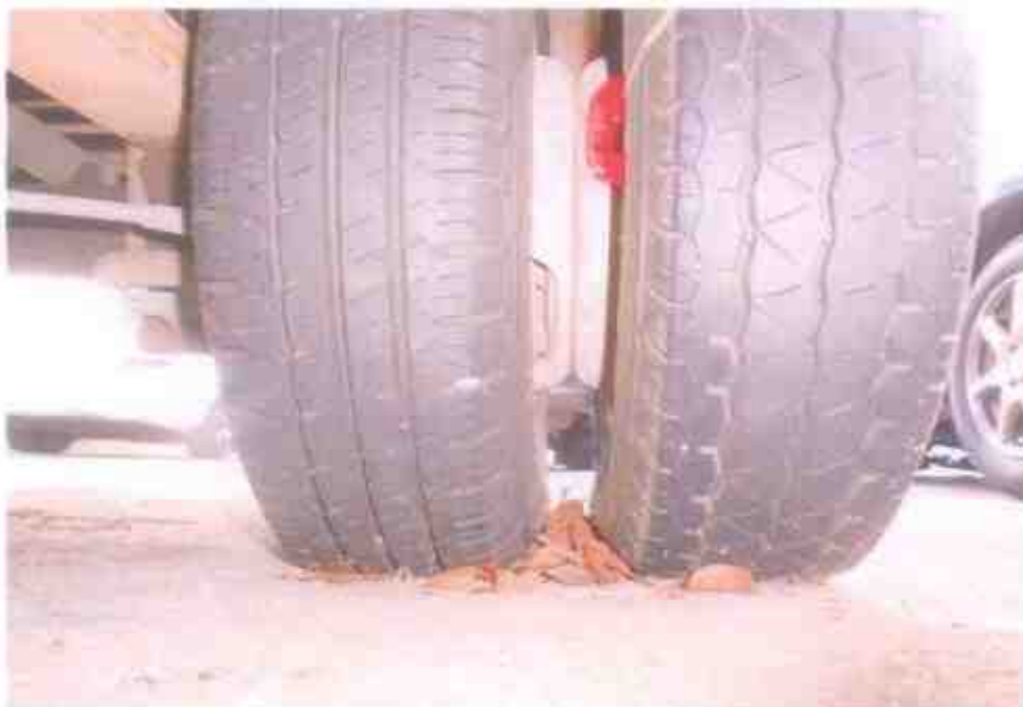
Photo 10 shows the condition of the rear left tyres of the Motor Lorry, which was observed to be in serviceable condition with remaining tread depth of approximately 5mm. The tyres, which were wrapped around standard alloy wheel rim, were also observed to be sufficiently inflated for vehicular operation.
