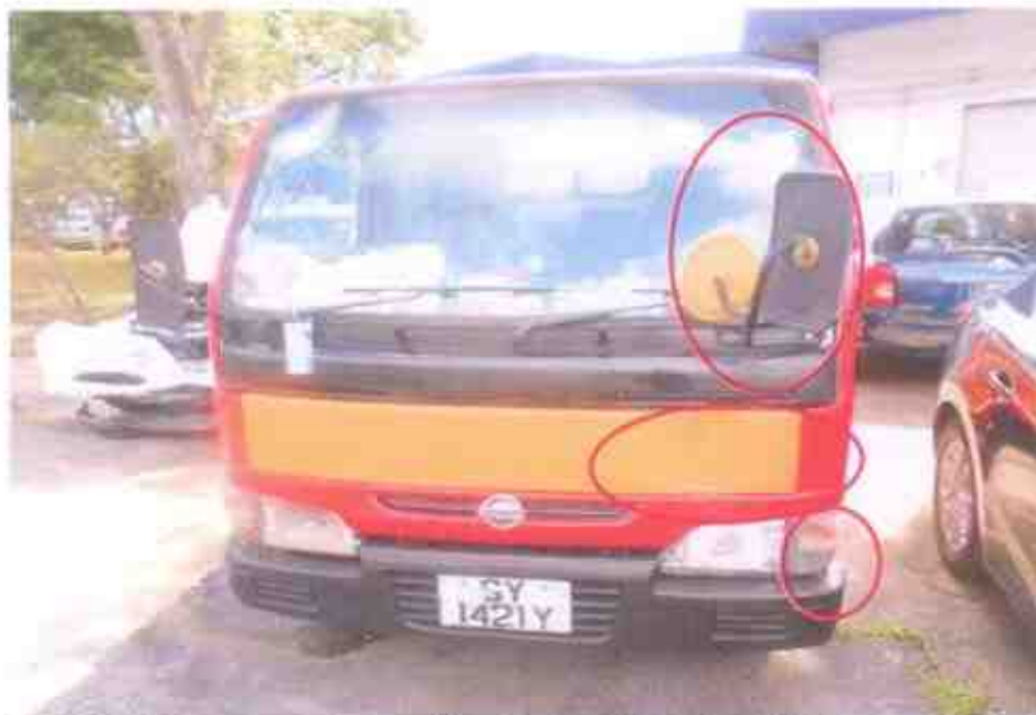
Photo 2 shows a general view of the front portion of the Motor Lorry at the time of our inspection. The Motor Lorry was observed to have sustained minor damage at its front left signal lamp and its front panel were amongst the body parts that were damaged as a result of the accident.
