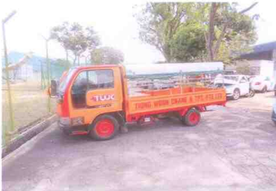
Photo 19 shows the operational test on the Motor Lorry. It was observed to be in serviceable condition. Operational test such as moving forward, turn left & right and also braking test on the Motor Lorry was conducted successfully.
