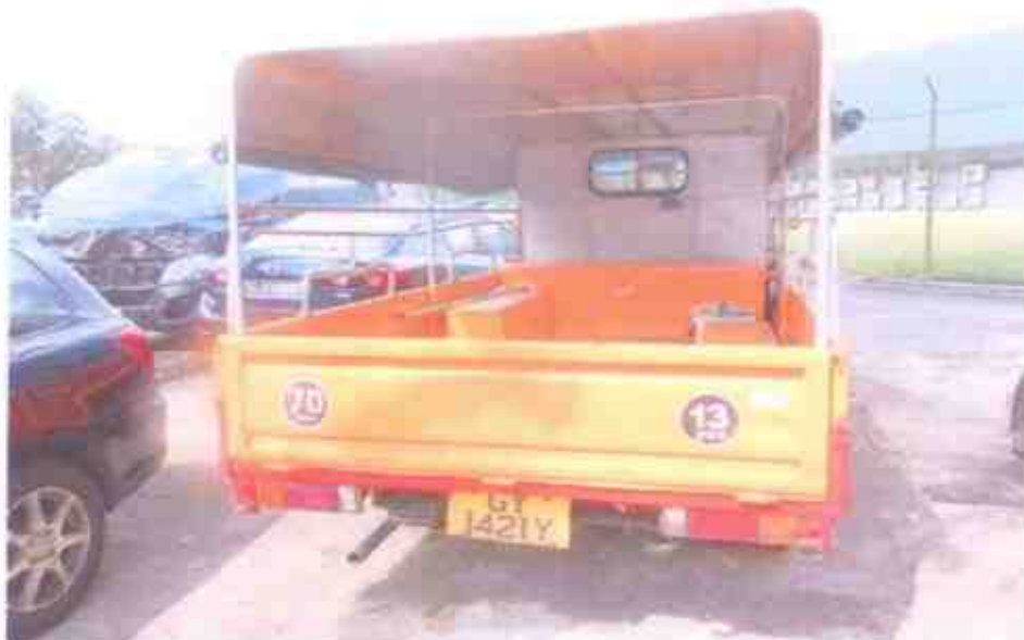
Photo 7 shows a general view of the Motor Lorry's rear body at the time of our inspection. There was no damage found to the rear portion of the Motor Lorry.
