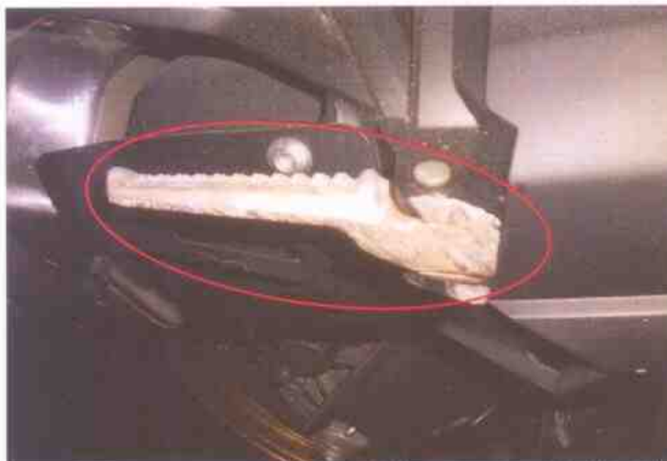
Photo 7 shows a closer view of the pillion's foot rest on the right side of the Motorcycle at the time of our inspection. It was observed to sustained deep scratches due to the accident collision. (Circled)
