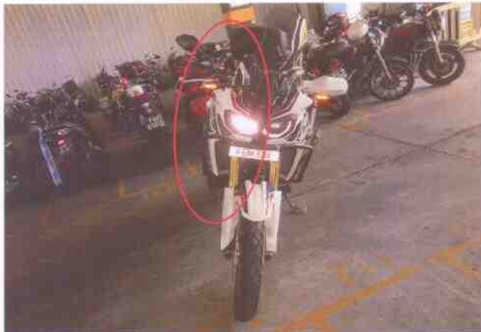
Photo 2 shows a general view of the front portion of the Motorcycle at the time of our inspection. The Motorcycle was observed to be sustained with relatively minor impact due to the accident collision. (Circled)
