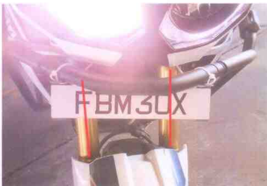
Photo 16 shows the front fork was observed to be slightly bent likely due to the accident's impact.
