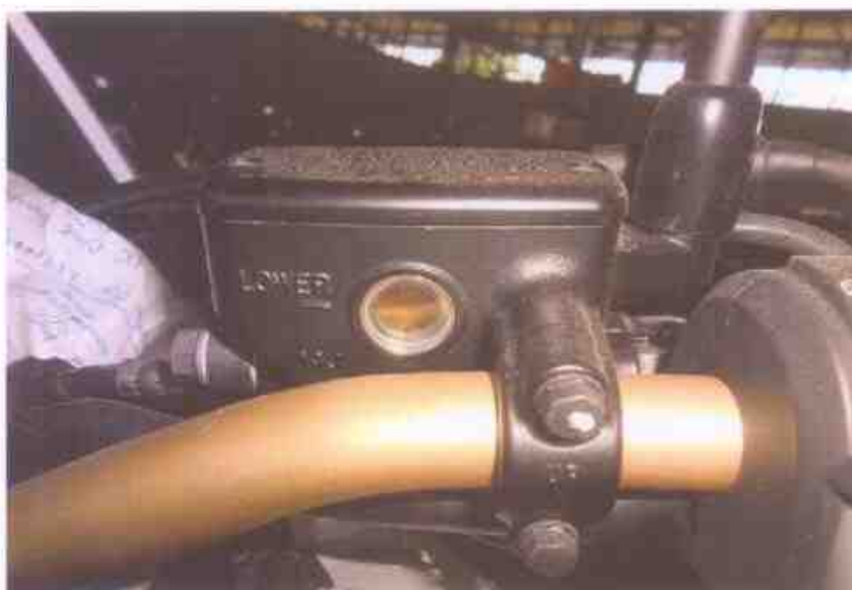
Photo 17 shows the brake fluid reservoir for front brake observed to be sufficient at time of our inspection.
