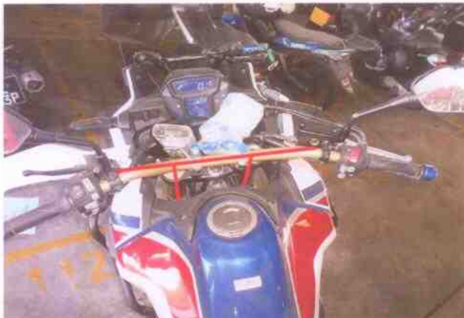
Photo 15 shows the steering system was observed to be slightly bent likely due to the accident's impact.
