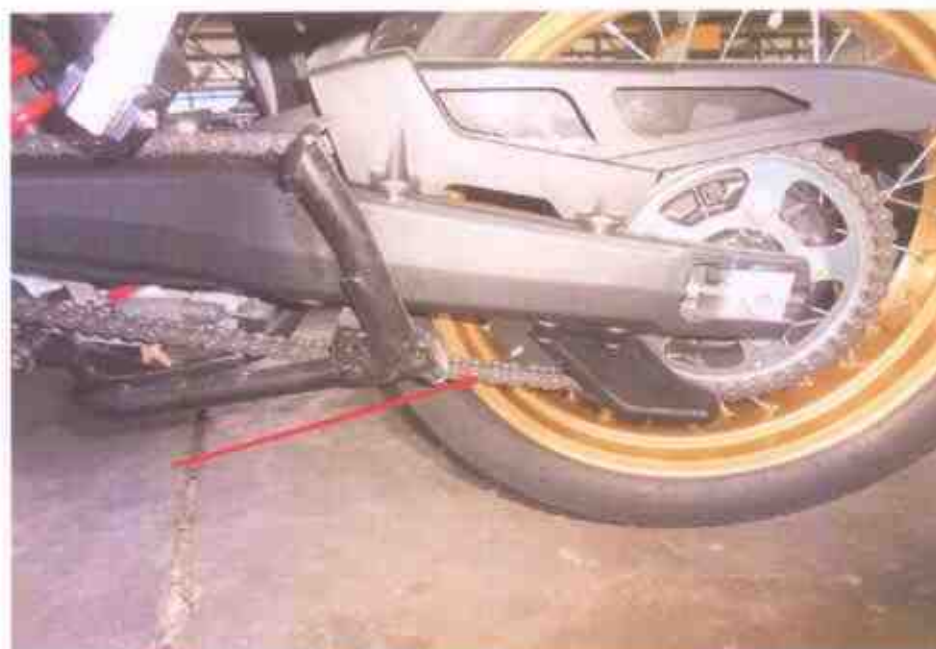
Photo 13 shows the general view of the gear train (arrowed) of the Motorcycle, which was observed to be intact with no misalignment. It was also adequately lubricated for operating purposes.
