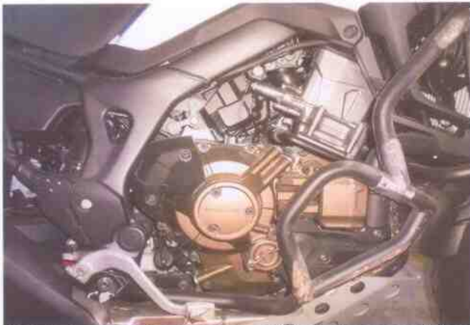
Photo 11 shows no sign(s) or indication(s) of fluid leak observed around the top side of the engine area of the Motorcycle.
