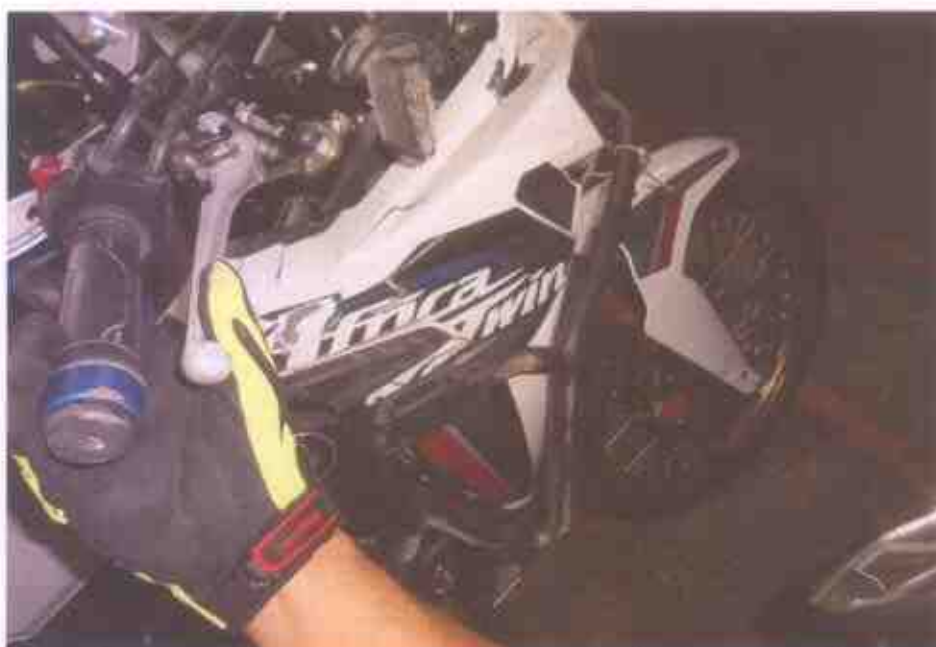
Photo 21 shows testing of the braking of the front brake in progress. There was some resistance felt (spongy like feel) upon pressing the brake lever.
