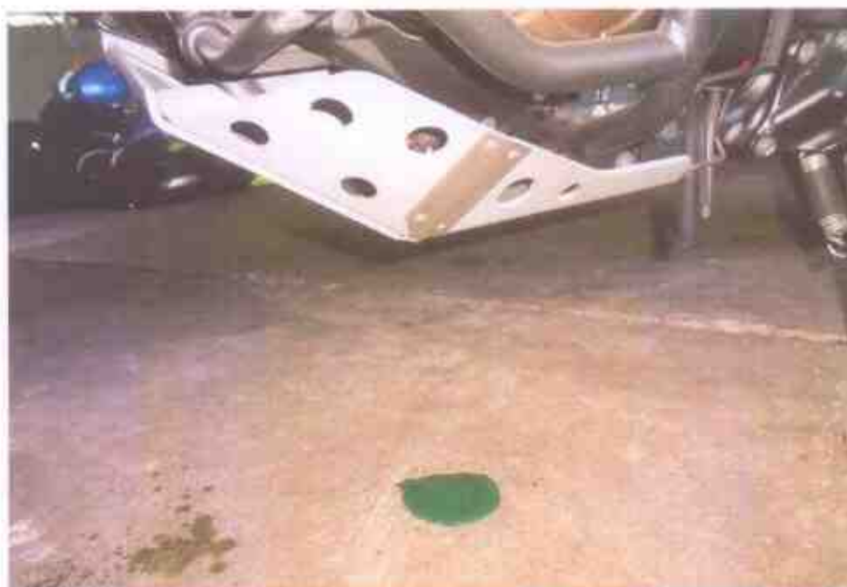
Photo 12 shows sign(s) or indication(s) of fluid leakage was observed around the underside of the engine area of the Motorcycle. The fluid was believe to be engine coolant gushed out from the underside of the engine compartment upon cranking of the Motor Cycle.
