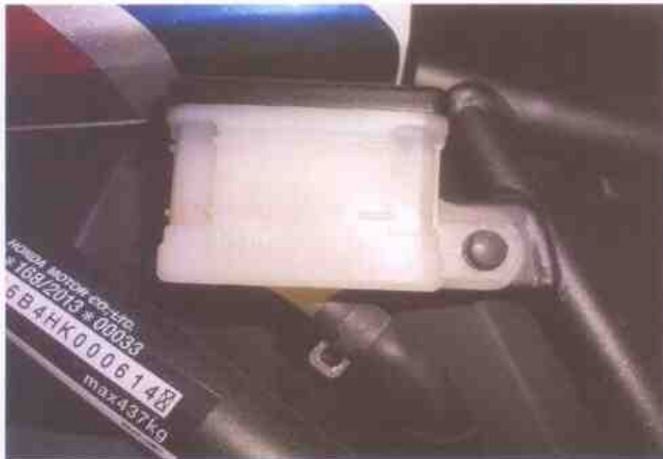
Photo 18 shows the brake fluid reservoir for rear brake observed to be sufficient at time of our inspection.
