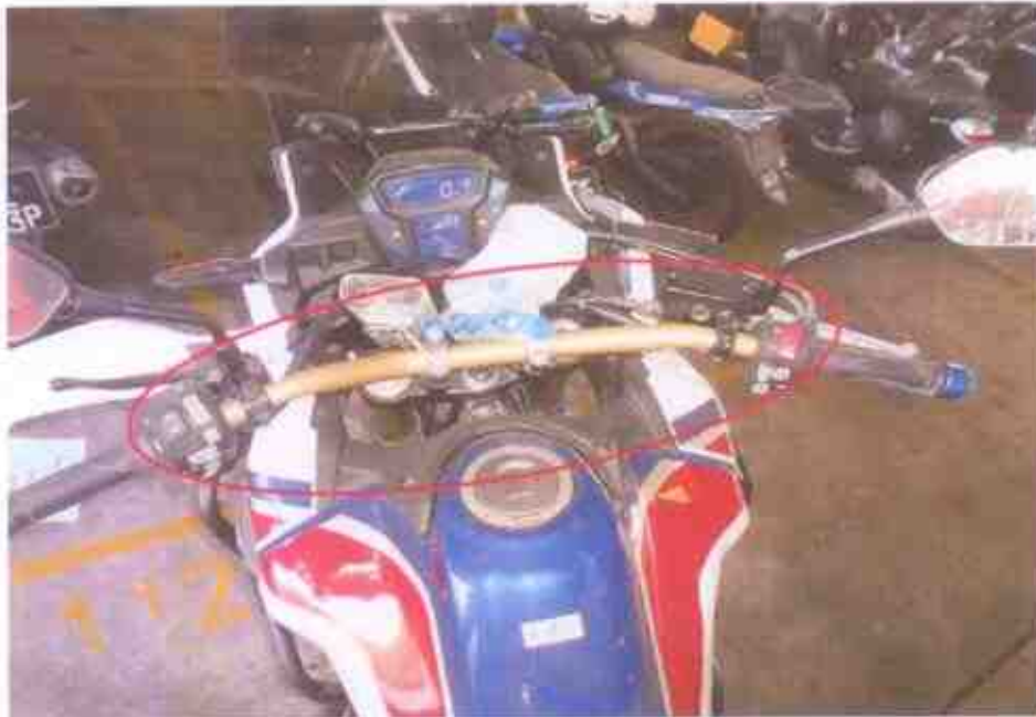
Photo 5 shows a closer view of the handle bar of the Motorcycle at the time of our inspection. It was observed to be misaligned from the front fork due to the accident collision. (Circled)
