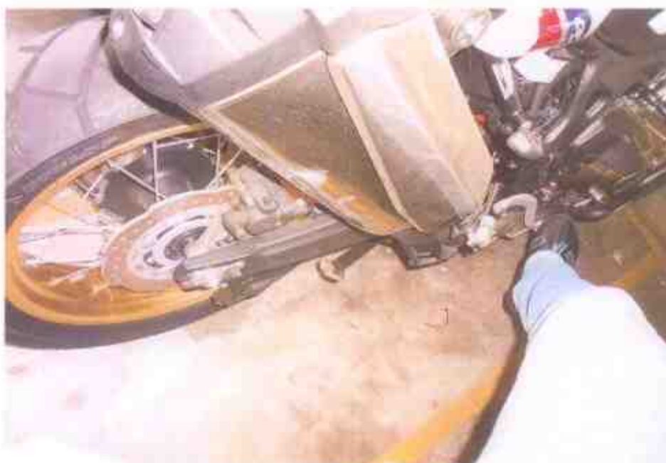
Photo 22 shows testing of the braking of the front brake in progress. There was some resistance felt (spongy like feel) upon pressing the brake lever.
