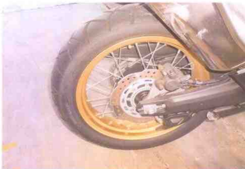
Photo 20 shows the braking system for the rear brake. It was observed to be in serviceable condition at time of our inspection. The braking components were found to be intact unaffected by the accident's impact collision.
