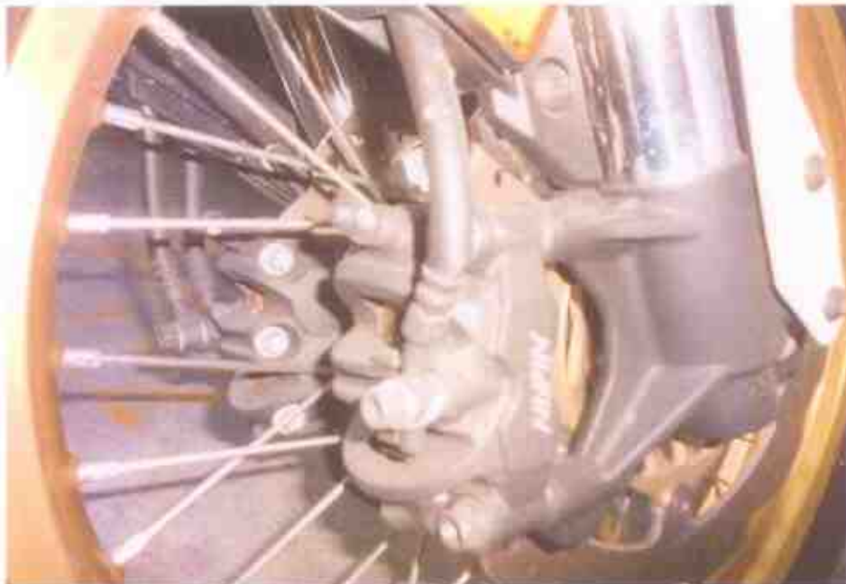
Photo 19 shows the braking system for the front brake. It was observed to be in serviceable condition at time of our inspection. The braking components were found to be intact unaffected by the accident's impact collision.
