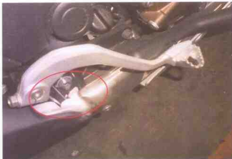
Photo 6 shows a closer view of the rider's foot rest on the right side of the Motorcycle at the time of our inspection. It was observed to be broken due to the accident collision. (Circled)
