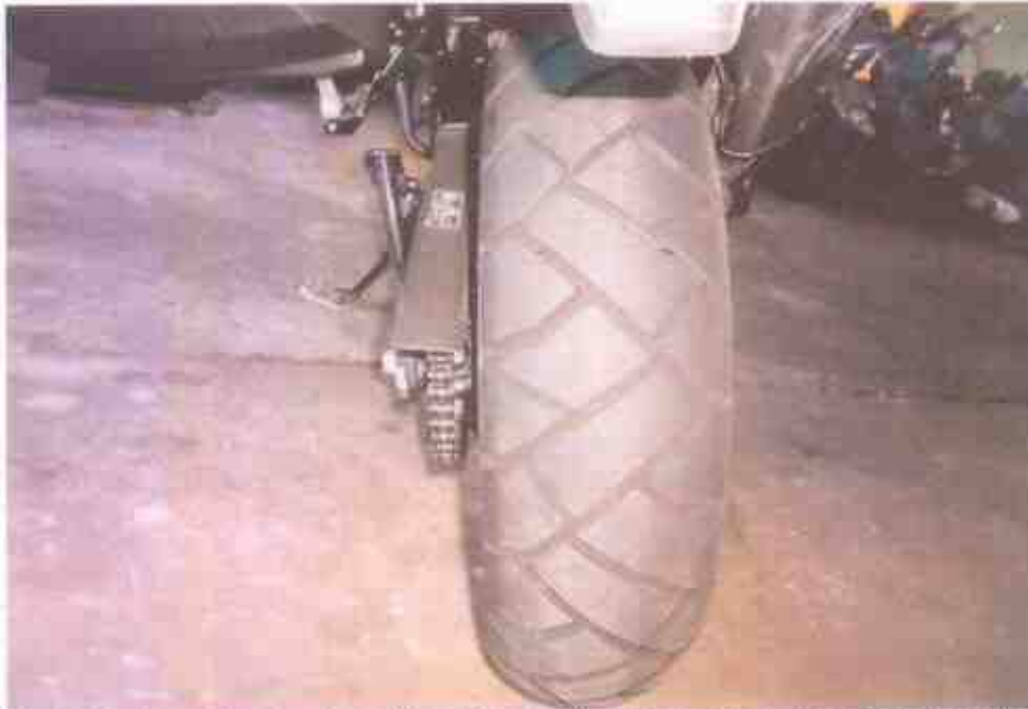
Photo 9 shows the rear tyre of the Motorcycle. The rear tyre was observed to be in serviceable condition with remaining tread depth of approximately 7mm. The tyre was also observed to be sufficiently inflated for vehicular operation.
