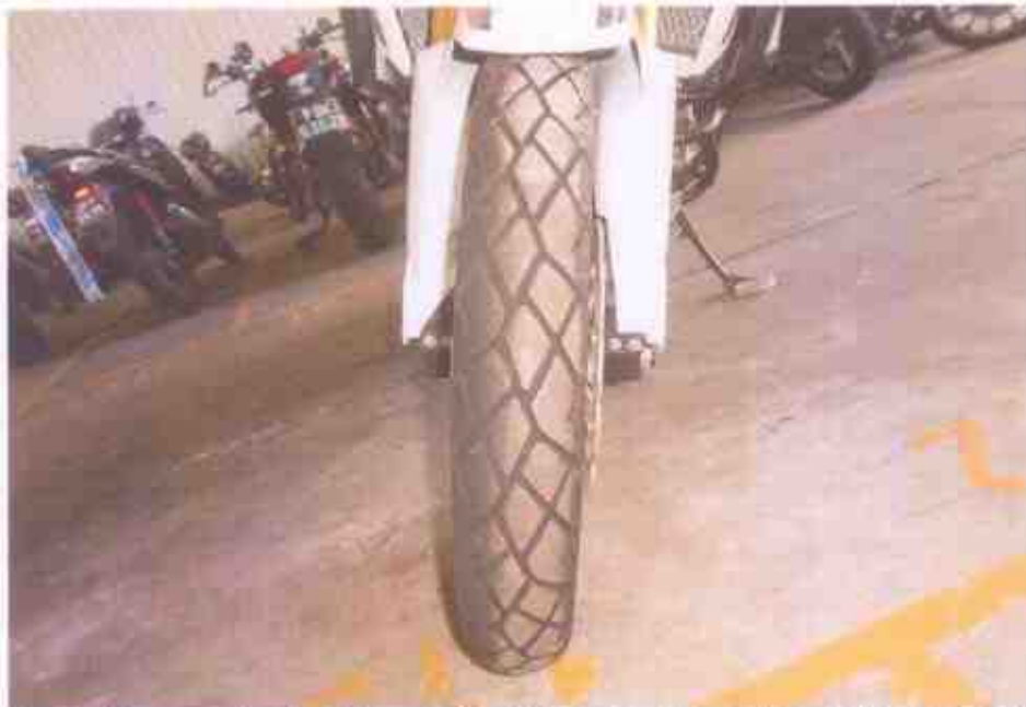
Photo 10 shows the front tyre of the Motorcycle. The pattern of the tread was clearly visible with remaining tread depth of approximately 7mm. There was no tear, burst mark(s) and/or punctured hole(s) on the sidewalls as well as across the tread of the front tyre.
