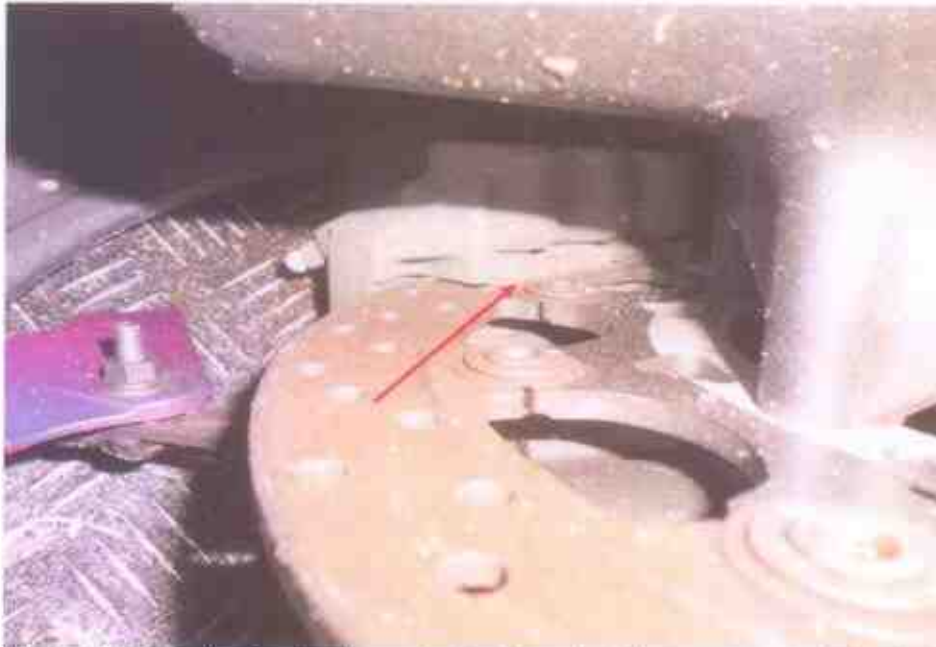
Photo 19 shows the front brake pad, which is part of the components in the front brake system of the Motorcycle. Our visual checks had revealed that it was still in serviceable condition, intact with no visible damage & sufficient frictional padding.
