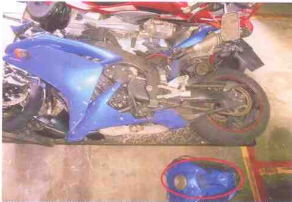
Photo 6 shows a close-up view of the frontal portion of the Motorcycle at the time of our inspection. The Motorcycle was observed to have sustained relatively extensive impact including damages to the fuel tank due to the accident collision.
