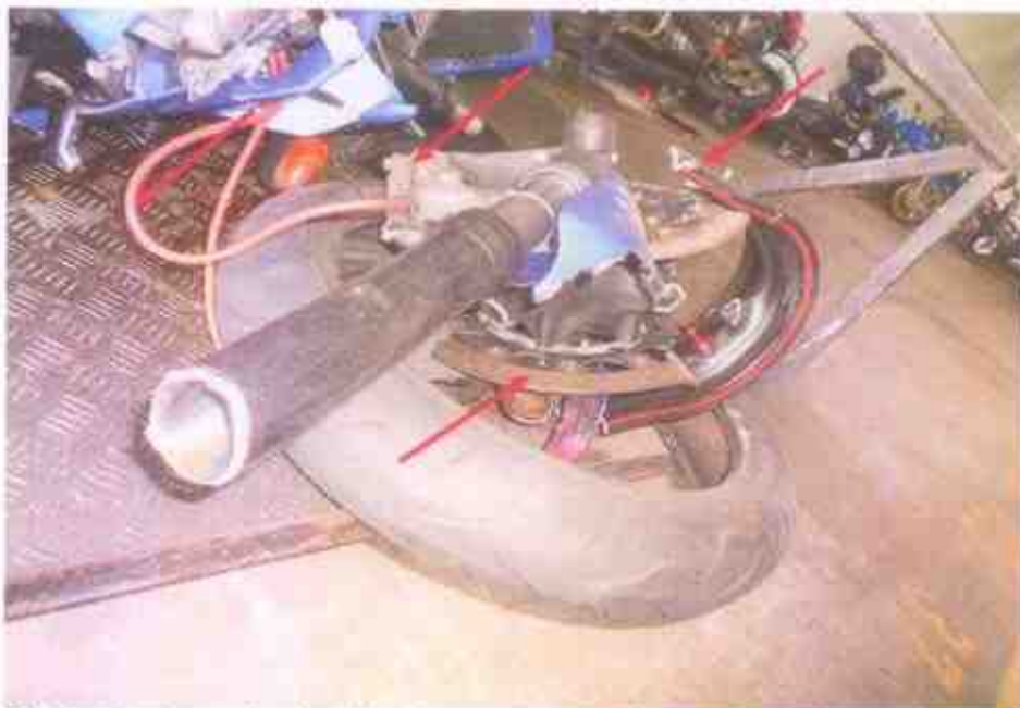
Photo 16 shows the front brake components (arrowed) was observed to be crushed as a result of the accident. Hence, we are unable to conduct any tests on the braking system of the Motorcycle.
