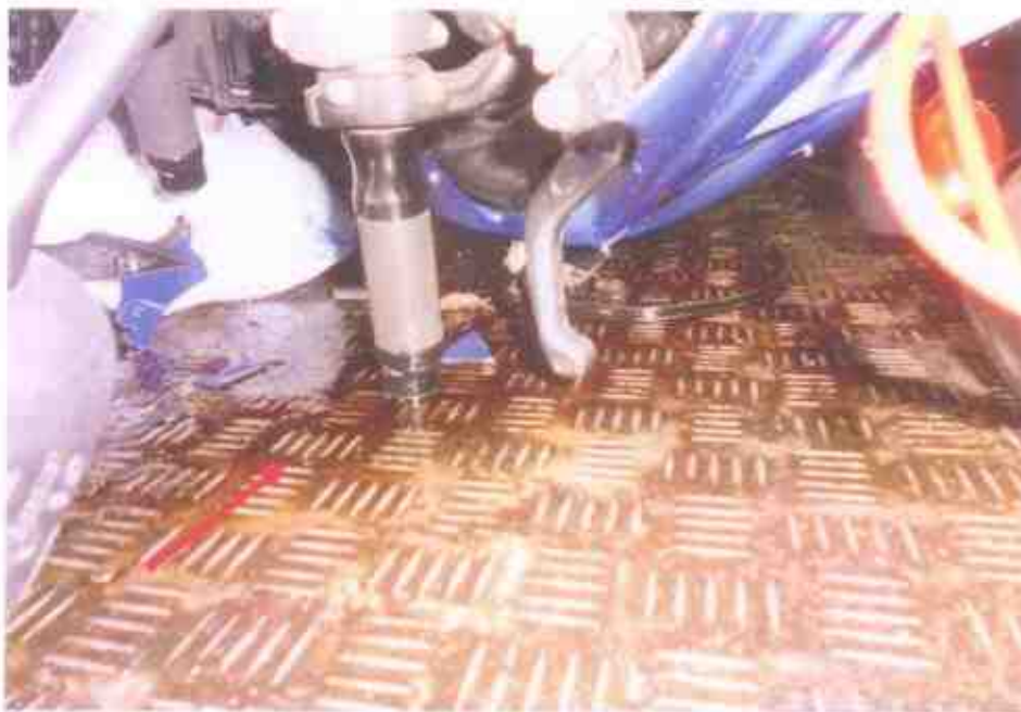
Photo 11 shows sign(s) or indication(s) of fluid leakage observed on the floor around the engine's underside area of the Motorcycle.
