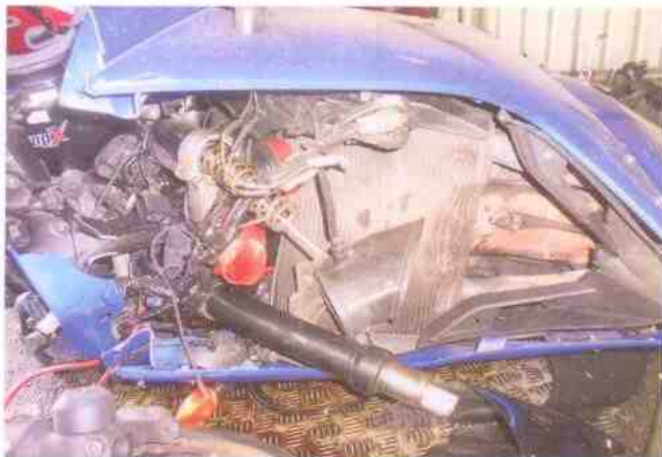
Photo 7 shows a close-up view of the front portion of the Motorcycle at the time of our inspection. The Motorcycle engine components such as radiator, front fork & other components were observed to have sustained relatively extensive impact due to the accident collision.
