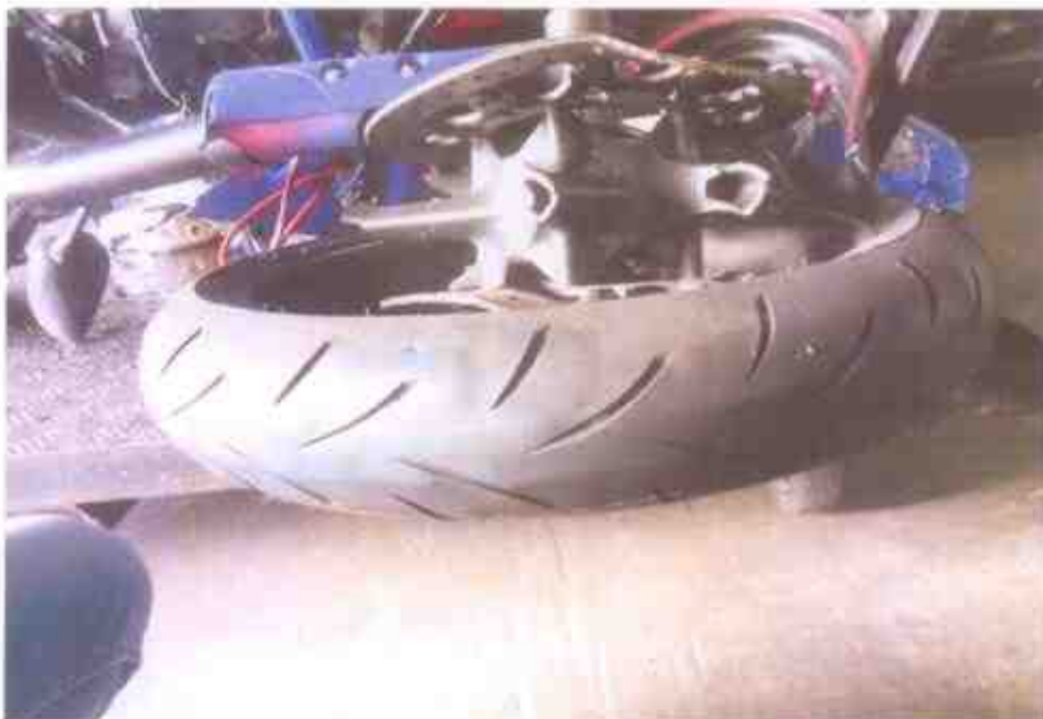
Photo 9 shows the front tyre of the Motorcycle and the tread pattern was clearly visible. There was no tear, burst mark(s) and/or punctured hole(s) on the sidewalls as well as across the tread of the front tyre with remaining tread depth of approximately 4mm. However, the wheel rim was observed to be broken & the tyre was dislodged from the wheel rim as a result of the accident.
