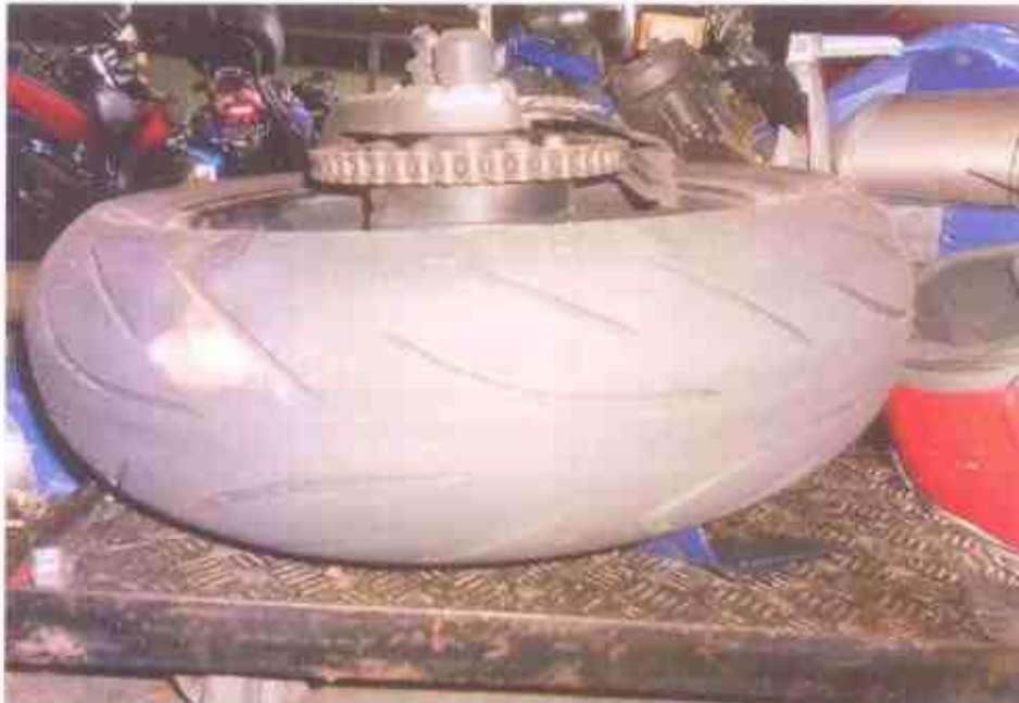
Photo 8 shows the rear tyre of the Motorcycle at the time of our inspection. The rear tyre was observed to be in serviceable condition with remaining tread depth of approximately 3mm. The tyre was also observed to be sufficiently inflated for vehicular operation. There was no significant damage observed on the rear wheel rim & tyre.
