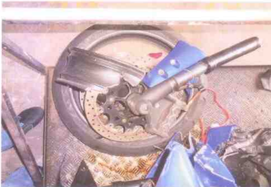
Photo 10 shows the cracked wheel rim on front tyre of the Motorcycle at the time of our inspection.
