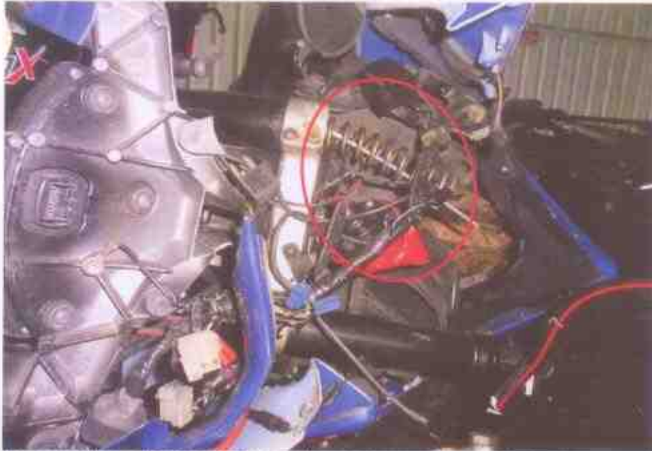
Photo 17 shows the front fork (circled) was observed to be dislodged as a result of the accident. Hence, we are unable to conduct any tests on the steering system of the Motorcycle.
