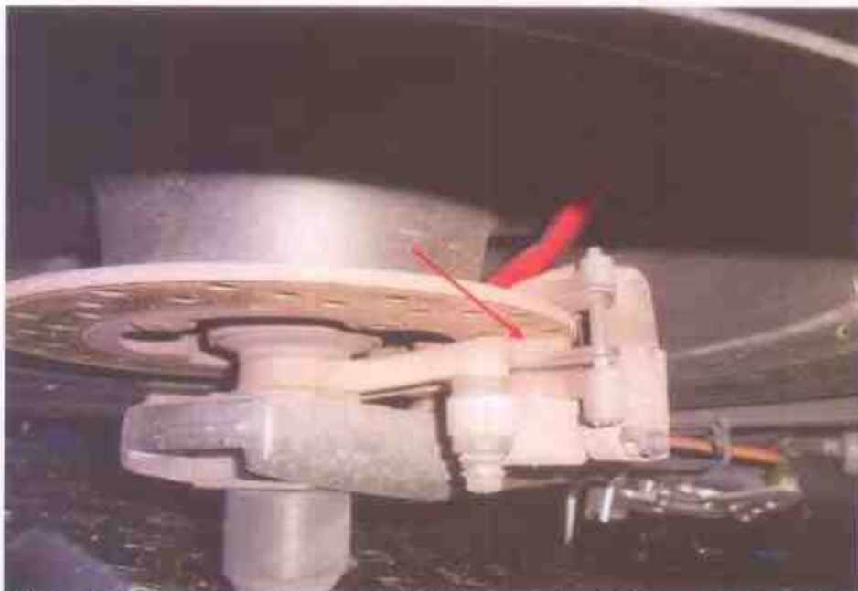
Photo 20 shows the rear brake pad of the Motorcycle which was observed to be in serviceable condition. No damages were found at time of our inspection to the rear braking components.
