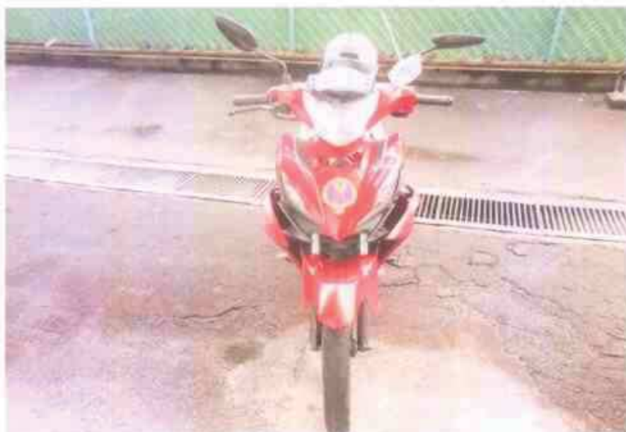
Photo 2 shows a general view of the front body of the Motorcycle at the time of our inspection. The Motorcycle was observed to have sustained relatively minor damages at time of inspection. The damages were observed to be confined to its left & right side of the front fairing.
