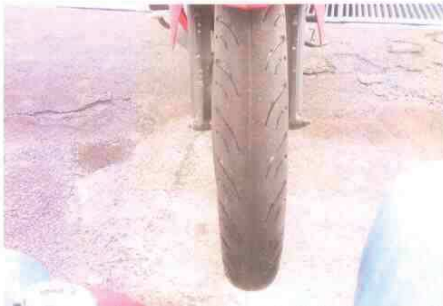
Photo 9 shows the front tyre of the Motorcycle. The front tyre was observed to be in serviceable condition with remaining tread depth of approximately 3mm. The tyre was also observed to be sufficiently inflated for vehicular operation.
