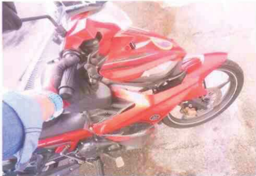
Photo 16 shows testing of the braking of the front brake in progress. There was some resistance felt (spongy like feel) upon pressing the brake lever.
