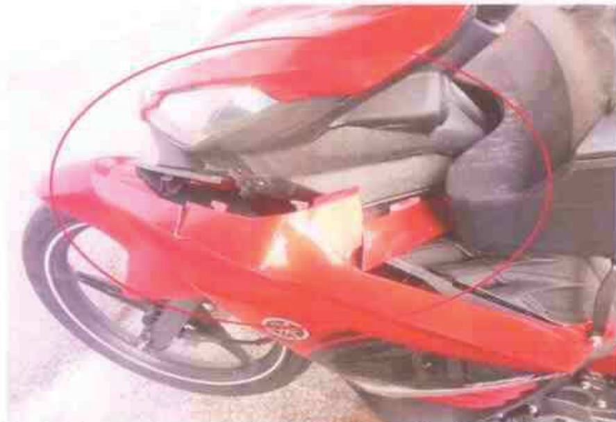
Photo 6 shows a closer view of the front left fairing of the Motorcycle at the time of our inspection. The Motorcycle was observed to have sustained with relatively minor damages due to the accident collision. (Circled)
