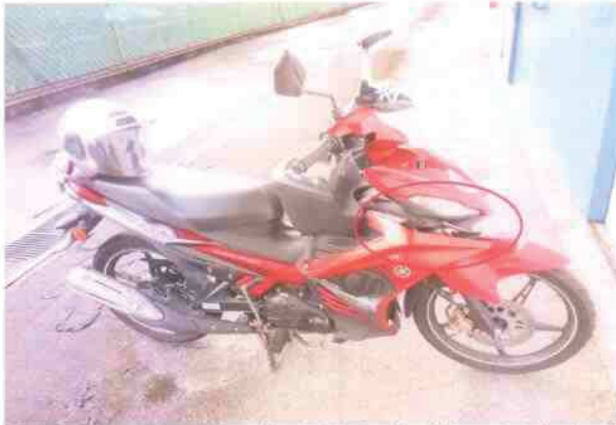
Photo 3 shows a general view of the right body of the Motorcycle at the time of our inspection. The Motorcycle was observed to have sustained relatively minor damages on the right side fairing at time of our inspection.
