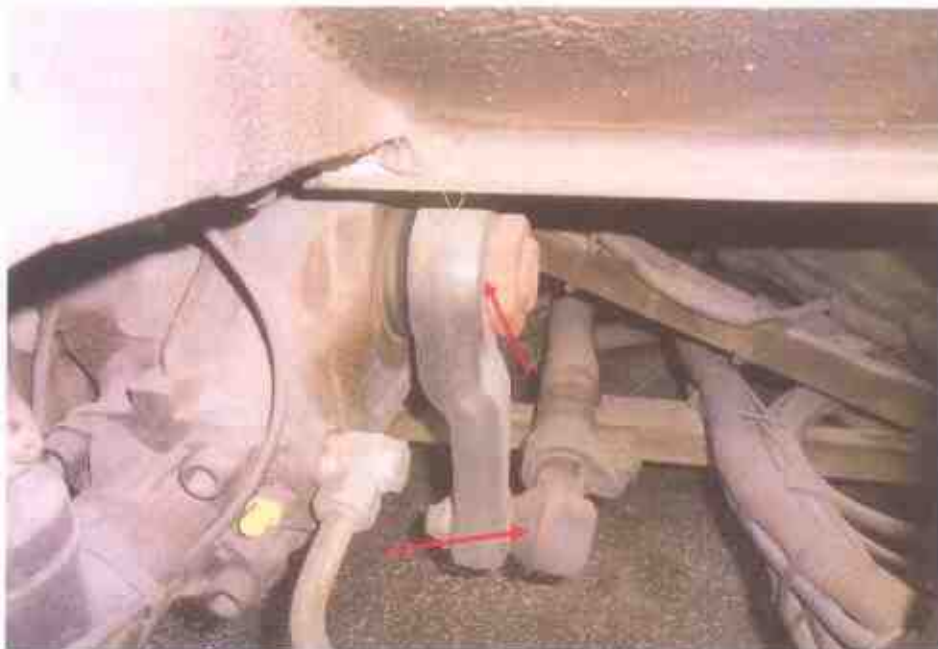
Photo 17 shows some of the mechanical components (arrowed) of the Motor Bus's steering system. Our visual check on the various mechanical components of the steering system revealed all to be intact and in good condition. The steering system of the Motor Bus likely to be in serviceable condition at the time of accident.
