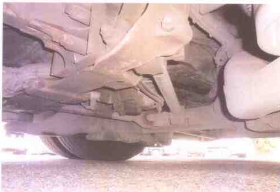
Photo 12 shows the engine undercarriage of the Motor Bus. Some pre-existed fluid was observed at time of our inspection.
