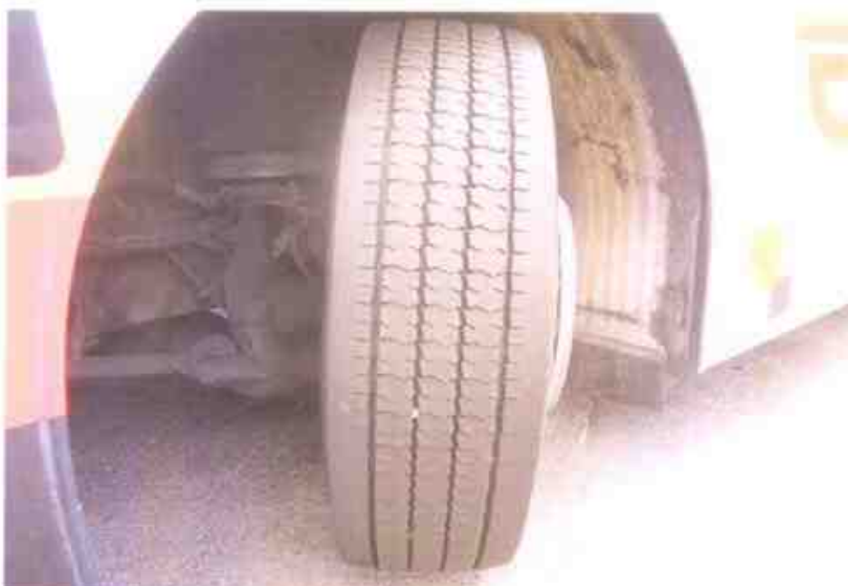
Photo 8 shows the condition of the front left tyre of the Motor Bus, which was observed to be in serviceable condition with remaining tread depth of approximately 9mm. The tyre was also observed to be sufficiently inflated for vehicular operation.
