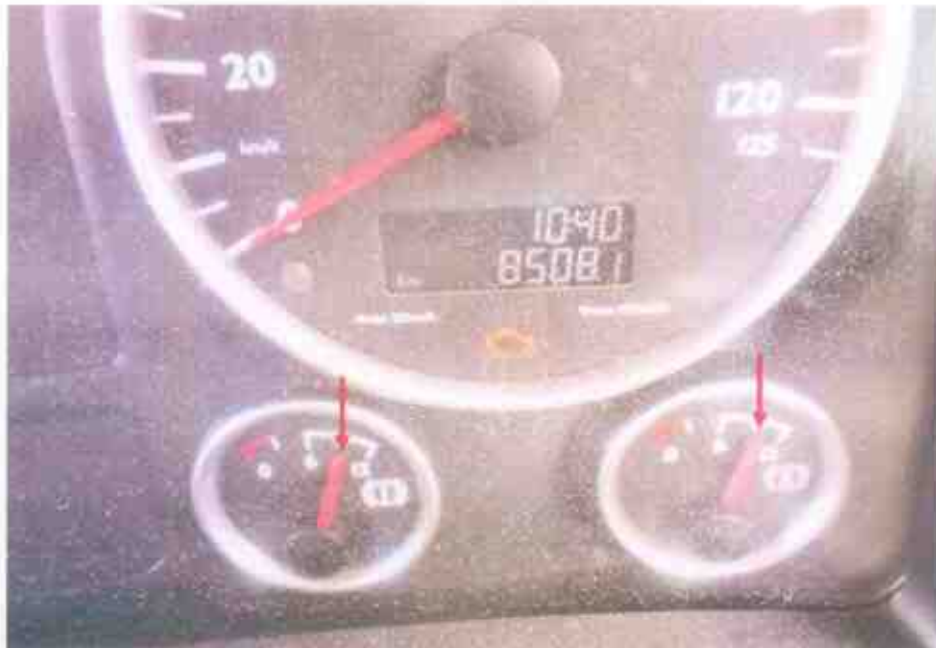
Photo 19 shows pressure tank 1 & tank 2 were observed to be pressurised up to 10bars after the engine start-up. No drop in the pressure after a few minutes which means there's no air leakage from the air-braking system.
