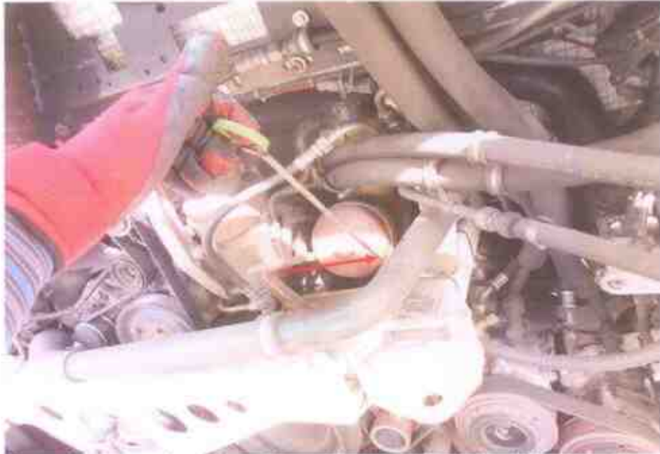
Photo 15 shows the engine fluid on the dip stick of the Motor Bus. It was observed to be of sufficient level without any contamination at time of our inspection.
