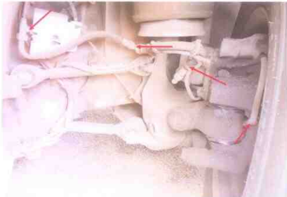
Photo 21 shows some of the mechanical components (arrowed) of the Motor Bus's braking system. Our visual check on the various mechanical components revealed all to be intact and in good condition. It was in serviceable condition at the time of accident.
