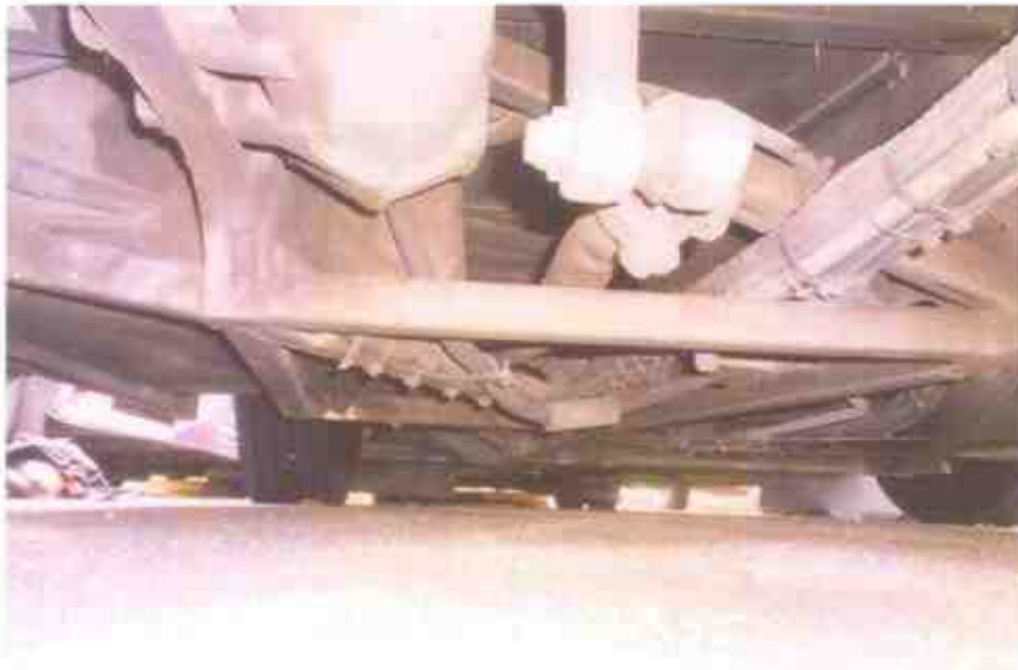
Photo 18 shows the undercarriage components from front to rear steering system of the Motor Bus. The various undercarriage components of the Motor Bus were all observed to be intact and without any visible damage. This had included the transmission system of the Motor Bus, which were observed to be securely attached to the rear wheels.
