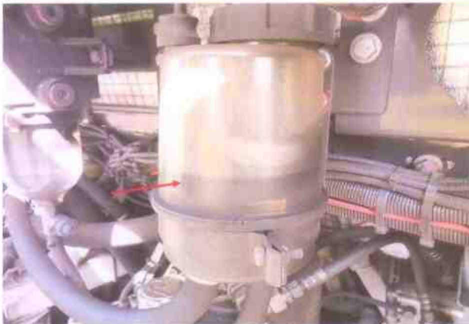
Photo 13 shows the steering fluid of the Motor Bus. It was observed to be of sufficient level without any contamination at time of our inspection.
