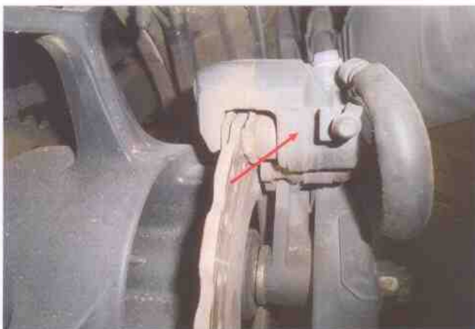
Photo 19 shows the rear wheel of the Motorcycle. The type of brake system for the rear wheel was of hydraulic type, controlled by the brake foot pedal of the Motorcycle. Our checks of the calliper (arrowed) & brake pad which are all part of the components in the rear brake system of the Motorcycle reveal all to be intact and without damage.
