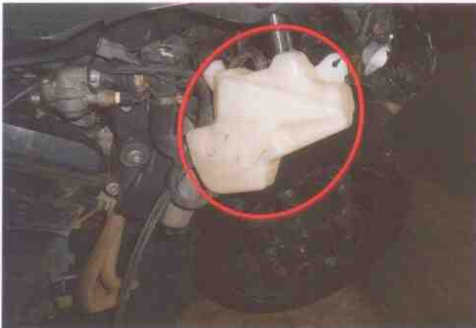
Photo 8 shows a close-up view of the dislodged coolant reservoir of the Motorcycle at the time of our inspection. It was observed to have sustained with damages due to the accident collision.
