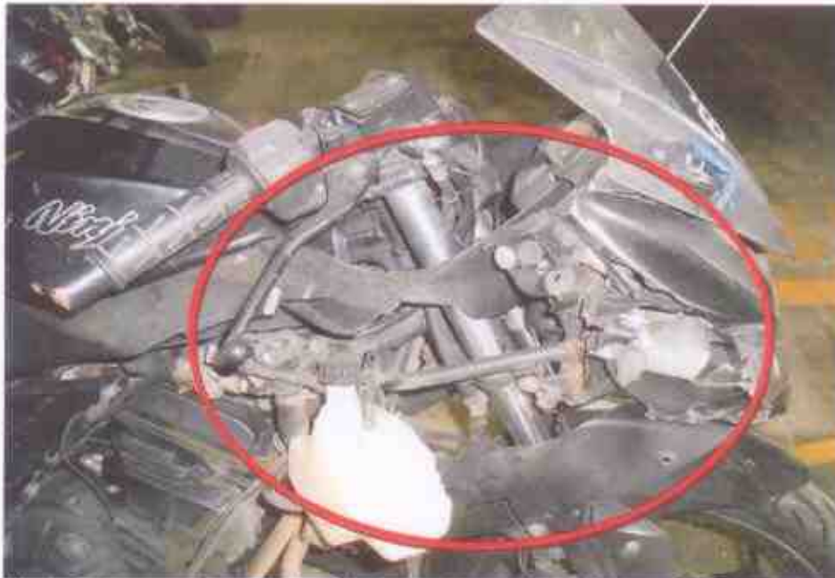
Photo 5 shows a close-up view of the head lamp & side fairing of the Motorcycle at the time of our inspection. It was observed to have sustained with damages due to the accident collision.
