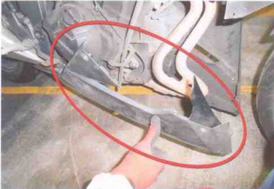
Photo 7 shows a close-up view of the side fairing of the Motorcycle at the time of our inspection. It was observed to have sustained with damages due to the accident collision.
