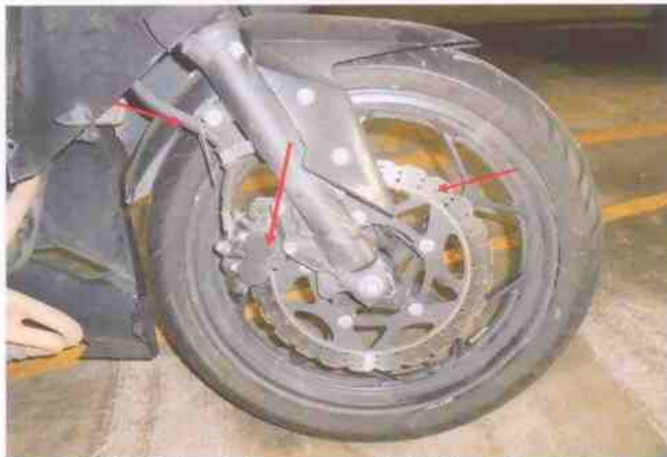
Photo 17 shows the front brake calliper, front brake disc and front brake hose of the Motorcycle (arrowed), which are all part of the components in the front brake system of the Motorcycle. Our visual checks of these various components had revealed all to be intact with no visible damage. No leakage of brake fluid was also observed.
