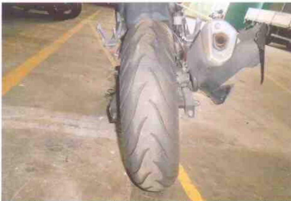
Photo 9 shows the rear tyre of the Motorcycle at the time of our inspection. The rear tyre was observed to be in serviceable condition with remaining tread depth of approximately 3mm. The tyre was also observed to be sufficiently inflated for vehicular operation. There was no significant damage observed on the rear wheel rim & tyre.
