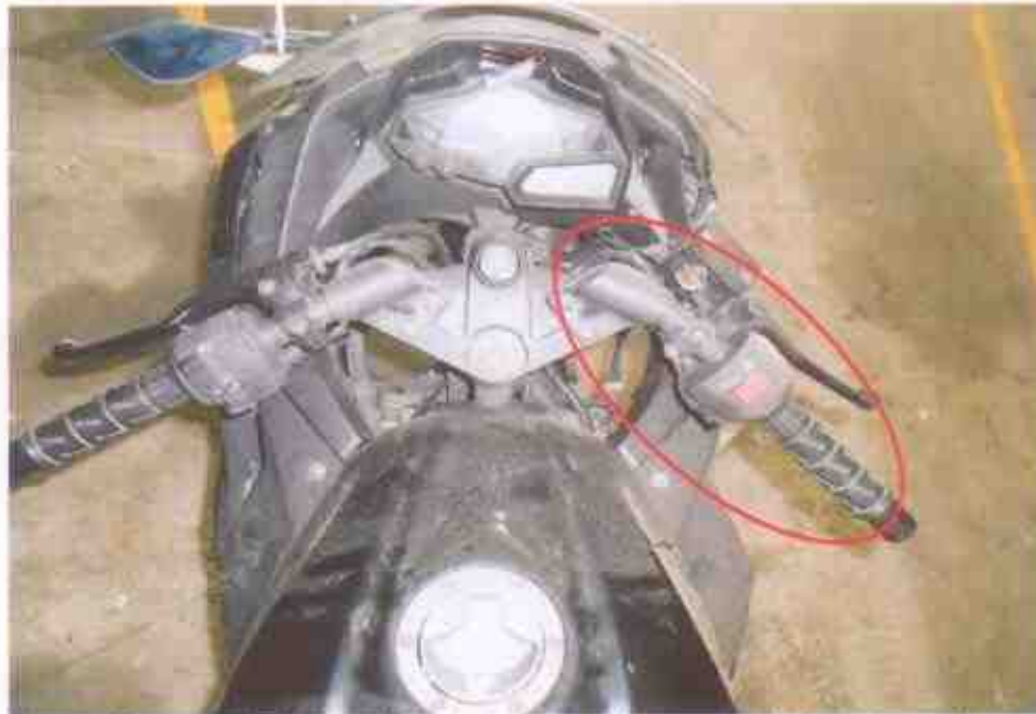
Photo 16 shows the handle bar (circled) was observed to be bent inwards as a result of the accident. Hence, we are not able to conduct any tests on the steering system of the Motorcycle.
