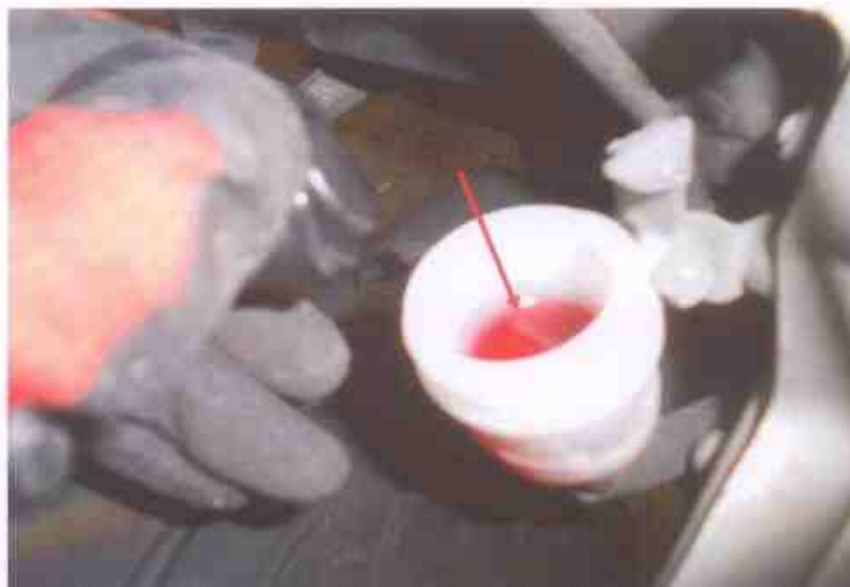
Photo 20 shows the rear brake fluid reservoir of the Motorcycle. It was observed to be of sufficient level without any contamination at time of our inspection.
