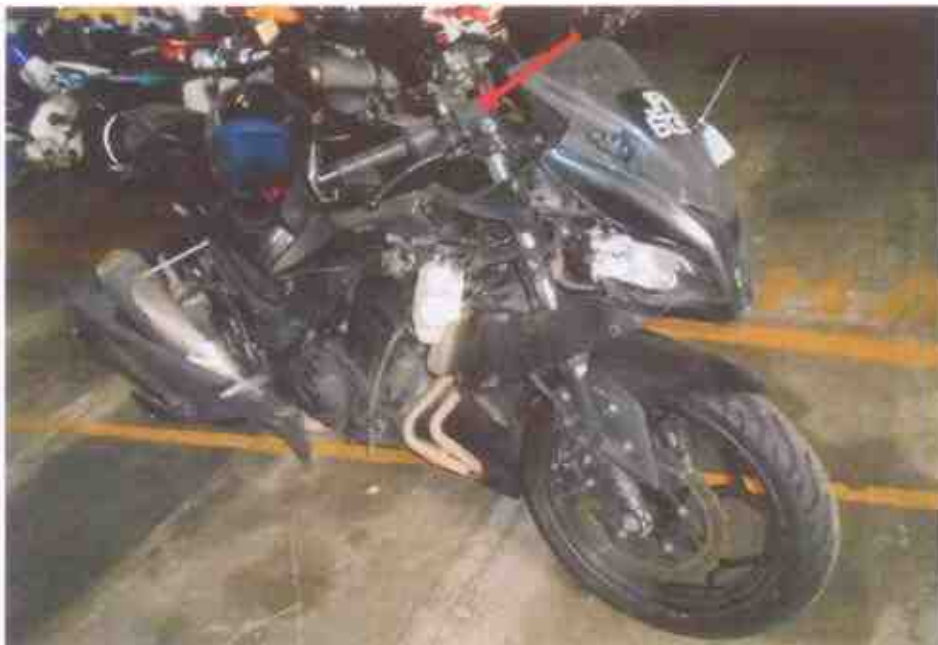
Photo 2 shows a general view of the front right body of the Motorcycle at the time of our inspection. The Motorcycle was observed to be sustained with relatively extensive impact due to the accident collision. Amongst the body parts damaged was its handle bar-steering system (arrowed), which was observed to be bent inwards.
