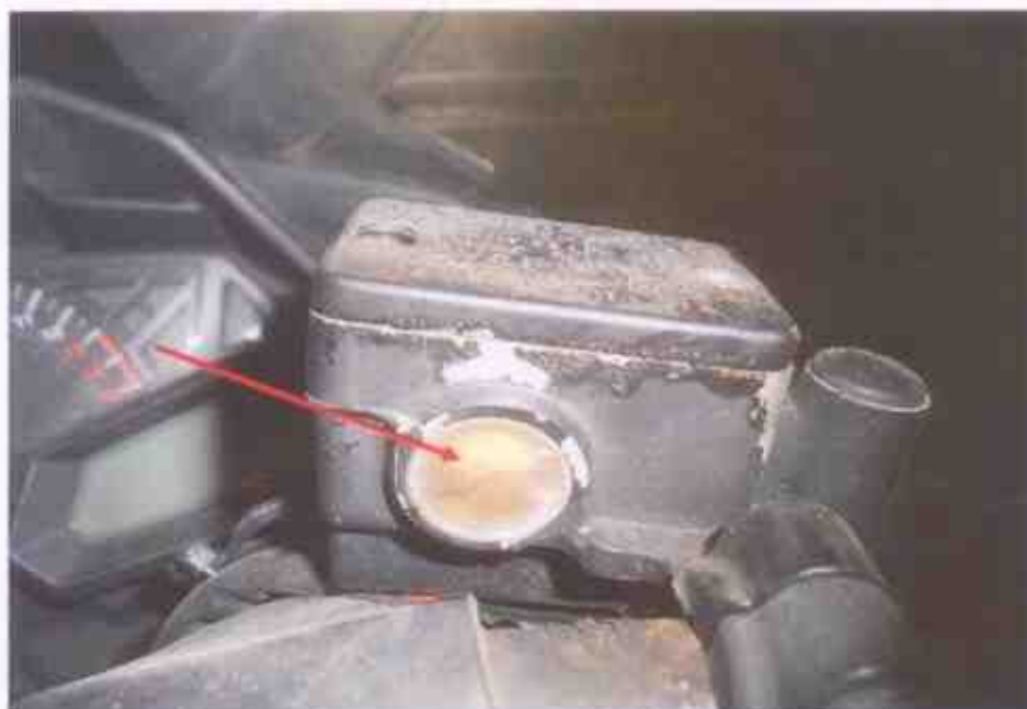
Photo 21 shows the front brake fluid reservoir of the Motorcycle. It was observed to be of sufficient level without any contamination at time of our inspection.
