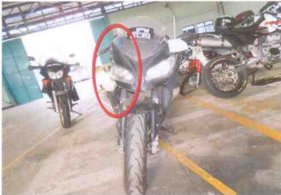
Photo 1 shows a general view of the front body of the Motorcycle at the time of our inspection. The Motorcycle was observed to be sustained with relatively extensive impact due to the accident collision. Amongst the body parts damaged was its steering system (circled), which was observed to be bent inwards.
