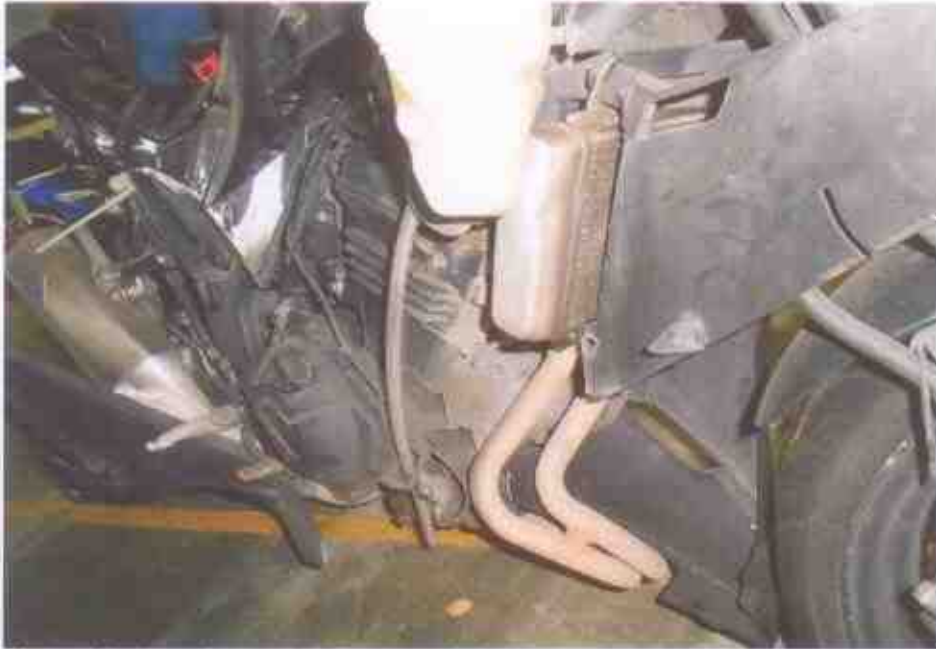
Photo 12 shows the semi-close view of the engine compartment. It was observed to be intact & undamaged unaffected by the accident's impact.
