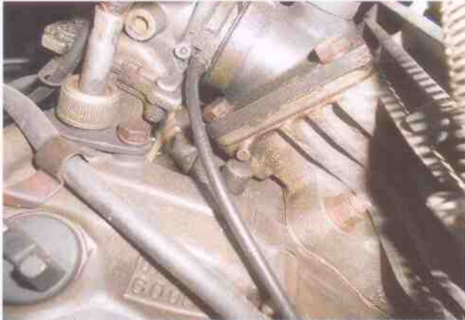
Photo 14 shows sign(s) or indication(s) of fluid leakage observed around the engine's area of the Motorcycle.
