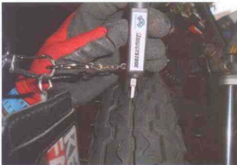
Photo 11 shows the front tyre of the Motorcycle at the time of our inspection. The pattern of the tread was measured and found to be around 4mm & the thread was clearly visible.
