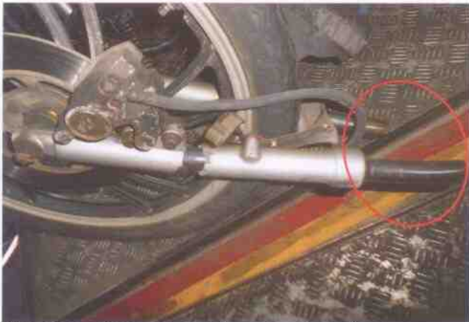
Photo 19 shows the front fork (circled) was observed to be dislodged as a result of the accident. Hence, we are unable to conduct any tests on the steering system of the Motorcycle.
