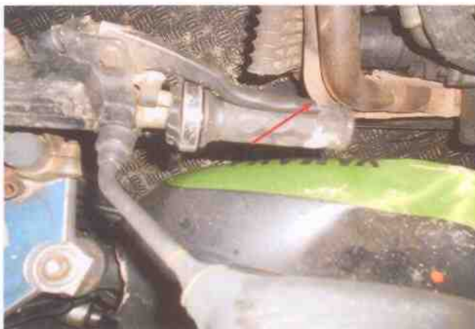
Photo 17 shows the hand brake lever (arrowed) was observed to be broken due to the result of the accident. Hence, we are unable to conduct any tests on the braking system of the Motorcycle.
