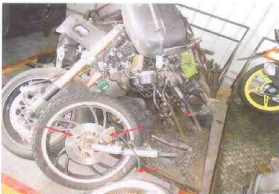
Photo 20 shows the front brake calliper and front brake disc of the Motorcycle (arrowed in red), which are all part of the components in the front brake system of the Motorcycle. Our visual checks of these various components had revealed all to be intact with no visible damage except for a cut brake fluid hose due to the accident.
