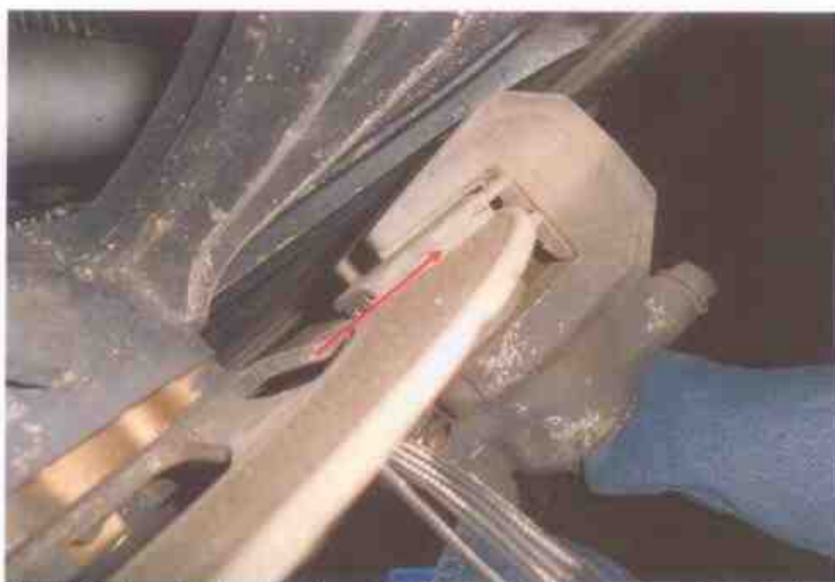
Photo 21 shows the front brake pad, which is part of the components in the front brake system of the Motorcycle. Our visual checks had revealed that it was still in serviceable condition, intact with no visible damage & sufficient frictional padding.
