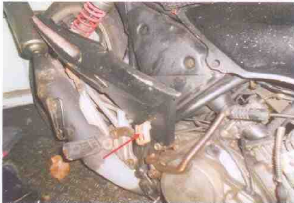
Photo 18 shows the rear brake pedal (arrowed) was observed to be crushed inwards as a result of the accident. Hence, we are unable to conduct any tests on the braking system of the Motorcycle.
