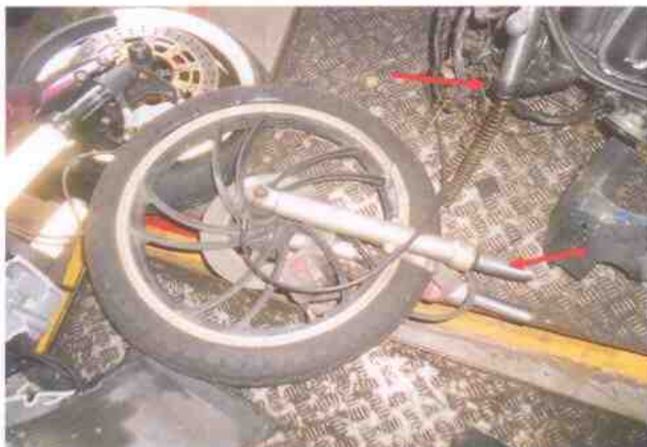
Photo 3 shows a general view of the front right body of the Motorcycle at the time of our inspection. The Motorcycle was observed to have sustained with relatively extensive impact due to the accident collision. Amongst the body parts damaged was its front fork (arrowed), which was observed to be broken into 2 pieces.
