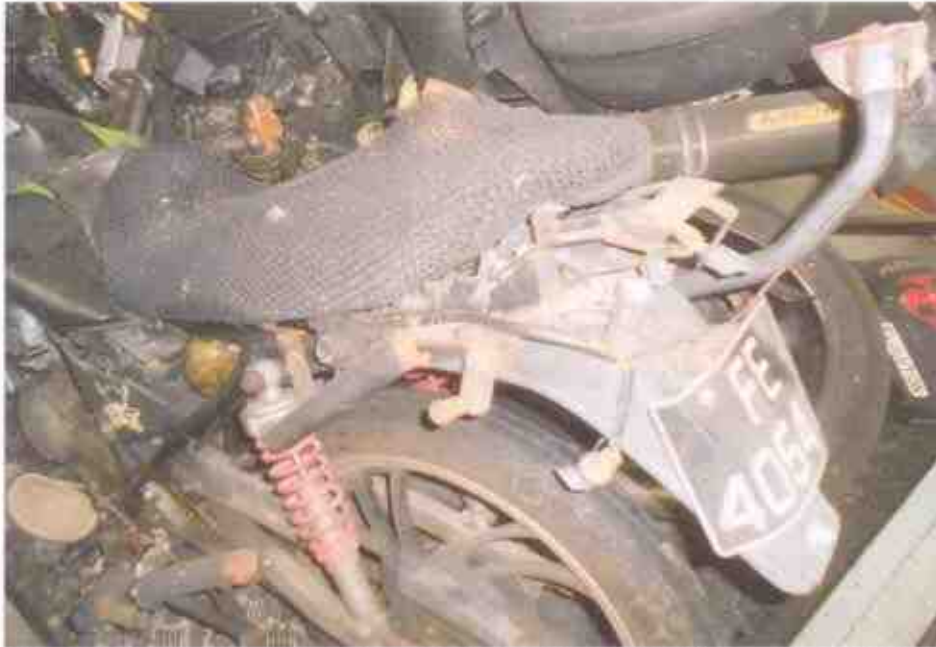
Photo 7 shows a close-up view of the rear portion of the Motorcycle at the time of our inspection. The Motorcycle was observed to have sustained relatively extensive impact due to the accident collision.
