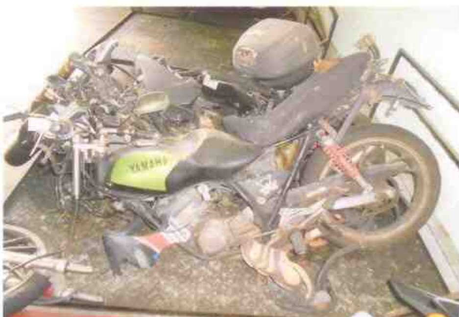
Photo 4 shows a general view of the rear left body of the Motorcycle at the time of our inspection. The Motorcycle was observed to have sustained damages at the frontal portion, rear portion, along both its left side and right side.
