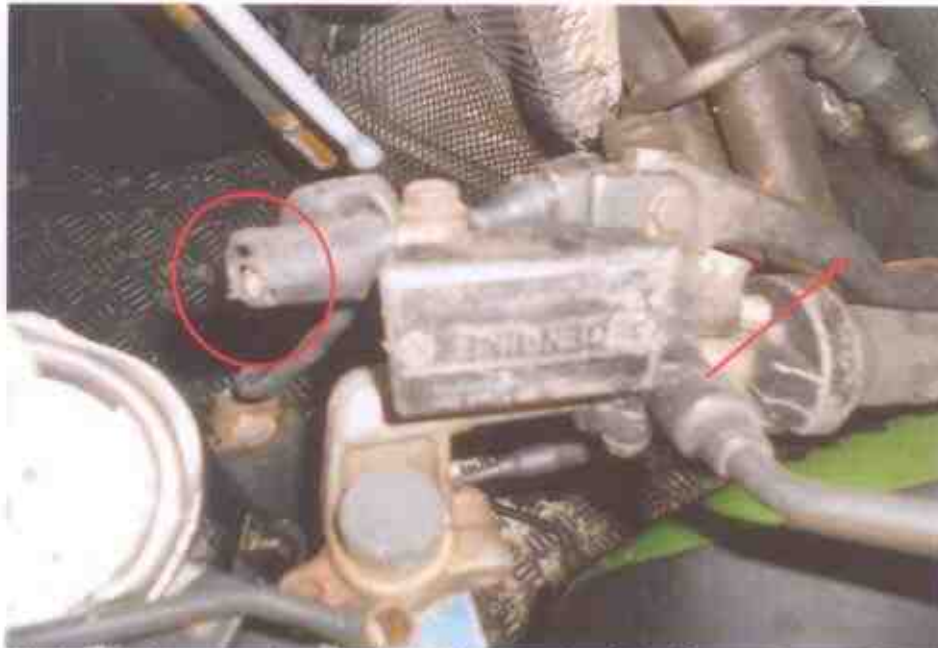
Photo 22 shows the front brake fluid reservoir of the Motorcycle which was observed to be with cut brake fluid hose & damaged brake lever caused by the accident's collision.
