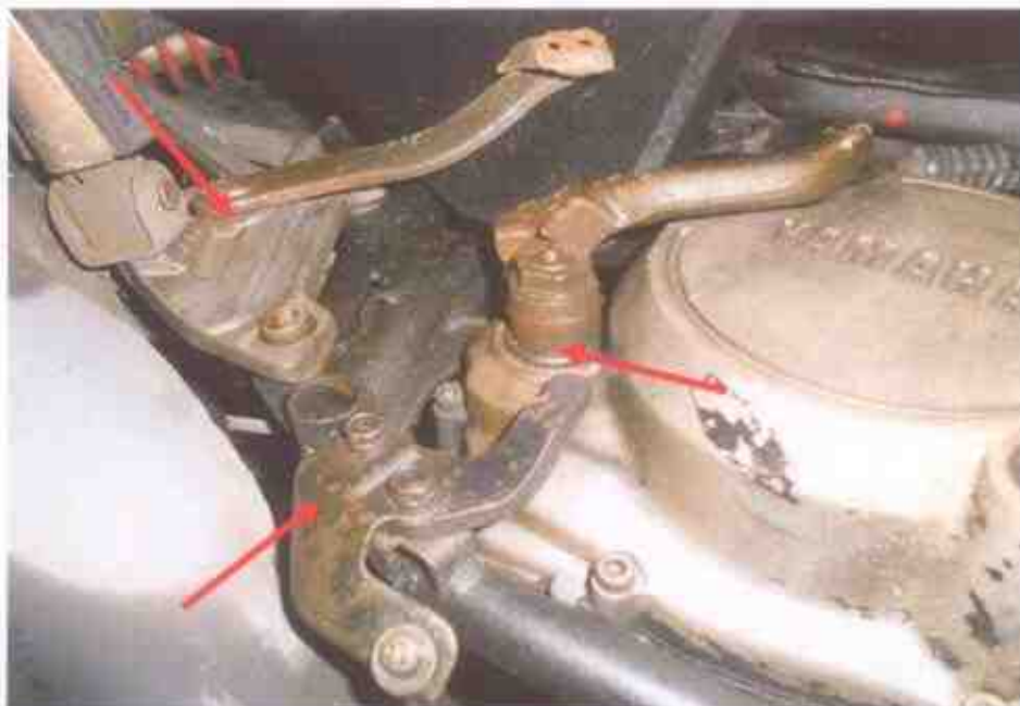
Photo 13 shows sign(s) or indication(s) of fluid leakage observed around the engine's underside area of the Motorcycle.
