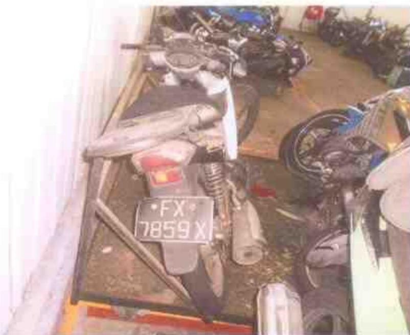
Photo 3 shows a general view of the rear left body of the Motorcycle at the time of our inspection. The Motorcycle was observed to have sustained minor damages at the rear portion as a result of the accident.
