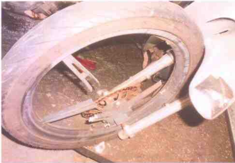
Photo 5 shows the front tyre of the Motorcycle at the time of our inspection. The front tyre was observed to be in serviceable condition with remaining tread depth of approximately 2mm. However, the wheel rim was observed to be broken into several pieces due to the accident's impact collision.
