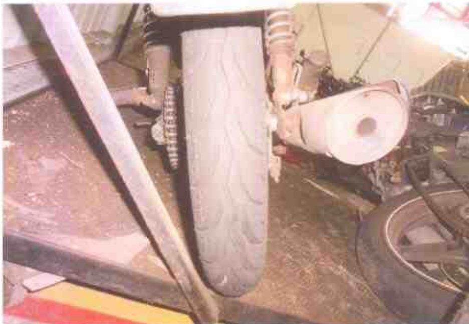
Photo 6 shows the rear tyre of the Motorcycle. The pattern of the tread was clearly visible. There was no tear, burst mark(s) and/or punctured hole(s) on the sidewalls as well as across the tread of the front tyre. The front tyre was observed to be in serviceable condition with remaining tread depth of approximately 4mm.
