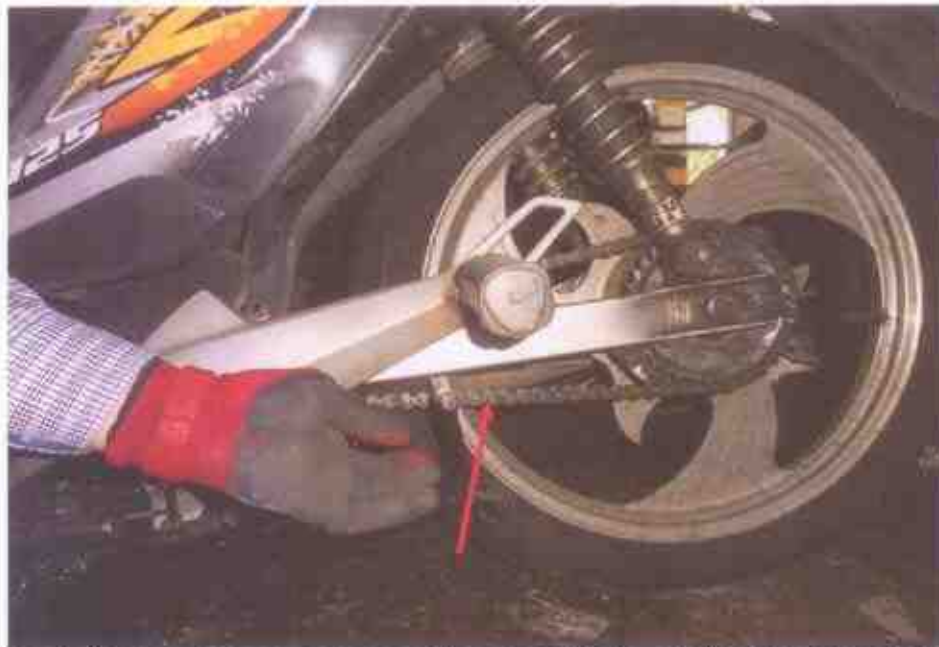
Photo 9 shows the general view of the gear train (arrowed) of the Motorcycle, which was observed to be intact with no misalignment. It was also adequately lubricated for operating purposes. Free play tension was also observed & found adequately acceptable.
