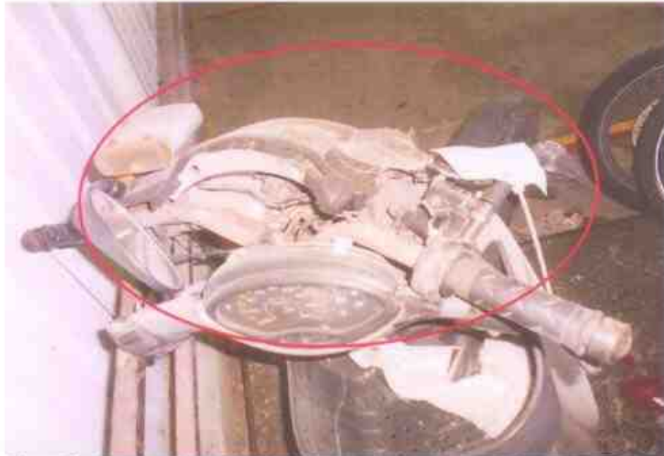
Photo 10 shows the front fork (circled) was observed to be dislocated as a result of the accident. Hence, we are not able to conduct any tests on the steering system of the Motorcycle.
