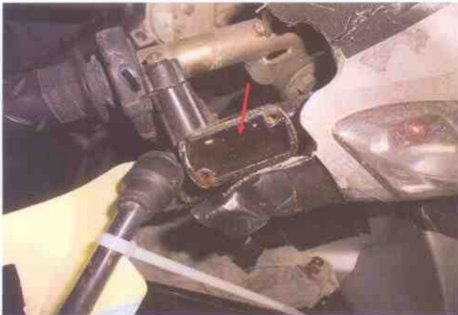
Photo 13 shows the front brake fluid reservoir that was found to be sufficient level despite broken hand brake lever due to the accident.
