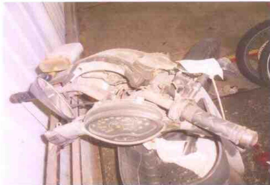
Photo 4 shows a general view of the dislodged speedometer, dislocated handle bar & damaged wing mirrors of the Motorcycle at the time of our inspection. The Motorcycle was observed to be sustained with relatively extensive impact due to the accident collision.
