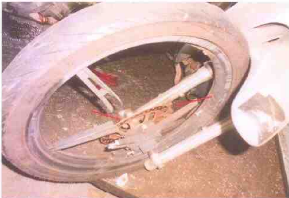
Photo 11 shows the front brake calliper, front brake disc and front brake hose of the Motorcycle, which are all part of the components in the front brake system of the Motorcycle. Our further observation had revealed that it was not affected although damages found on the wheel rim.
