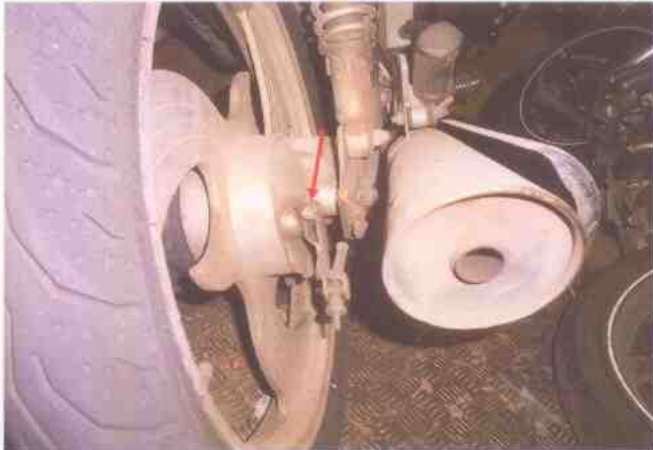
Photo 12 shows the rear brake of the Motorcycle. It was found to be unaffected by the accident.
