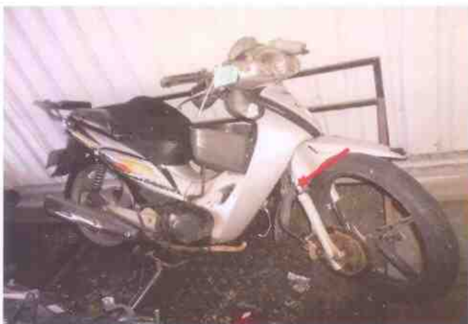
Photo 2 shows a general view of the front right body of the Motorcycle at the time of our inspection. The Motorcycle was observed to be sustained with relatively extensive impact due to the accident collision. Amongst the body parts damaged was its front fork (arrowed), which was observed to be dislocated.
