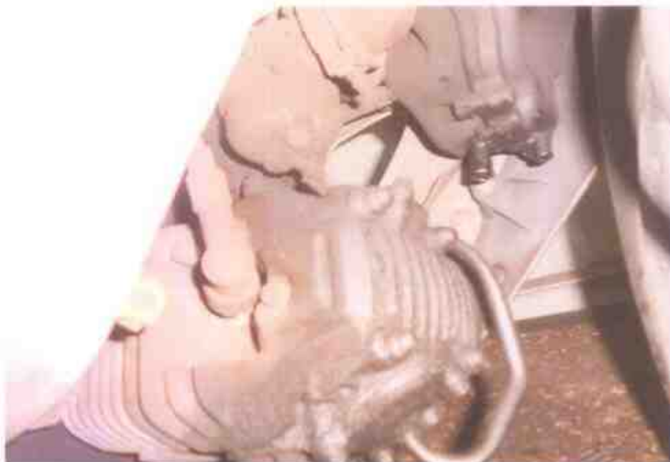
Photo 7 shows sign(s) or indication(s) of fluid leakage stain observed around the engine undercarriage area of the Motorcycle.
