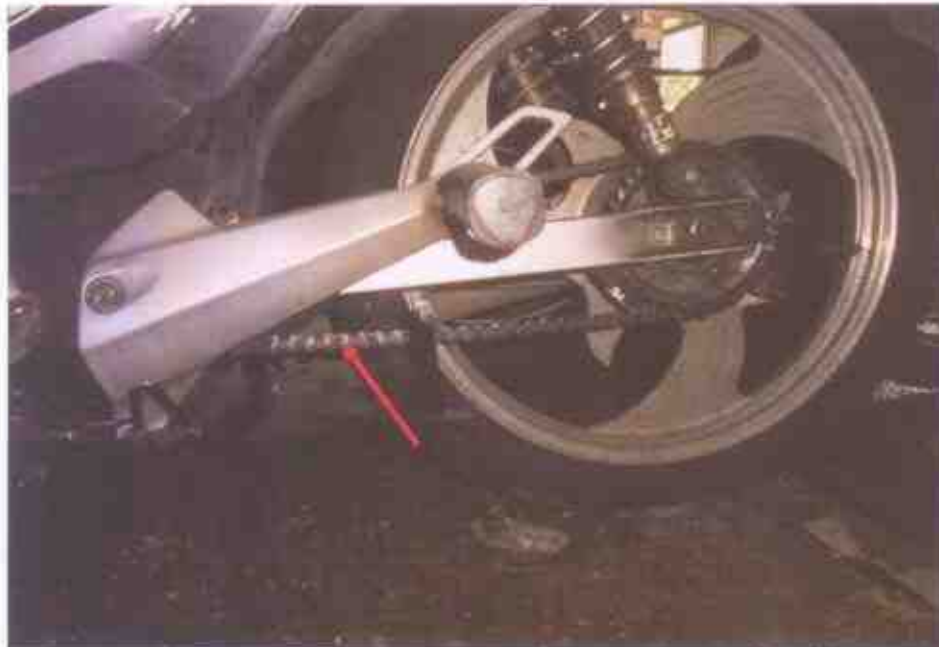
Photo 8 shows the general view of the gear train (arrowed) of the Motorcycle, which was observed to be intact with no misalignment. It was also adequately lubricated for operating purposes.
