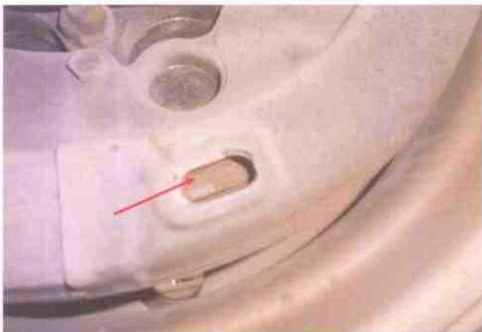
Photo 19 shows the brake shoes (brake pads) at the rear wheels of the Motor Lorry revealed that the brake shoes (brake pads) were in serviceable condition with sufficient frictional material for operational purposes.
