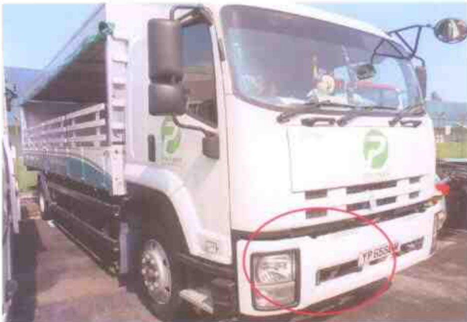
Photo 6 shows a general view of the front right portion of the Motor Lorry at the time of our inspection. The Motor Lorry was observed to have sustained minor impact at its front right bumper. Only stain marks was observed on the front right bumper as a result of the accident.
