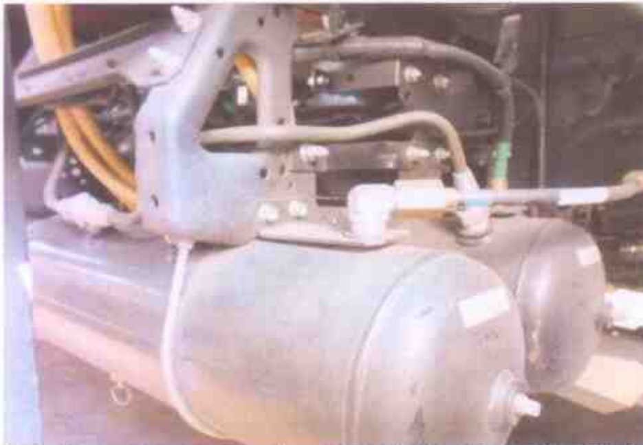
Photo 20 shows the air pressure tank of the Motor Lorry. It was observed to be unaffected by the accident. No air leakage was found at time of our inspection.
