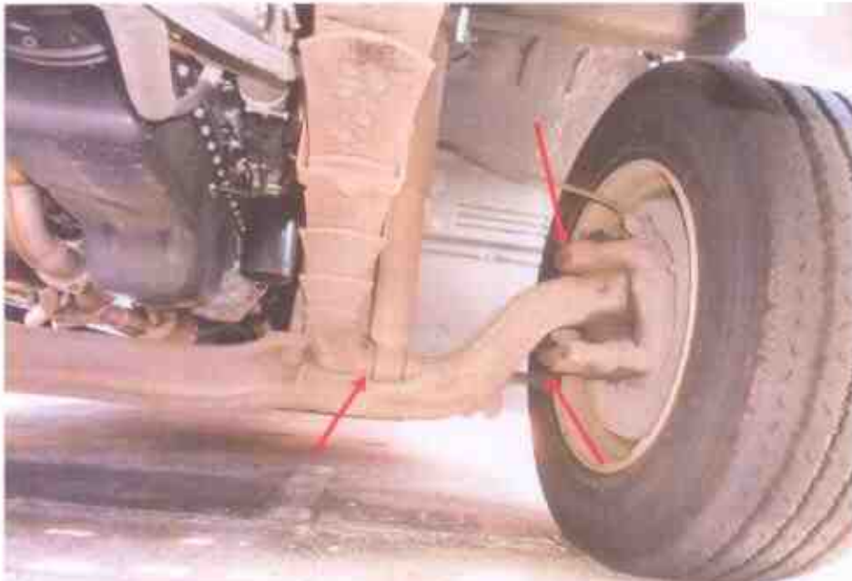
Photo 16 shows the various undercarriage components at the front left wheel of the Motor Lorry, in particular the steering tie rod end (arrowed). The various undercarriage components of the Motor Lorry were all found to be intact without any visible damage. There was also no sign of fluid stain(s) observed on the various undercarriage components.
