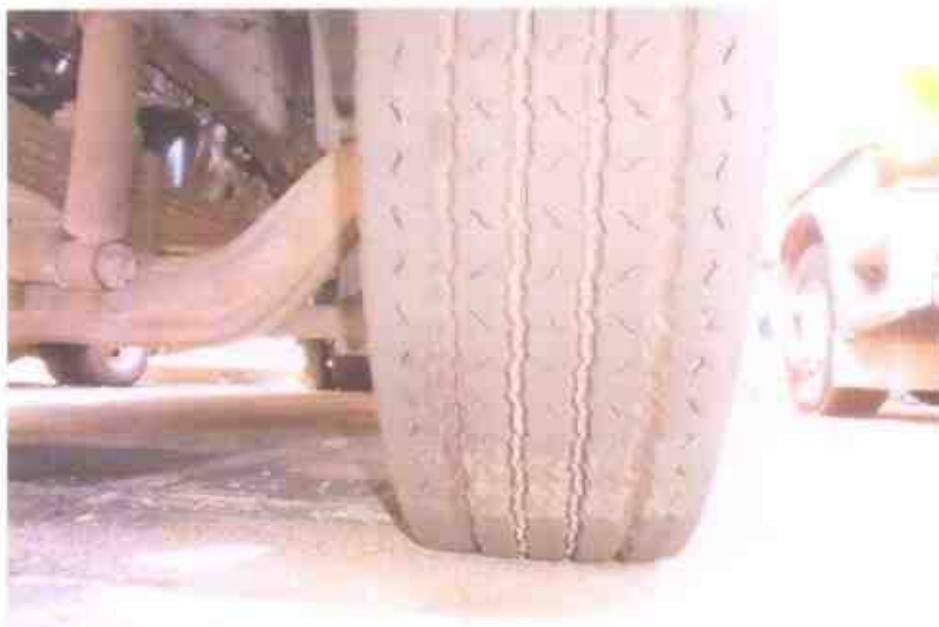
Photo 8 shows the condition of the front left tyre of the Motor Lorry, which was observed to be in serviceable condition with remaining tread depth of approximately 7mm. The tyre, which was wrapped around standard alloy wheel rim, was also observed to be sufficiently inflated for vehicular operation.
