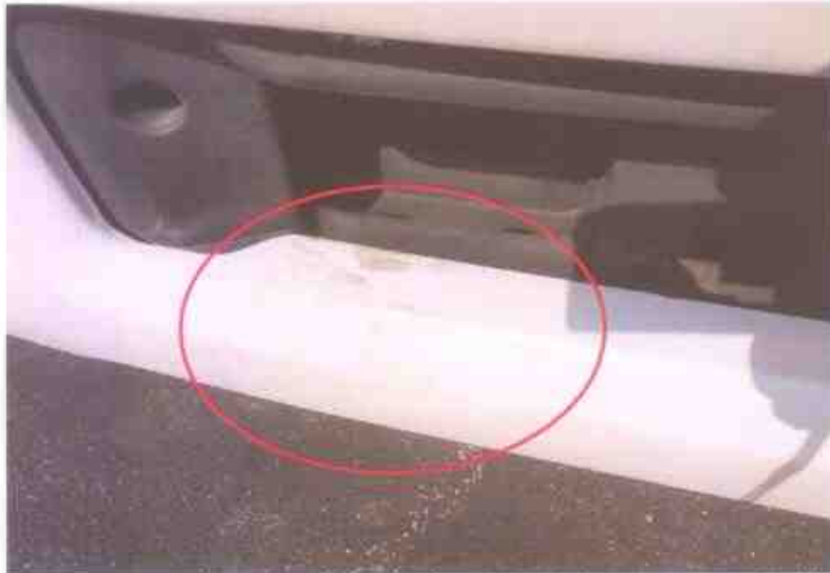
Photo 5 shows a minor stain mark on the front right side bumper as a result of the accident
