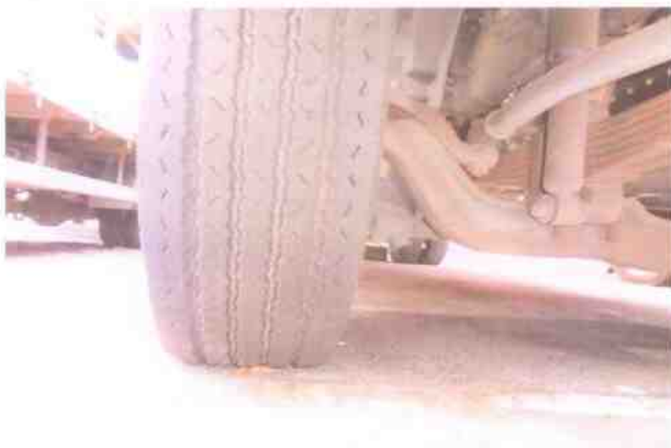
Photo 9 shows the condition of the front right tyre of the Motor Lorry, which was observed to be in serviceable condition with remaining tread depth of approximately 8mm. The tyre, which was wrapped around standard alloy wheel rim, was also observed to be sufficiently inflated for vehicular operation.
