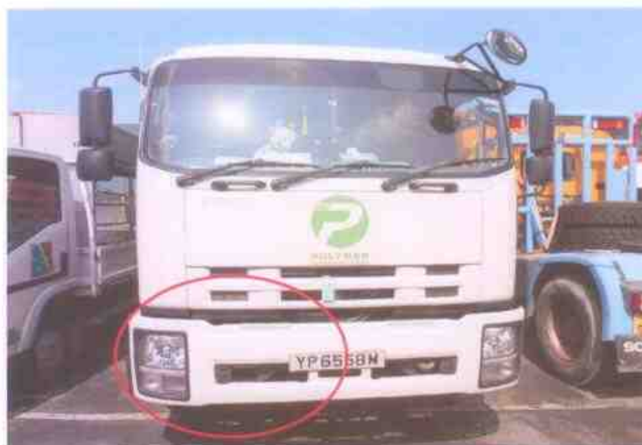
Photo 2 shows a general view of the front portion of the Motor Lorry at the time of our inspection. The Motor Lorry was observed to have sustained minor impact at its front right bumper. Only stain marks was observed on the front right bumper as a result of the accident.
