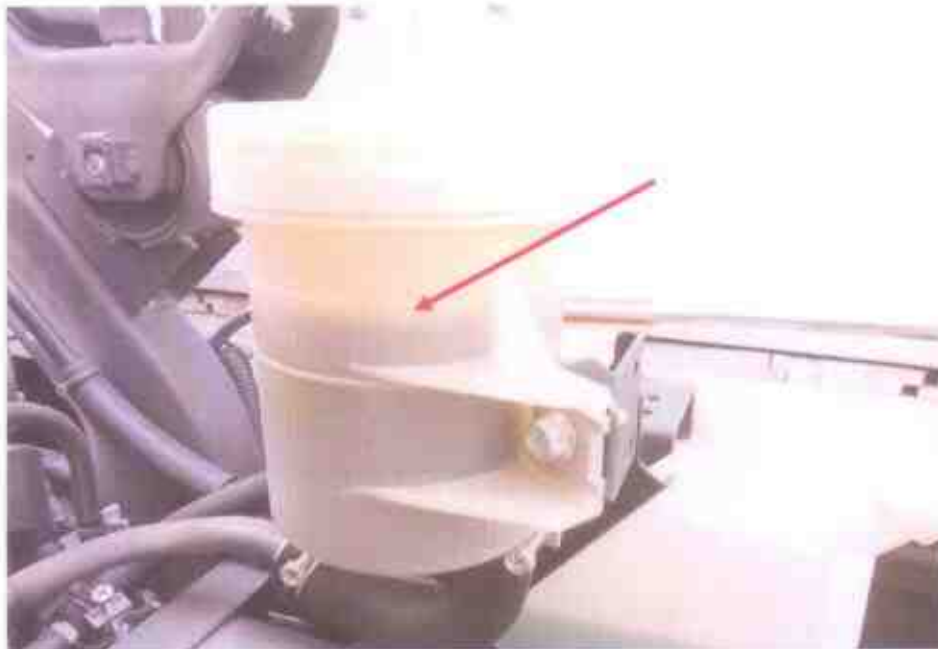
Photo 13 shows the power steering fluid reservoir of the Motor Lorry at the time of our inspection. It was observed to be of sufficient level and without any visible contamination (arrowed).
