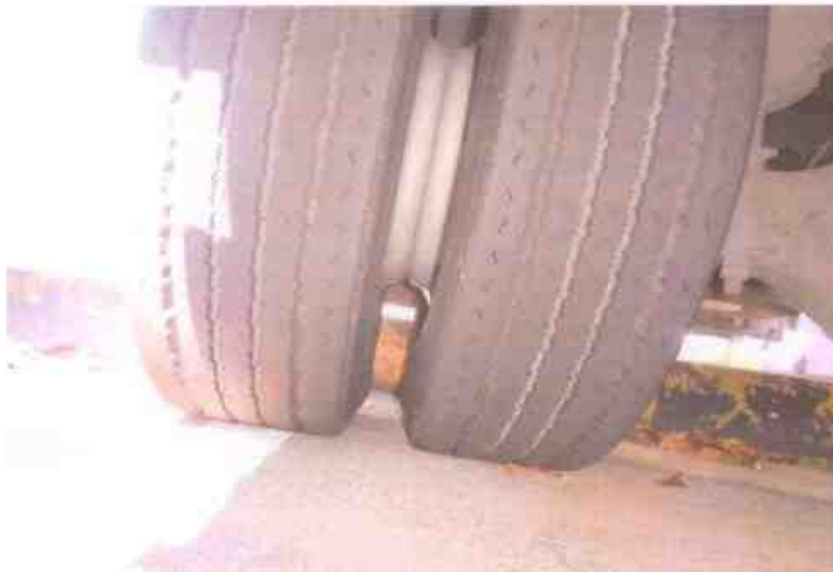
Photo 11 shows the condition of the rear right tyres of the Motor Lorry, which were observed to be in serviceable condition with remaining tread depth of approximately 9mm.
