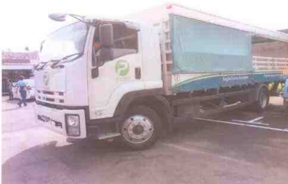
Photo 21 shows the operational test on the Motor Lorry. It was observed to be in serviceable condition. Operational test such as moving forward, turn left & right and also braking test on the Motor Lorry was conducted successfully.
