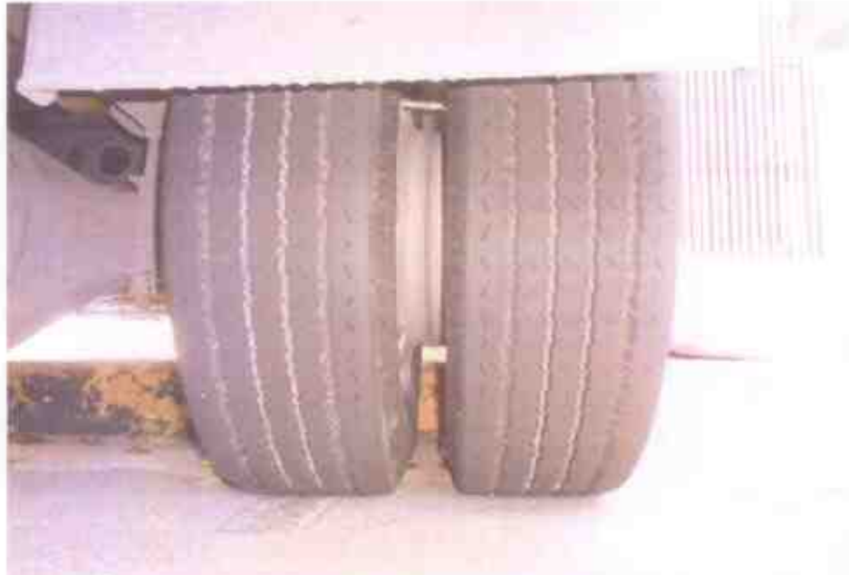
Photo 10 shows the condition of the rear left tyres of the Motor Lorry, which was observed to be in serviceable condition with remaining tread depth of approximately 8mm. The tyres, which were wrapped around standard alloy wheel rim, were also observed to be sufficiently inflated for vehicular operation.
