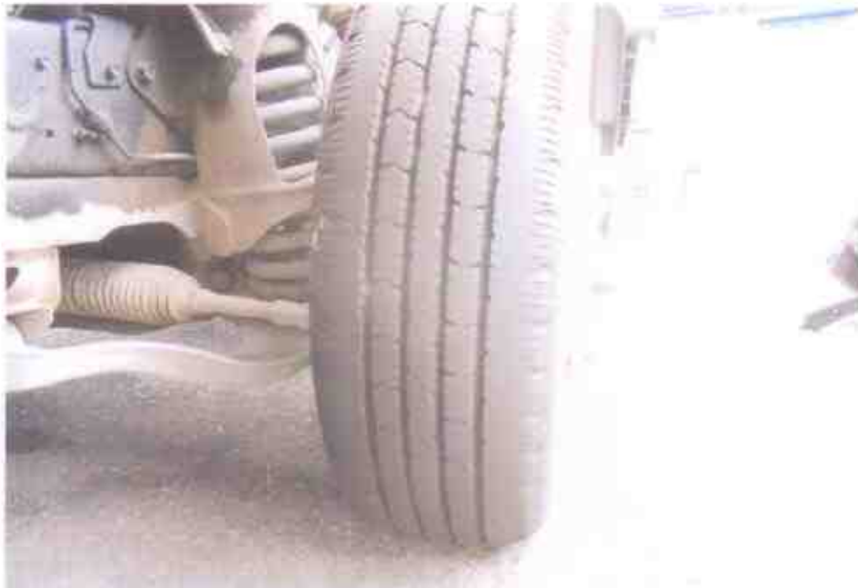
Photo 8 shows the condition of the front left tyre of the Motor Lorry, which was observed to be in serviceable condition with remaining tread depth of approximately 6mm. The tyre, which was wrapped around standard steel wheel rim, was also observed to be sufficiently inflated for vehicular operation.
