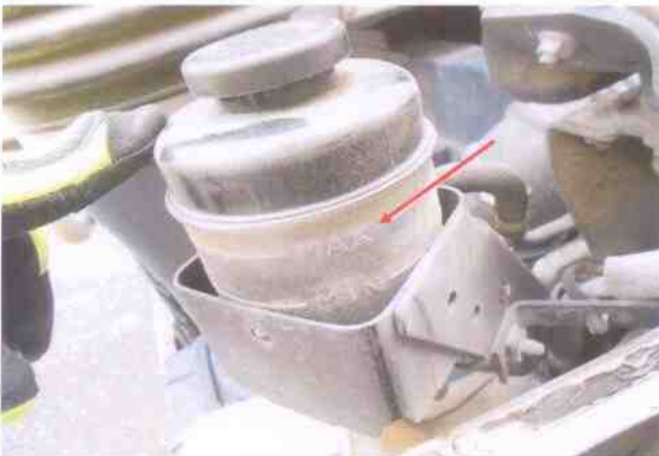
Photo 16 shows the transmission fluid of the Motor Lorry at the time of our inspection. It was observed to be of sufficient level and without any visible contamination (circled).
