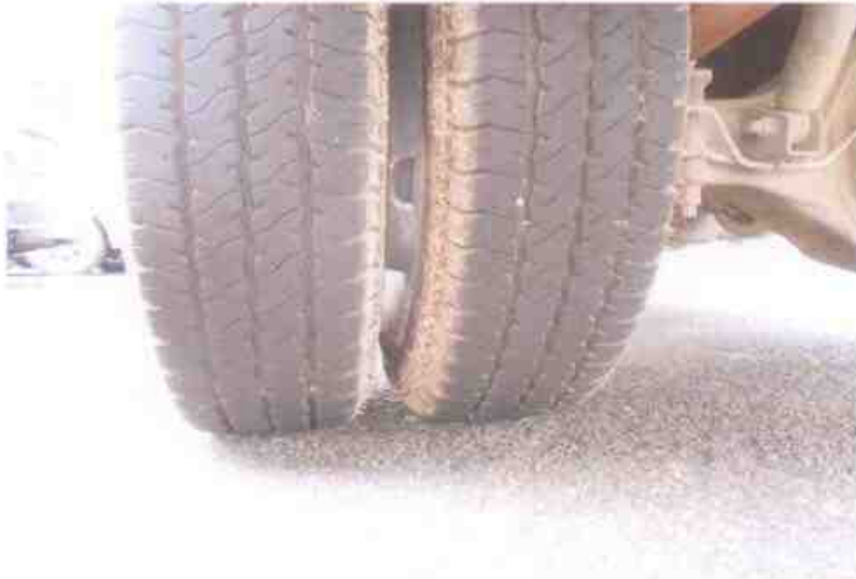
Photo 10 shows the condition of the rear left tyres of the Motor Lorry, which was observed to be in serviceable condition with remaining tread depth of approximately 7mm. The tyres, which were wrapped around standard steel wheel rim, were also observed to be sufficiently inflated for vehicular operation.
