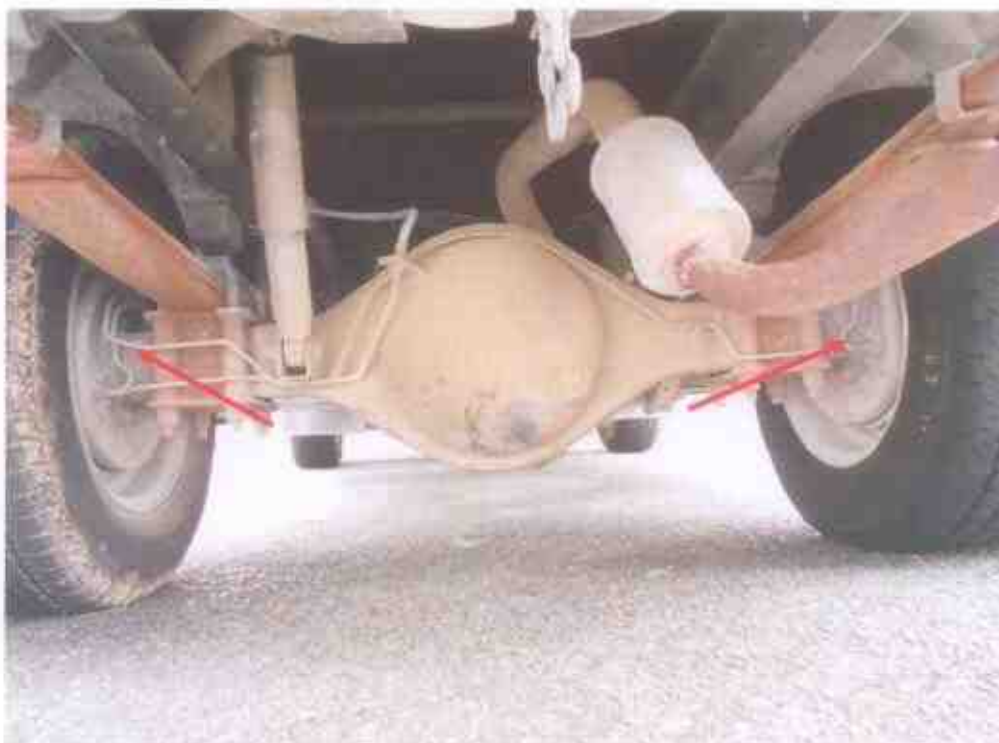
Photo 19 shows the various undercarriage components at the rear wheels of the Motor Lorry. There was no sign(s) of brake fluid leakage along the brake hoses and brake pipes.
