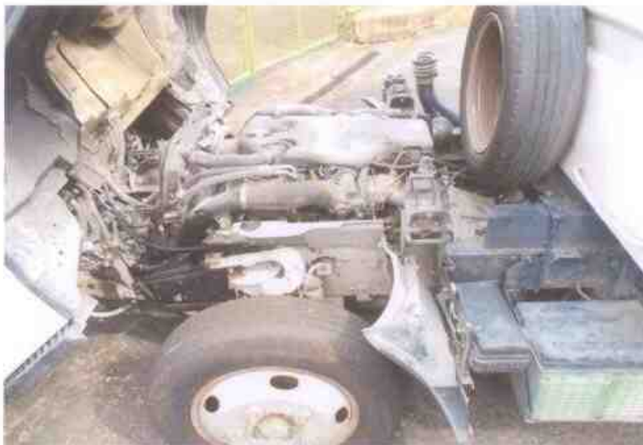
Photo 12 shows a general view of the Motor Lorry's engine compartment, which was accessed by lifting the front cabin of the Motor Lorry. The various parts and components inside the engine compartment were unaffected by the accident. There was also no sign(s) or indication(s) of fresh fluid leakage and/or fluid stain within the engine.
