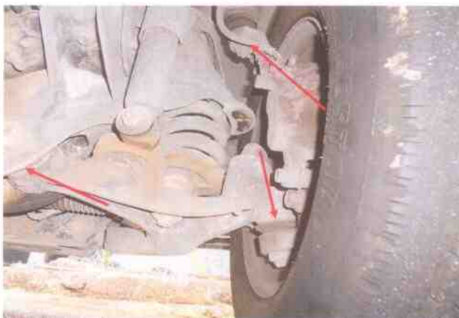
Photo 18 shows the various undercarriage components at the front right wheel of the Motor Lorry, in particular the steering tie rod end (arrowed). The various undercarriage components of the Motor Lorry were all found to be intact without any visible damage. There was also no sign of fluid stain(s) observed on the various undercarriage components.
