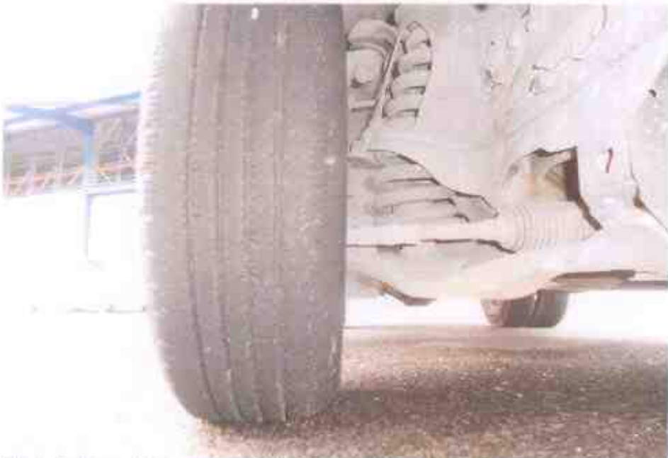
Photo 9 shows the condition of the front right tyre of the Motor Lorry, which was observed to be in serviceable condition with remaining tread depth of approximately 6mm. The tyre, which was wrapped around standard steel wheel rim, was also observed to be sufficiently inflated for vehicular operation.
