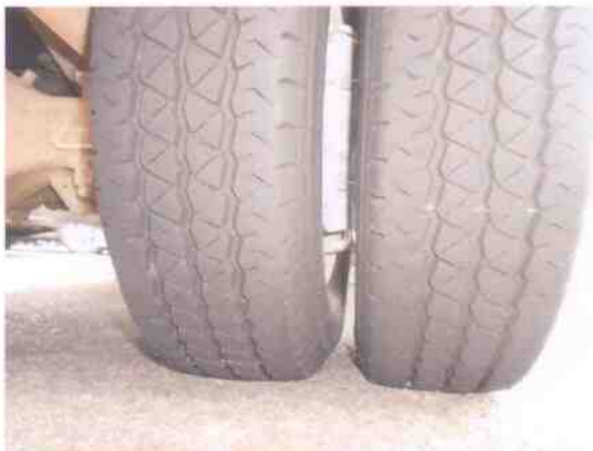
Photo 11 shows the condition of the rear right tyres of the Motor Lorry, which were observed to be in serviceable condition with remaining, tread depth of approximately 7mm.
