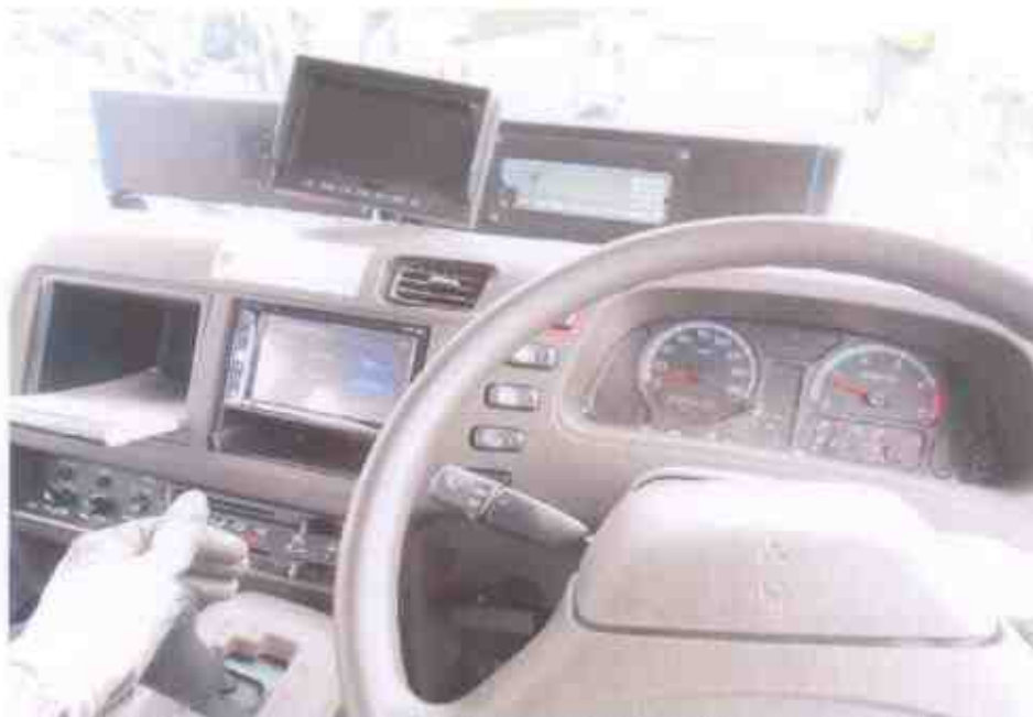
Photo 22 shows a short operational test of the Motor Bus, to primarily determine whether there was any abnormality to its various operating systems like its engine system, its transmission system, steering system and braking system was subsequently carried out. The test was conducted by driving the Motor Bus forward, stopping, before reversing and coming to a stop again.
