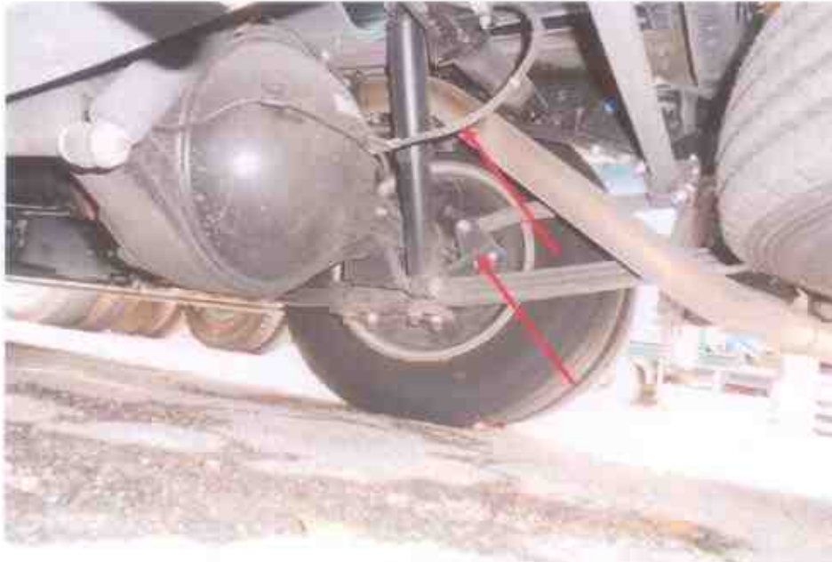
Photo 19 shows the various undercarriage components at the rear right wheel of the Motor Bus. The various steering components were all found to be intact, suggesting that the steering system of the Motor Bus was likely to be in serviceable condition at the material time of accident. There was also no sign of fluid stain(s) observed on the various undercarriage components at the 4 wheels of the Motor Van.
