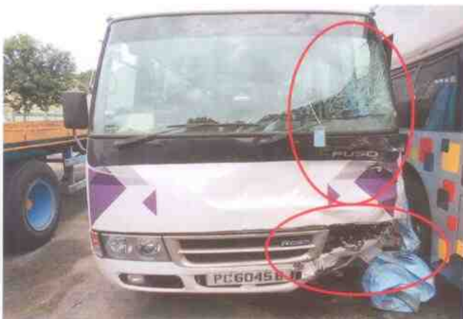
Photo 2 shows a general view of the front right body of the Motor Bus at the time of our inspection. The Motor Bus was observed to sustained damages at the front left portion due to the accident's impact.
