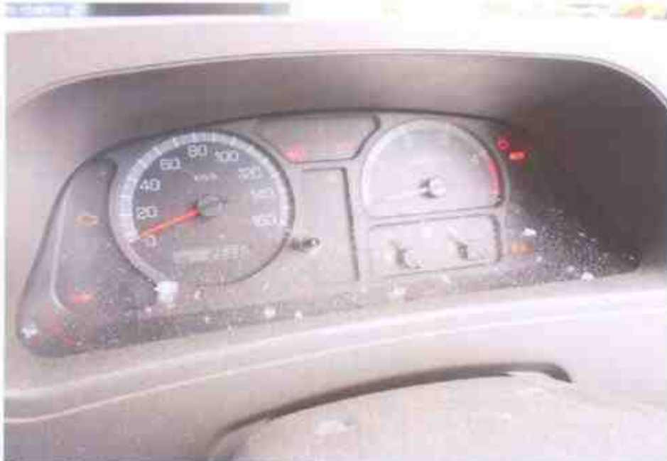
Photo 20 shows the warning lights for the various electronic operating systems of the Motor Bus appearing on its instrument panel during the self-test when the engine was cranked.
