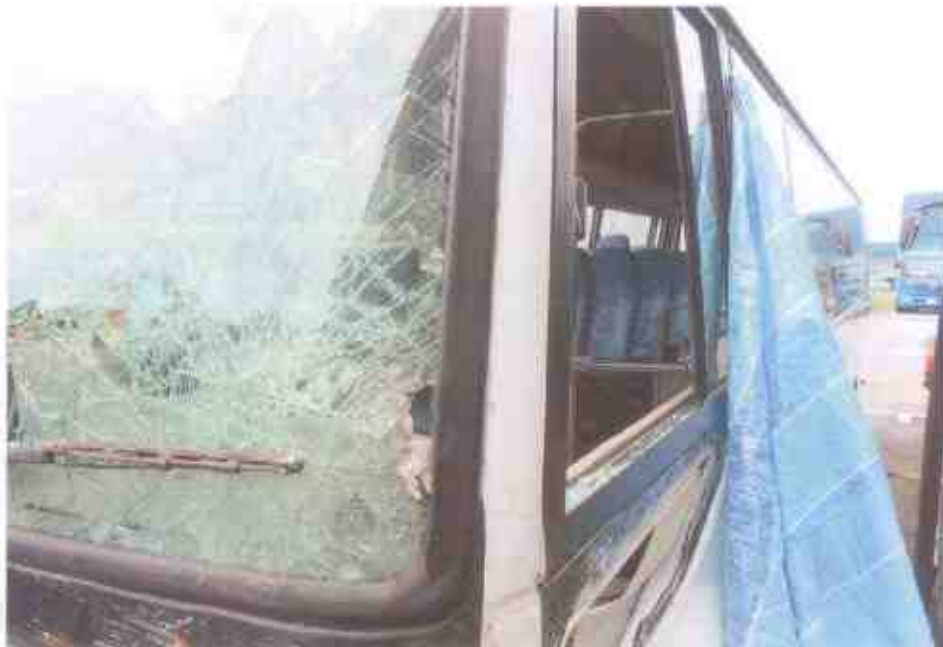
Photo 4 shows a close-up view of the shattered windshield & left side window glass of the Motor Bus at the time of our inspection. It was likely due to the accident's impact collision.
