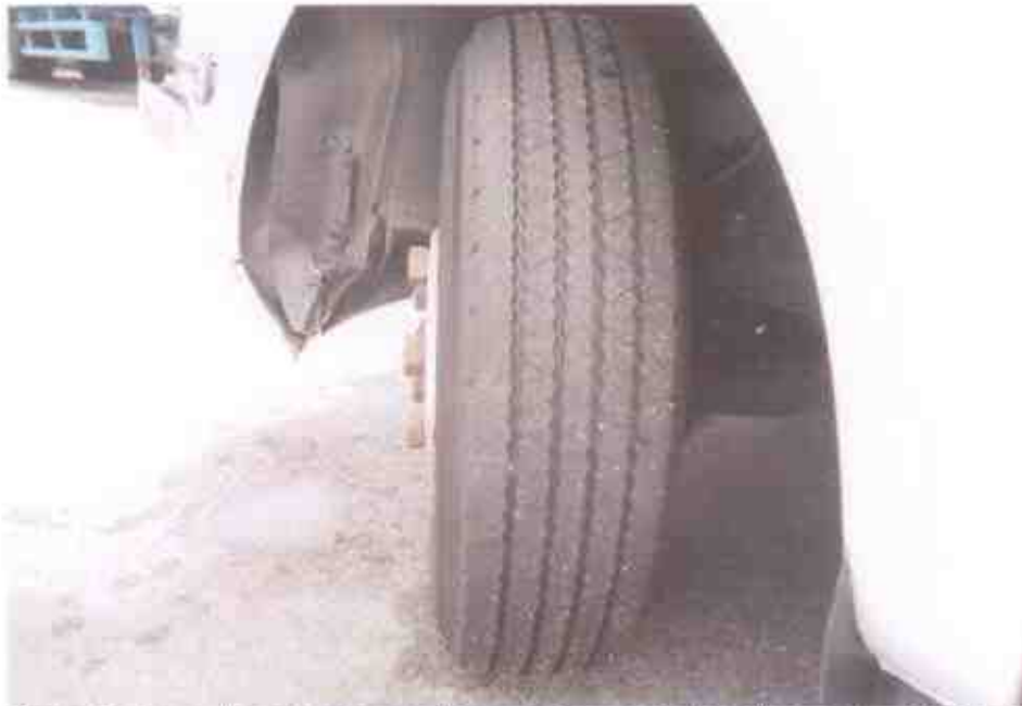
Photo 9 shows the condition of the front left tyre of the Motor Bus, which was observed to be in serviceable condition with remaining tread depth of approximately 5mm. The tyre, which was wrapped around standard wheel rim, was also observed to be sufficiently inflated for vehicular operation.
