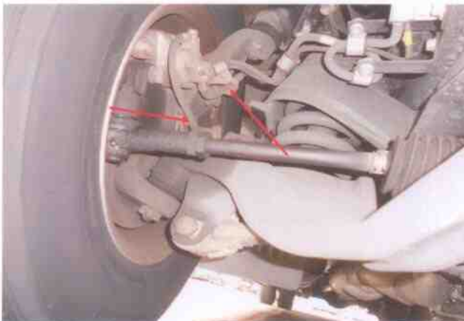
Photo 18 shows the brake hose (arrowed) at the front right wheel of the Motor Bus. We did not observed any leakage of brake fluid at the time of our inspection of the Motor Bus. Our visual inspection of the various mechanical components of the Motor Van's braking system, including its brake calliper, revealed all to be intact and without visible damage.
