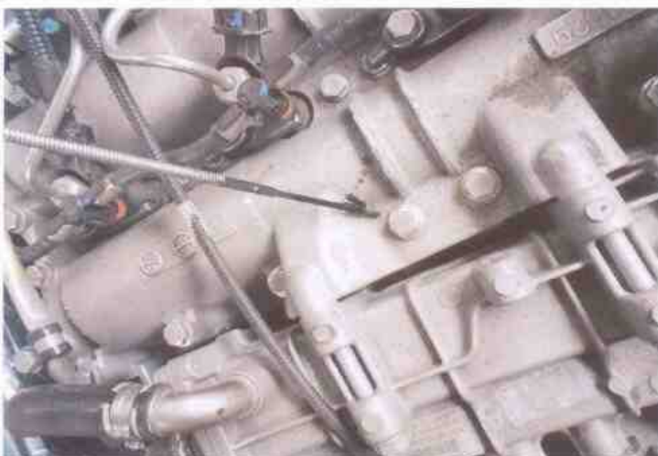
Photo 15 shows the engine dip stick of the Motor Bus at the time of our inspection. The engine oil was observed to be of sufficient level and without any visible contamination.
