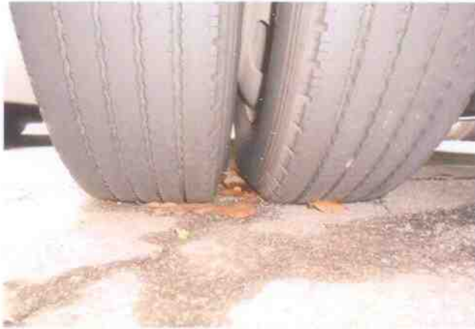
Photo 11 shows the condition of the rear right tyre of the Motor Bus, which was observed to be in serviceable condition with remaining tread depth of approximately 4mm. There was also no tear, cut or burst mark(s) on the outer and the inner sidewalls as well as across the tread of the tyre, which was also sufficiently inflated for vehicular operation.
