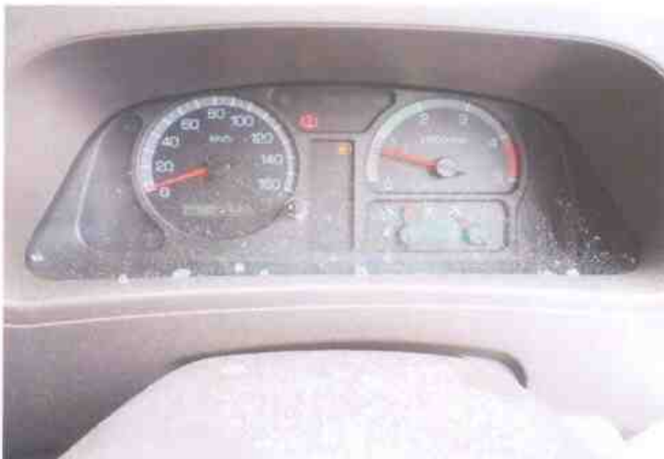
Photo 21 shows no warning lights illuminated on the instrument panel of the Motor Bus after the engine was cranked. This would suggest that there was no abnormality to the various electronic operating systems of the Motor Car.
