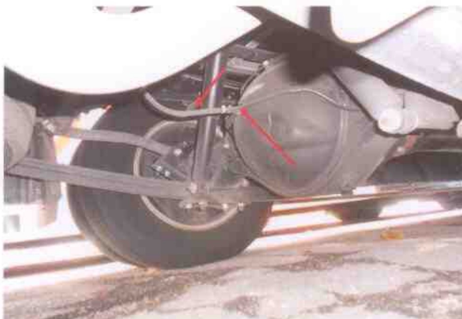
Photo 16 shows the various undercarriage components at the rear left wheel of the Motor Bus, in particular the brake hose (arrowed). We did not observe any leakage of brake fluid at the time of our inspection of the Motor Bus.
