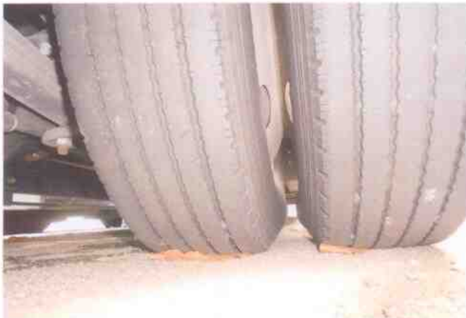
Photo 10 shows the condition of the rear left tyre of the Motor Bus, which was observed to be in serviceable condition with remaining tread depth of approximately 4mm. The tyre, which was wrapped around standard wheel rim, was also observed to be sufficiently inflated for vehicular operation. There was also no significant damage found on the 4 wheel rims of the Motor Bus.
