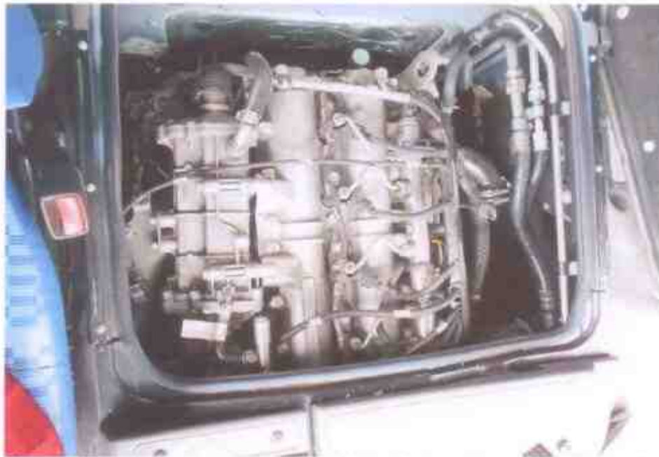
Photo 12 shows a general view of the Motor Bus's engine compartment. The various parts and components inside the engine compartment were unaffected by the accident. There was also no sign(s) or indication(s) of fluid leakage and/or fluid stain within the engine compartment.
