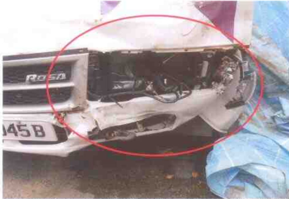
Photo 3 shows a close-up view of the damages on the left side headlamp of the Motor Bus at the time of our inspection. It was likely due to the accident's impact collision.
