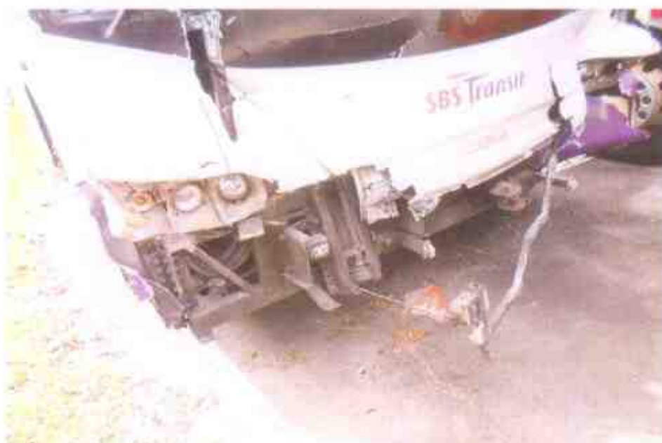
Photo 4 shows a close-up view of the front right body of the Motor Bus at the time of our inspection. The Motor Bus was observed to sustained damages due to the accident's impact.
