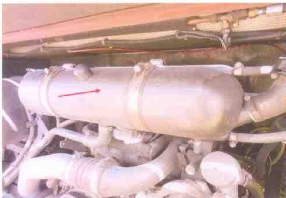
Photo 15 shows the engine coolant cylinder of the Motor Bus. It was observed to be of sufficient level without any contamination at time of our inspection.
