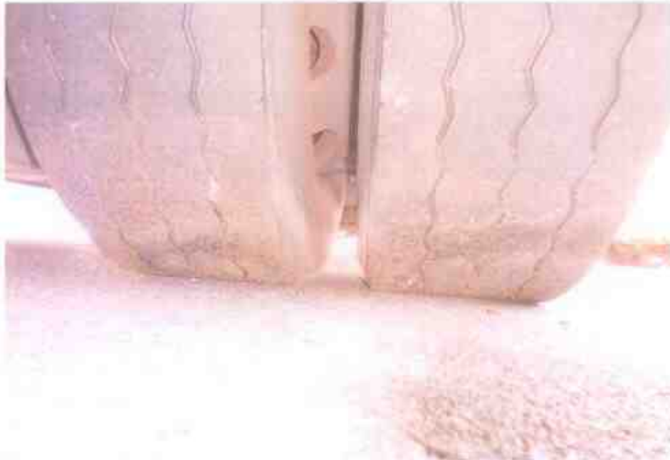
Photo 10 shows the condition of the rear right tyres of the Motor Bus, which were observed to be in serviceable condition with remaining tread depth of approximately 6mm. The tyres, which were wrapped around standard alloy wheels rims, were also observed to be sufficiently inflated for vehicular operation.
