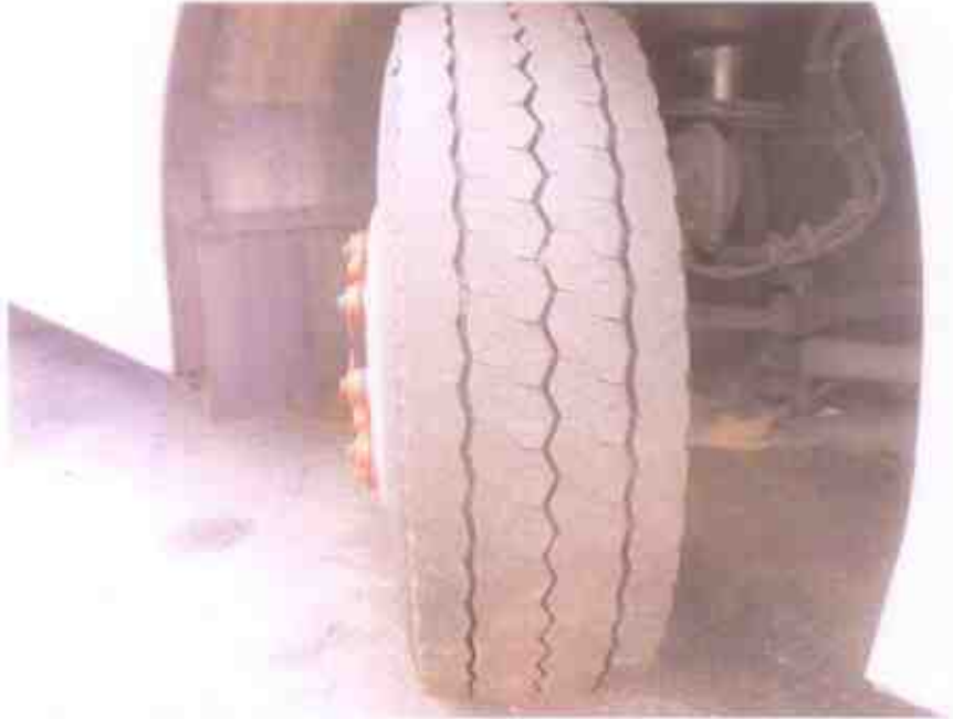
Photo 8 shows the condition of the front right tyre of the Motor Bus, which was observed to be in serviceable condition with remaining tread depth of approximately 8mm. The tyre was also observed to be sufficiently inflated for vehicular operation.
