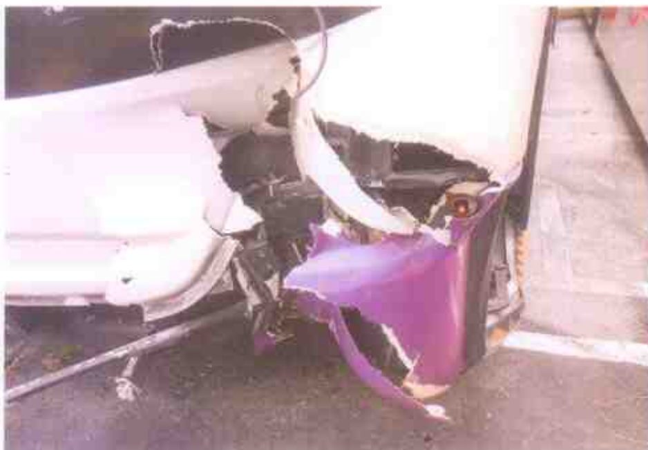
Photo 3 shows a close-up view of the front left body of the Motor Bus at the time of our inspection. The Motor Bus was observed to sustained damages due to the accident's impact.
