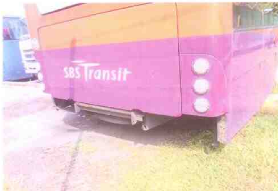
Photo 2 shows a general view of the rear portion of the Motor Bus at the time of our inspection. The Motor Bus was observed to be in good condition unaffected by the accident. The rear bumper was dismantled for towing purposes.
