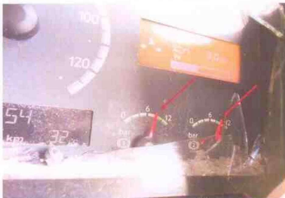
Photo 20 shows pressure tank 1 & tank 2 were observed to be pressurised up to 10bars after the engine start-up. No drop in the pressure after a few minutes which means there's no air leakage from the air-braking system.
