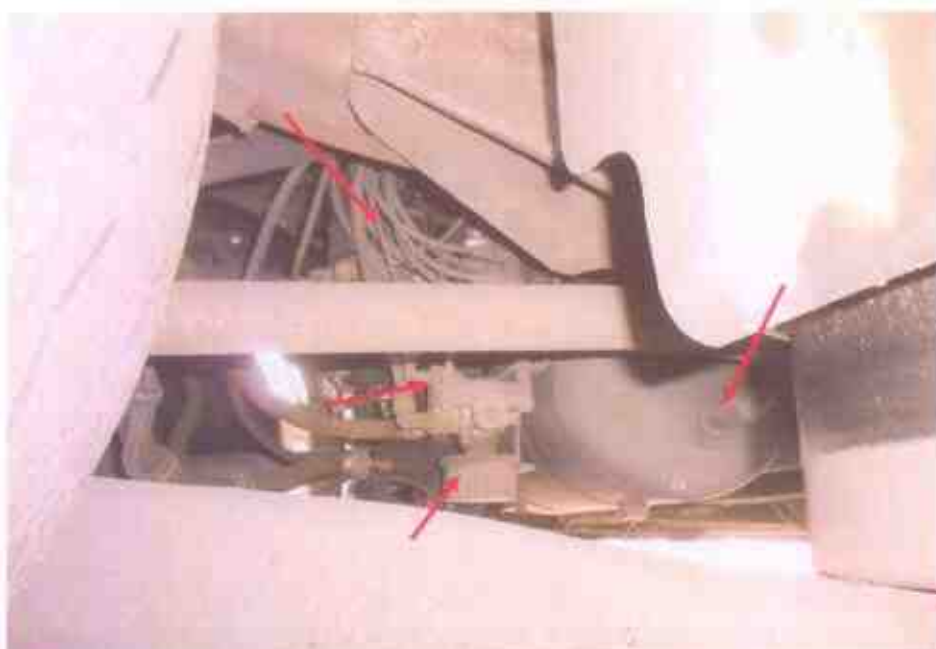
Photo 21 shows a general view of the air tank, valves, pipes and hoses, which are some of the components for the air-assisted braking system of the Motor Bus. This was at the underside of the Motor Bus's body. There were no damages observed at time of our inspection.
