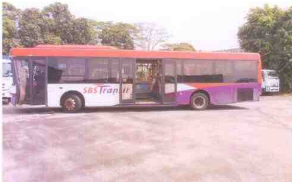
Photo 28 shows the operational test on the Motor Bus. SBS driver were able to move the Motor Bus forward, backward, turning left & right & stopping without any abnormalities
