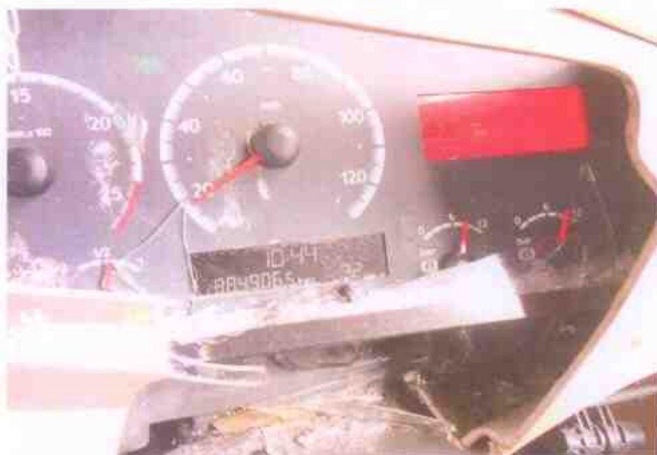
Photo 25 shows the indicators at the driver's seat, these systems were in working condition. This can be established from the warning lights disappearing from the instrument panel after the self-test. However, only the Anti-Locking Braking System (ABS) stayed lighted up amongst others.
