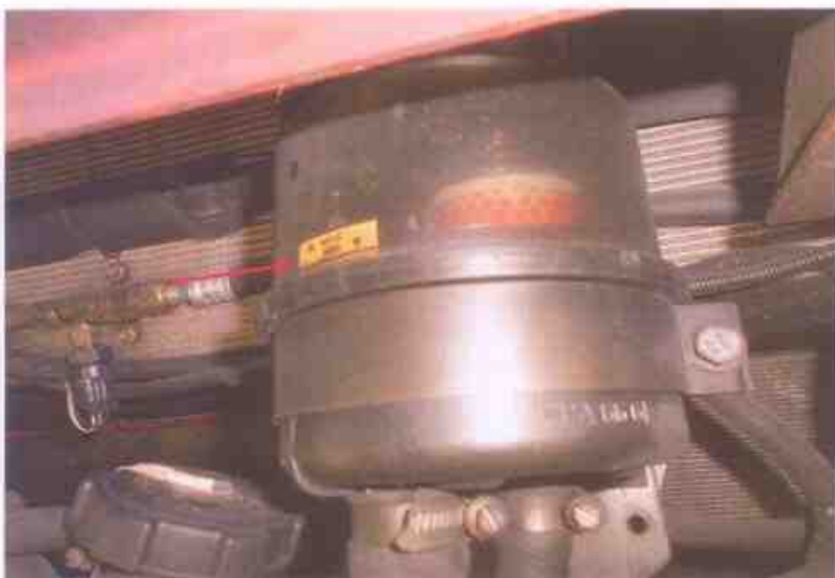
Photo 14 shows the steering fluid of the Motor Bus. It was observed to be of sufficient level without any contamination at time of our inspection.
