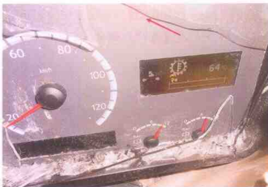
Photo 24 shows the warning lights for the various electronic operating systems of the Motor Bus appearing on its instrument panel during the self-test when the engine was cranked.
