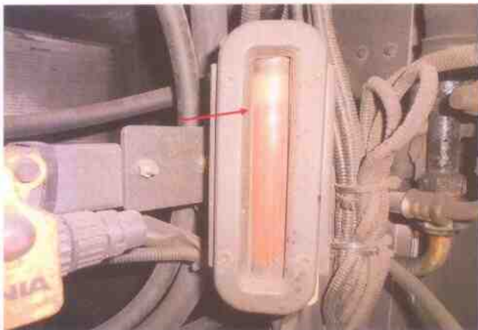
Photo 16 shows the engine coolant indicator of the Motor Bus. It was observed to be of sufficient level without any contamination at time of our inspection.
