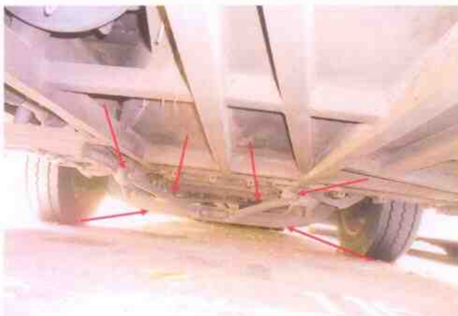
Photo 19 shows the undercarriage components at the front steering system of the Motor Bus. The various undercarriage components of the Motor Bus were all observed to be intact and without any visible damage. This had included the steering rack and steering ball joints (arrowed) of the Motor Bus, which were observed to be securely attached to the front left wheel and front right wheel.
