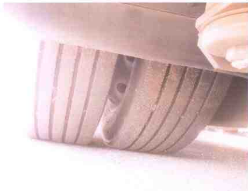
Photo 11 shows the condition of the rear left tyres of the Motor Bus, which were observed to be in serviceable condition with remaining tread depth of approximately 8mm. The tyres, which were wrapped around standard alloy wheel rims, were also observed to be sufficiently inflated for vehicular operation.
