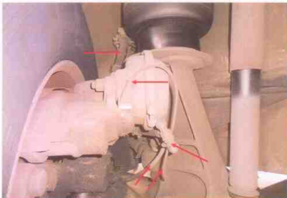
Photo 22 shows some of the mechanical components (arrowed) of the Motor Bus's braking system. Our visual check on the various mechanical components revealed all to be intact and in good condition. It was in serviceable condition at the time of accident.
