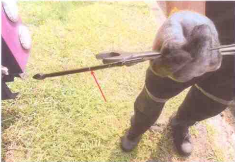
Photo 17 shows the engine fluid on the dip stick of the Motor Bus. It was observed to be of sufficient level without any contamination at time of our inspection.
