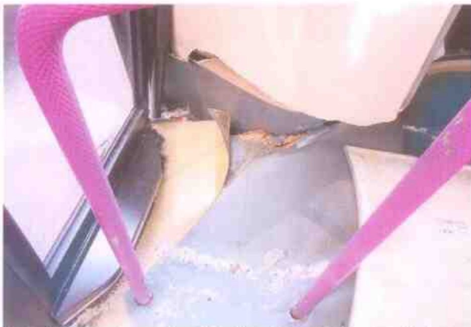
Photo 7 shows a close-up view of the Motor Bus's floor board next to the front passenger's glass door that was observed to be damaged due to the accident's impact.
