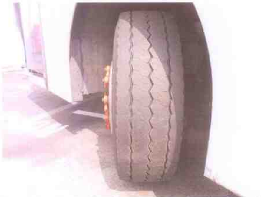
Photo 9 shows the condition of the front left tyre of the Motor Bus, which was observed to be in serviceable condition with remaining tread depth of approximately 9mm. The tyre was also observed to be sufficiently inflated for vehicular operation.
