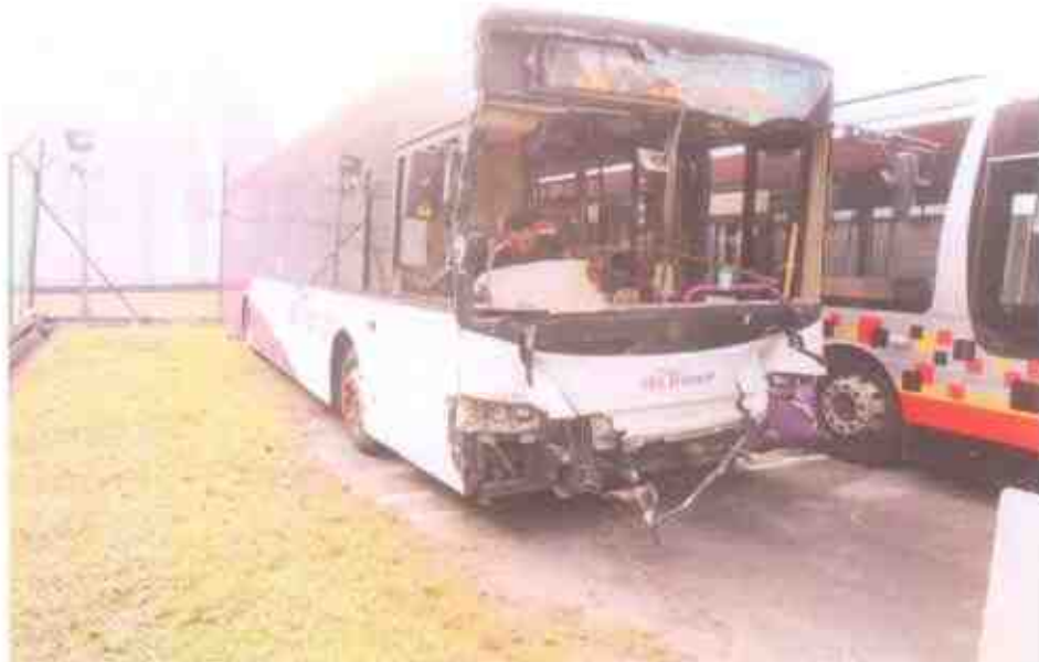
Photo 1 shows a general view of the front body of the Motor Bus at the time of our inspection. The Motor Bus was observed to have sustained damages at its front portion as a result of the accident's collision.
