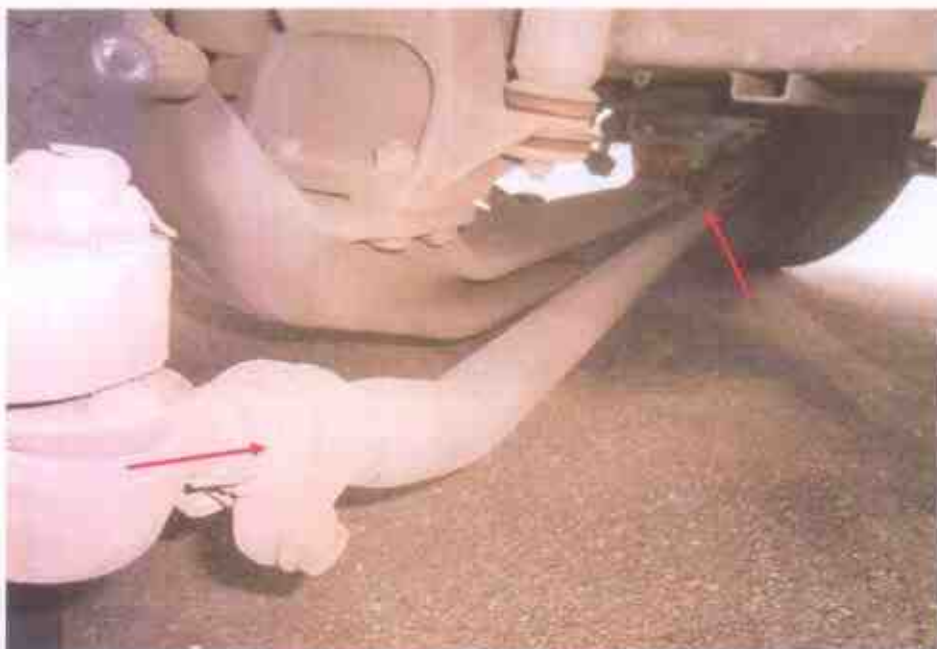
Photo 18 shows some of the mechanical components (arrowed) of the Motor Bus's steering system. Our visual check on the various mechanical components of the steering system revealed all to be intact and in good condition. The steering system of the Motor Bus likely to be in serviceable condition at the time of accident.
