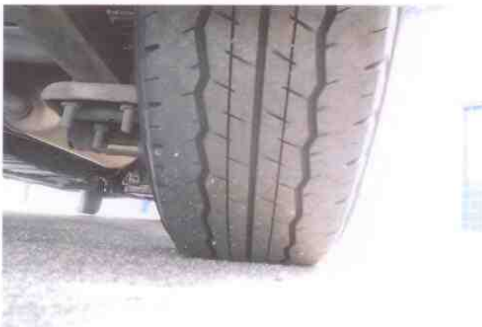
Photo 11 shows the condition of the rear right tyre of the Motor Bus, which was observed to be in serviceable condition with remaining tread depth of approximately 6mm. There was also no tear, cut or burst mark(s) on the outer and the inner sidewalls as well as across the tread of the tyre, which was also sufficiently inflated for vehicular operation.
