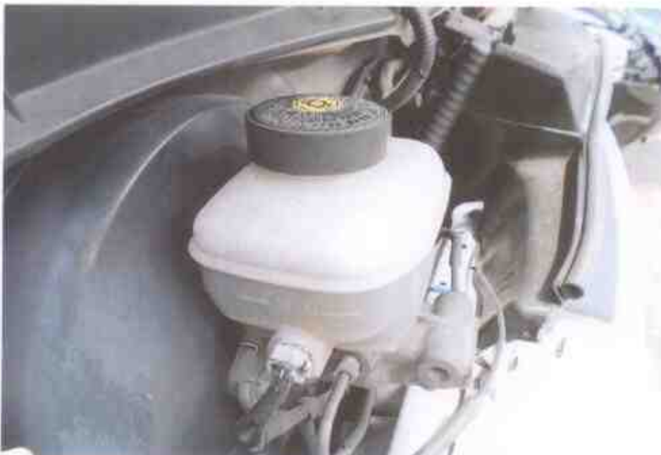
Photo 13 shows the brake fluid reservoir of the Motor Bus at the time of our inspection. The brake fluid was observed to be of sufficient level and without any visible contamination.
