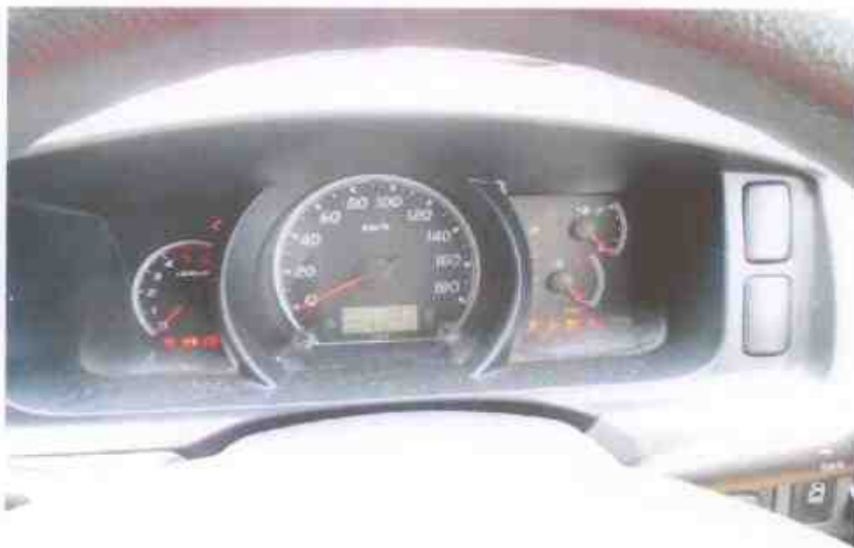
Photo 21 shows the warning lights for the various electronic operating systems of the Motor Bus appearing on its instrument panel during the self-test when the engine was cranked.
