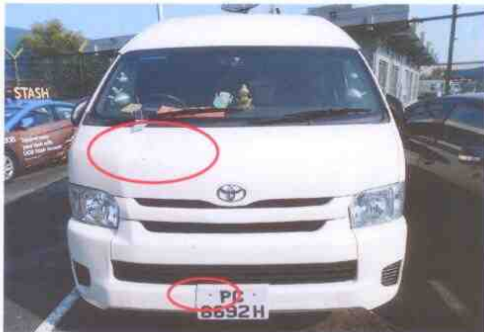
Photo 2 shows a general view of the front right body of the Motor Bus at the time of our inspection. The Motor Bus was observed to sustained minor damage at the front right panel & lower bumper.
