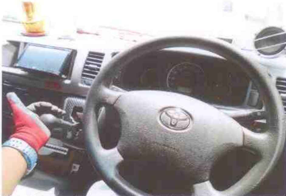
Photo 23 shows a short operational test of the Motor Bus, to primarily determine whether there was any abnormality to its various operating systems like its engine system, its transmission system, steering system and braking system was subsequently carried out. The test was conducted by driving the Motor Bus forward, stopping, before reversing and coming to a stop again.
