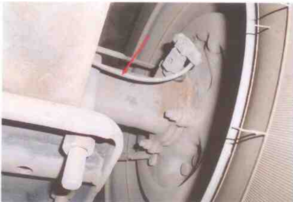
Photo 20 shows the various undercarriage components at the rear right wheel of the Motor Bus. The various steering components were all found to be intact, suggesting that the steering system of the Motor Bus was likely to be in serviceable condition at the material time of accident. There was also no sign of fluid stain(s) observed on the various undercarriage components at the 4 wheels of the Motor Van.
