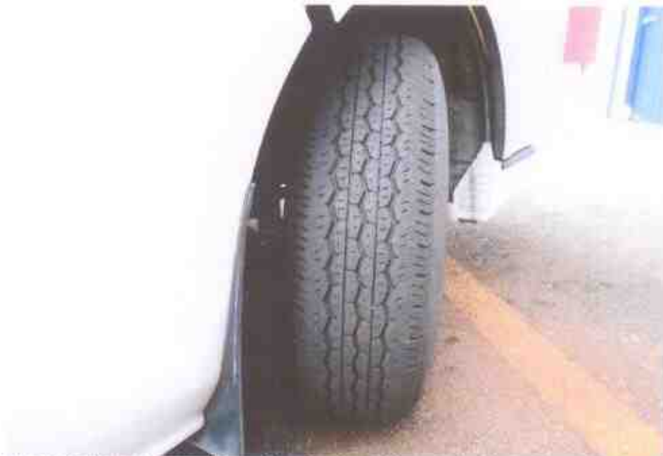
Photo 8 shows the condition of the front right tyre of the Motor Bus, which was observed to be in serviceable condition with remaining tread depth of approximately 8mm. The tyres were all observed to be sufficiently inflated for vehicular operation with no tear, cut or burst mark(s) on the outer and the inner sidewalls as well as across the tread.
