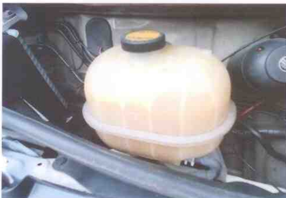
Photo 14 shows the engine coolant reservoir of the Motor Bus at the time of our inspection. The engine coolant was observed to be of sufficient level and without any visible contamination.
