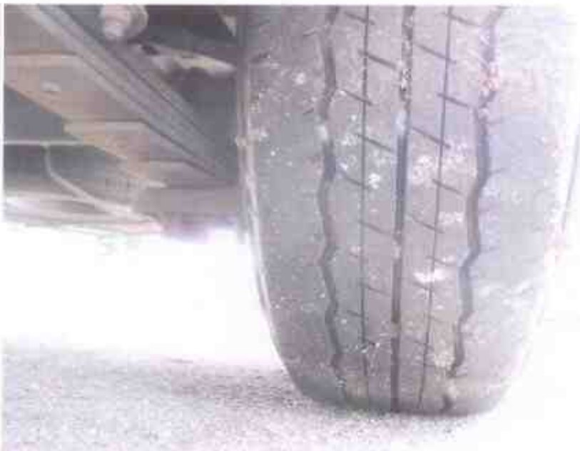
Photo 10 shows the condition of the rear left tyre of the Motor Bus, which was observed to be in serviceable condition with remaining tread depth of approximately 7mm. The tyre, which was wrapped around standard wheel rim, was also observed to be sufficiently inflated for vehicular operation. There was also no significant damage found on the 4 wheel rims of the Motor Bus.
