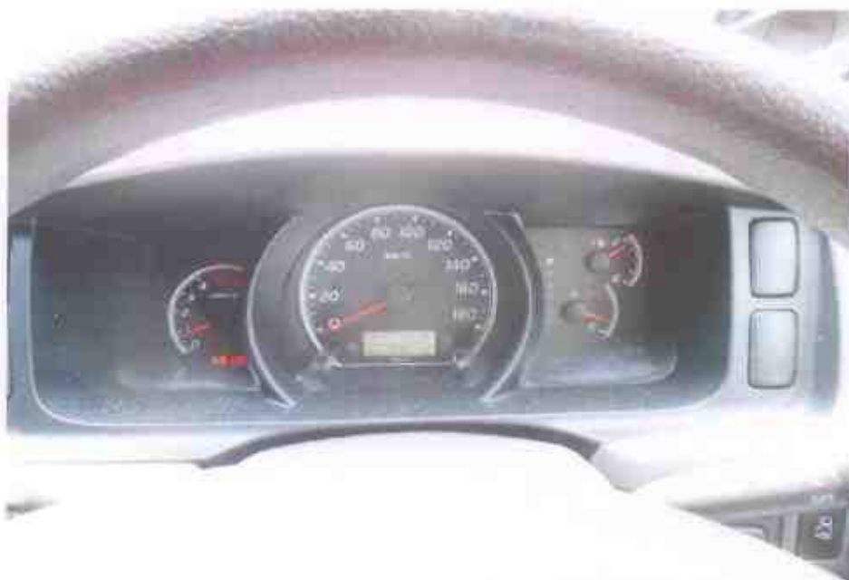
Photo 22 shows no warning lights illuminated on the instrument panel of the Motor Bus after the engine was cranked. This would suggest that there was no abnormality to the various electronic operating systems of the Motor Car except for only ABS warning light stayed lighted up.
