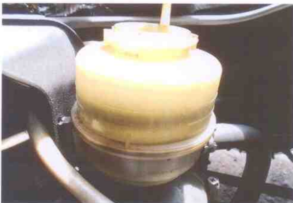
Photo 15 shows the power steering reservoir of the Motor Bus at the time of our inspection. It was observed to be of sufficient level and without any visible contamination.
