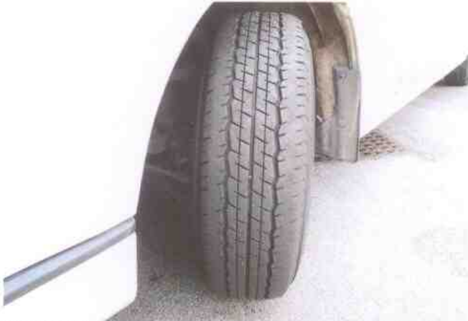
Photo 9 shows the condition of the front left tyre of the Motor Bus, which was observed to be in serviceable condition with remaining tread depth of approximately 8mm. The tyre, which was wrapped around standard wheel rim, was also observed to be sufficiently inflated for vehicular operation.
