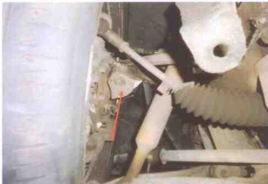
Photo 22 shows the front right side wheel upper arm that was observed to be broken/damaged likely due to the accident's impact.
