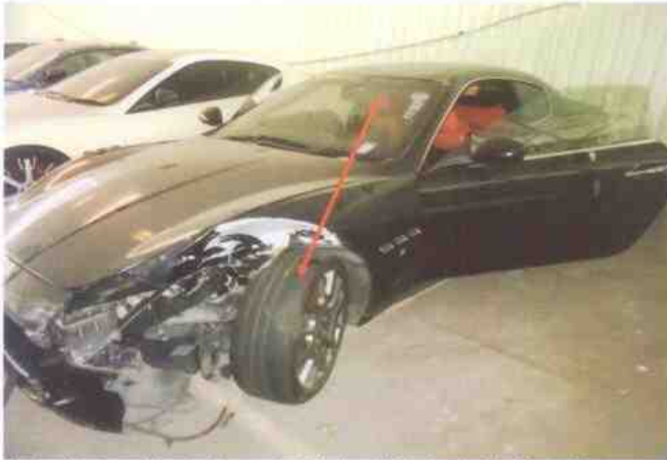
Photo 19 shows the misalignment at the front left wheel of the Motor Car.
