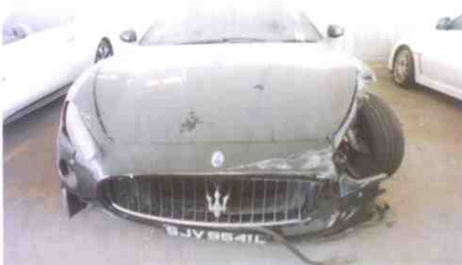
Photo 1 shows a general view of the frontal portion of the Motor Car at the time of our inspection. The Motor Car was observed to have sustained extensive impact damage at its frontal left & right portion. The impact force was significant, causing the various parts and components to be damaged as a result of the accident.
