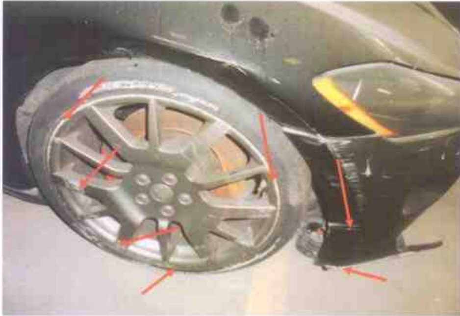
Photo 4 shows the damages at the front right side wheel & front lower right bumper of the Motor Car. Such damages were likely caused by road kerb grazing at the material time of the accident.
