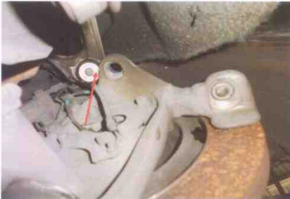
Photo 20 shows the dislodged upper arm that was observed to be damaged likely due to the accident's impact.
