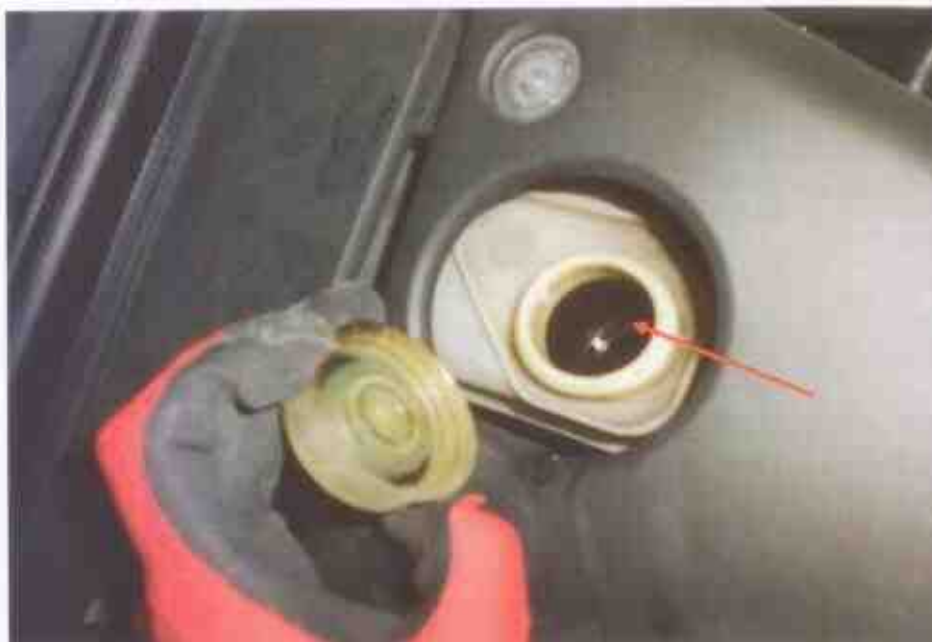
Photo 17 shows the close up view of the brake fluid that was seen with sufficient level not affected by the accident's impact.
