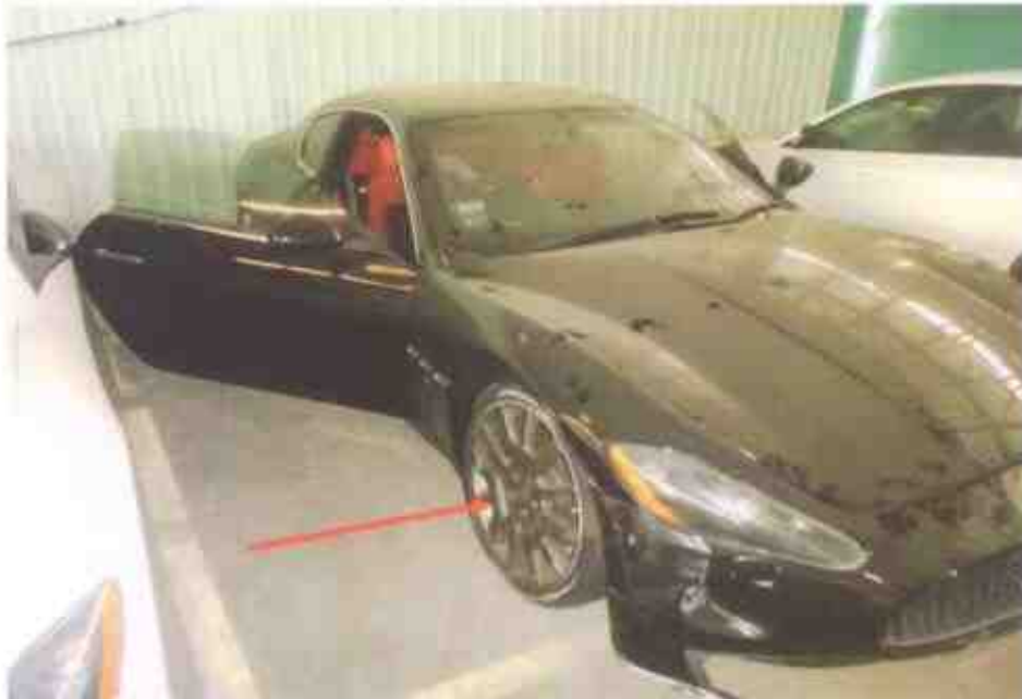
Photo 21 shows the correct alignment at the front right side wheel of the Motor Car. However, further investigation found broken supporting part (upper arm) likely due to the accident's collision impact.
