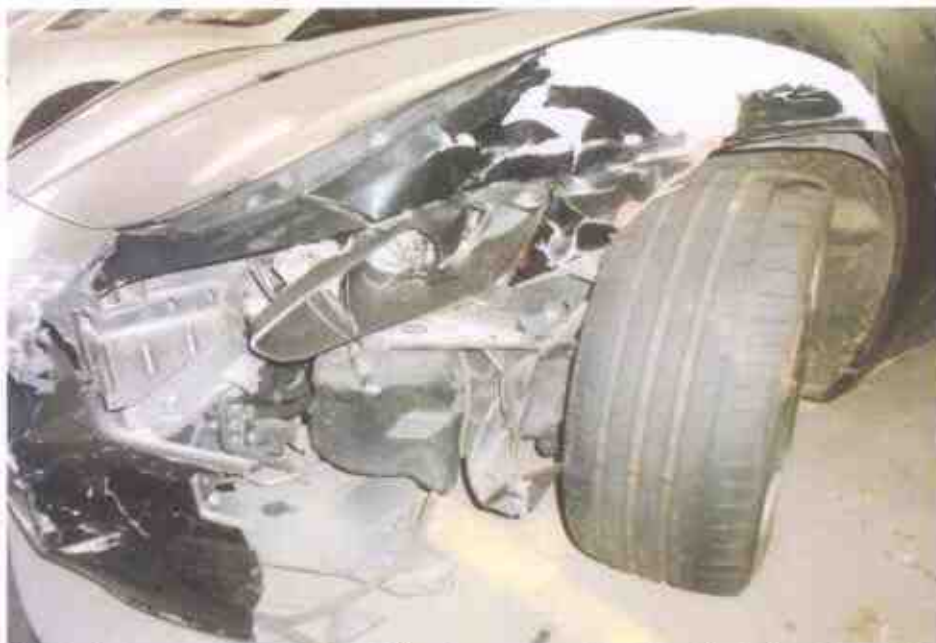
Photo 7 shows a closer view of the damage sustained on the left portion of the Motor Car. The impact force was significant, causing the left portion of the Motor Car to be pushed inwards as a result of the accident.
