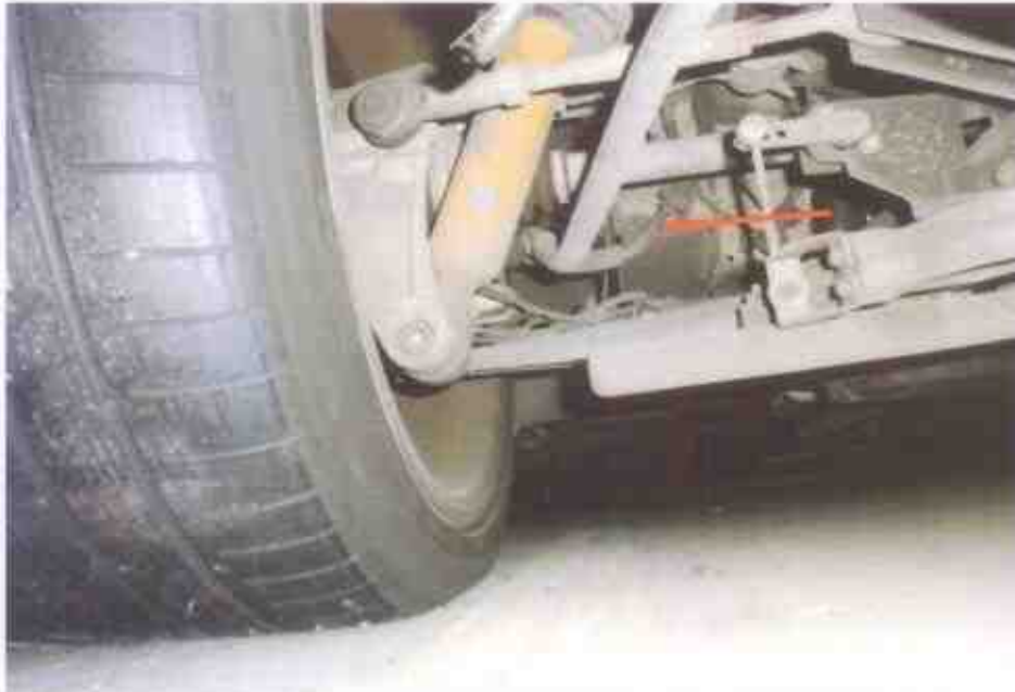
Photo 26 shows the braking components at the rear right wheel of the Motor Car. We did not observe any leakage of brake fluid at the time of our inspection of the Motor Car.
