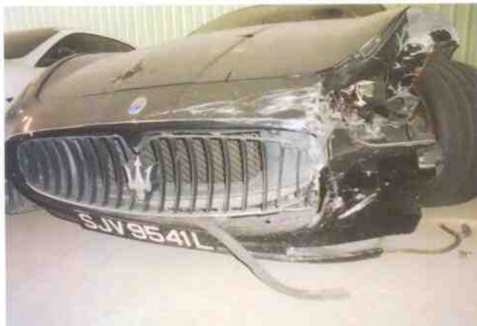
Photo 8 shows a closer view of the damage sustained on the front left of the Motor Car. The impact force was significant, causing the various parts and components such as front bumper, front grille amongst others to be damaged due to the accident's collision impact.
