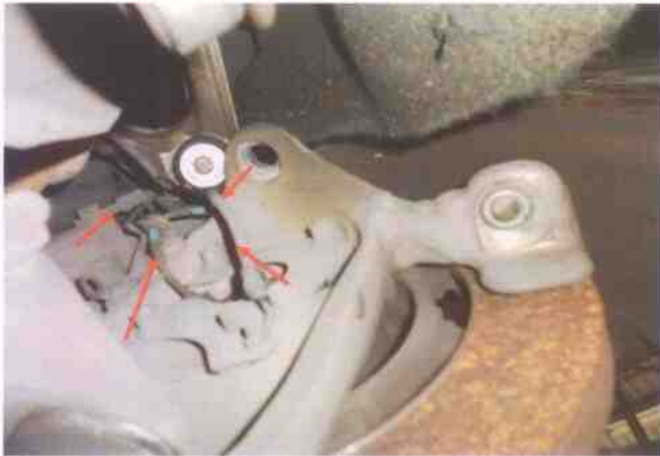
Photo 23 shows the braking components at the front left wheel of the Motor Taxi. We did not observe any leakage of brake fluid at the time of our inspection of the Motor Car.
