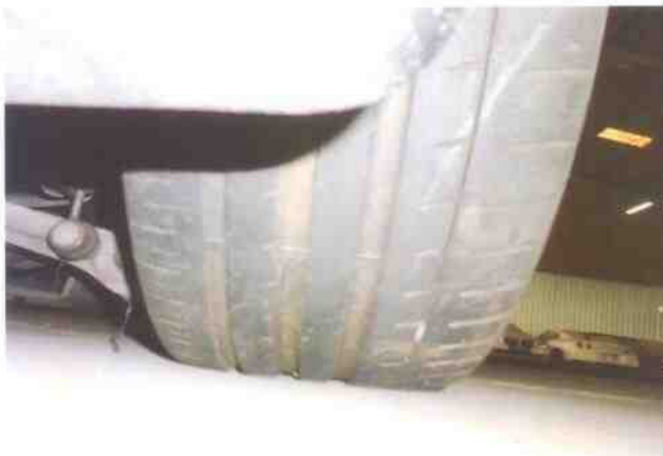
Photo 11 shows the condition of the front right tyre of the Motor Car, which was observed to be in serviceable condition with remaining tread depth of approximately 4mm. There was no tear, cut or burst mark(s) on the outer and the inner sidewalls as well as across the tread of this tyre.
