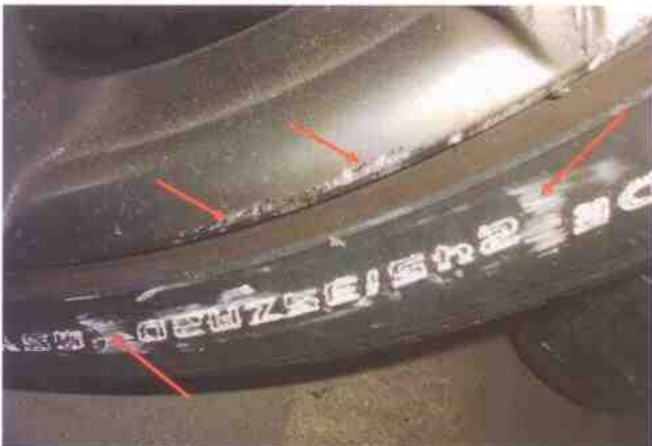
Photo 5 shows a close-up view of the damages at the front right side wheel of the Motor Car. Such damages were likely caused by road kerb grazing at the material time of the accident.
