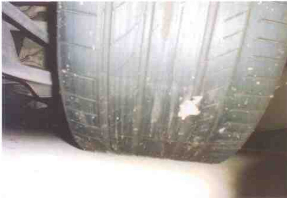
Photo 13 shows the condition of the rear right tyre of the Motor Car, which was observed to be in serviceable condition with remaining tread depth of approximately 3mm. There was also no tear, cut or burst mark(s) on the outer and the inner sidewalls as well as across the tread of this tyre.
