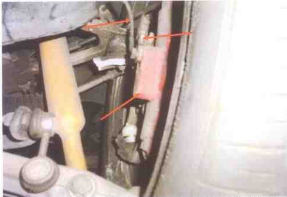
Photo 24 shows the braking components at the front right wheel of the Motor Car. We did not observe any leakage of brake fluid at the time of our inspection of the Motor Car.
