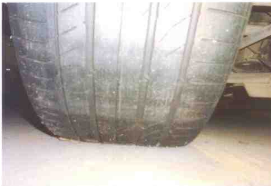
Photo 14 shows the condition of the rear left tyre of the Motor Car, which was observed to be in serviceable condition with remaining tread depth of approximately 3mm. There was also no tear, cut or burst mark(s) on the outer and the inner sidewalls as well as across the tread of this tyre.
