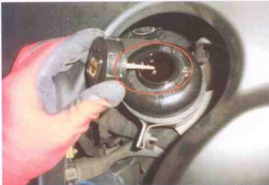
Photo 16 shows the close up view of the power steering fluid that was seen with sufficient level not affected by the accident's impact
