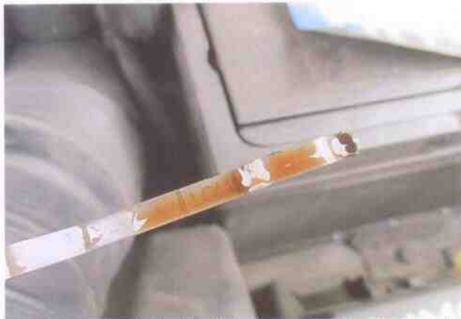
Photo 16 shows the ATF dipstick of the Motor Taxi at the time of our inspection. The ATF was observed to be of sufficient level and without any visible contamination.
