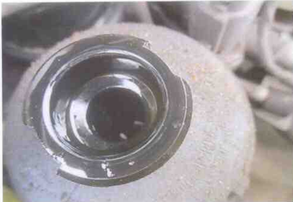
Photo 13 shows the power steering fluid reservoir of the Motor Taxi at the time of our inspection. The power steering fluid was observed to be of sufficient level and without any visible contamination.
