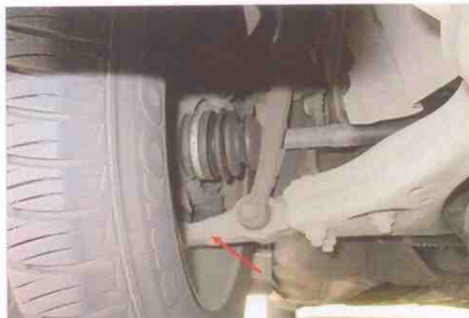
Photo 19 shows the various undercarriage components at the front right wheel of the Motor Taxi, in particular the steering tie rod (arrowed). The various steering components were all found to be intact, suggesting that the steering system of the Motor Taxi was likely to be in serviceable condition at the material time of accident. There was also no sign of fluid stain observed on the various undercarriage components at the front right wheel of the Motor Taxi.
