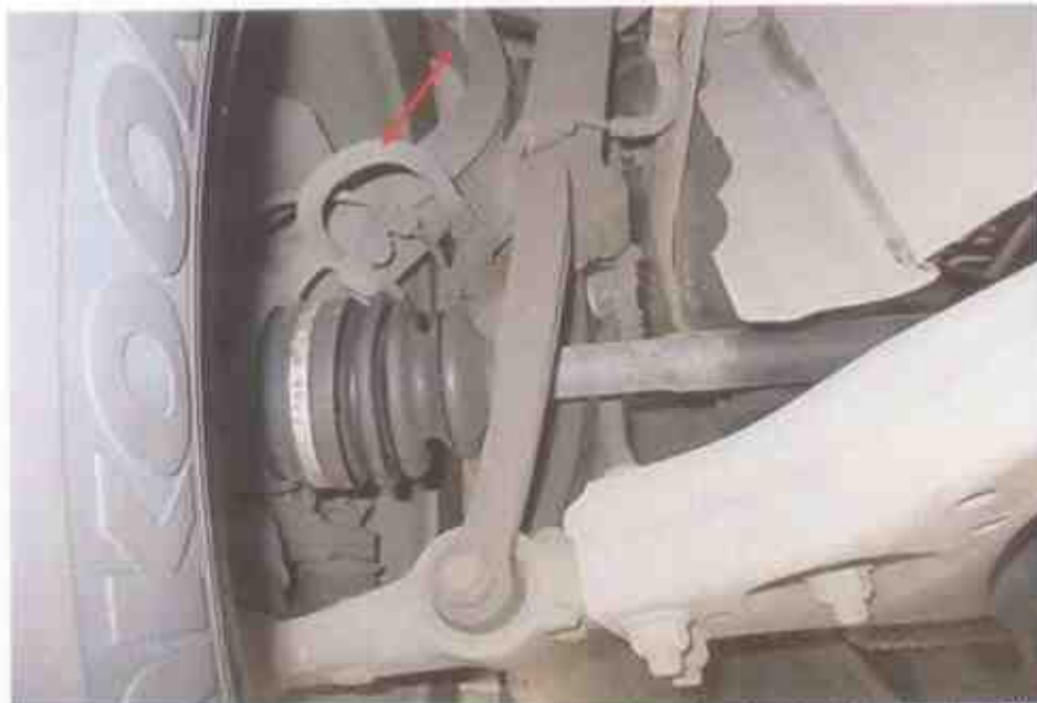
Photo 18 shows the brake hose/pipe (arrowed) at the front right wheel of the Motor Taxi. No leakage of brake fluid was observed. Visual examination of the various components of the braking system like the brake caliper, brake booster, brake pedal etc had revealed all to be intact and without visible damage.
