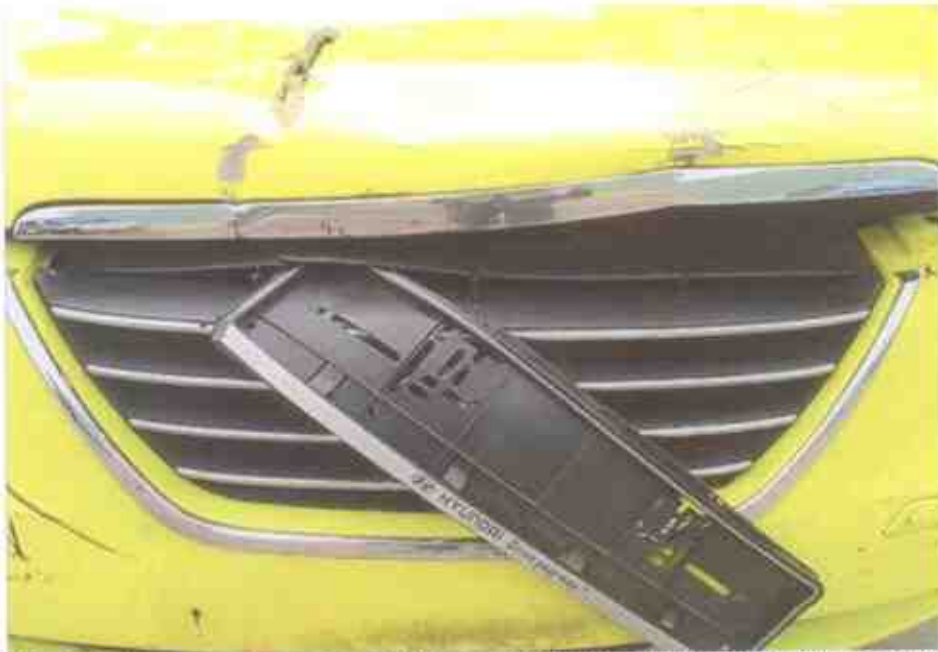
Photo 2 shows a closer view of the cracked front number plate holder of the Motor Taxi at the time of our inspection.
