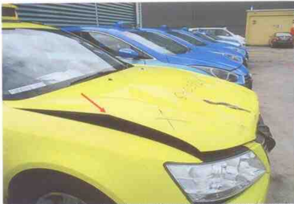
Photo 6 shows a closer view of the bent front bonnet of the Motor Taxi at the time of our inspection (arrowed).
