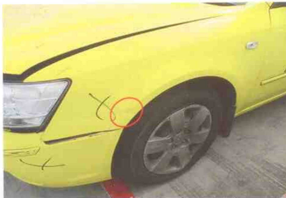
Photo 7 shows a closer view of the dent observed at the right side panel of the Motor Taxi at the time of our inspection (circled).
