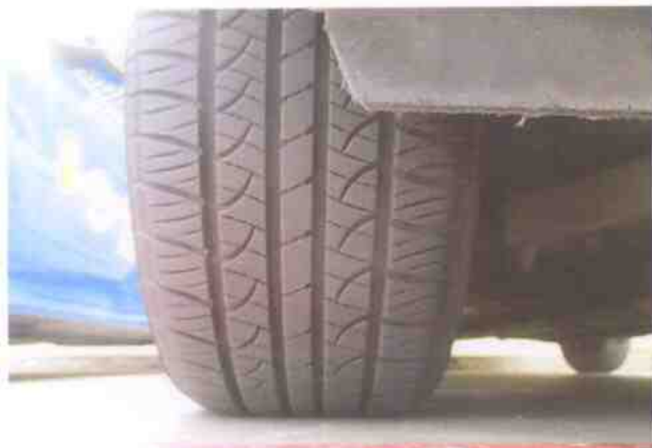
Photo 11 shows the condition of the rear left tyre of the Motor Taxi, which was observed to be in serviceable condition with remaining tread depth of approximately 6mm. The tyre, which was wrapped around standard wheel rim, was also observed to be sufficiently inflated for vehicular operation.
