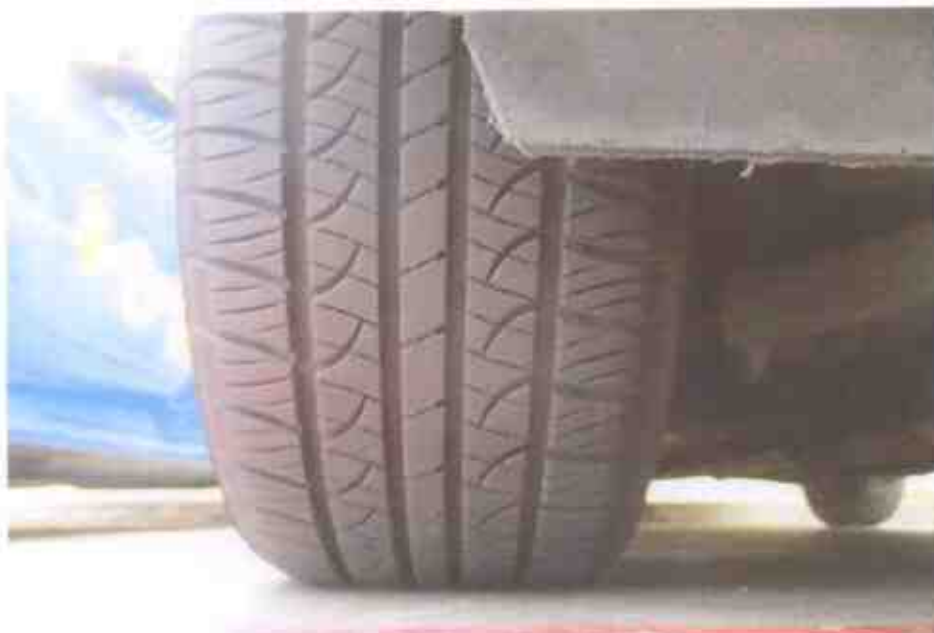
Photo 9 shows the condition of the front right tyre of the Motor Taxi, which was observed to be in serviceable condition with remaining tread depth of approximately 5mm. The tyre, which was wrapped around standard wheel rim, was also observed to be sufficiently inflated for vehicular operation. The 4 wheel caps fitted on the outer side of the wheel rims of the Motor Taxi were found to be with kerb grazing type of damage.
