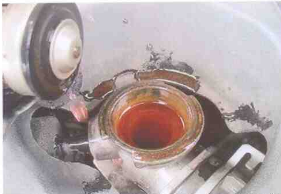
Photo 14 shows checks being carried out to the engine coolant of the Motor Taxi at the time of our inspection. The engine coolant was observed to be of sufficient level and without any visible contamination.
