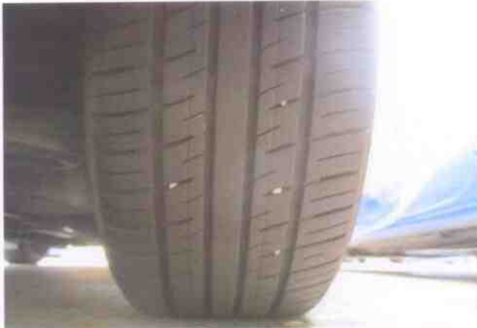
Photo 10 shows the condition of the rear right tyre of the Motor Taxi, which was observed to be in serviceable condition with remaining tread depth of approximately 6mm. The tyre, which was wrapped around standard wheel rim, was also observed to be sufficiently inflated for vehicular operation.
