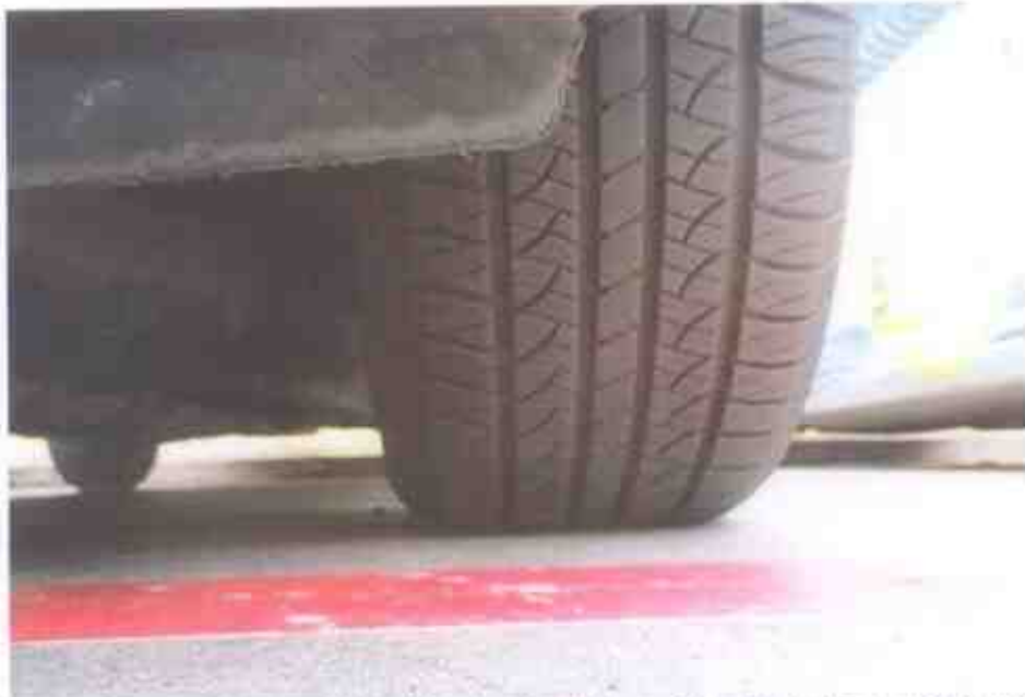
Photo 8 shows the condition of the front right tyre of the Motor Taxi, which was observed to be in serviceable condition with remaining tread depth of approximately 5mm. The tyre, which was wrapped around standard wheel rim, was also observed to be sufficiently inflated for vehicular operation.
