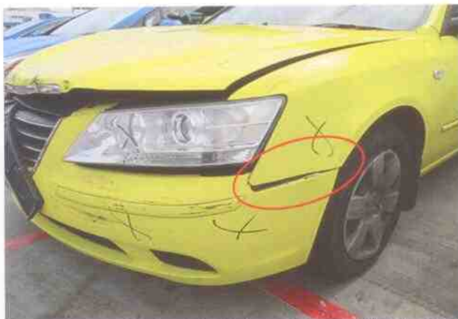
Photo 4 shows a closer view of the dislodgement observed at the left corner of the front bumper of the Motor Taxi at the time of our inspection (circled).
