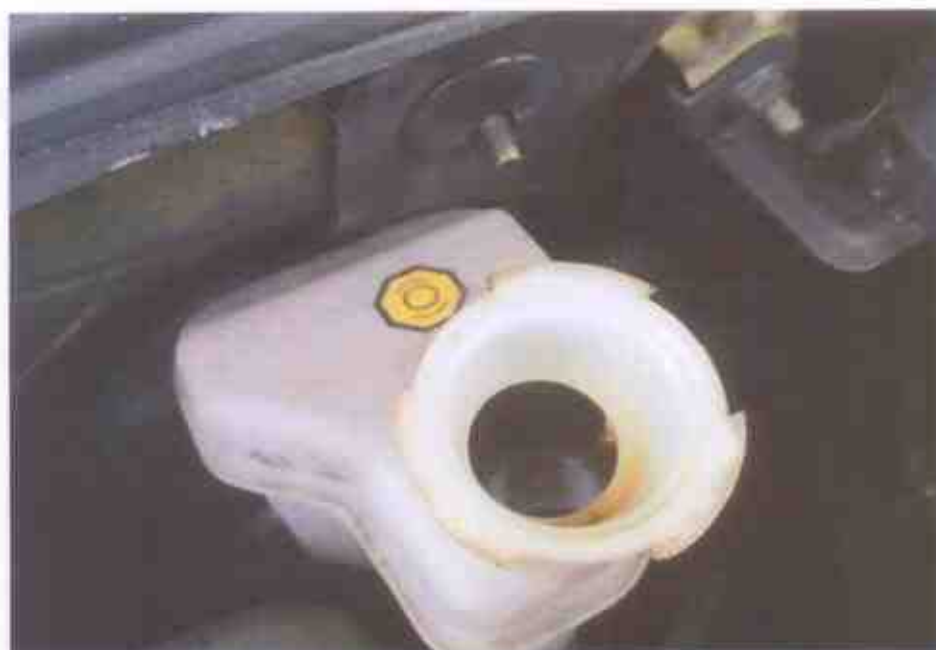
Photo 12 shows the brake fluid reservoir of the Motor Taxi at the time of our inspection. The brake fluid was observed to be of sufficient level and without any visible contamination.
