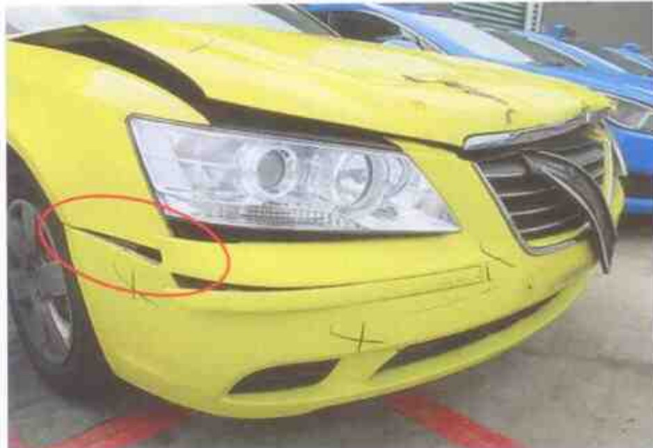
Photo 3 shows a closer view of the dislodgement observed at the right corner of the front bumper of the Motor Taxi at the time of our inspection (circled).
