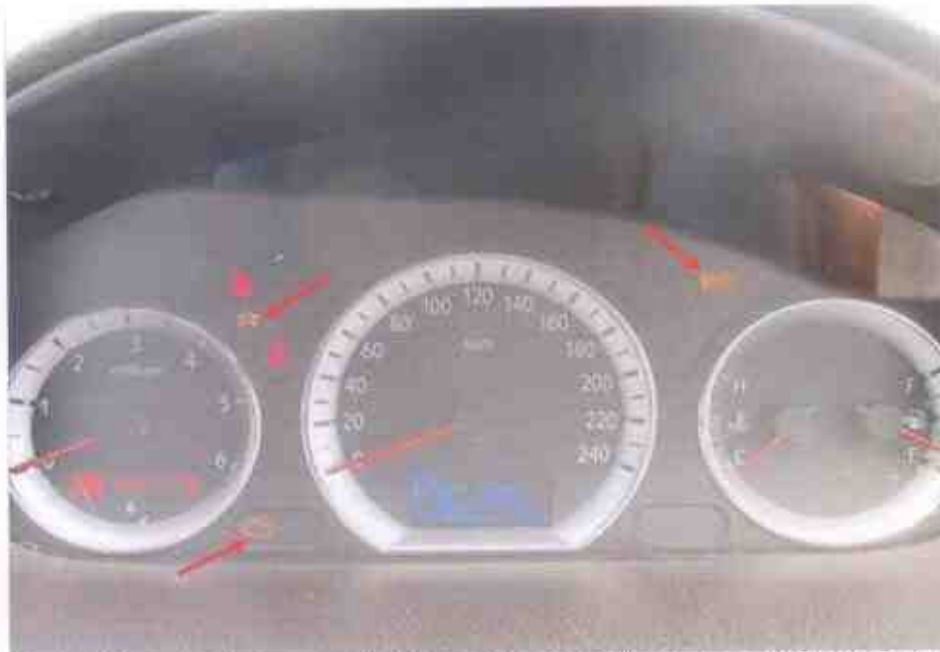
Photo 21 shows the warning lights for the various electronic operating systems and indicators of the Motor Taxi appearing on its instrument panel during the self-test when the engine is cranked, in particular the ABS light, glow plugs indicator and engine warning light (arrowed).
