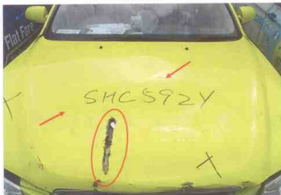
Photo 5 shows a closer view of the dents (arrowed) as well as a vertical tear (circled) observed on the front bonnet of the Motor Taxi at the time of our inspection.
