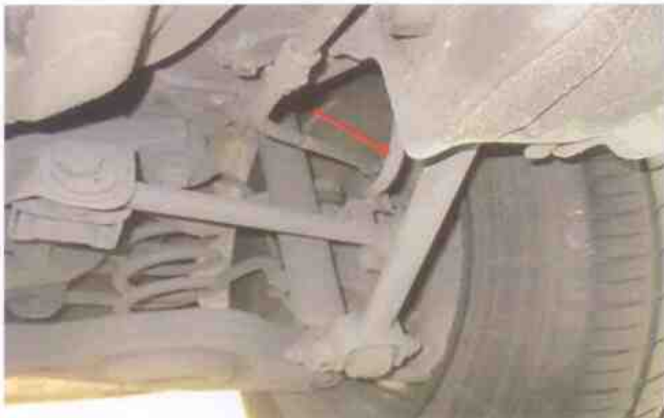
Photo 17 shows the brake hose/pipe (arrowed) at the rear left wheel of the Motor Taxi. We did not observe any leakage of brake fluid at the time of our inspection of the Motor Taxi. Static tests of the Motor Taxi's braking system had indicated that there was no internal leakage of pressure/vacuum. Hence the braking system was likely to be in serviceable condition at the material time of accident. The undercarriage components of the Motor Taxi were also all found to be intact and without any visible damage.
