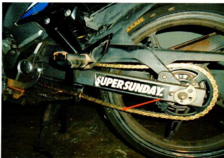
Photo 9 shows the general view of the gear train (arrowed) of the Motorcycle, which was observed to be intact with no misalignment. It was also adequately lubricated for operating purposes.
