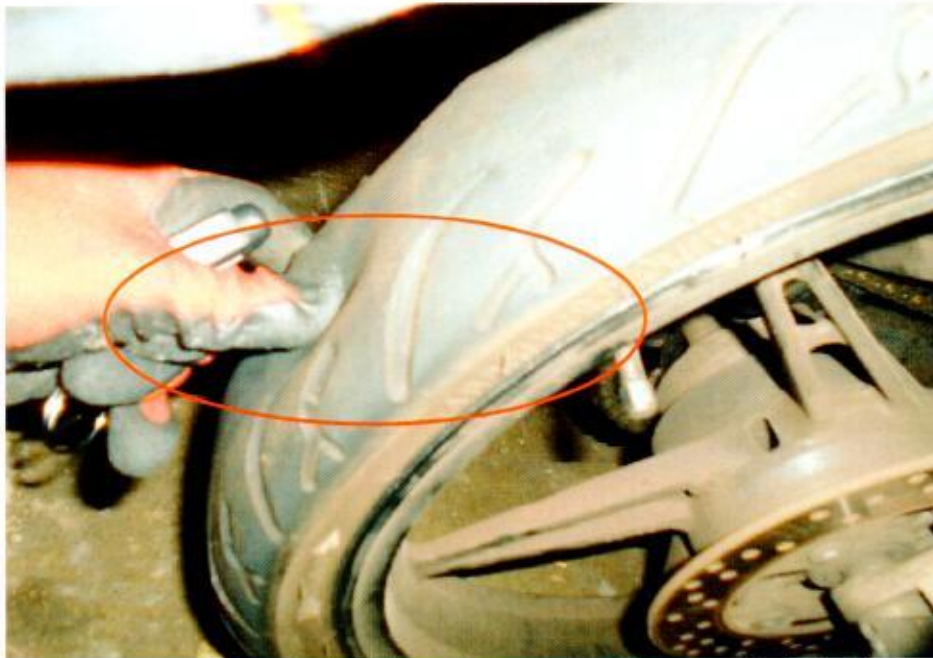
Photo 7 shows further observation on the rear tyre that was deflated at time of our inspection due to damage front rim likely caused by the accident collision impact.
