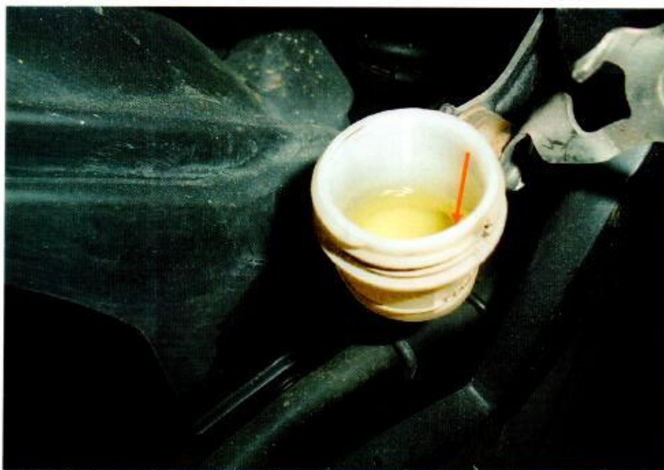
Photo 13 shows the rear brake fluid reservoir of the Motorcycle. It was found to be at a sufficient level at time our inspection.
