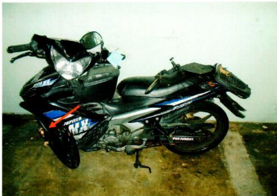
Photo 2 shows a general view of the front left body of the Motorcycle at the time of our inspection. The Motorcycle was observed to be sustained with relatively extensive impact due to the accident collision. Amongst the body parts damaged was its front fork (arrowed), which was observed to be bent inwards.
