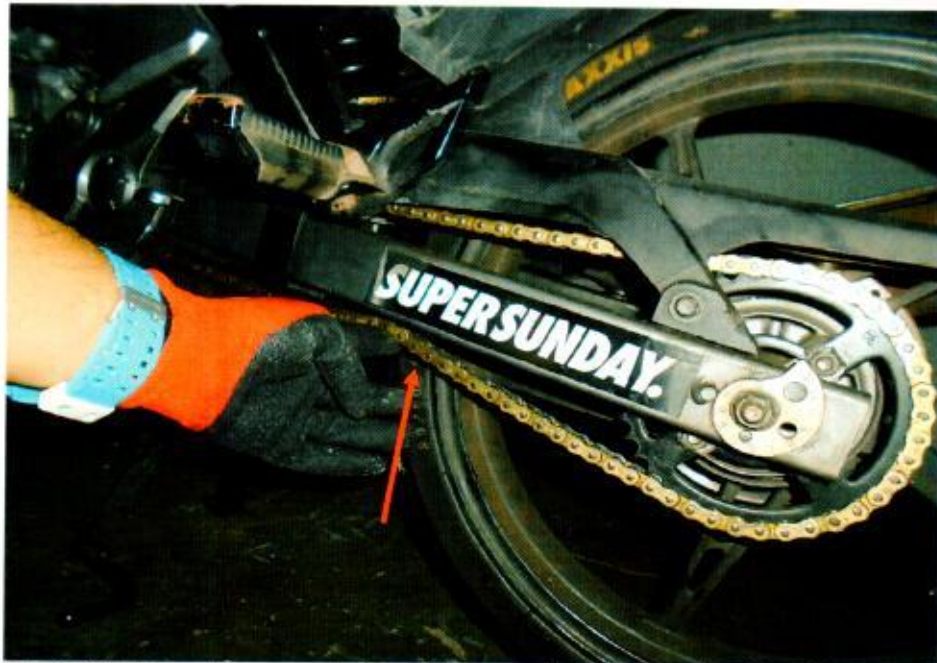
Photo 10 shows the general view of the gear train (arrowed) of the Motorcycle, which was observed to be intact with no misalignment. It was also adequately lubricated for operating purposes. Free play tension was also observed & found adequately acceptable.
