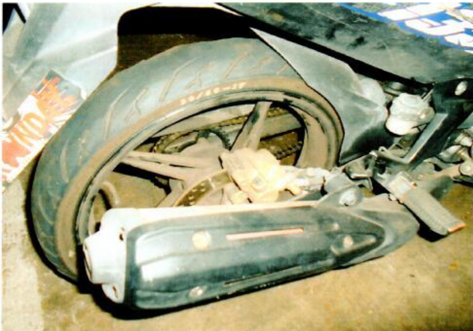
Photo 6 shows the rear tyre of the Motorcycle. The pattern of the tread was clearly visible. There was no tear, burst mark(s) and/or punctured hole(s) on the sidewalls as well as across the tread of the front tyre. Except further observation found that the rear tyre that was deflated likely due to the accident's collision impact.
