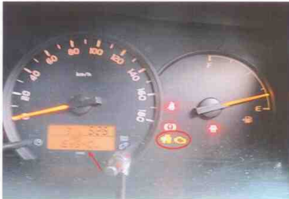
Photo 4 shows the 'brake override system failure' warning light and 'check engine' warning light that were still visible on the instrument panel of the Insured Vehicle (circled) after performing the short operational test of approximately 2km based on the odometer reading (arrowed). The results of the short operational test corroborated with Mr Joe's complaint, which is the gears of the transmission system could not be automatically shifted.
