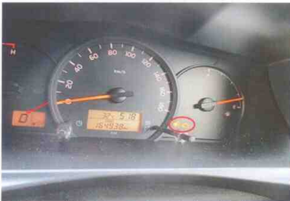
Photo 3 shows the brake 'override system failure' warning light and 'check engine' warning light that had appeared on the instrument panel of the Motor Bus (circled) after its engine was started and the gear was engaged to 'drive' mode (arrowed).
