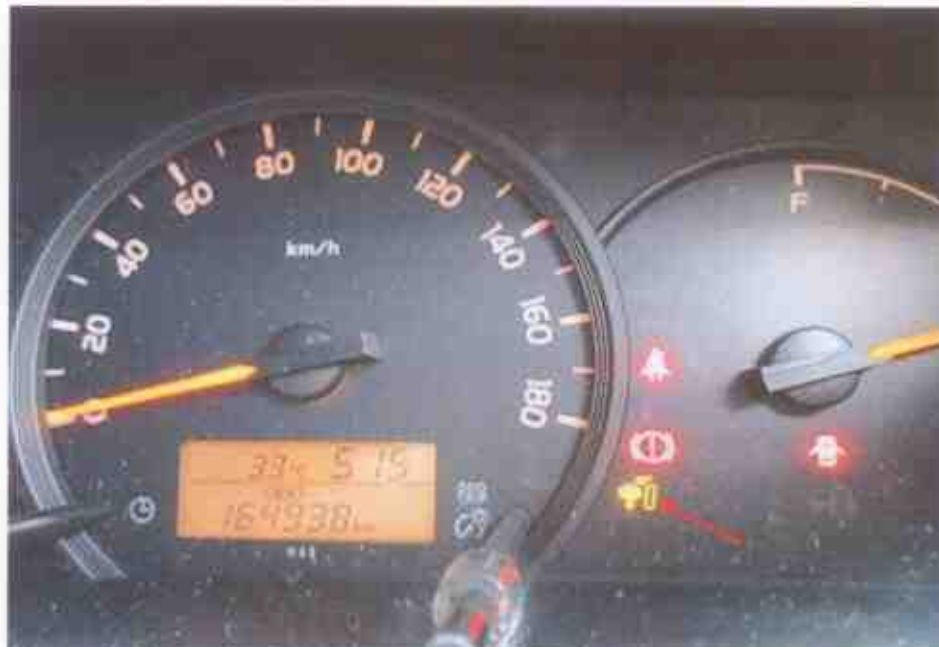
Photo 2 shows the 'brake override system failure' warning light that had appeared on the instrument panel of the Motor Bus after its ignition was switched on (arrowed).
