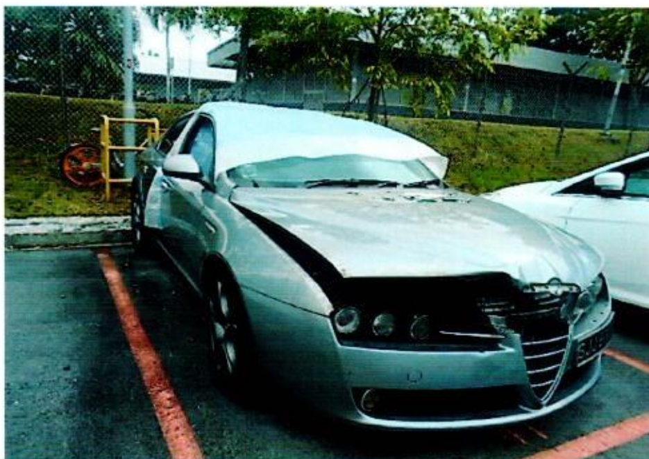
Photo 1 shows a general view of the front right body of the Insured Vehicle at the time of inspection. The Insured Vehicle was observed to have sustained fire damage at its frontal body. Its front bumper, front bonnet, front grille, front right headlamp and front right fender were amongst the body parts that were found to have been burnt as a result of the fire.
