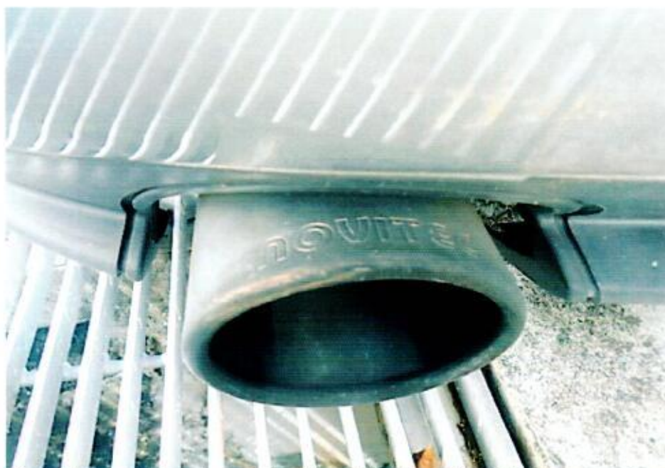
Photo 5 shows the rear exhaust muffler of the Insured Vehicle. The rear exhaust muffler fitted on the Insured Vehicle is non-original. The brand of the rear exhaust muffler was observed to be "Novitec".
