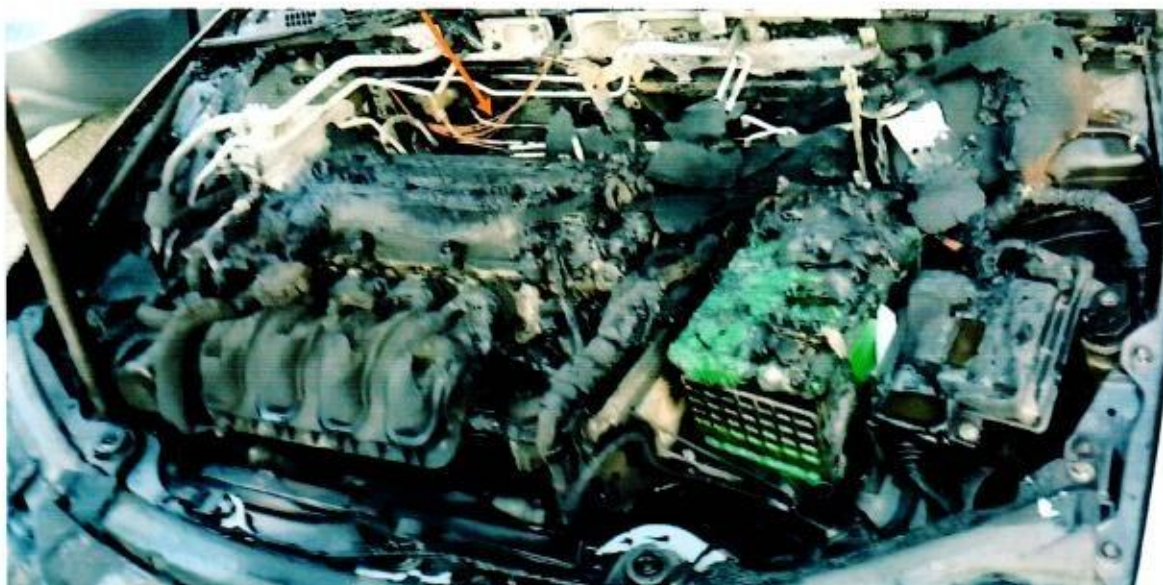
Photo 13 shows the engine compartment of the Insured Vehicle immediately after the fire was extinguished. This was from photographs taken by Mr Chan at the incident location. The same wirings (arrowed) as photograph 12 were noted to be bright reddish in colour immediately after the fire. Such condition suggest that the wirings were exposed to high heat, indicating internal heating of copper wires. This is a sign of an electrical short circuit occurring.
