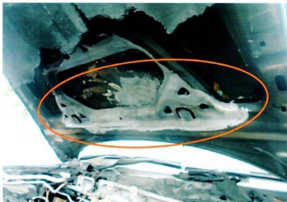
Photo 11 shows the whitish burn marks (circled) that were found on the underside of the front bonnet, directly above the firewall panel where similar high heat intensity burn marks (whitish burn marks) were found. This burn pattern to the underside of the front bonnet supports my comment of the fire originating at the rear centre area of the engine compartment of the Insured Vehicle.
