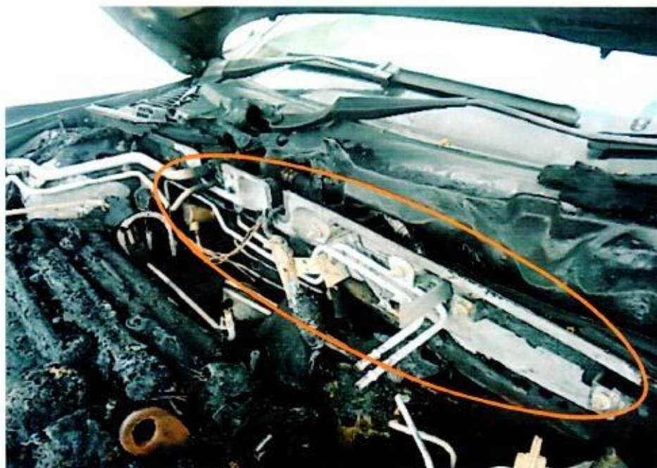
Photo 10 shows the whitish burn marks (circled) that were found on the firewall panel, towards the rear of the Insured Vehicle's engine compartment. Such whitish burn marks are a result of exposure to prolong heat intensity. The fire to the Insured Vehicle can then be established to have originated around the rear centre of the engine compartment.
