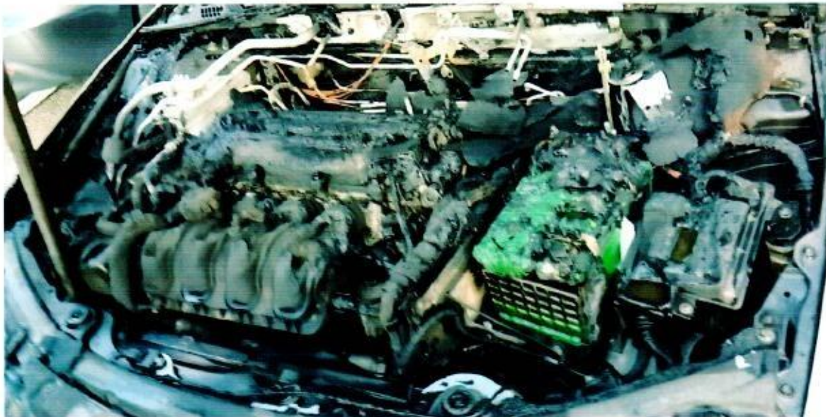
Photo 9 shows the engine compartment of the Insured Vehicle after the fire was extinguished by SCDF personnel. The damage of burnt nature to the Insured Vehicle had corresponded to the damages as seen by me during my inspection of the Insured Vehicle.
