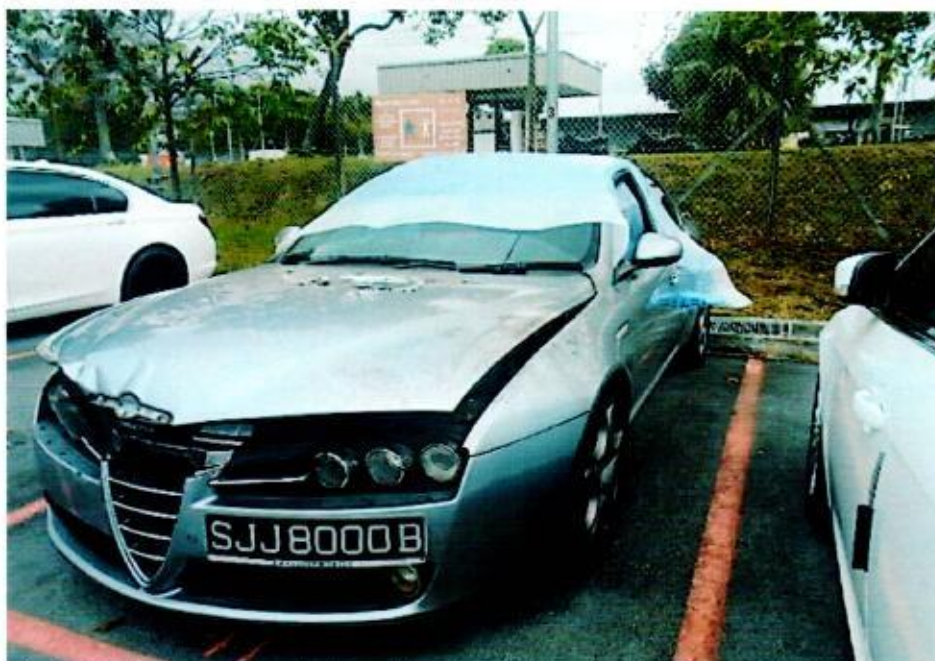
Photo 2 shows a general view of the front left body of the Insured Vehicle at the time of inspection. The Insured Vehicle was observed to have sustained fire damage at its frontal body. Its front bumper, front left fender, front left headlamp, front bonnet and front windscreen were amongst the body parts that were found to have been burnt as a result of the fire.
