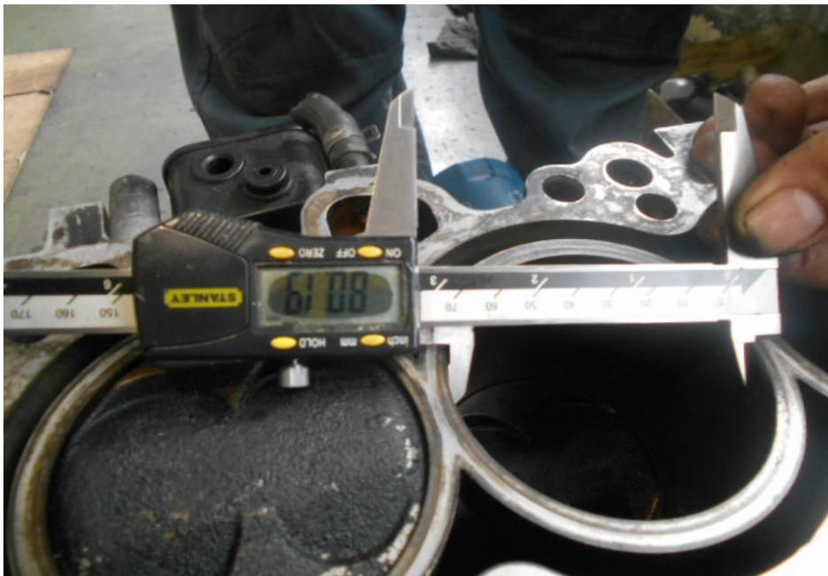
**Photo 12** shows measurement being carried out to the bore of cylinder 3 of the Honda engine. The bore and stroke measurements of the Honda engine were carried out using a digital Vernier Caliper. The bore measurement of cylinder 3 was recorded to be 80.19mm.
