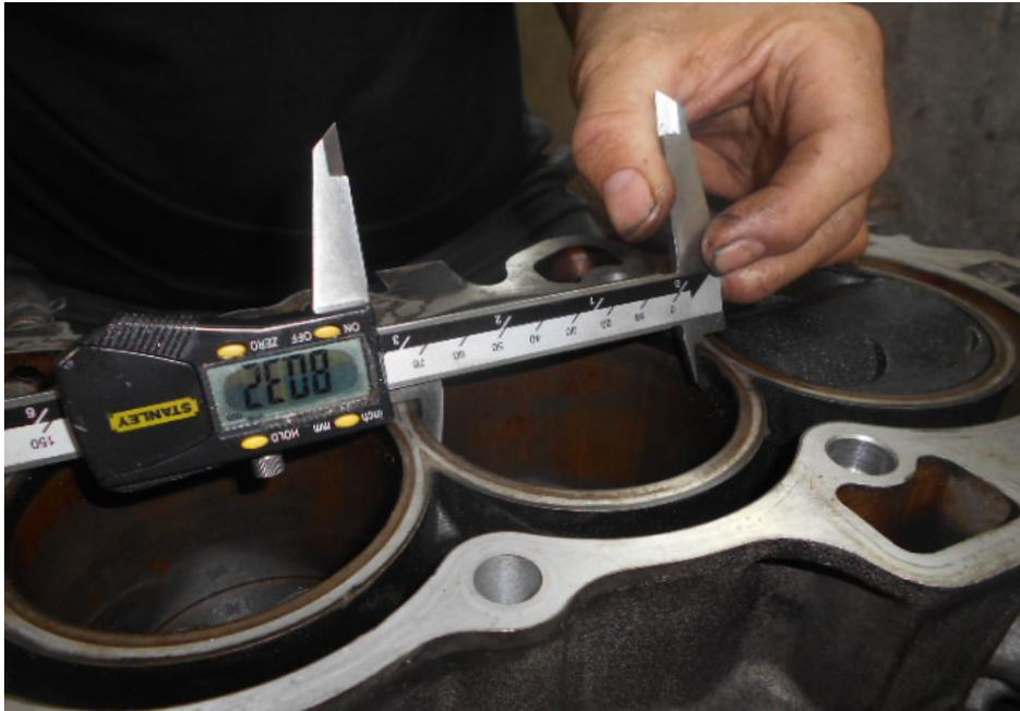
**Photo 9** shows measurement being carried out to the bore of cylinder 2 of the Honda engine. The bore measurement of cylinder 2 was recorded to be 80.32mm.
