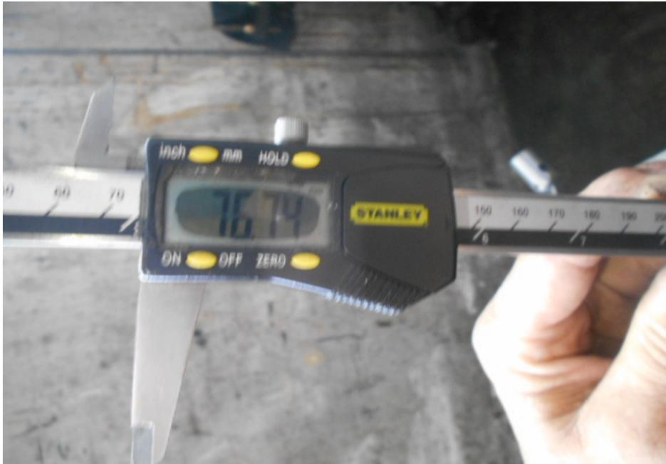
**Photo 11** shows the stroke measurement of cylinder 2, which was recorded to be 76.74mm.
