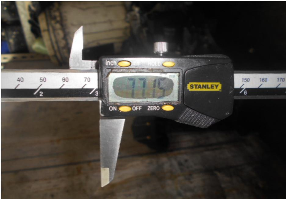
**Photo 8** shows the stroke measurement of cylinder 1, which was recorded to be 77.15mm.
