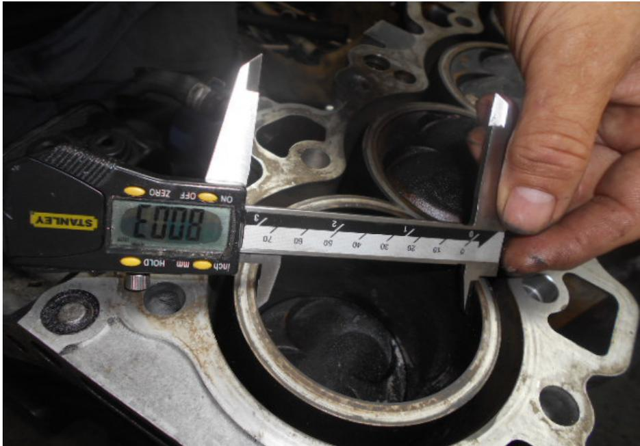
**Photo 15** shows measurement being carried out to the bore of cylinder 4 of the Honda engine. The bore and stroke measurements of the Honda engine were carried out using a digital Vernier Caliper. The bore measurement of cylinder 4 was recorded to be 80.03mm.
