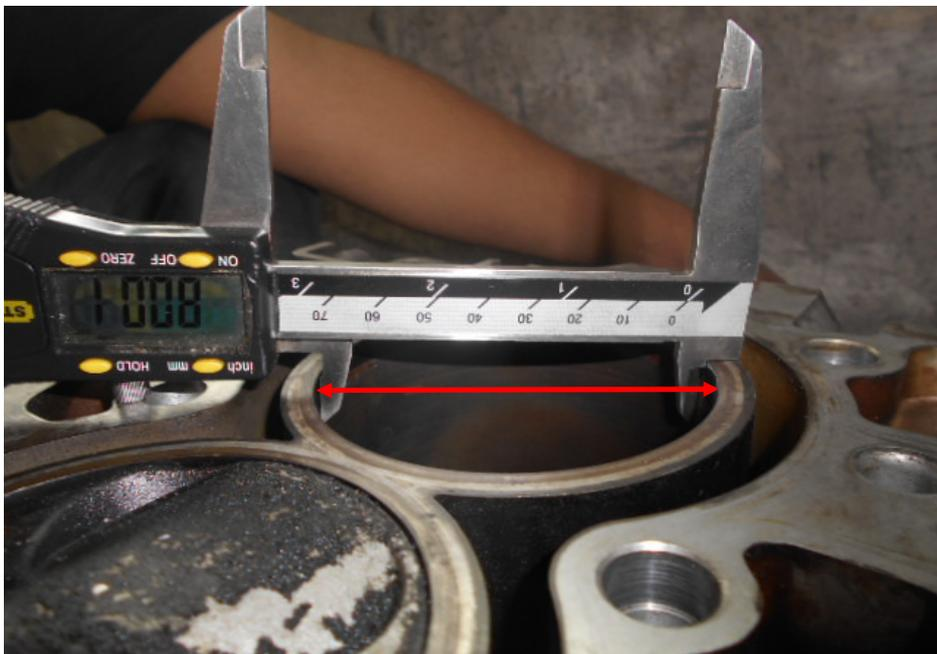
**Photo 6** shows measurement being carried out to the bore of cylinder 1 of the Honda engine. The bore measurement of cylinder 1 was recorded to be 80.01mm.
