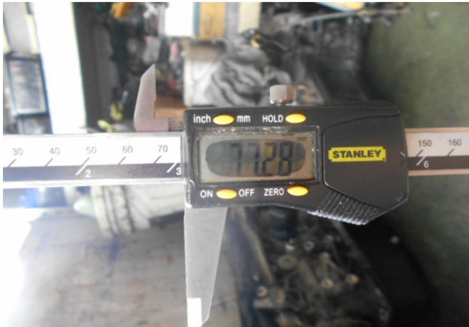
**Photo 17** shows the stroke measurement of cylinder 4, which was recorded to be 77.28mm.
