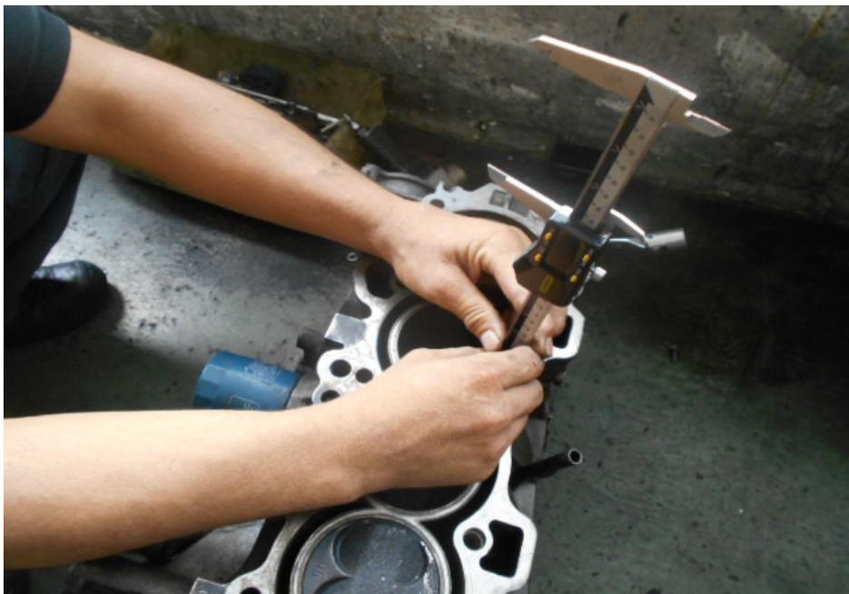
**Photo 10** shows measurement of the stroke of cylinder 2 of the Honda engine that I had inspected.
