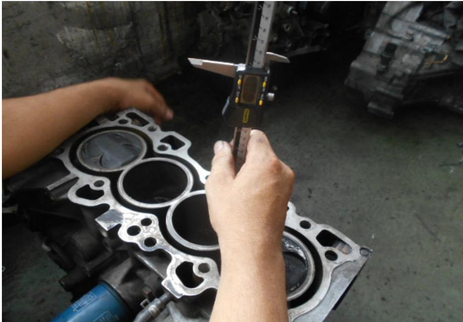
**Photo 13** shows measurement of the stroke of cylinder 3 of the Honda engine that I had inspected. The bore and stroke measurements of the Honda engine were carried out using a digital Vernier Caliper that was calibrated before the start of measurements.
