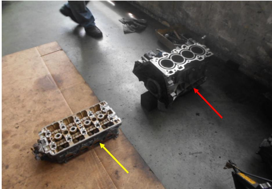
**Photo 1** shows a general view of the Honda engine that I had inspected. The Honda engine was observed to be a used engine and was not fitted on any motor car. The top block (yellow arrow) of the Honda engine was separated from its bottom block (red arrow). This was to enable me to carry out measurements of its cylinders, in particular the bore and stroke measurements of each cylinder, which typically can be used to determine the engine displacement or more commonly referred to as engine cc.
