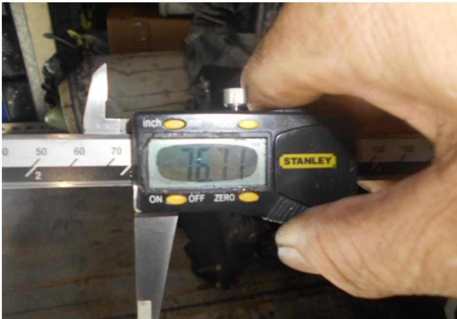
**Photo 14** shows the stroke measurement of cylinder 3, which was recorded to be 76.71mm.
