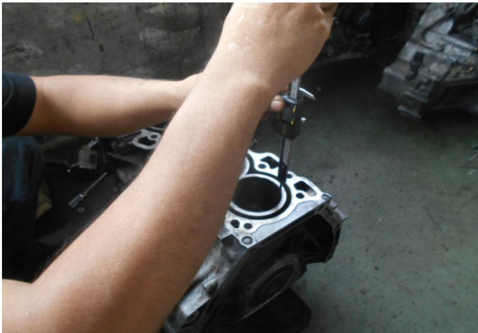
**Photo 16** shows measurement being carried out to the stroke of cylinder 4 of the Honda engine. The bore and stroke measurements of the Honda engine were carried out using a digital Vernier Caliper that was calibrated before the start of measurements.
