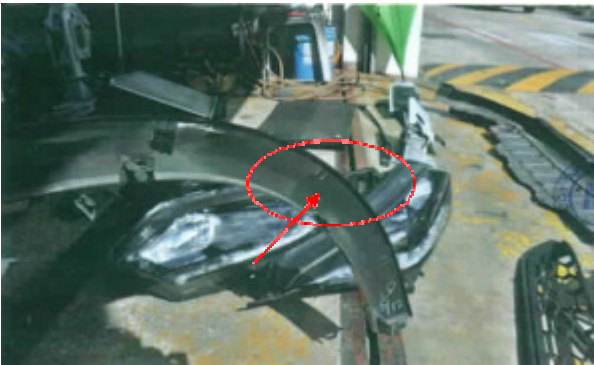
Fender arch garnish Torn/Deformed
