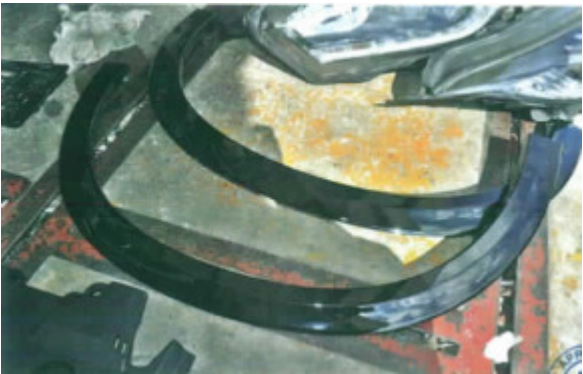
Front n/s fender, arch garnish retainer give way, have impact.
