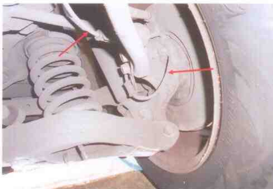
Photo 26 shows the braking components at the rear left wheel of the Motor Taxi. We did not observe any leakage of brake fluid at the time of our inspection of the Motor Taxi.
