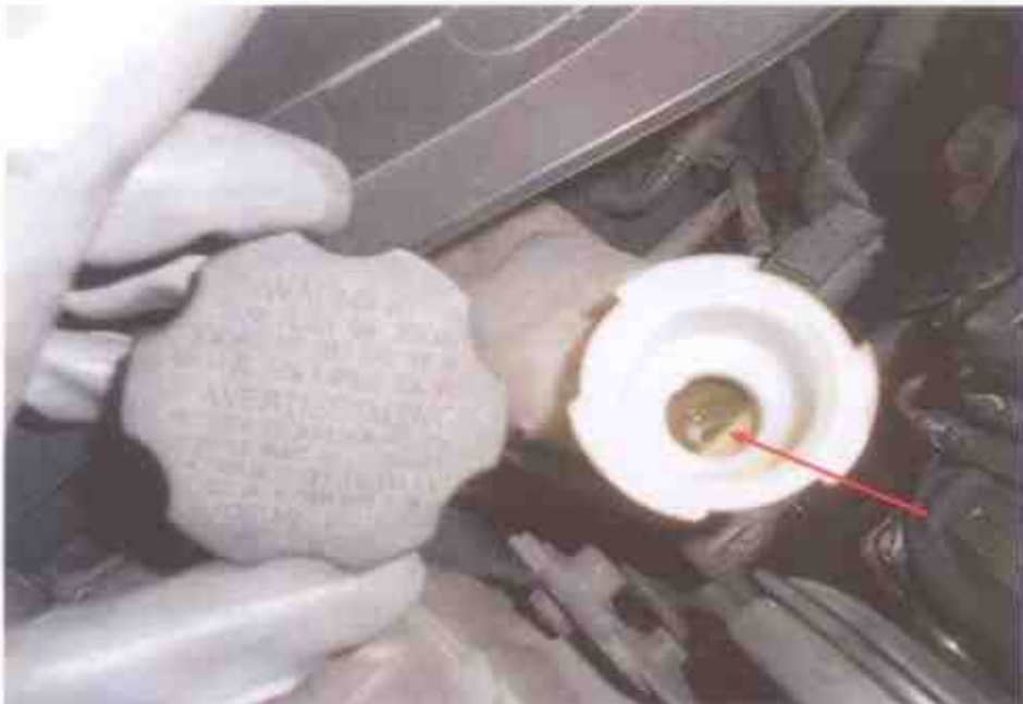
Photo 16 shows the close up view of the brake fluid that was seen with sufficient level not affected by the accident's impact.
