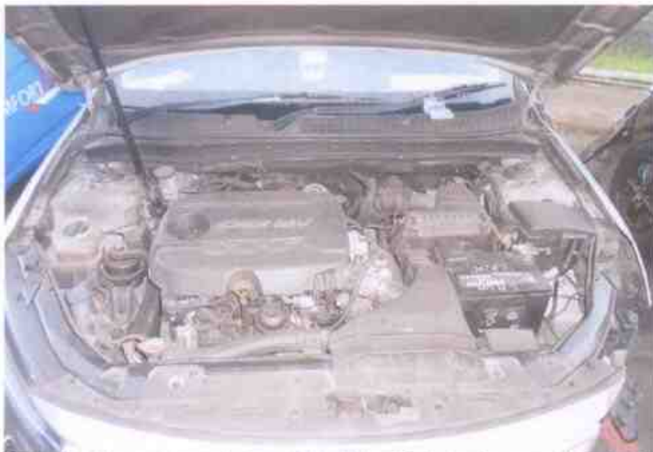
Photo 14 shows a general view of the Motor Car's engine compartment. The various parts and components inside the engine compartment were unaffected by the accident. There was also no sign(s) or indication(s) of fluid leakage and/or fluid stain within the engine compartment.
