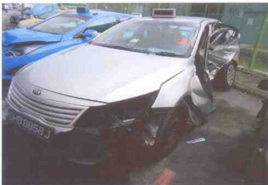
Photo 3 shows a general view of the front left portion of the Motor Taxi at the time of our inspection. The Motor Taxi was observed to have sustained extensive impact damage at its front left portion.
