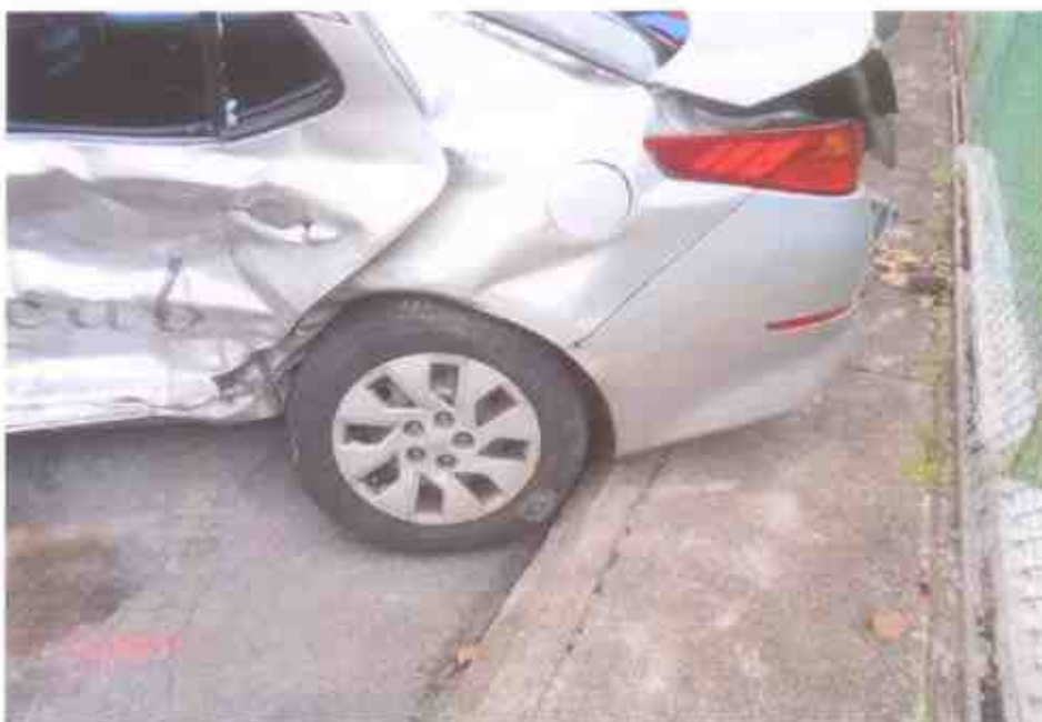
Photo 7 shows a closer view of the damaged rear boot lid. The impact force was significant, causing it to be misaligned due to the accident's impact.
