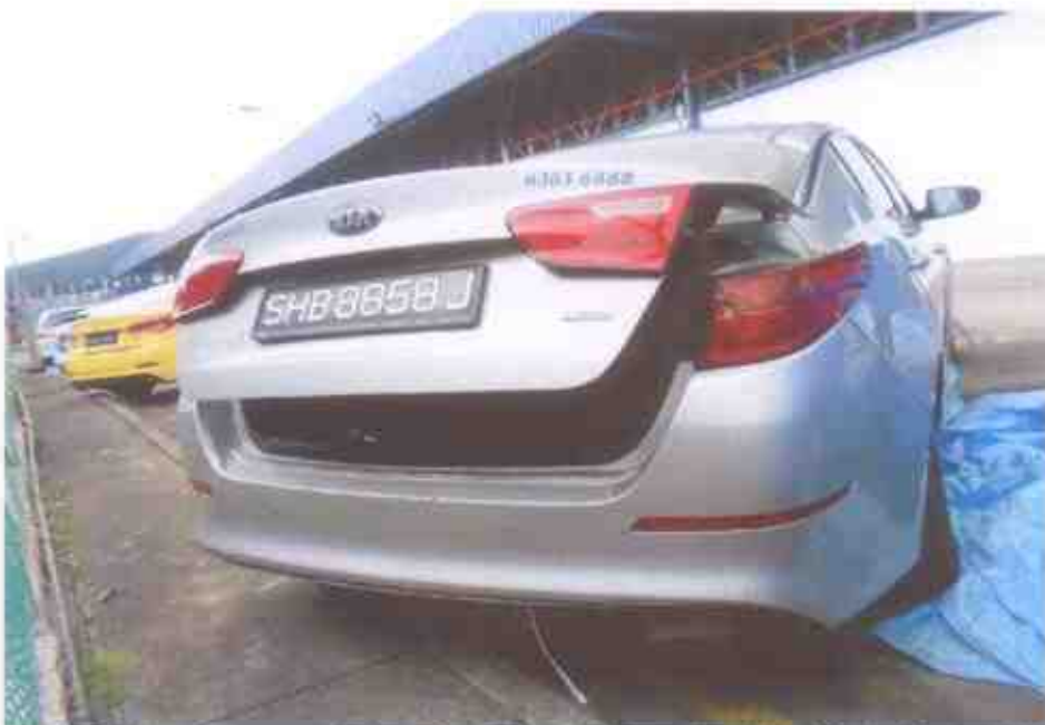
Photo 9 shows a general view of the rear right portion of the Motor Taxi at the time of our inspection. The rear portion was observed to have minor misalignment by the accident.
