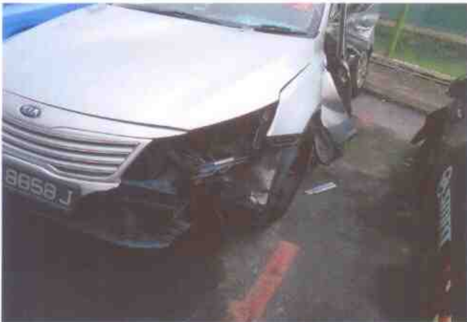
Photo 5 shows a closer view of the damage sustained on the front left of the Motor Taxi. The impact force was significant, causing the various parts and components inside the engine compartment to be damaged.
