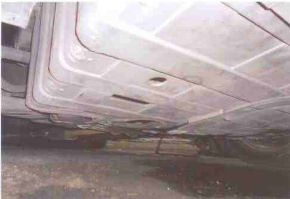
Photo 20 shows the undercarriage of the engine area. It was observed to be unaffected by the accident's impact.
