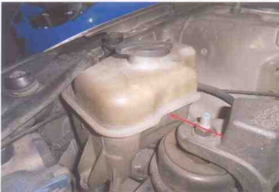
Photo 18 shows the close up view of the engine coolant reservoir that was seen with sufficient level not affected by the accident's impact.
