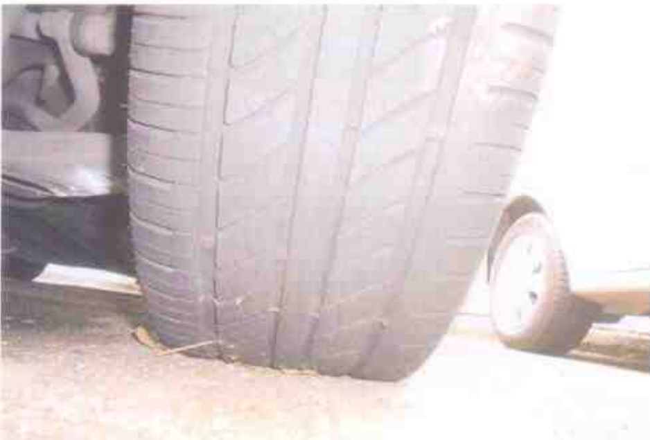
Photo 11 shows the condition of the front left tyre of the Motor Taxi, which was observed to be in serviceable condition with remaining tread depth of approximately 4mm. There was no tear, cut or burst mark(s) on the outer and the inner sidewalls as well as across the tread of this tyre, which was also sufficiently inflated for vehicular operation.
