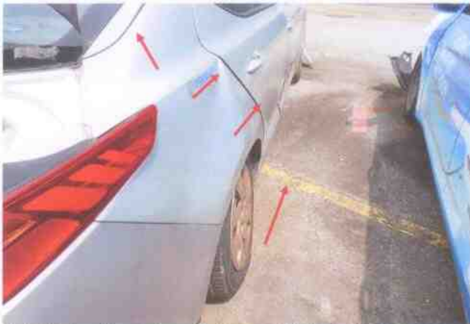
Photo 22 shows the misalignment at the rear right wheel of the Motor Taxi as a result of the accident's impact collision.
