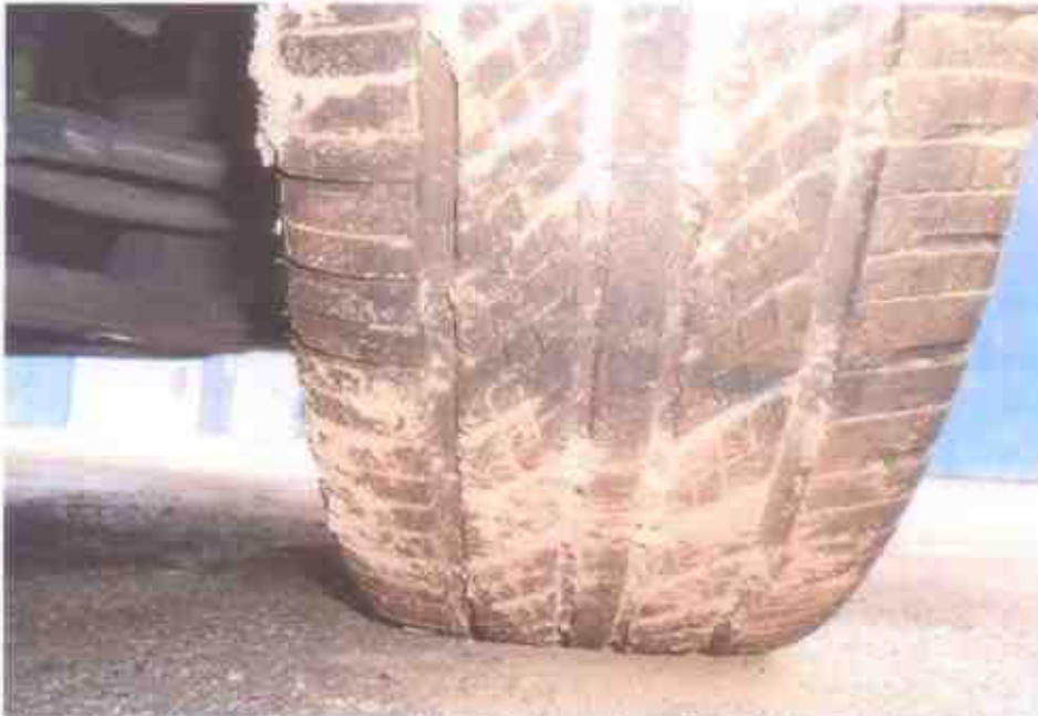
Photo 10 shows the condition of the front right tyre of the Motor Taxi, which was observed to be in serviceable condition with remaining tread depth of approximately 3mm. There was no tear, cut or burst mark(s) on the outer and the inner sidewalls as well as across the tread of this tyre.
