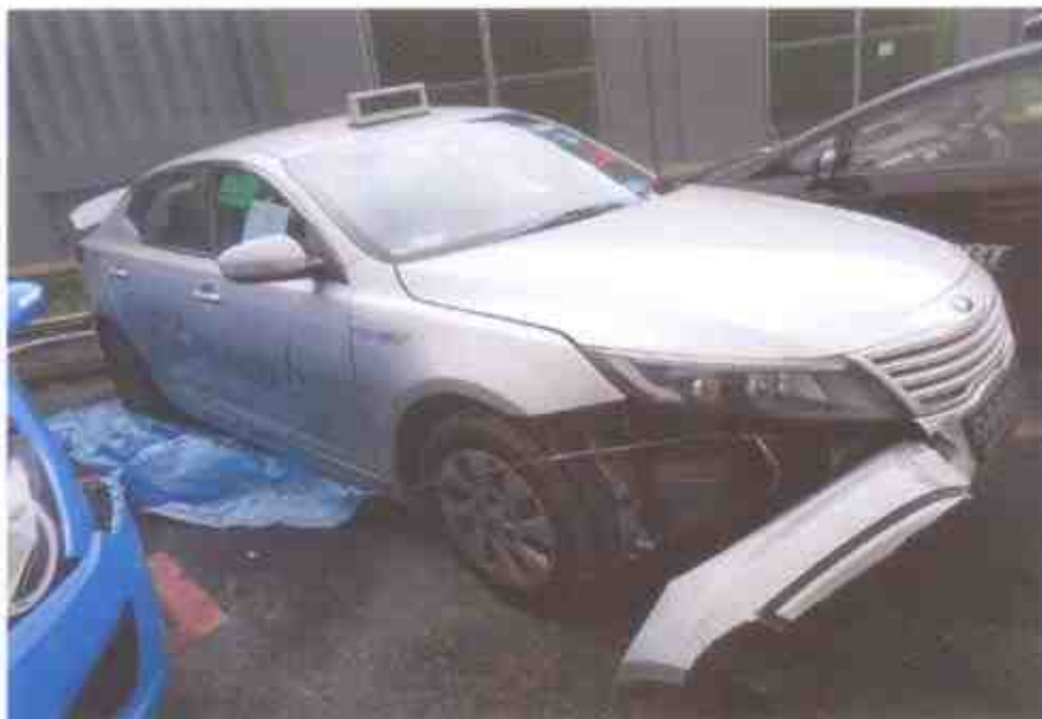
Photo 2 shows a general view of the front right portion of the Motor Taxi at the time of our inspection. The Motor Taxi was observed to have sustained extensive impact damage at its front right portion.
