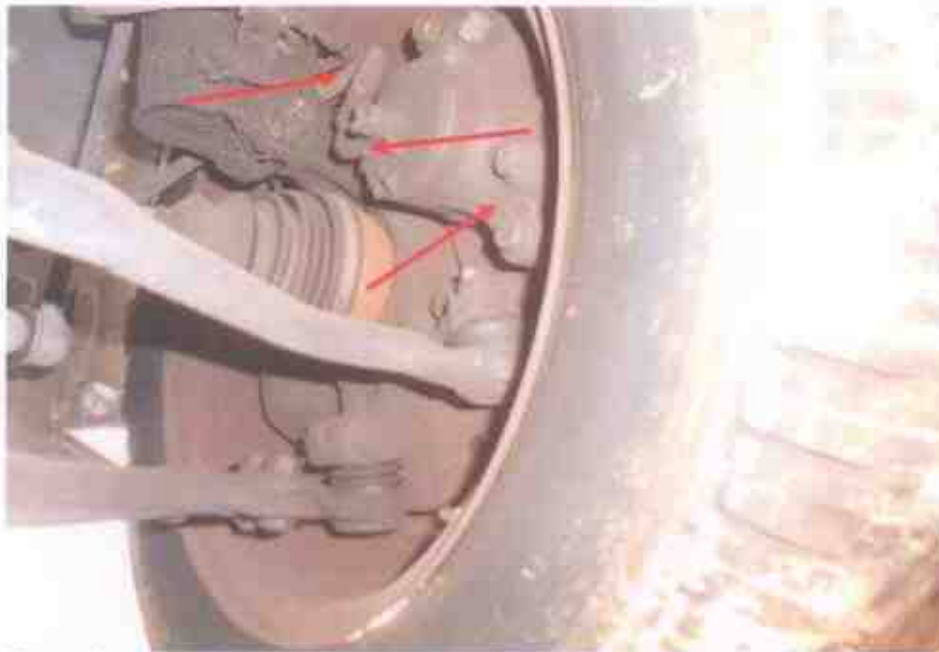
Photo 24 shows the braking components at the front right wheel of the Motor Taxi. We did not observe any leakage of brake fluid at the time of our inspection of the Motor Taxi.
