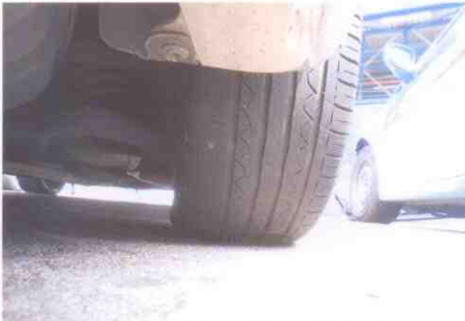
Photo 12 shows the condition of the rear right tyre of the Motor Taxi, which was observed to be in serviceable condition with remaining tread depth of approximately 4mm. There was also no tear, cut or burst mark(s) on the outer and the inner sidewalls as well as across the tread of this tyre.
