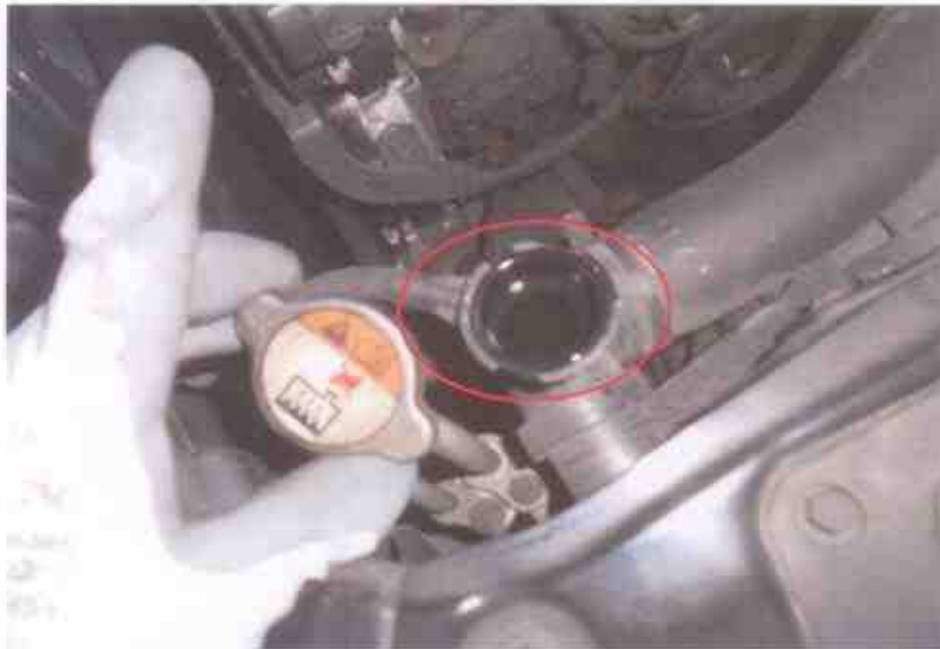
Photo 15 shows the close up view of the engine coolant that was seen with sufficient level not affected by the accident's impact.
