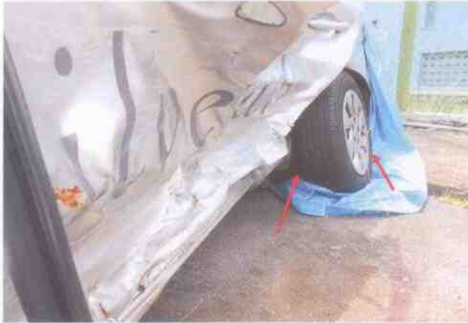
Photo 21 shows the misalignment at the rear left wheel of the Motor Taxi.
