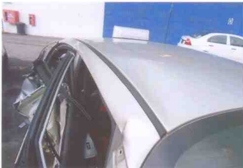
Photo 6 shows a closer view of the Motor Taxi roof top. The impact force was significant, causing it to be corrugated.
