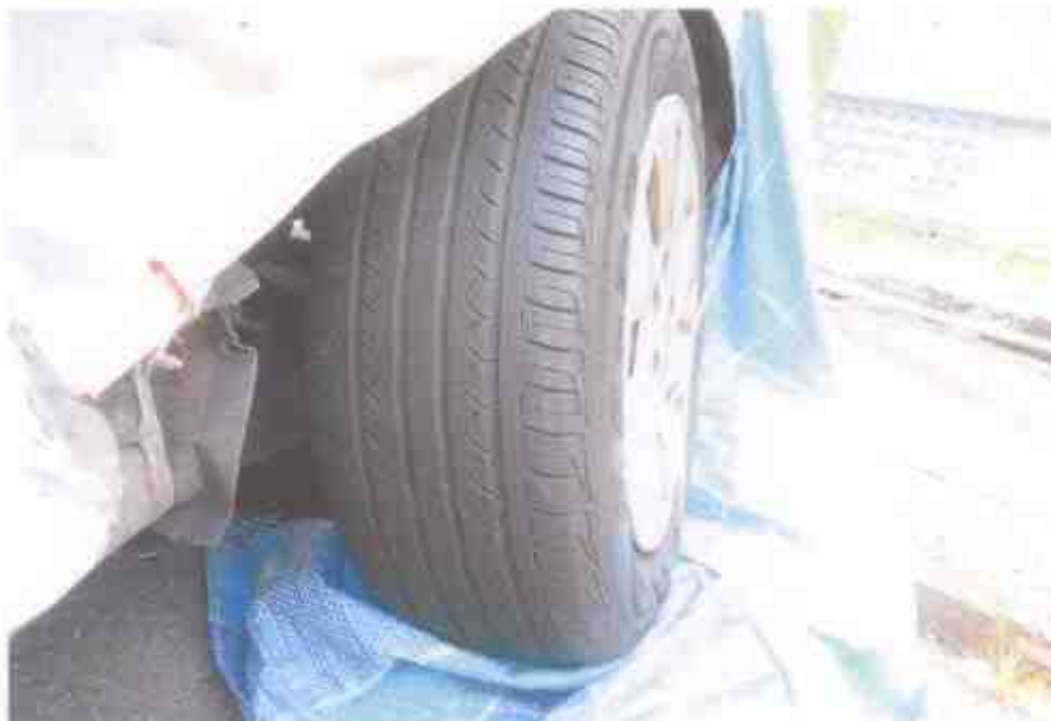
Photo 13 shows the condition of the rear left tyre of the Motor Taxi, which was observed to be in serviceable condition with remaining tread depth of approximately 3mm. There was also no tear, cut or burst mark(s) on the outer and the inner sidewalls as well as across the tread of this tyre.
