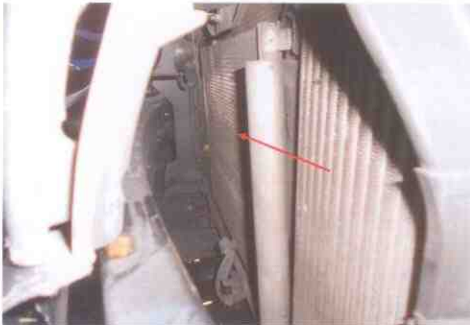
Photo 17 shows the close up view of the radiator that was not affected by the accident's impact
