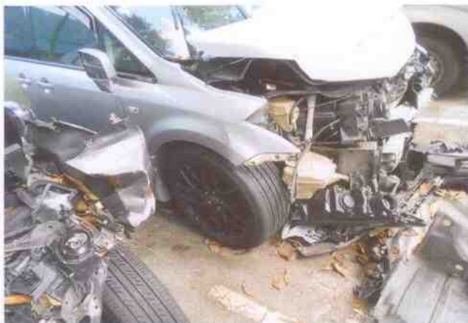
Photo 5 shows a closer view of the damage at the frontal right portion of the Motor Car. The impact force was significant, causing the various parts and components inside the engine compartment to be pushed inwards, towards the rear of the Motor Car.
