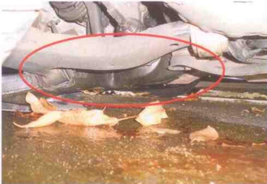
Photo 21 shows the close up view of the fluid leakage at the undercarriage area likely due to the accident impact.
