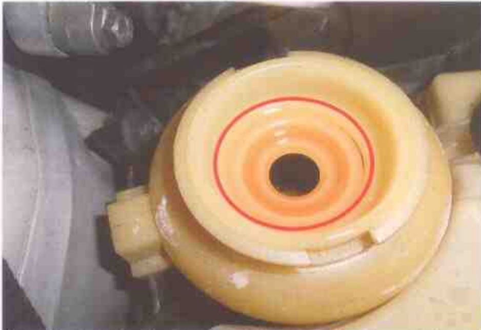
Photo 19 shows the close up view of the steering fluid reservoir that was insufficient (leakage) likely due to the accident impact.
