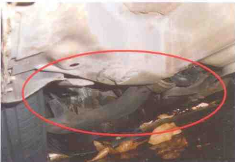
Photo 20 shows the close up view of the fluid leakage at the undercarriage area likely due to the accident impact.
