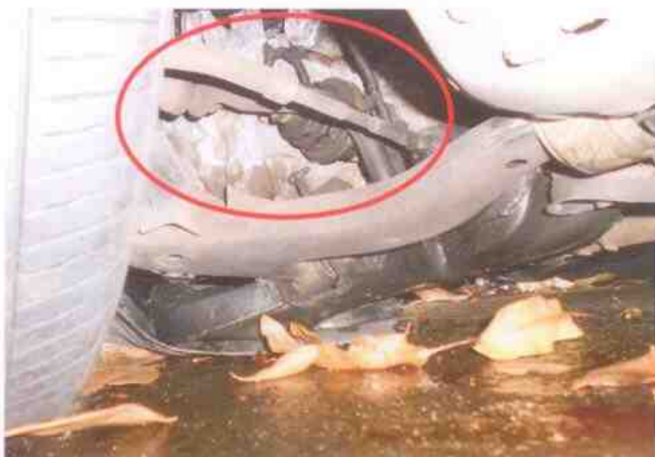
Photo 22 shows a close up view on the front right drive shaft of the Motor Car. We were not able to conduct any tests on the steering system of the Motor Car due to the damage to this components, as well as leakage of power steering fluid.
