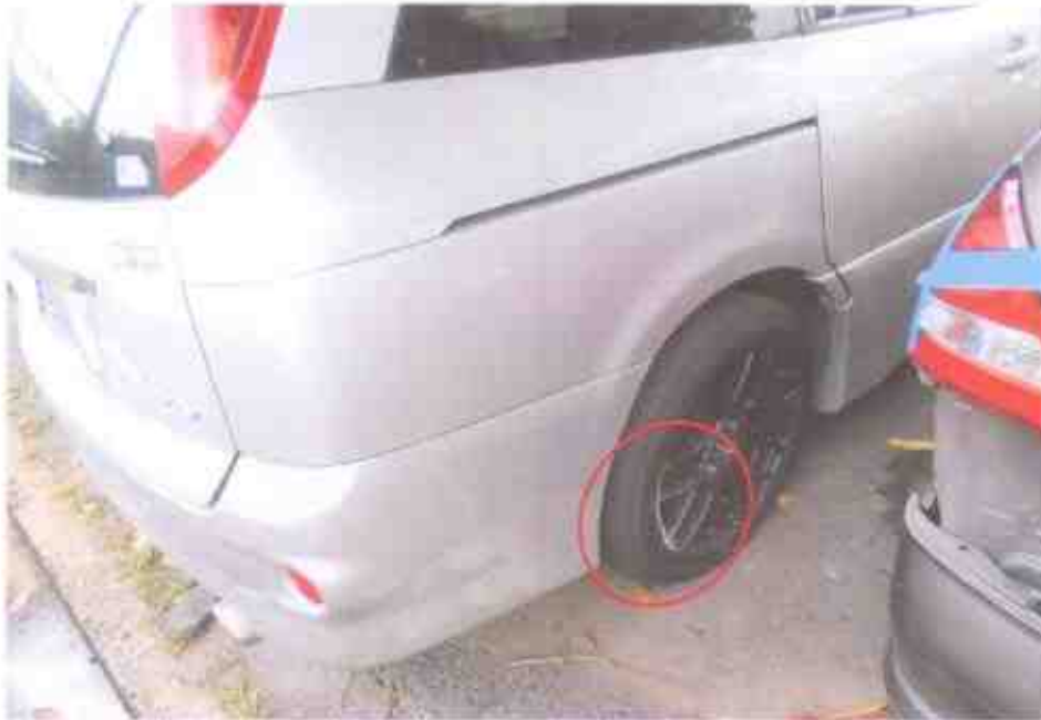
Photo 12 shows the general condition of the rear right tyre of the Motor Car. The alloy rim was observed to be chipped off at the side due to the accident's impact.
