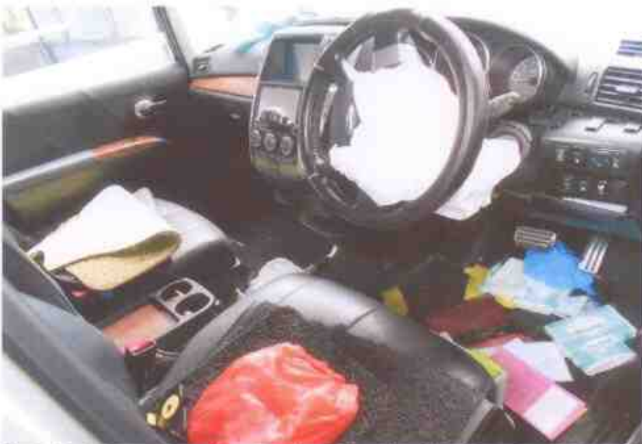
Photo 7 shows a closer view of the interior cabin of the Motor Car. The impact force didn't cause damages to the interior cabin. However, it activated both driver's & passenger's airbag at time of impact.
