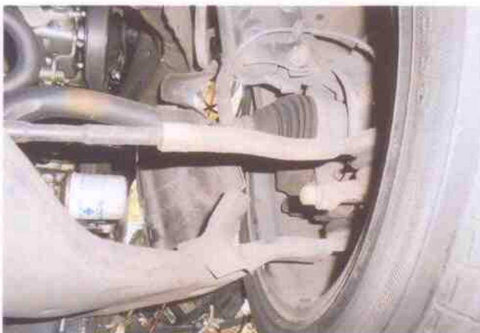
Photo 26 shows the braking & steering components at the front right wheel of the Motor Car. We did not observe any leakage of brake fluid at the time of our inspection of the Motor Car. However, the steering system was observed to be damaged due to the accident's impact.
