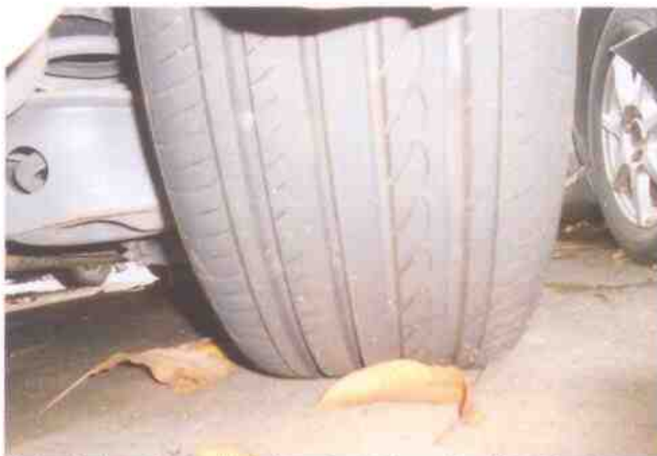
Photo 14 shows the condition of the rear right tyre of the Motor Car. The tread patterns were obvious visually. The remaining tread depth of the rear right tyre was approximately 8mm.
