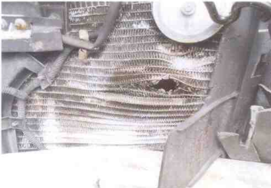
Photo 6 shows a closer view of the damage at the frontal portion of the Motor Car. The impact force was significant, causing extensive damage to the radiator.
