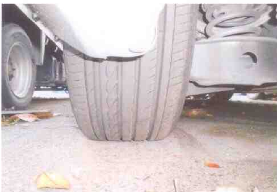
Photo 15 shows the condition of the rear left tyre of the Motor Car. The tread patterns were obvious visually. The remaining tread depth of the rear left tyre was approximately 6mm.
