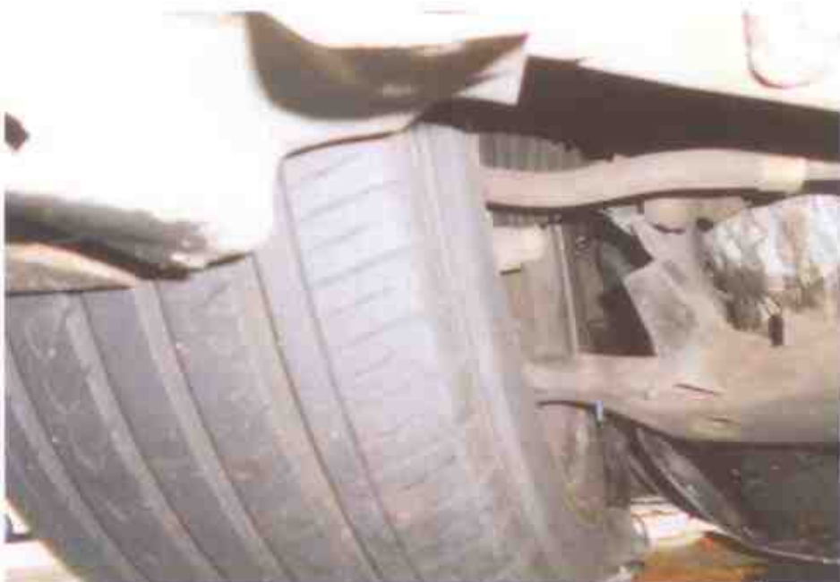
Photo 17 shows the condition of the front left tyre of the Motor Car. The tread patterns were obvious visually. The remaining tread depth of the front left tyre was approximately 6mm.
