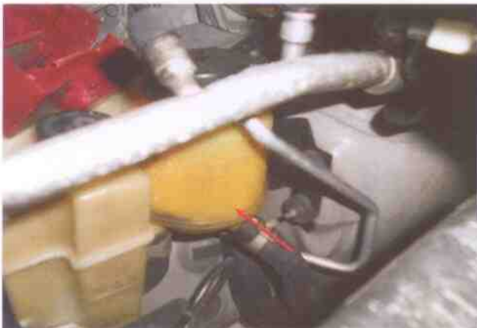
Photo 23 shows the power steering fluid reservoir of the Motor Car was observed to be insufficient level due to leakage of fluids.
