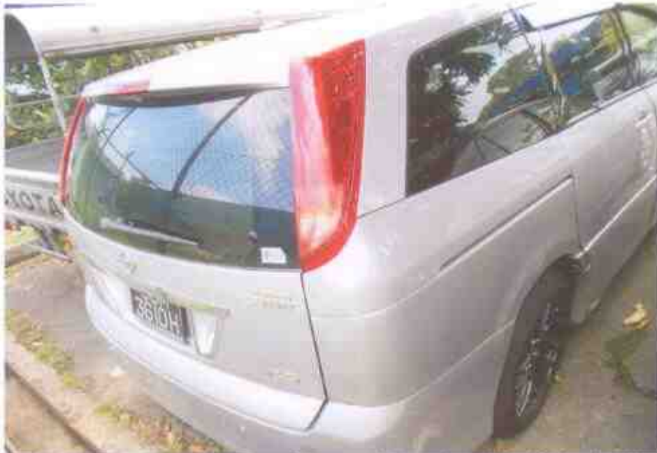
Photo 10 shows a general view of the rear right portion of the Motor Car. The rear portion was observed to be in good condition, no damages found on the Motor Car's body at time of our inspection. However, we found that the rear right tyre was deflated due to the accident.
