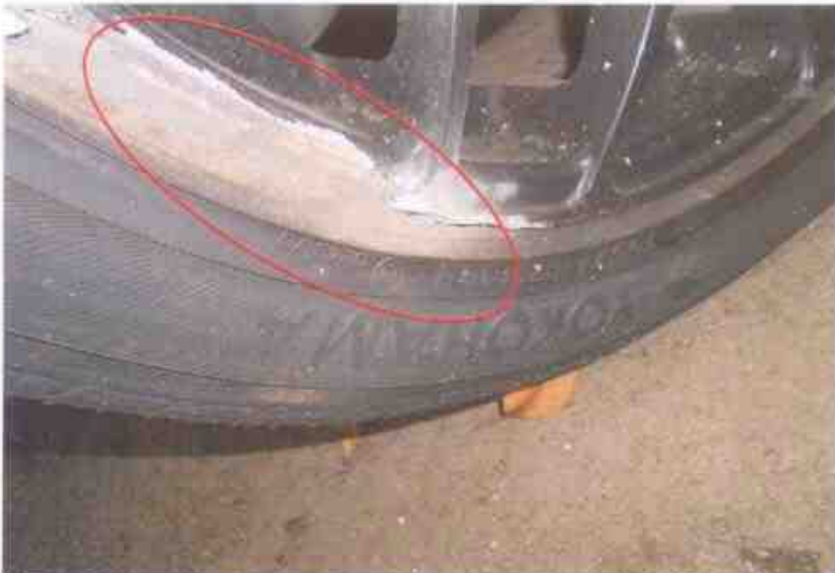
Photo 13 shows the close-up view of the rear right tyre of the Motor Car. The alloy rim was observed to be chipped off at the side due to the accident's impact.
