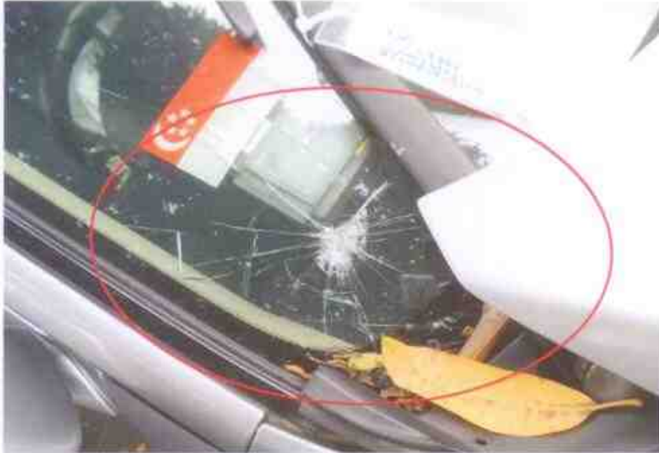
Photo 8 shows a closer view of the damage at the windscreen area of the Motor Car. The impact force was significant, causing the windscreen to sustain cracked.
