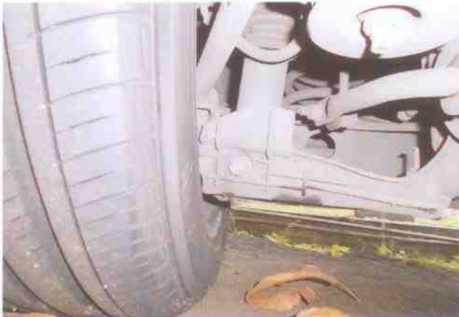
Photo 24 shows the braking & steering components at the rear right wheel of the Motor Car. We did not observe any leakage of brake fluid at the time of our inspection of the Motor Car.
