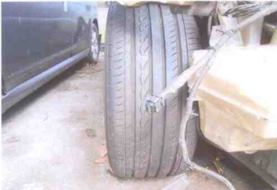
Photo 16 shows the condition of the front right tyre of the Motor Car. The tread patterns were obvious visually. The remaining tread depth of the rear left tyre was approximately 6mm.
