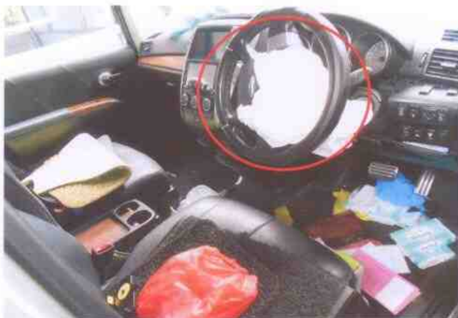
Photo 28 shows the Supplemental Restraint System (SRS) of the Motor Car was however likely to be in normal operating condition at the material time of the accident. The evidence of the deployed driver's airbag indicates that the impact sensors and control module of the Motor Car's SRS were all in serviceable condition at the material time of accident.
