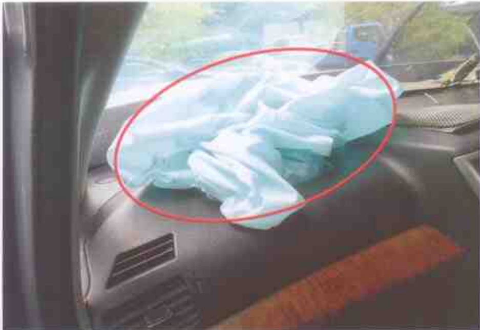
Photo 29 shows the Supplemental Restraint System (SRS) of the Motor Car was however likely to be in normal operating condition at the material time of the accident. The evidence of the deployed front passenger's airbag indicates that the impact sensors and control module of the Motor Car's SRS were all in serviceable condition at the material time of accident.
