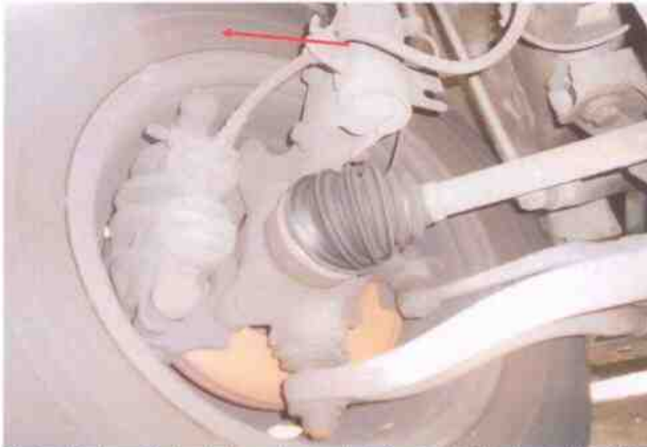
Photo 19 shows the brake hose (arrowed) at the front right wheel of the Motor Van. We did not observe any leakage of brake fluid at the time of our inspection of the Motor Van. Our visual inspection of the various mechanical components of the Motor Van's braking system, including its brake calliper, revealed all to be intact and without visible damage.
