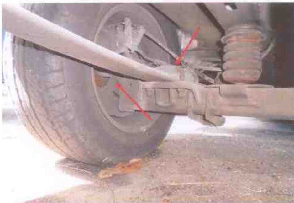
Photo 17 shows the various undercarriage components at the rear left wheel of the Motor Van, in particular the brake hose (arrowed). We did not observe any leakage of brake fluid at the time of our inspection of the Motor Van.
