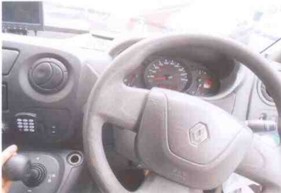
Photo 22 shows no warning lights illuminated on the instrument panel of the Motor Van after the engine was cranked. This would suggest that there was no abnormality to the various electronic operating systems of the Motor Car.
