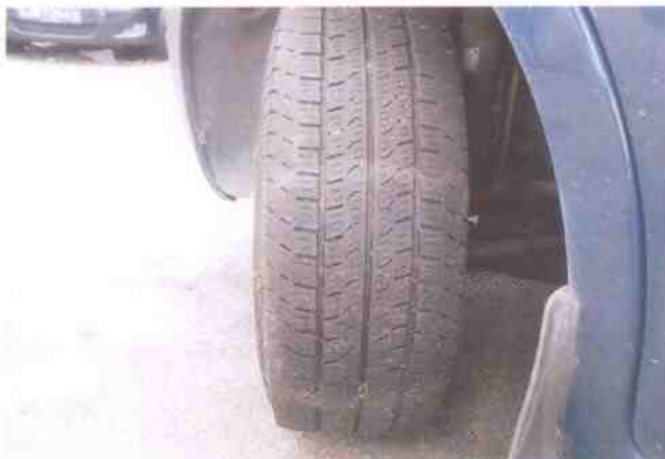
Photo 9 shows the condition of the front left tyre of the Motor Van, which was observed to be in serviceable condition with remaining tread depth of approximately 5mm. The tyre, which was wrapped around standard wheel rim, was also observed to be sufficiently inflated for vehicular operation.
