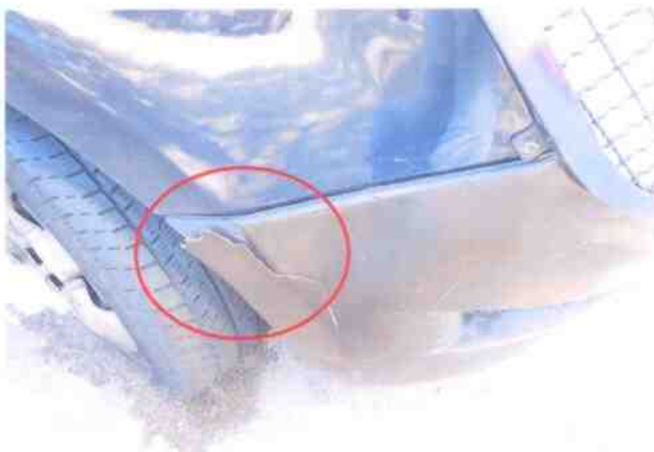
Photo 3 shows a close-up view of the damages on the front right lower bumper of the Motor Van at the time of our inspection. It was observed to have sustained with minor damage likely due to the accident.
