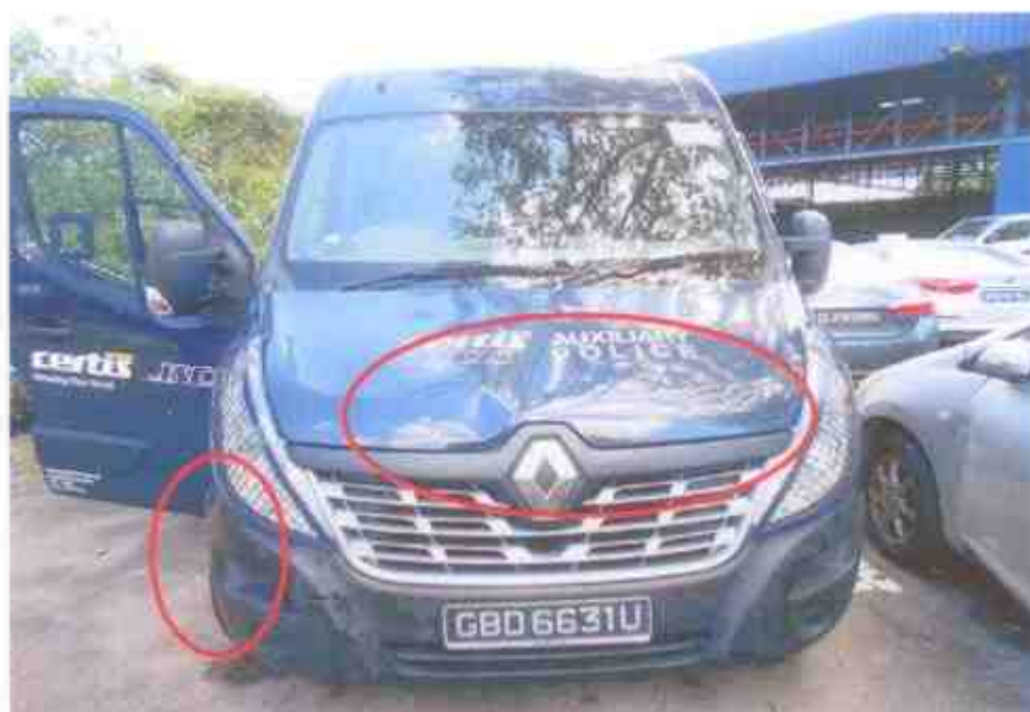
Photo 2 shows a general view of the front body of the Motor Van at the time of our inspection. The Motor Van was observed to sustained minor damage at the front bonnet & right lower bumper.
