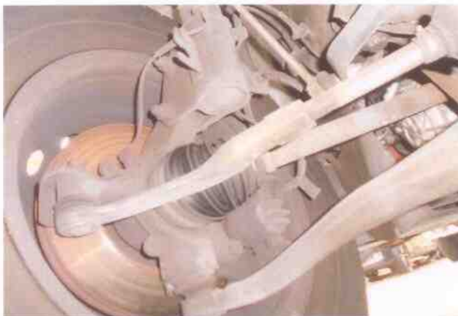
Photo 18 shows the brake hose at the front left wheel of the Motor Van. We did not observe any leakage of brake fluid. Our visual inspection of the various mechanical components of the Motor Van's braking system revealed all to be intact and without visible damage, indicating that the braking system was likely to be in serviceable condition at the material time of accident.
