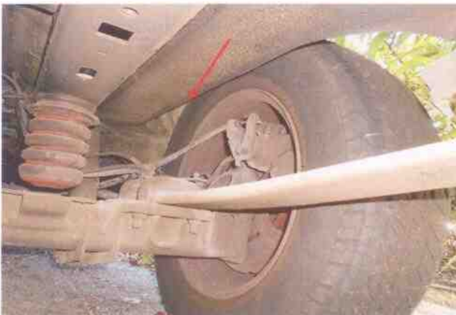
Photo 20 shows the various undercarriage components at the rear right wheel of the Motor Van. The various steering components were all found to be intact, suggesting that the steering system of the Motor Van was likely to be in serviceable condition at the material time of accident. There was also no sign of fluid stain(s) observed on the various undercarriage components at the 4 wheels of the Motor Van.
