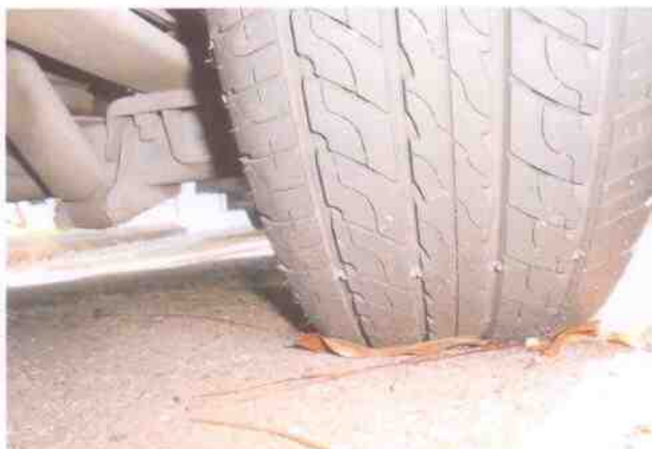
Photo 10 shows the condition of the rear left tyre of the Motor Van, which was observed to be in serviceable condition with remaining tread depth of approximately 7mm. The tyre, which was wrapped around standard wheel rim, was also observed to be sufficiently inflated for vehicular operation. There was also no significant damage found on the 4 wheel rims of the Motor Van.
