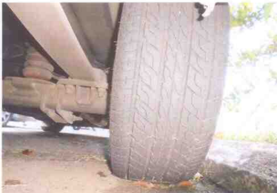
Photo 11 shows the condition of the rear right tyre of the Motor Van, which was observed to be in serviceable condition with remaining tread depth of approximately 8mm. There was also no tear, cut or burst mark(s) on the outer and the inner sidewalls as well as across the tread of the tyre, which was also sufficiently inflated for vehicular operation.
