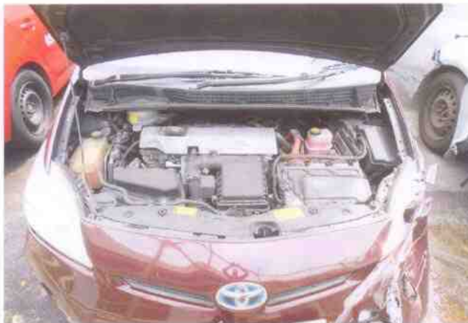
Photo 15 shows a general view of the Motor Car's engine compartment. The various parts and components inside the engine compartment were unaffected by the accident. There was also no sign(s) or indication(s) of fluid leakage and/or fluid stain within the engine compartment.
