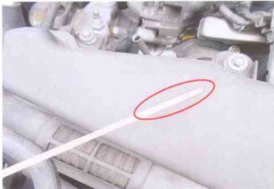
Photo 18 shows the engine oil dip stick of the Motor Taxi at the time of our inspection. The engine oil was observed to be of sufficient level and without any visible contamination.
