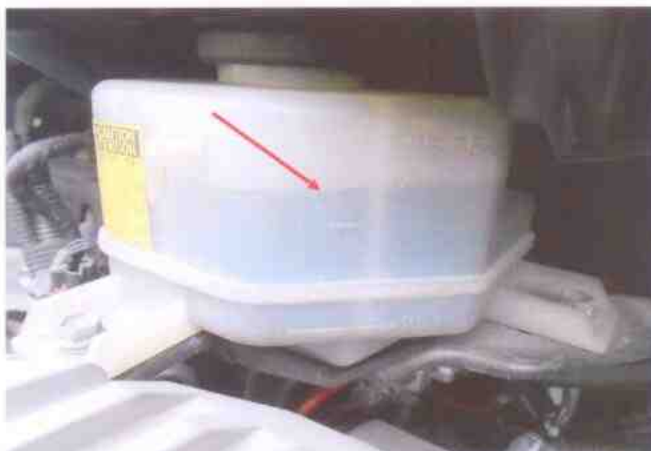
Photo 16 shows the brake fluid reservoir of the Motor Taxi at the time of our inspection. The brake fluid was observed to be of sufficient level (arrowed) and without any visible contamination.
