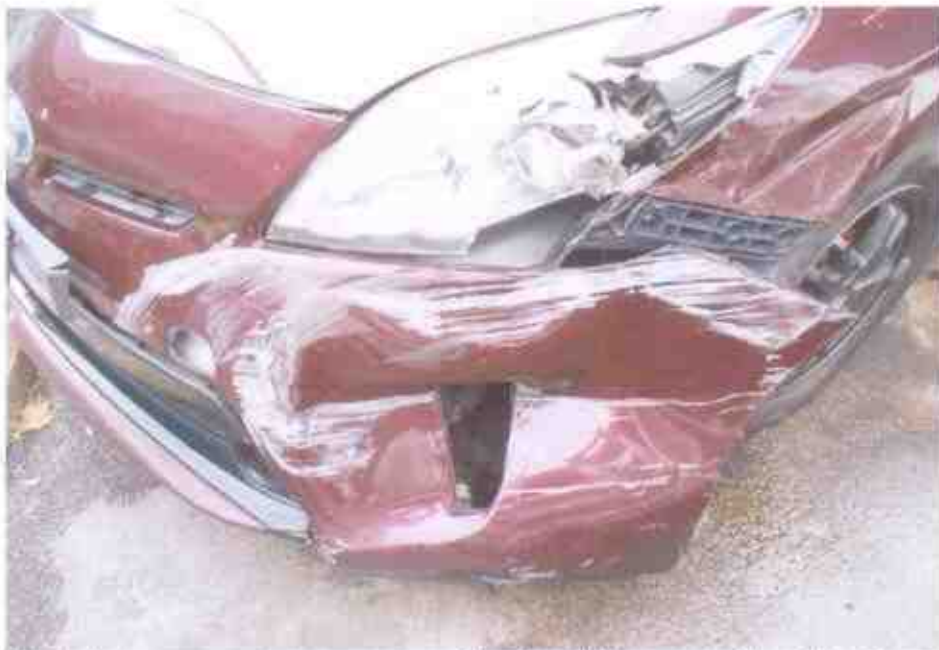
Photo 6 shows a semi close up view of the front left bumper of the Motor Taxi at the time of our inspection. The Motor Taxi had sustained damages at the front left bumper of the Motor Taxi.
