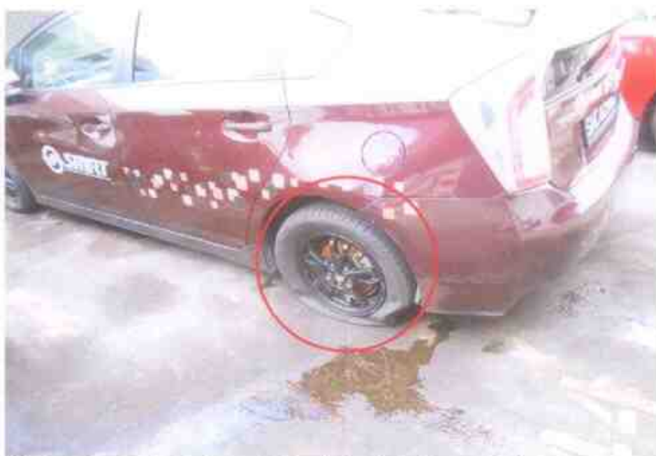
Photo 8 shows a deflated rear left tyre likely due to the accident's impact.
