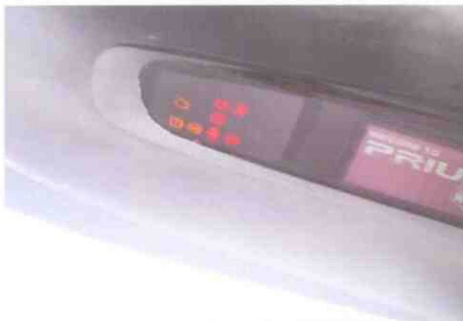
Photo 23 shows the warning lights for the various electronic operating systems of the Motor Taxi appearing on its instrument panel during the self-test when the engine is cranked, in particular the ABS light and SRS light.
