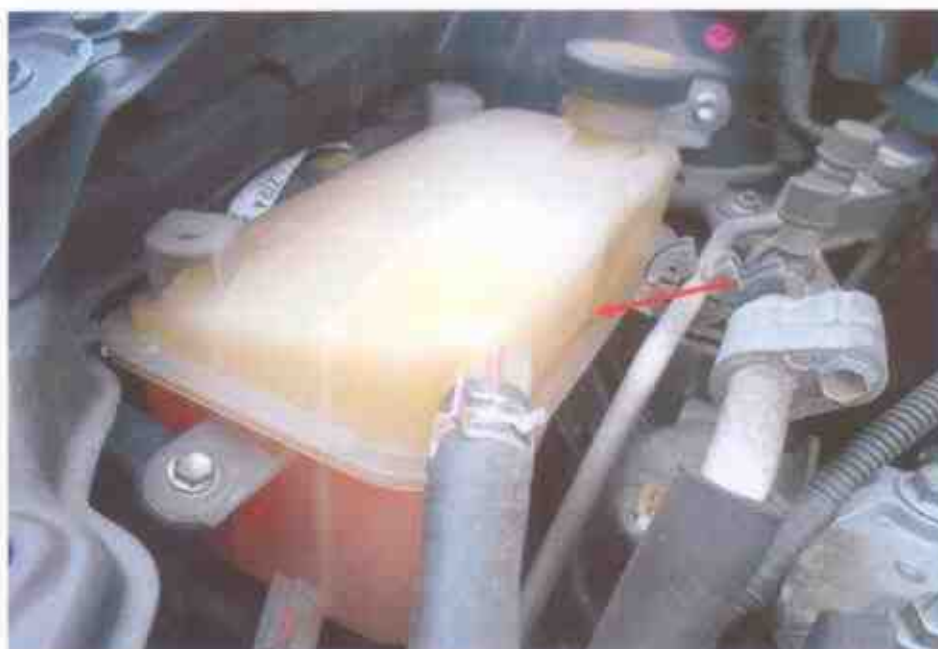
Photo 17 shows the engine coolant fluid reservoir of the Motor Taxi at the time of our inspection. The engine coolant fluid was observed to be of sufficient level and without any visible contamination.
