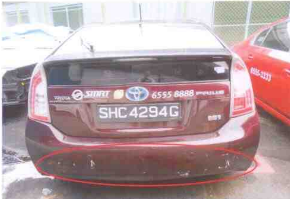
Photo 3 shows a general view of the rear body of the Motor Taxi at the time of our inspection. The Motor Taxi rear portion was observed to sustain multiple scratches likely due to the accident.
