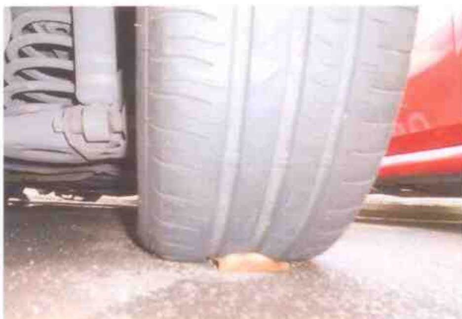
Photo 14 shows the condition of the rear right tyre of the Motor Taxi, which was observed to be in serviceable condition with remaining tread depth of approximately 7mm. There was also no tear, cut or burst mark(s) on the outer and the inner sidewalls.
