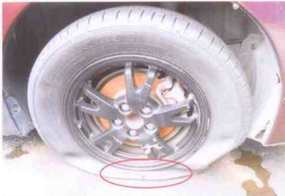
Photo 12 shows the condition of the rear left tyre of the Motor Taxi, which was observed to be deflated as a result of the accident. The remaining tread depth was approximately 5mm.
