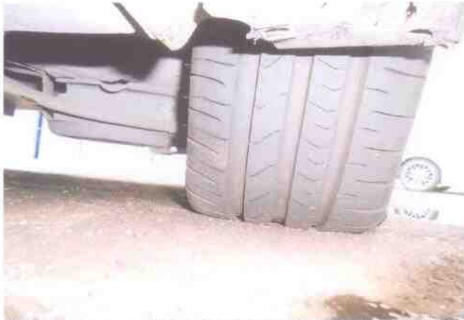
Photo 11 shows the condition of the rear left tyre of the Motor Taxi, which was observed to be deflated as a result of the accident. The remaining tread depth was approximately 5mm.
