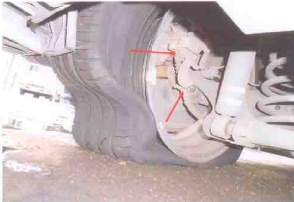
Photo 19 shows the brake hose (arrowed) at the rear left wheel of the Motor Taxi. We did not observe any leakage of brake fluid at the time of our inspection of the Motor Taxi. Our visual inspection of the various mechanical components of the Motor Taxi's braking system revealed all to be intact and without visible damage.
