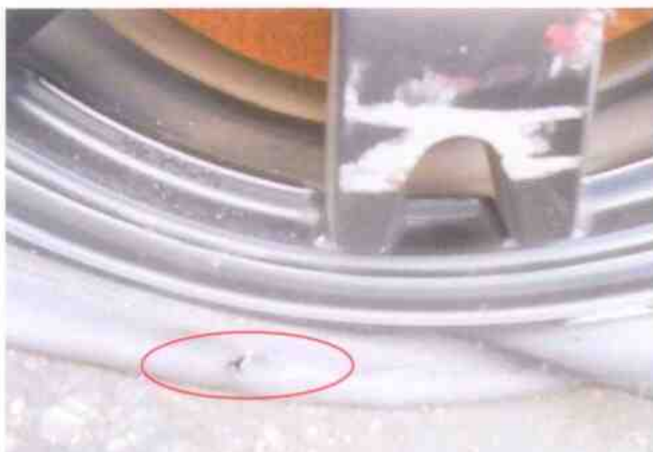
Photo 13 shows the close-up view of the rear left tyre of the Motor Taxi, which was observed to be deflated. Further observation found that the tyre was torn on the outer sidewalls as a result of the accident.
