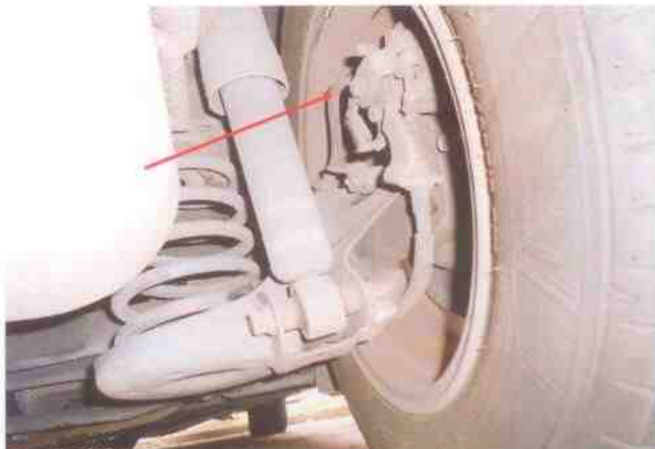
Photo 20 shows the brake hose (arrowed) at the rear right wheel of the Motor Taxi. We did not observe any leakage of brake fluid at the time of our inspection of the Motor Taxi. Our visual inspection of the various mechanical components of the Motor Taxi's braking system, including its brake calliper (circled), revealed all to be intact and without visible damage.
