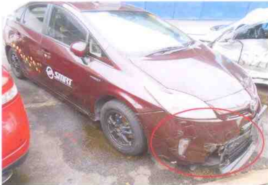
Photo 5 shows a general view of the front right body of the Motor Taxi at the time of our inspection. The Motor Taxi was observed to have sustained with damages on the front left portion as a result of the accident.
