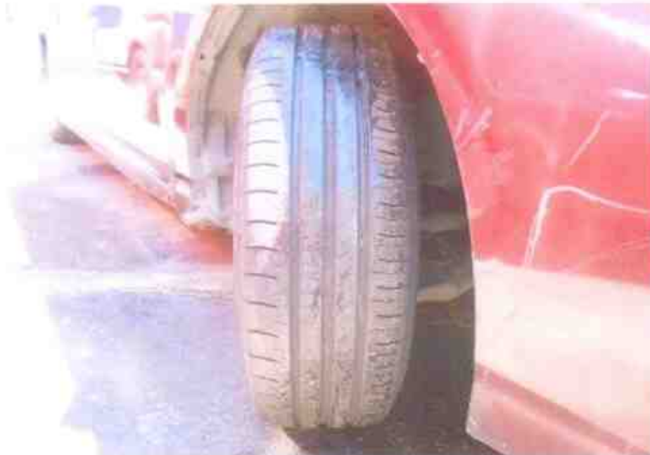
Photo 9 shows the condition of the front right tyre of the Motor Taxi, which was observed to be in serviceable condition. The remaining tread depth measured approximately around 7mm. There was no tear, cut or burst mark(s) on the outer and the inner sidewalls.
