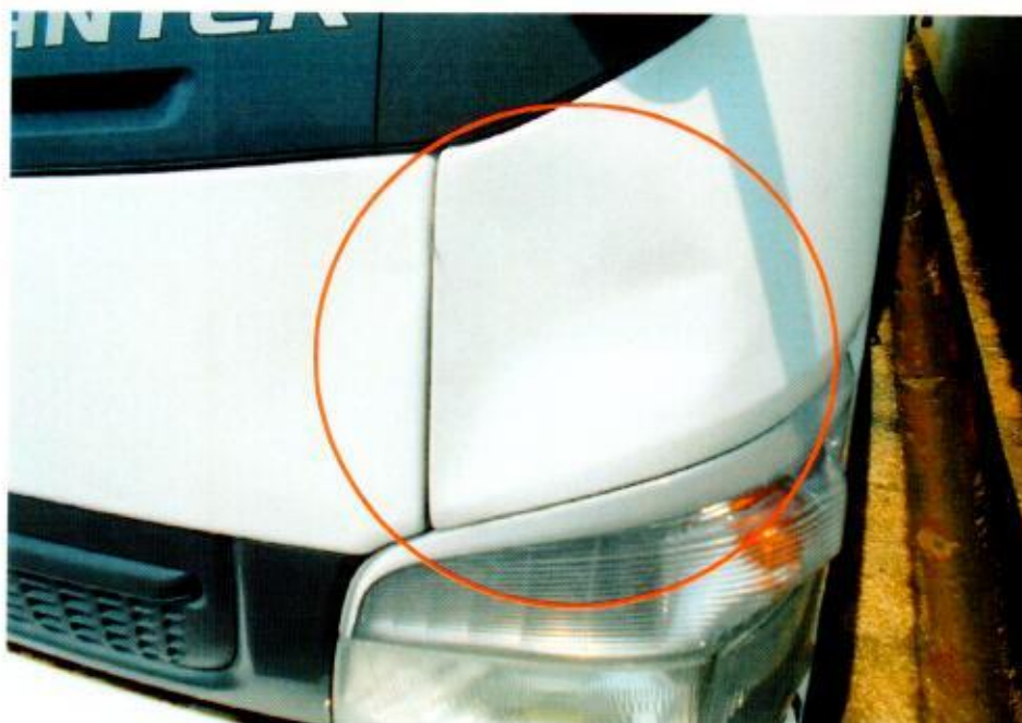
Photo 4 shows a dented portion on the left front panel at time of our inspection.
