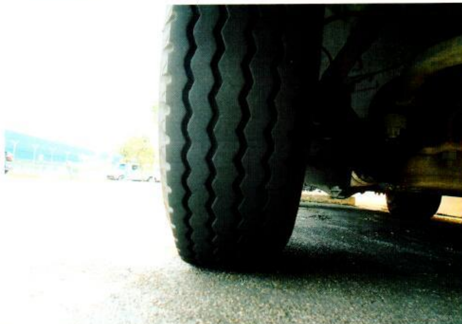
Photo 8 shows the condition of the front right tyre of the Motor Lorry, which was observed to be in serviceable condition with remaining tread depth of approximately 7mm. The tyre, which was wrapped around standard alloy wheel rim, was also observed to be sufficiently inflated for vehicular operation.
