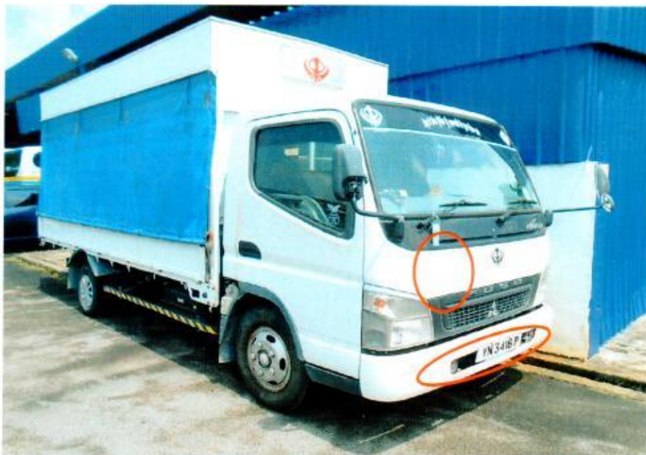
Photo 2 shows a general view of the front right of the Motor Lorry at the time of our inspection. The Motor Lorry was observed to have sustained minor damage at its front left hand side panel; its right hand side panel; its number plate were amongst the body parts that were damaged as a result of the accident.
