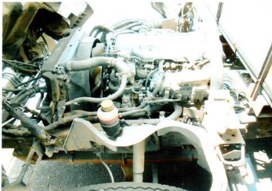
Photo 11 shows a general view of the Motor Lorry's engine compartment, which was accessed by lifting the front cabin of the Motor Lorry. The various parts and components inside the engine compartment were unaffected by the accident. There was also no sign(s) or indication(s) of fresh fluid leakage and/or fluid stain within the engine.
