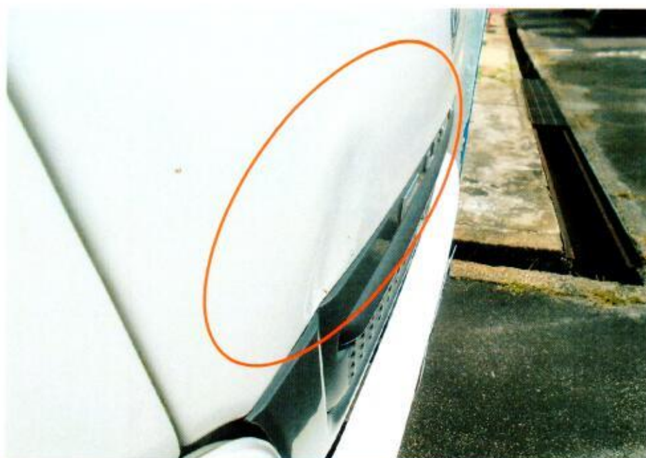
Photo 3 shows a dented portion on the right front panel at time of our inspection.
