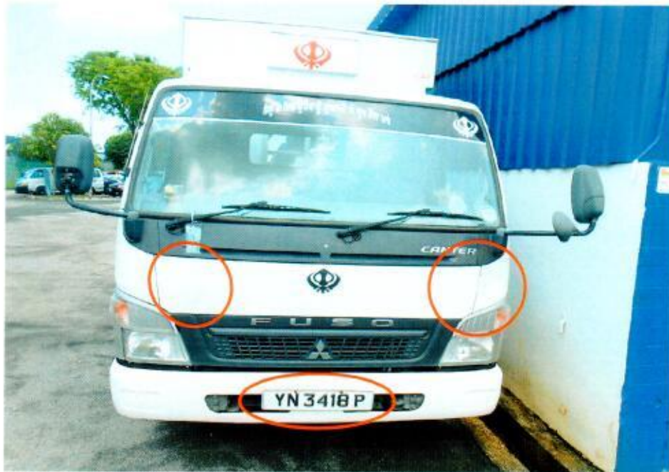
Photo 1 shows a general view of the front portion of the Motor Lorry at the time of our inspection. The Motor Lorry was observed to have sustained minor damage at its front left hand side panel; its right hand side panel; its number plate were amongst the body parts that were damaged as a result of the accident.
