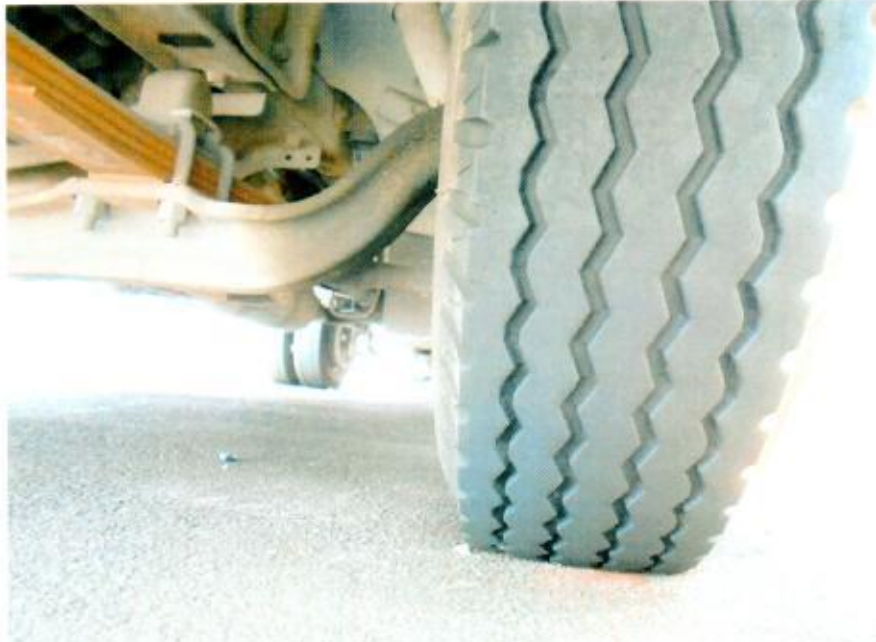
Photo 7 shows the condition of the front left tyre of the Motor Lorry, which was observed to be in serviceable condition with remaining tread depth of approximately 7mm. The tyre, which was wrapped around standard alloy wheel rim, was also observed to be sufficiently inflated for vehicular operation.
