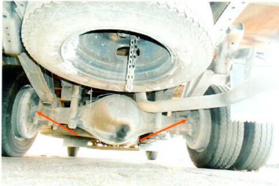
Photo 18 shows the various undercarriage components at the rear wheels of the Motor Lorry. There was no sign(s) of brake fluid leakage along the brake hoses and brake pipes.
