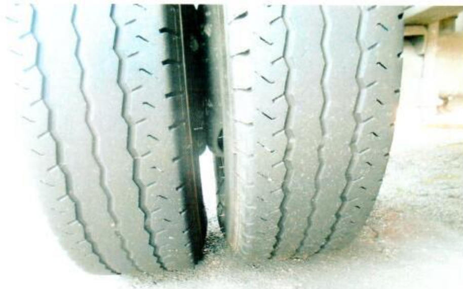
Photo 9 shows the condition of the rear left tyres of the Motor Lorry, which was observed to be in serviceable condition with remaining tread depth of approximately 6mm. The tyres, which were wrapped around standard alloy wheel rim, were also observed to be sufficiently inflated for vehicular operation.
