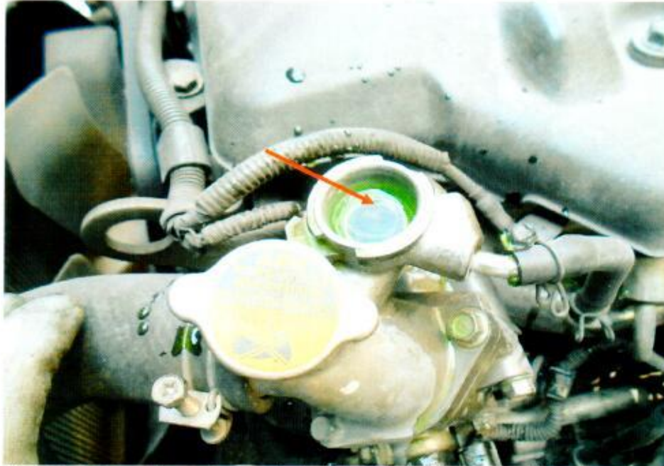
Photo 14 shows the engine coolant fluid of the Motor Lorry at the time of our inspection. It was observed to be of sufficient level and without any visible contamination (arrowed).
