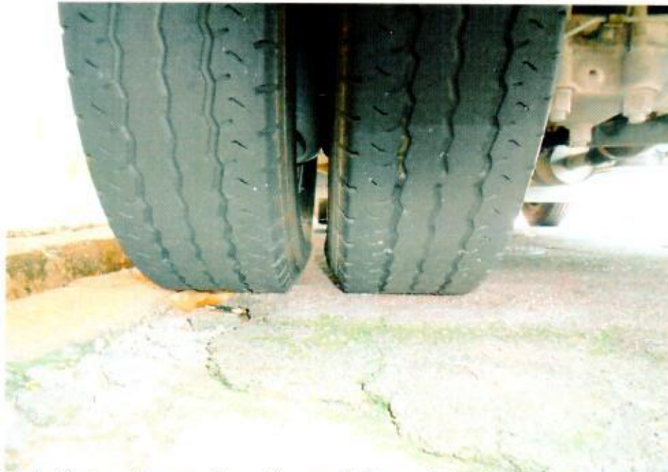
Photo 9 shows the condition of the rear left tyres of the Motor Lorry, which was observed to be in serviceable condition with remaining tread depth of approximately 6mm. The tyres, which were wrapped around standard alloy wheel rim, were also observed to be sufficiently inflated for vehicular operation.
