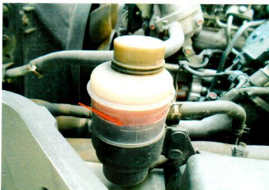
Photo 13 shows the power steering fluid reservoir of the Motor Lorry at the time of our inspection. power steering fluid was observed to be of sufficient level and without any visible contamination (arrowed).
