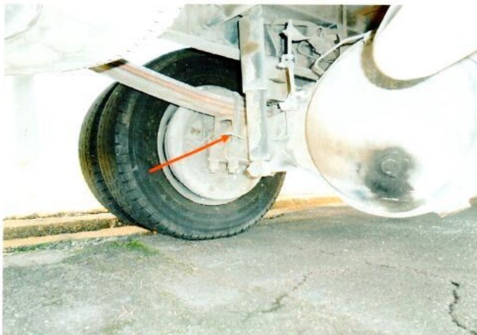
Photo 19 shows the brake hoses at the rear wheels of the Motor Lorry revealed that there was no sign(s) of brake fluid leakage along the brake hoses and brake pipes.
