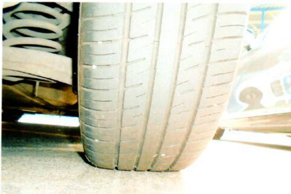
Photo 10 shows the condition of the rear right tyre of the Motor Taxi, which was observed to be in serviceable condition with remaining tread depth of approximately 6mm. There was also no tear, cut or burst mark(s) on the outer and the inner sidewalls as well as across the tread of the 4 tyres.
