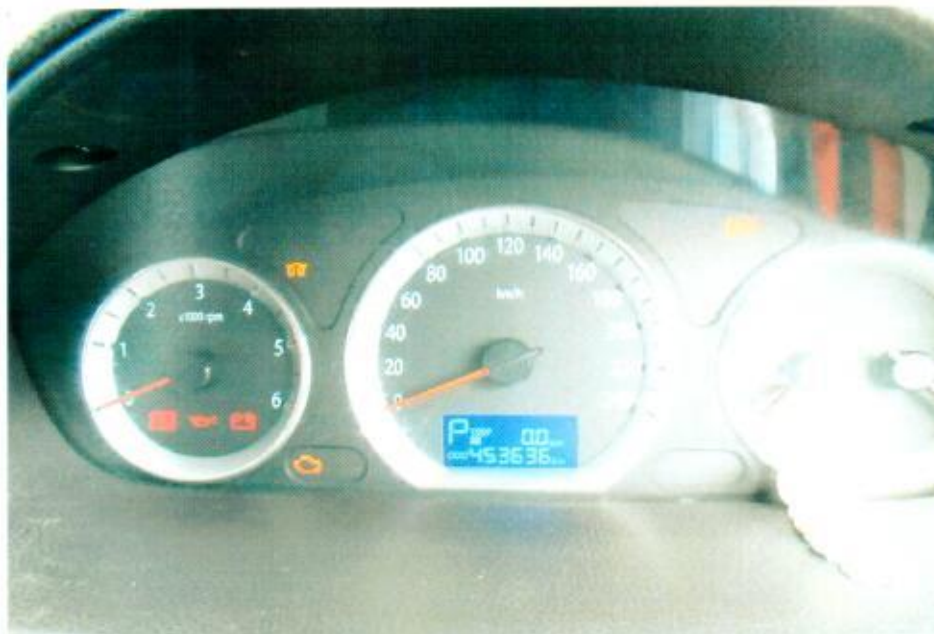
Photo 20 shows the warning lights for the various electronic operating systems of the Motor Taxi appearing on its instrument panel during the self-test when the engine is cranked, in particular the ABS light and SRS light.
