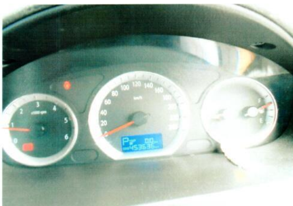
Photo 21 shows no warning lights illuminated on the instrument panel of the Motor Taxi after the engine was cranked. This would suggest that there was no abnormality to the various electronic operating systems of the Motor Taxi, like the ABS and SRS.
