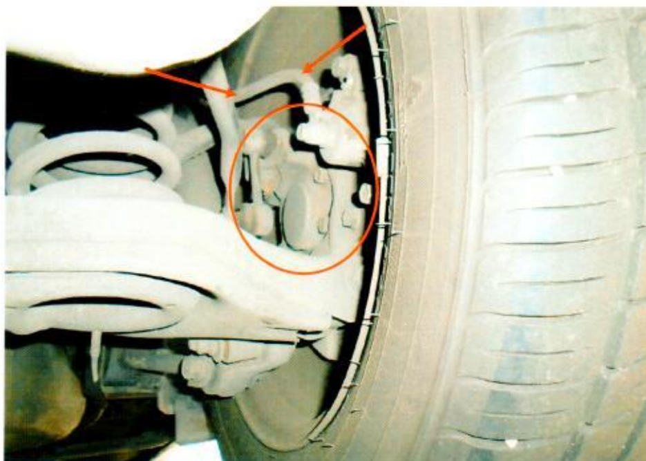
Photo 17 shows the brake hose (arrowed) at the rear right wheel of the Motor Taxi. We did not observe any leakage of brake fluid at the time of our inspection of the Motor Taxi. Our visual inspection of the various mechanical components of the Motor Taxi's braking system, including its brake calliper (circled), revealed all to be intact and without visible damage, indicating that the braking system was likely to be in serviceable condition at the material time of accident.
