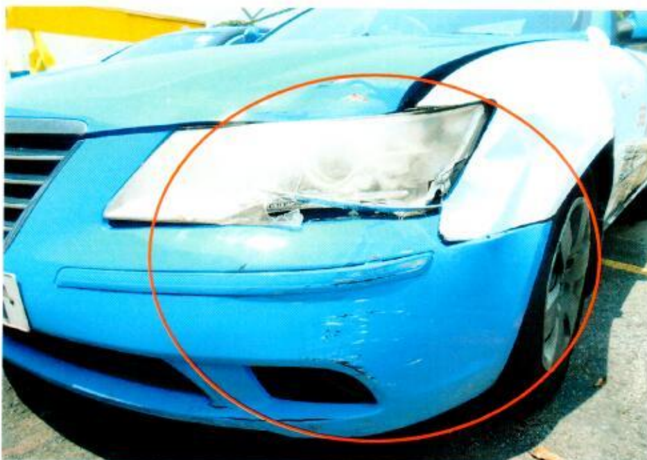
Photo 6 shows a close up view of the front number plate/base of the Motor Taxi at the time of our inspection. The Motor Taxi had sustained relatively minor impact at the front left of the Motor Car.
