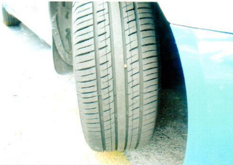
Photo 7 shows the condition of the front right tyre of the Motor Taxi, which was observed to be in serviceable condition with remaining tread depth of approximately 6mm. There was no tear, cut or burst mark(s) on the outer and the inner sidewalls.
