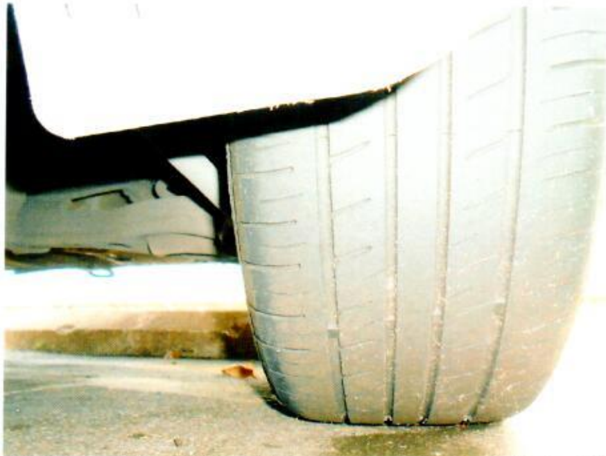
Photo 9 shows the condition of the rear left tyre of the Motor Taxi, which was observed to be in serviceable condition with remaining tread depth of approximately 4mm. The tyre, which was wrapped around alloy wheel rim, was also observed to be sufficiently inflated for vehicular operation.
