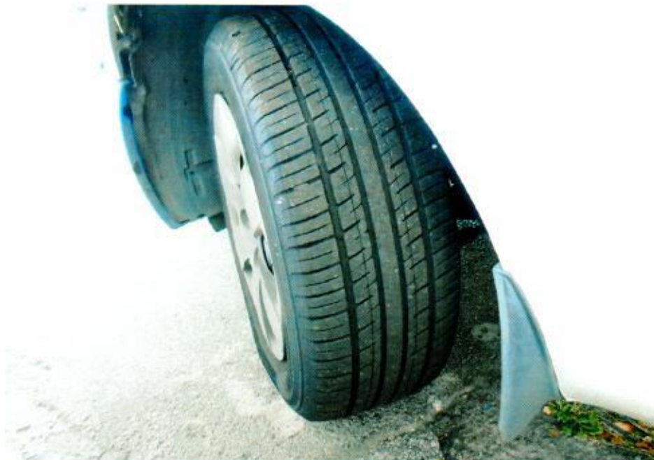
Photo 8 shows the condition of the front left tyre of the Motor Taxi, which was observed to be in serviceable condition with remaining tread depth of approximately 6mm. The tyre, which was wrapped around alloy wheel rim, was also observed to be sufficiently inflated for vehicular operation.
