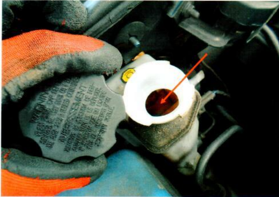
Photo 12 shows the brake fluid reservoir of the Motor Taxi at the time of our inspection. The brake fluid was observed to be of sufficient level (arrowed) and without any visible contamination.
