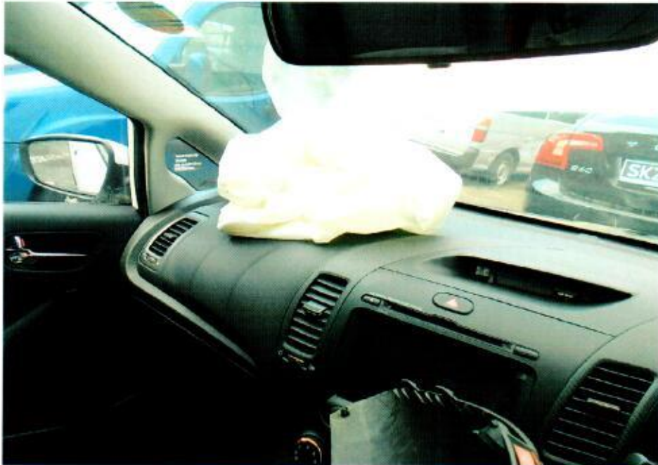
Photo 34 shows the front passenger's seat airbag was activated indicating that the airbag system was in serviceable condition prior to the accident.
