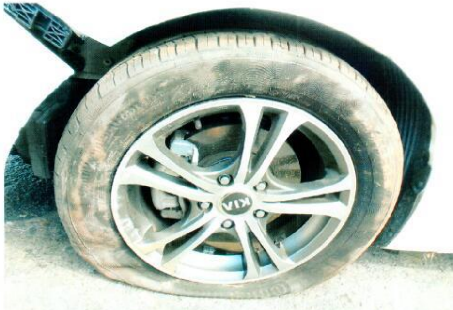
Photo 10 shows the condition of the front left tyre of the Motor Car, which was observed to be deflated due to the accident. Its alloy wheel rim also found to have sustained with scratches.
