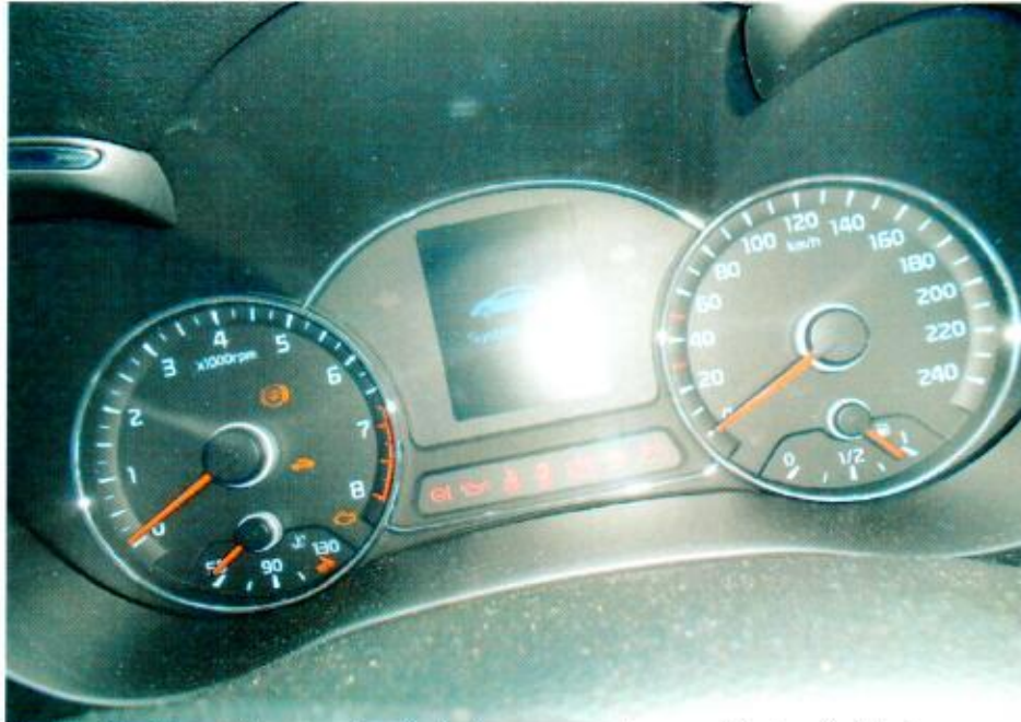
Photo 32 shows the warning indicators were observed to be lighted up upon cranking of the engine. It was observed to be operating abnormally likely due to the accident's impact collision. This indicates that the Motor Car electronic systems sustained system malfunction as a result of the accident.
