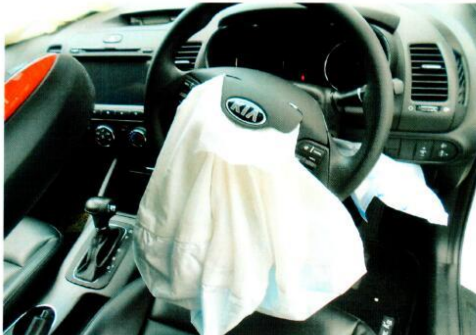
Photo 33 shows the driver seat airbag was activated indicating that the airbag system was in serviceable condition prior to the accident.
