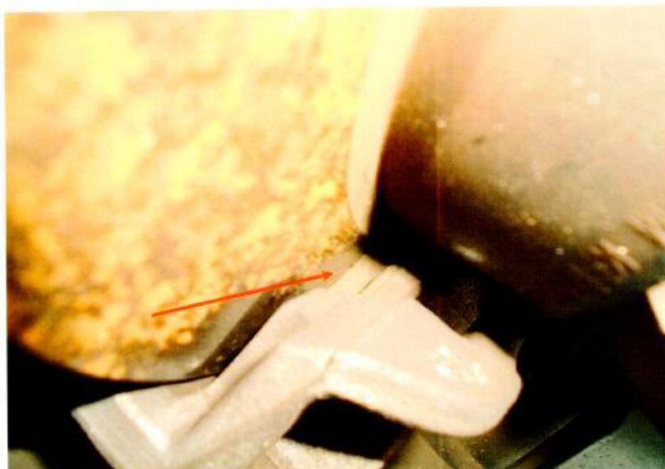
Photo 30 shows the rear right brake pad of the Motor Car. It was observed to be in serviceable condition looking at the thickness of the brake pad at time of our inspection.
