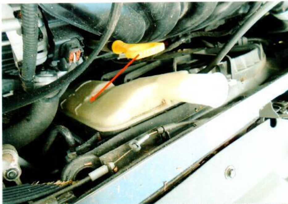
Photo 18 shows the fluid component such as coolant fluid was visible and found to be of sufficient level for operating purposes. Visually, there was also no contamination found to this fluid.
