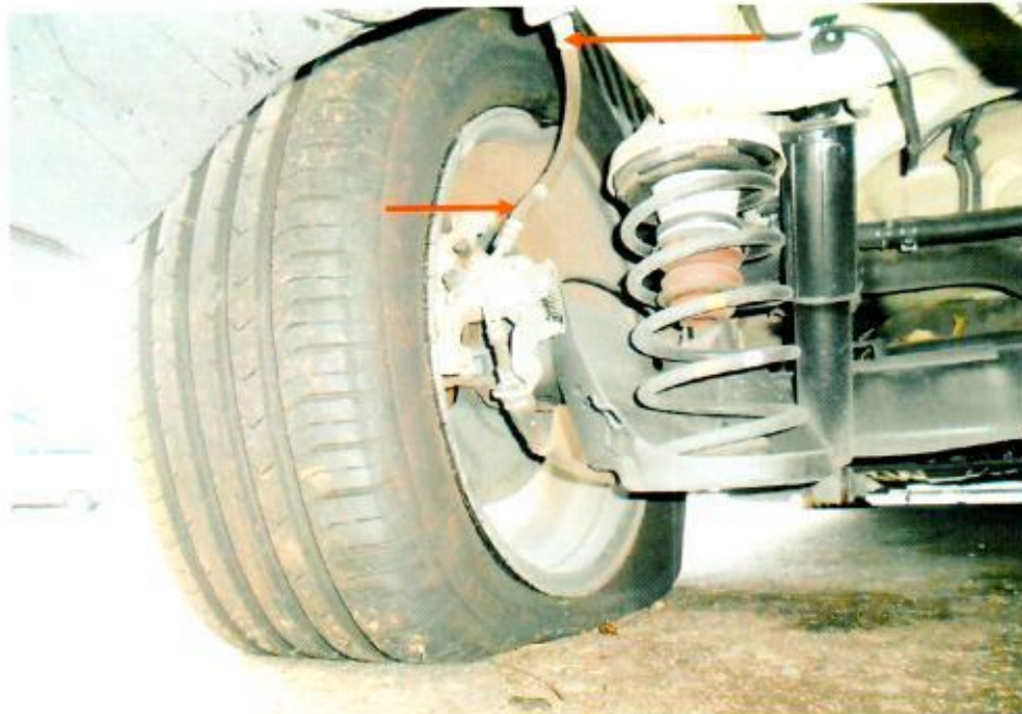
Photo 23 shows the brake hose (arrowed) at the rear left wheel of the Motor Car. Our visual inspection of the various mechanical components of the Motor Car's braking system revealed all to be intact and without visible damage, indicating that the braking system was likely to be in serviceable condition at the material time of accident.
