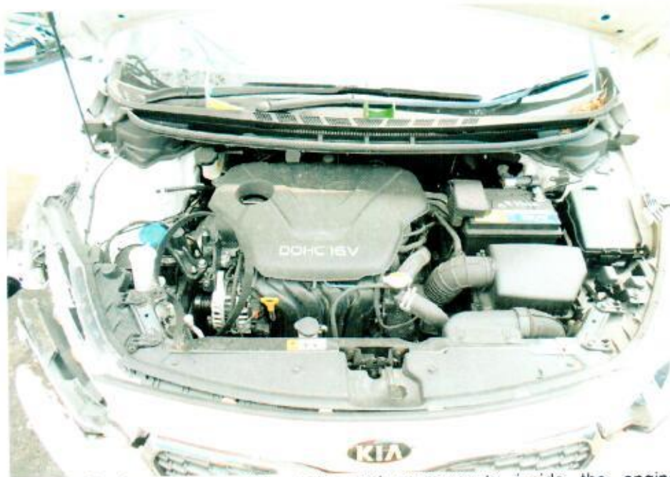
Photo 16 shows the visible parts and components inside the engine compartment to be intact and unaffected by the accident.
