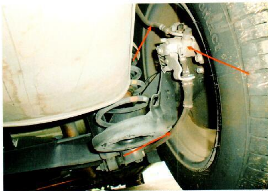
Photo 26 shows the various undercarriage components at the rear right wheel of the Motor Car. We did not observe any leakage of brake fluid at the time of our inspection of the Motor Car. Our visual inspection of the various mechanical components of the Motor Car's braking system revealed all to be intact and without visible damage, indicating that the braking system was likely to be in serviceable condition at the material time of accident.
