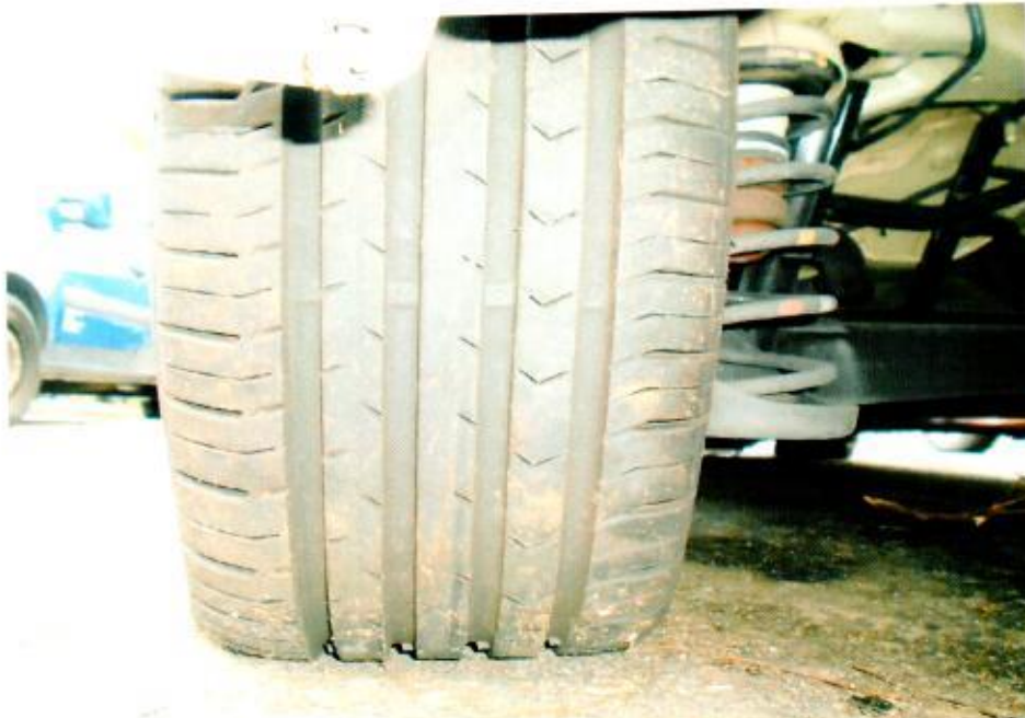
Photo 13 shows the condition of the rear left tyre of the Motor Car, with remaining tread depth of approximately 7mm. However, it was observed to be deflated due to the accident's impact.
