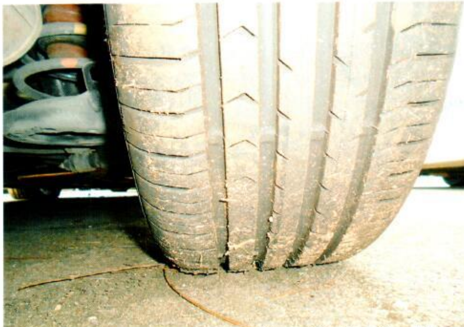
Photo 15 shows the condition of the rear right tyre of the Motor Car, which was observed to be in serviceable condition with remaining tread depth of approximately 8mm. The tyre was also observed to be sufficiently inflated for vehicular operation.
