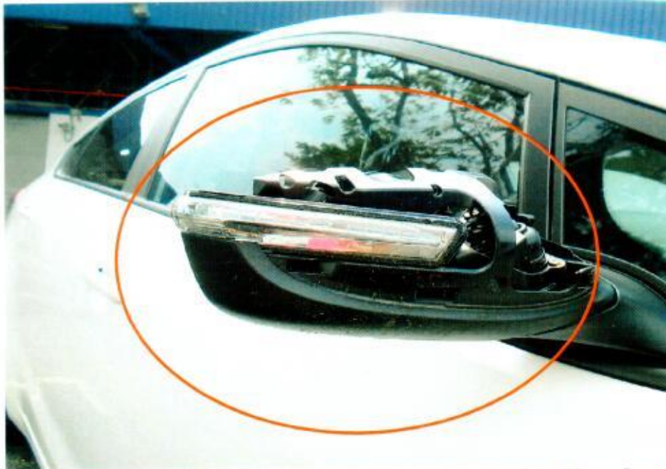
Photo 7 shows a close up view of the front right side mirror of the Motor Car at the time of our inspection. It had sustained damages likely due to the accident.
