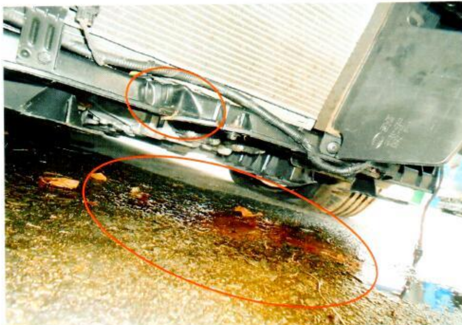
Photo 21 shows our subsequent checks on the underside of the Motor Car also reveals there's fluid stain on the ground right underneath the engine pan. This indicates that there's fluid leakage exist likely due to the accident's impact.
