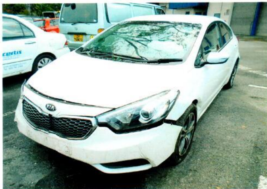
Photo 4 shows a general view of the front left body of the Motor Car at the time of our inspection. The Motor Car was observed to have sustained damages at the left frontal portion.
