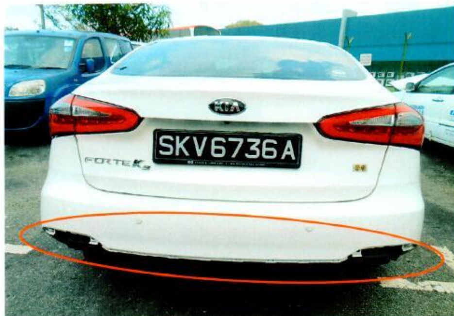
Photo 8 shows a general view of the rear body of the Motor Car at the time of our inspection. It had sustained damages likely due to the accident.
