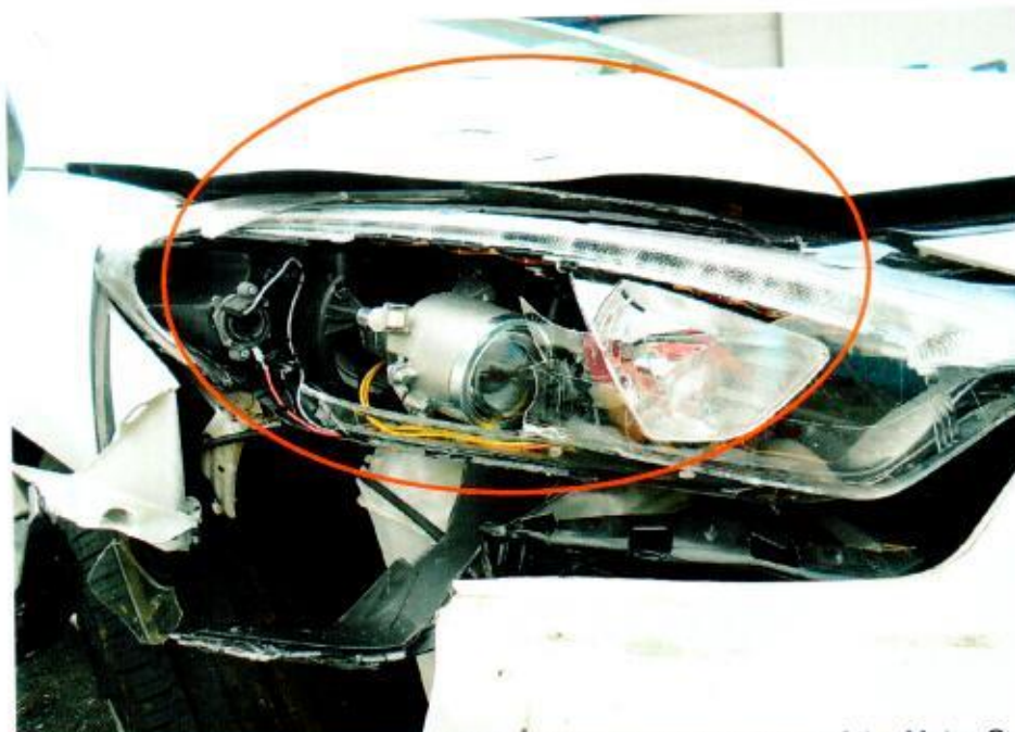
Photo 5 shows a close up view of the front right side headlamp of the Motor Car at the time of our inspection. It had sustained damages likely due to the accident.
