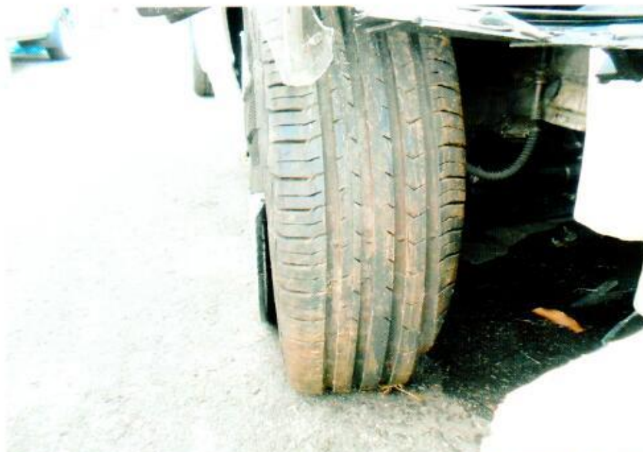
Photo 11 shows the condition of the front right tyre of the Motor Car, with remaining tread depth of approximately 7mm. However, it was observed to be deflated due to the accident's impact.
