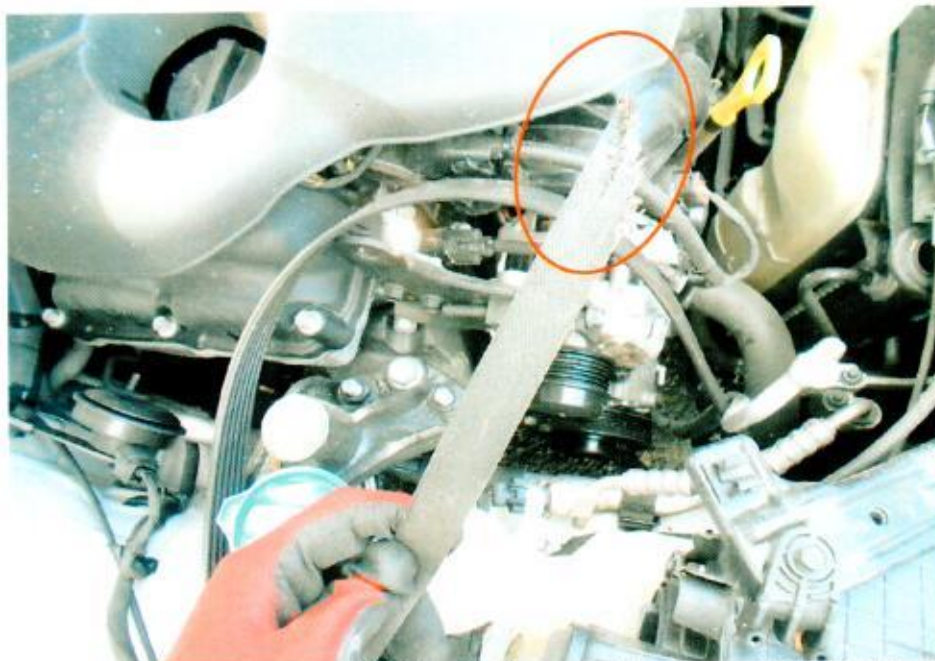
Photo 22 showed damaged belting for the operational components such as alternator, air-conditioning compressor amongst others for the normal operation.
