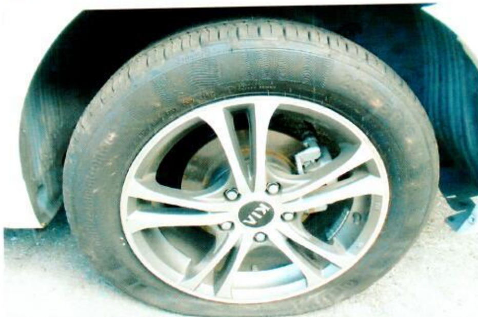
Photo 14 shows the condition of the rear left tyre of the Motor Car, which was observed to be deflated due to the accident. Its alloy wheel rim also found to have sustained with scratches.
