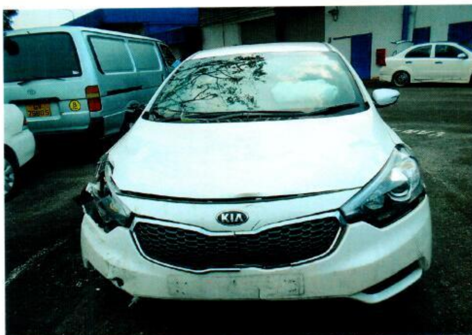
Photo 2 shows a general view of the front body of the Motor Car at the time of our inspection. The Motor Car was observed to have sustained damages at the frontal, front left & front right portion.
