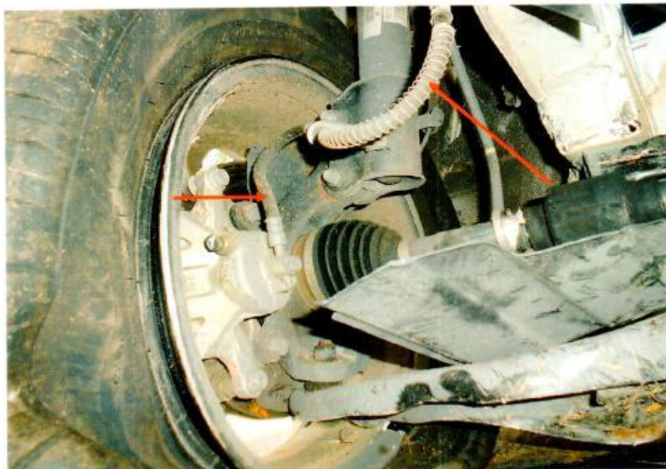
Photo 24 shows the brake hose (arrowed) at the front right wheel of the Motor Car. Our visual inspection of the various mechanical components of the Motor Car's braking system, including its brake calliper, revealed all to be intact and without visible damage, indicating that the braking system was likely to be in serviceable condition at the material time of accident.
