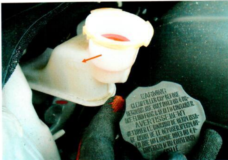
Photo 17 shows the fluid component such as brake fluid was visible and found to be of sufficient level for operating purposes. Visually, there was also no contamination found to this fluid.
