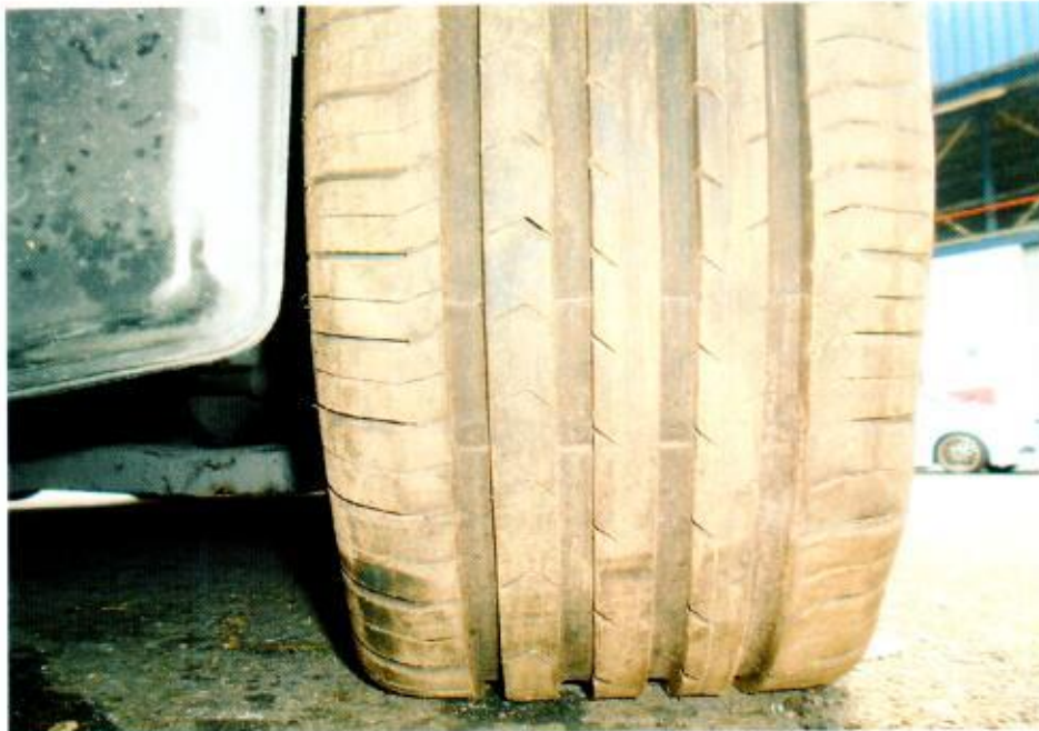
Photo 9 shows the condition of the front left tyre of the Motor Car, with remaining tread depth of approximately 7mm. However, it was observed to be deflated due to the accident's impact.
