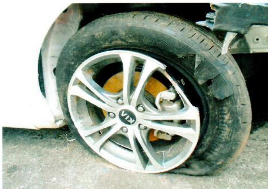
Photo 12 shows the condition of the front right tyre of the Motor Car, with remaining tread depth of approximately 7mm. Further observation found that the sidewall was torn & deflated. The alloy wheel rim found to be damaged as a result of the accident.
