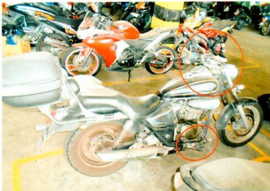
Photo 3 shows a general view of the right body of the Motorcycle at the time of our inspection. The Motorcycle was observed to have sustained minor damages at the frontal, rear portion & along its right side. (Circled)
