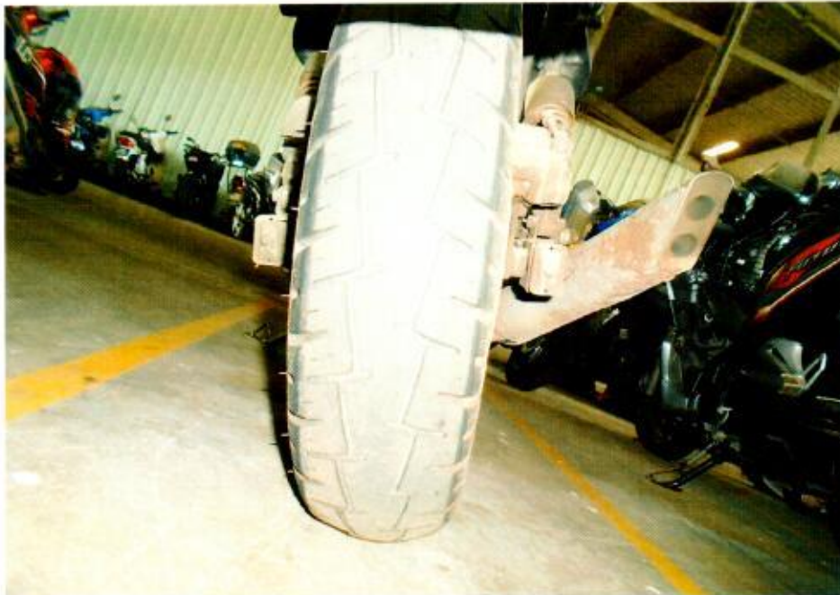
Photo 7 shows the rear tyre of the Motorcycle. The rear tyre was observed to be in serviceable condition with remaining tread depth of approximately 4mm. The tyre was also observed to be sufficiently inflated for vehicular operation.
