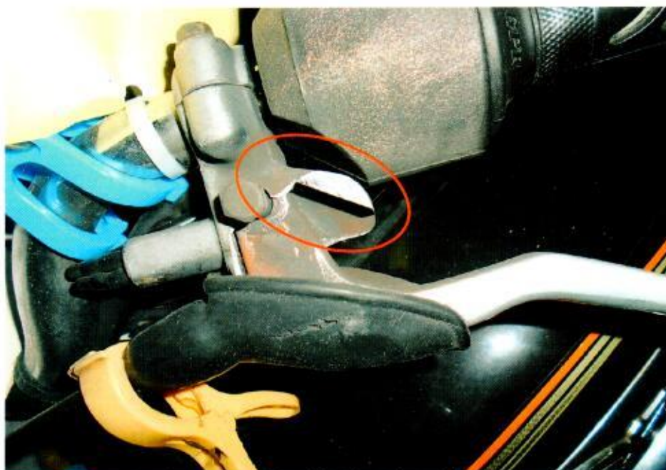
Photo 4 shows a closer view of the left wing mirror of the Motorcycle at the time of our inspection that was observed to be damaged due to the accident collision. (Circled)
