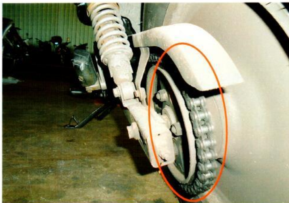
Photo 11 shows the gear chain of the motorcycle was found to be intact without any misalignment. It was also adequately lubricated for operating purposes.
