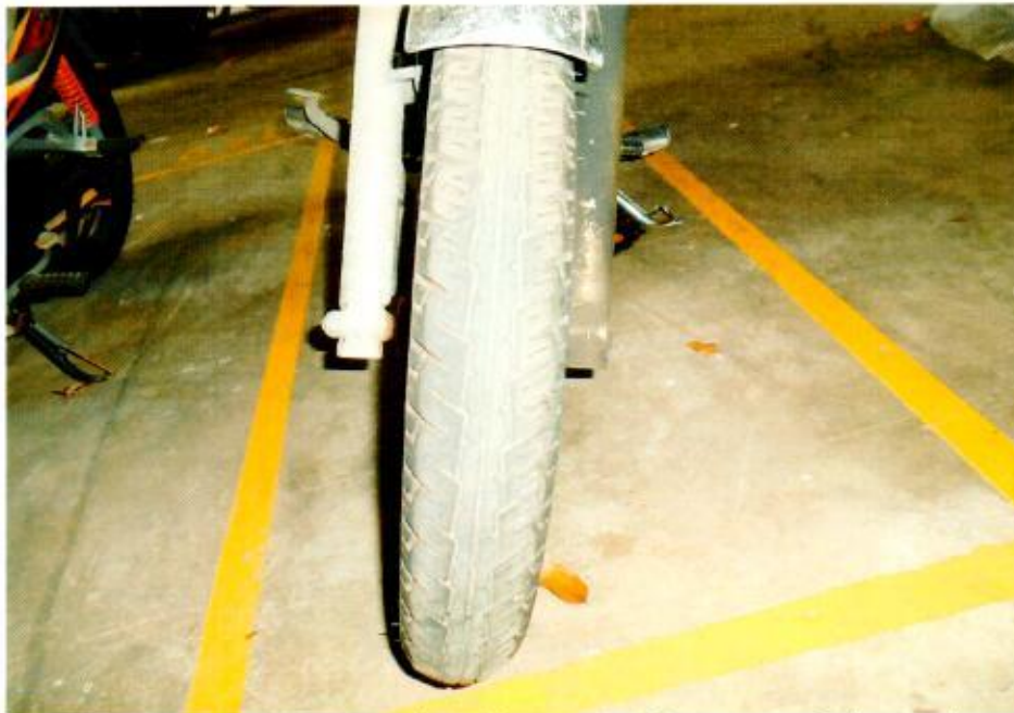
Photo 8 shows the front tyre of the Motorcycle. The pattern of the tread was clearly visible. There was no tear, burst mark(s) and/or punctured hole(s) on the sidewalls as well as across the tread of the front tyre.
