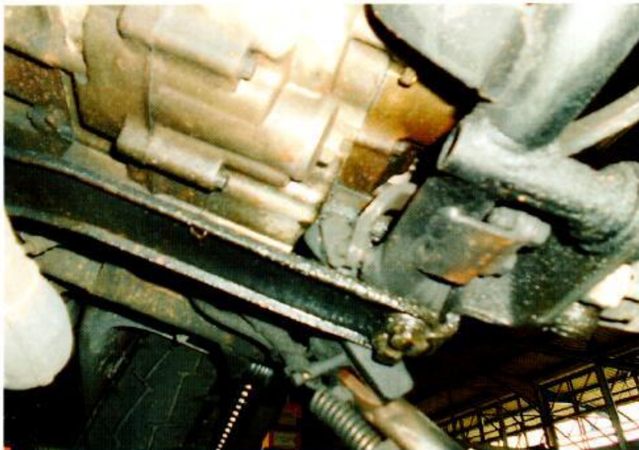
Photo 9 shows sign(s) or indication(s) of fluid leak observed around the underside engine area of the Motorcycle.
