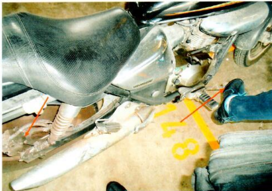
Photo 20 shows testing of the braking of the rear brake in progress. There was some resistance felt (spongy like feel) upon stepping on the brake pedal.
