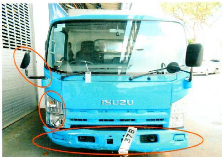
Photo 1 shows a general view of the front portion of the Motor Lorry at the time of our inspection. The Motor Lorry was observed to have sustained minor damage at its front lower bumper; its right headlamp; its right hand side mirror and number plate were amongst the body parts that were damaged as a result of the accident.
