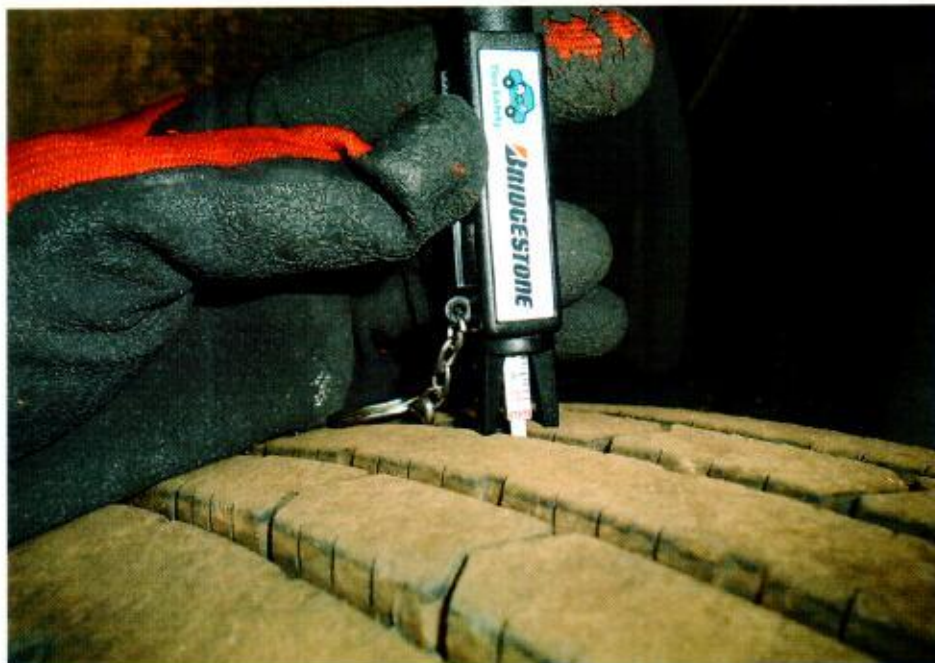
Photo 7 shows the remaining tread depth of the front left tyre of the Motor Lorry, which was observed to be in serviceable condition with remaining tread depth of approximately 8mm.
