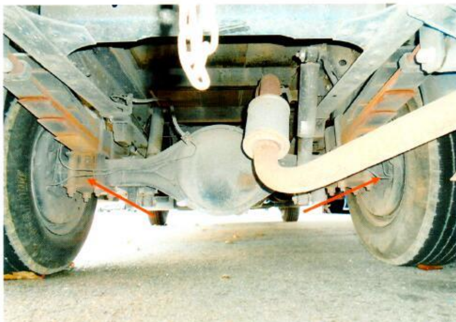
Photo 18 shows the various undercarriage components at the rear wheels of the Motor Lorry. There was no sign(s) of brake fluid leakage along the brake hoses and brake pipes.
