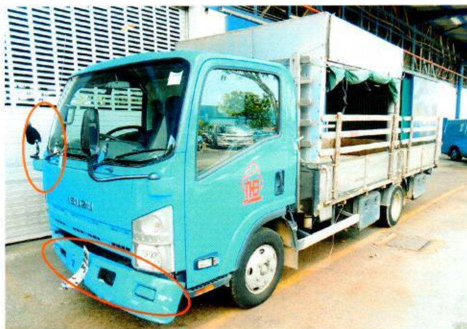
Photo 2 shows a general view of the front left of the Motor Lorry at the time of our inspection. The Motor Lorry was observed to have sustained minor damage at its front lower bumper; its right headlamp; its right hand side mirror and number plate were amongst the body parts that were damaged as a result of the accident.
