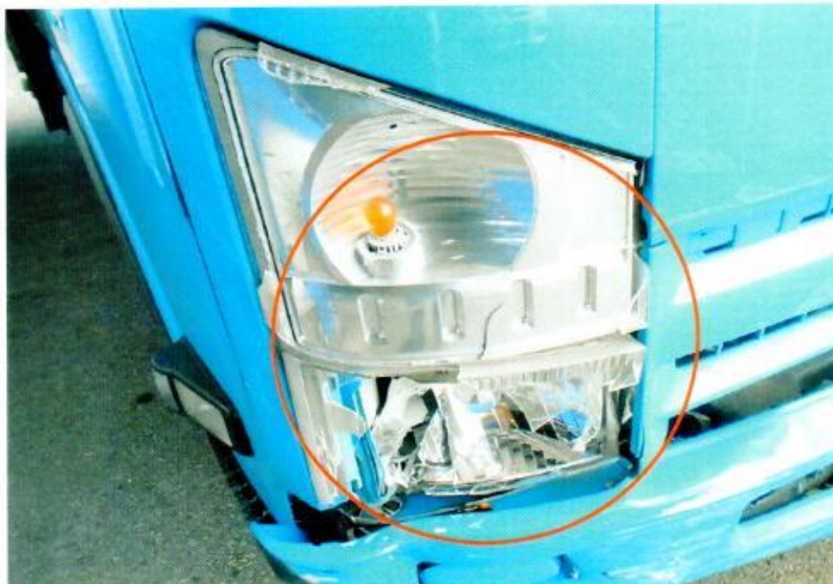
Photo 4 shows the right headlamp of the Motor Lorry. It was observed to have sustained damages as a result of the accidents.
