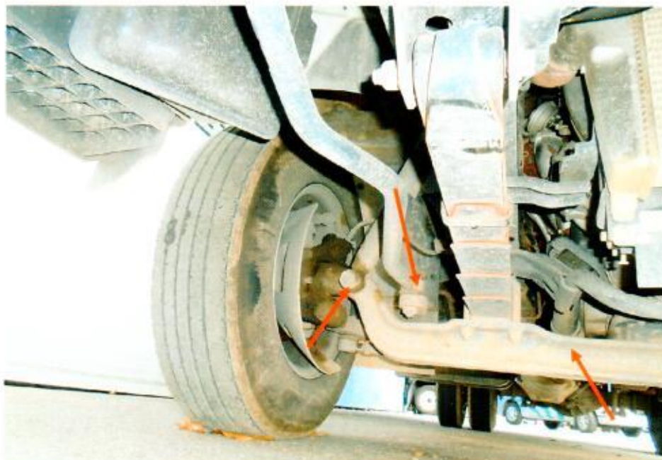
Photo 16 shows the various undercarriage components at the front left wheel of the Motor Lorry, in particular the steering tie rod end (arrowed). The various undercarriage components of the Motor Lorry were all found to be intact without any visible damage. There was also no sign of fluid stain(s) observed on the various undercarriage components.
