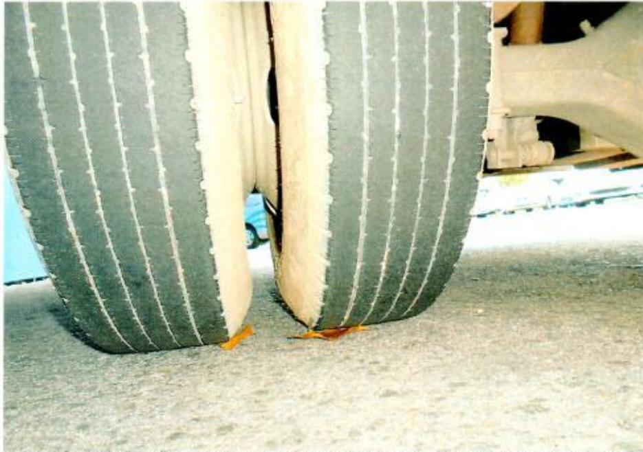
Photo 11 shows the condition of the rear right tyres of the Motor Lorry, which were observed to be in serviceable condition with remaining, tread depth of approximately 7mm.
