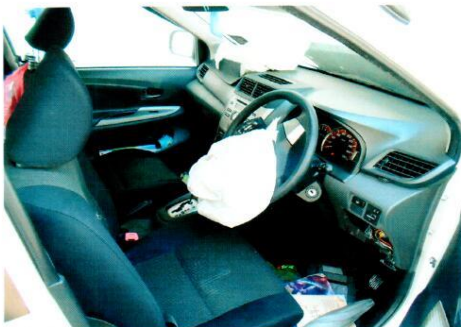
Photo 8 shows the interior portion of the Motor Car. The impact force was significant causing the driver's airbag & front passenger's airbag to be dislodged.
