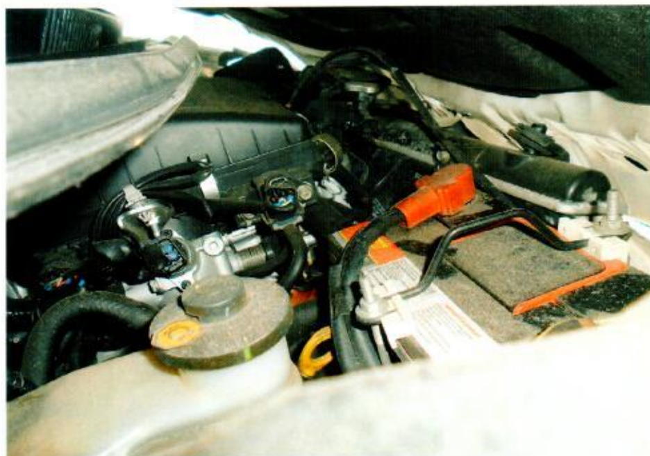
Photo 7 shows a closer view of the engine compartment of the Motor Car from the right hand side of the bonnet opening. The impact force was significant, causing the various parts and components inside the engine compartment to be pushed inwards, towards the rear of the Motor Car.
