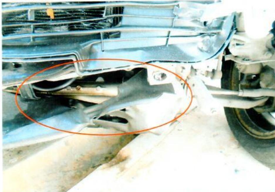
Photo 15 shows the close up view of the steering rack of the Motor Car. Leakage of the various operating fluids like the power steering fluid was seen.
