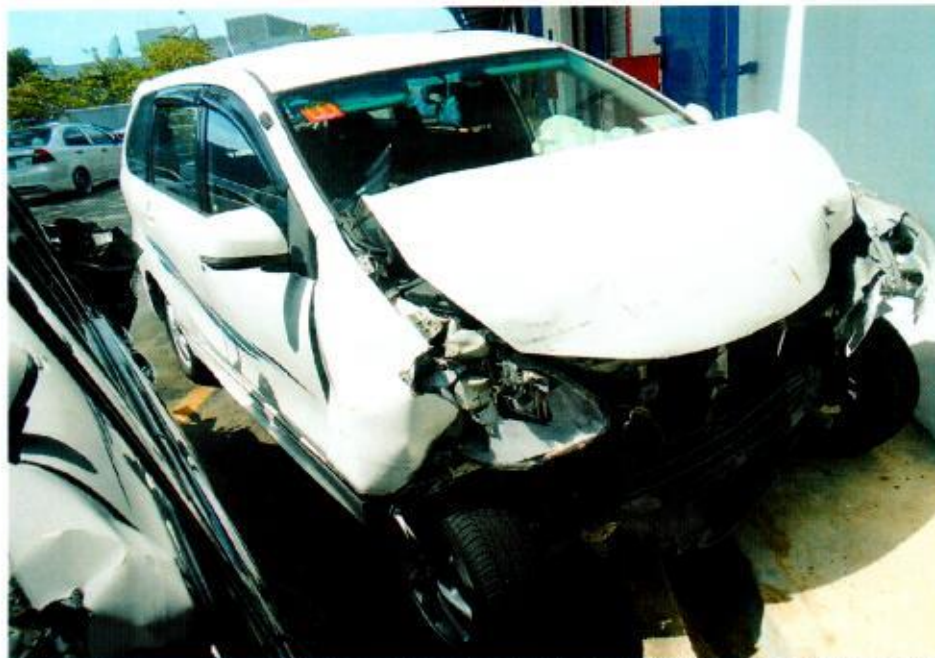
Photo 3 shows a general view of the front right portion of the Motor Car at the time of our inspection. The Motor Car was observed to have sustained extensive impact damage at its frontal portion.
