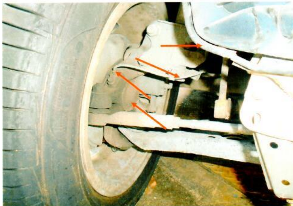
Photo 21 shows the braking components at the front left wheel of the Motor Car. We did not observe any leakage of brake fluid at the time of our inspection of the Motor Car.
