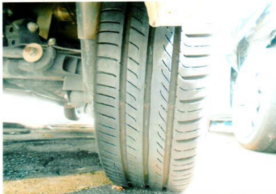
Photo 13 shows the condition of the rear right tyre of the Motor Car, which was observed to be in serviceable condition with remaining tread depth of approximately 6mm. There was also no tear, cut or burst mark(s) on the outer and the inner sidewalls as well as across the tread of this tyre.
