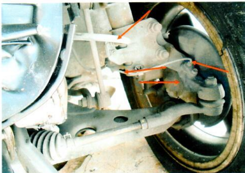
Photo 22 shows the braking components at the front right wheel of the Motor Car. We did not observe any leakage of brake fluid at the time of our inspection of the Motor Car.
