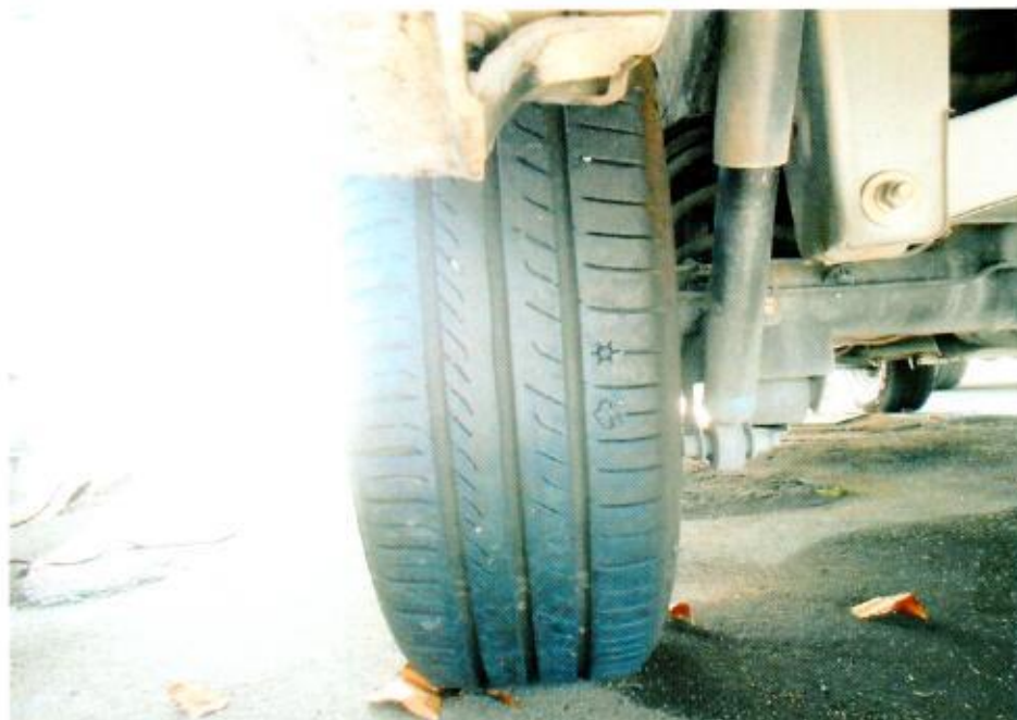
Photo 14 shows the condition of the rear left tyre of the Motor Car, which was observed to be in serviceable condition with remaining tread depth of approximately 6mm. There was also no tear, cut or burst mark(s) on the outer and the inner sidewalls as well as across the tread of this tyre.
