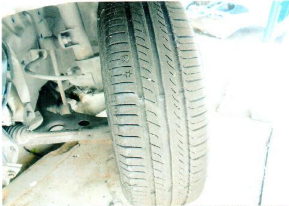
Photo 12 shows the condition of the front left tyre of the Motor Car, which was observed to be in serviceable condition with remaining tread depth of approximately 7mm. There was no tear, cut or burst mark(s) on the outer and the inner sidewalls as well as across the tread of this tyre, which was also sufficiently inflated for vehicular operation.
