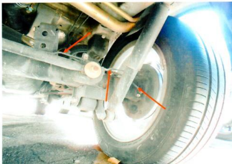
Photo 23 shows the braking components at the rear right wheel of the Motor Car. We did not observe any leakage of brake fluid at the time of our inspection of the Motor Car.
