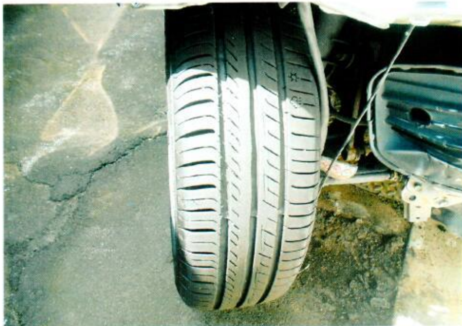
Photo 11 shows the condition of the front right tyre of the Motor Car, which was observed to be in serviceable condition with remaining tread depth of approximately 7mm. There was no tear, cut or burst mark(s) on the outer and the inner sidewalls as well as across the tread of this tyre.
