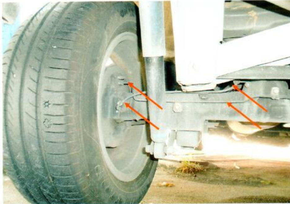
Photo 24 shows the braking components at the rear left wheel of the Motor Car. We did not observe any leakage of brake fluid at the time of our inspection of the Motor Car.
