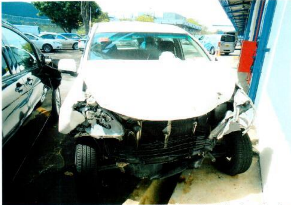
Photo 2 shows a general view of the frontal portion of the Motor Car at the time of our inspection. The Motor Car was observed to have sustained extensive impact damage at its frontal portion. The impact force was significant, causing the various parts and components inside the engine compartment to be damaged.
