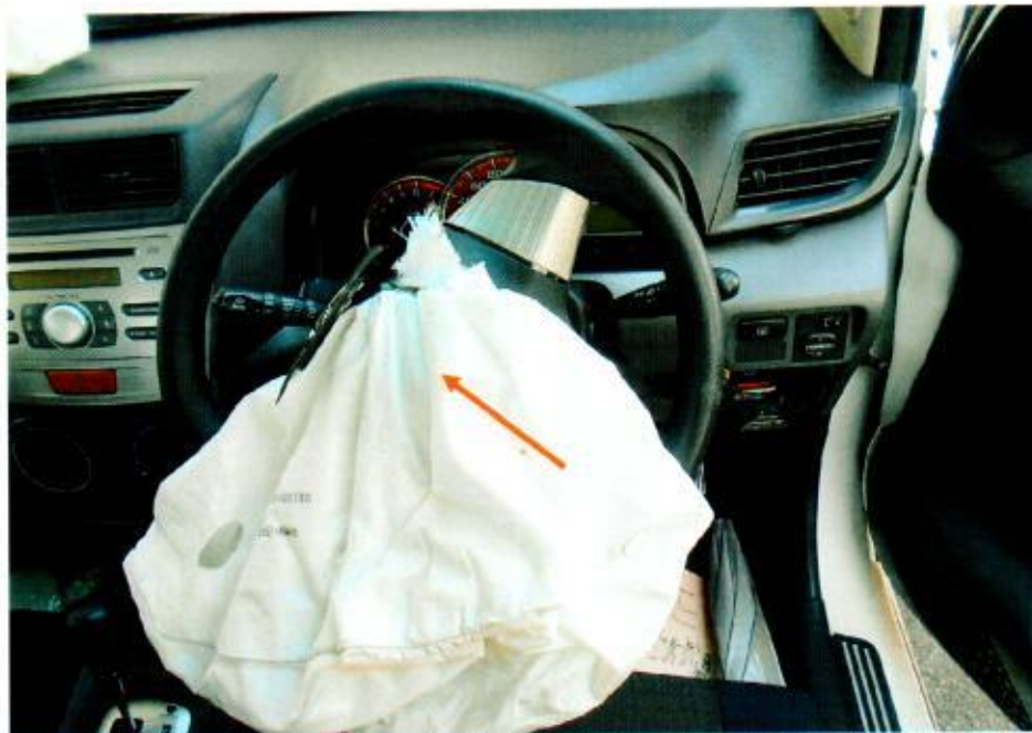
Photo 25 shows the evidence of the deployed driver's airbag indicates that the impact sensors and control module of the Motor Car's SRS were all in serviceable condition at the material time of accident.
