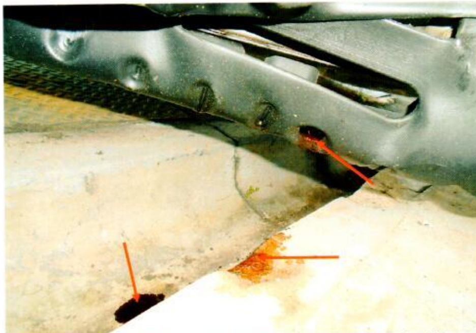
Photo 19 shows the damaged on the steering rack of the Motor Car. We were not able to conduct any tests on the steering system of the Motor Car due to the damage to this components, as well as leakage of power steering fluid.
