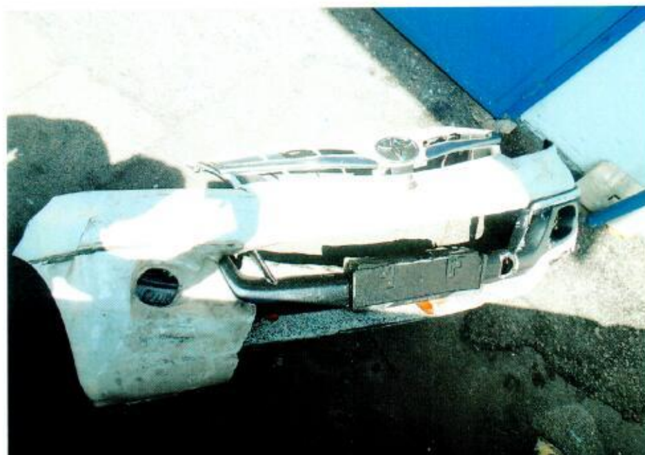
Photo 5 shows a closer view of the dislodged lower bumper of the Motor Car. The impact force was significant, causing the various parts and components inside the engine compartment to be pushed inwards, towards the rear of the Motor Car.
