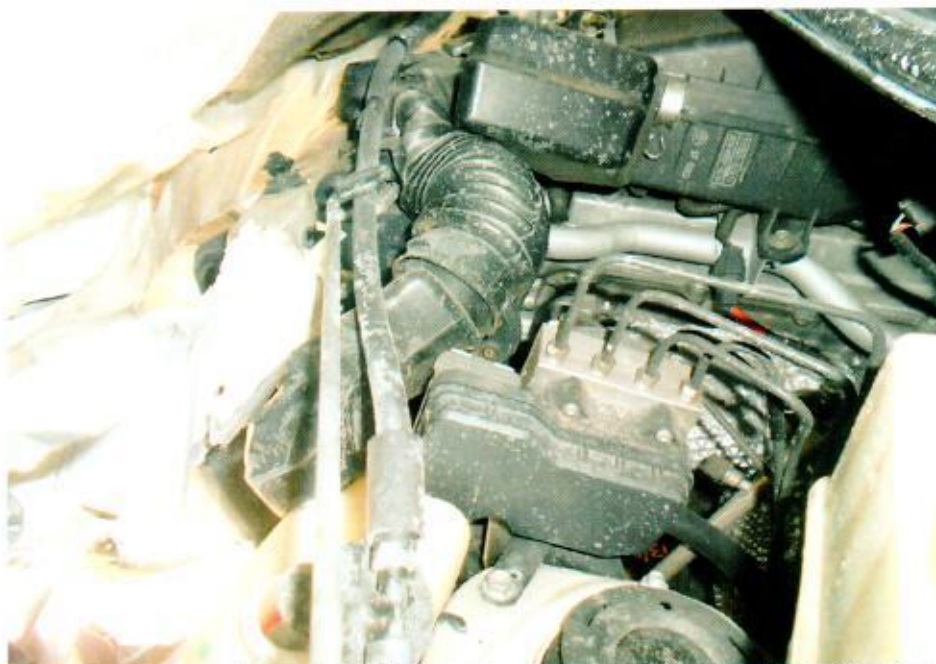
Photo 6 shows a closer view of the engine compartment of the Motor Car from the left hand side of the bonnet opening. The impact force was significant, causing the various parts and components inside the engine compartment to be pushed inwards, towards the rear of the Motor Car.
