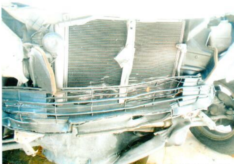
Photo 4 shows a general view of the front portion of the Motor Car at the time of our inspection. Its radiator was observed to have sustained extensive impact damage due to the accident's impact.
