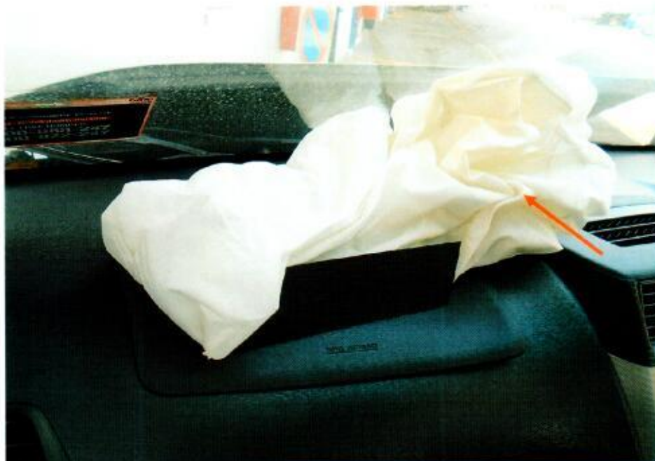
Photo 26 shows the evidence of the deployed front passenger's airbag indicates that the impact sensors and control module of the Motor Car's SRS were all in serviceable condition at the material time of accident.
