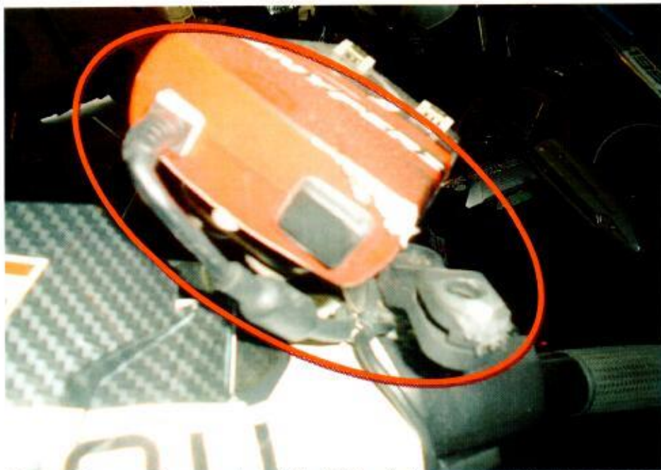
Photo 7 shows a close-up view of the ERP unit c/w bracket of the Motorcycle at the time of our inspection. It was observed to have sustained with damages due to the accident collision.
