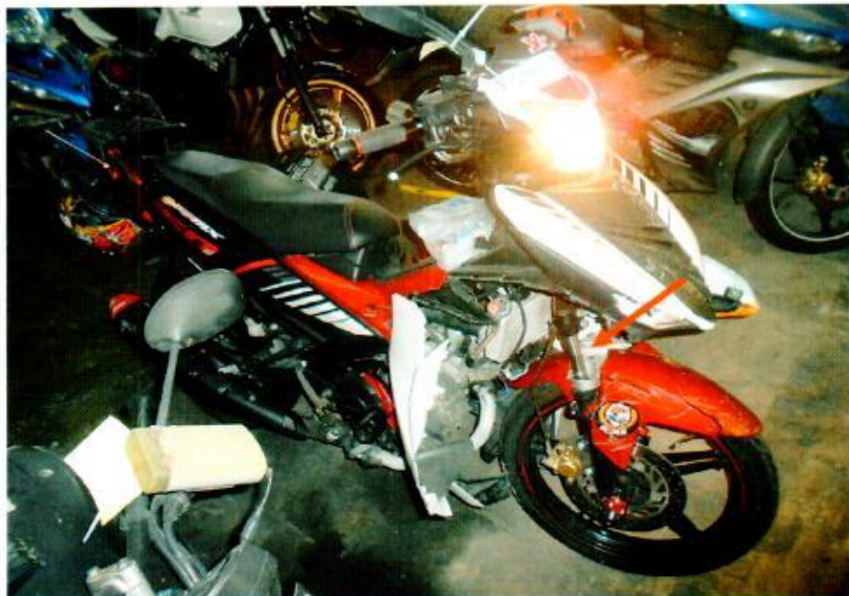
Photo 2 shows a general view of the front right body of the Motorcycle at the time of our inspection. The Motorcycle was observed to be sustained with relatively extensive impact due to the accident collision. Amongst the body parts damaged was its front fork (arrowed), which was observed to be bent inwards.
