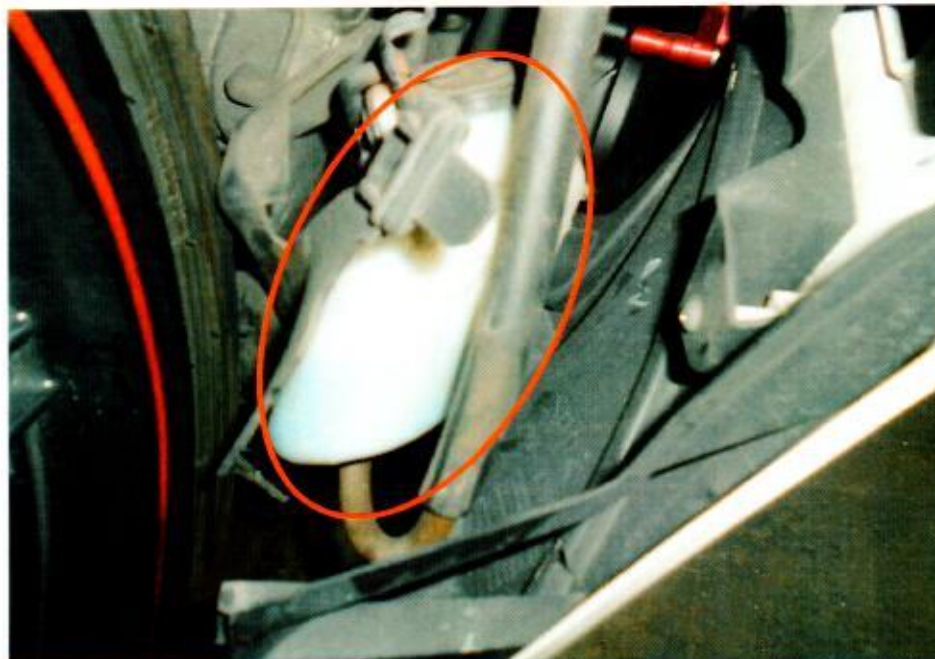
Photo 13 shows the radiator reservoir was not affected by the accident's collision impact.
