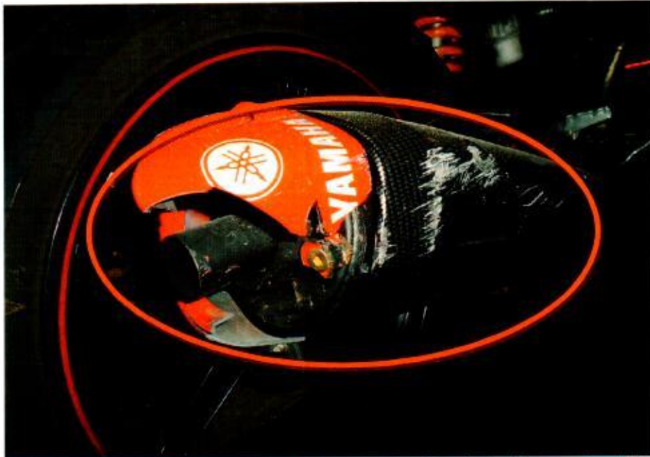
Photo 5 shows a close-up view of the exhaust muffler of the Motorcycle at the time of our inspection. It was observed to have sustained with damages due to the accident collision.
