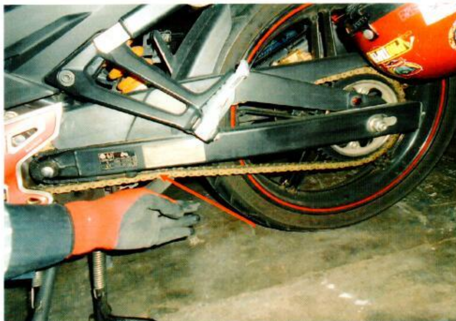
Photo 15 shows the general view of the gear train (arrowed) of the Motorcycle, which was observed to be intact with no misalignment. It was also adequately lubricated for operating purposes. Free play tension was also observed & found adequately acceptable.
