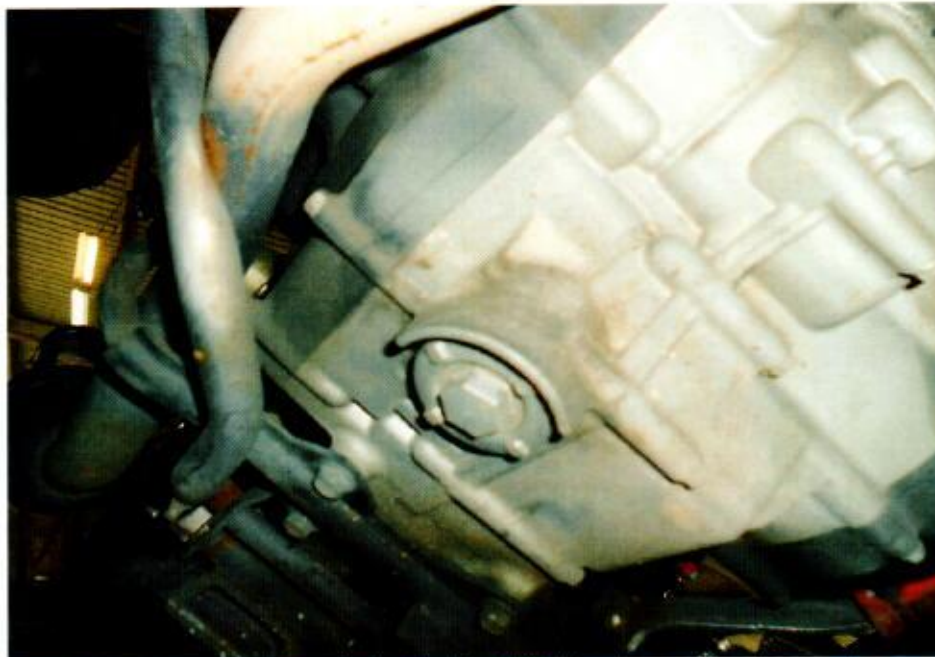
Photo 11 shows sign(s) or indication(s) of fluid leakage stain observed around the engine undercarriage area of the Motorcycle.
