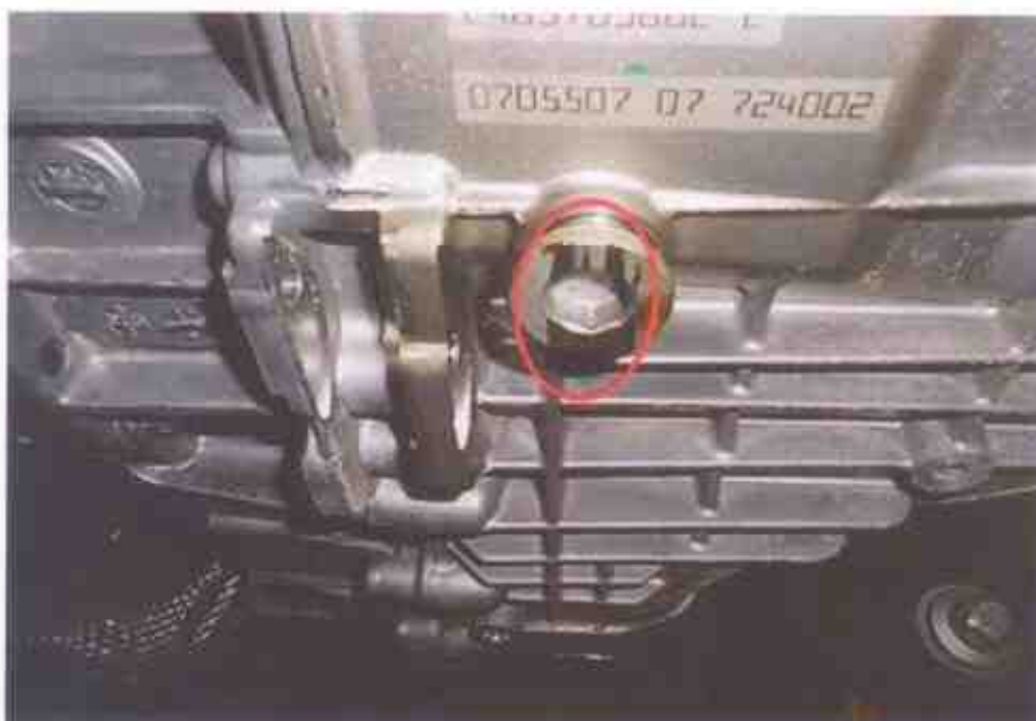
Photo 6 shows a closer view of the drain plug for the transmission fluid of the Insured Vehicle. Upon closer examination, a single cut mark (circled) was observed, stretching across the underside of the drain plug. The cut on the underside of the drain plug correspond to the Insured Vehicle going over an object.
