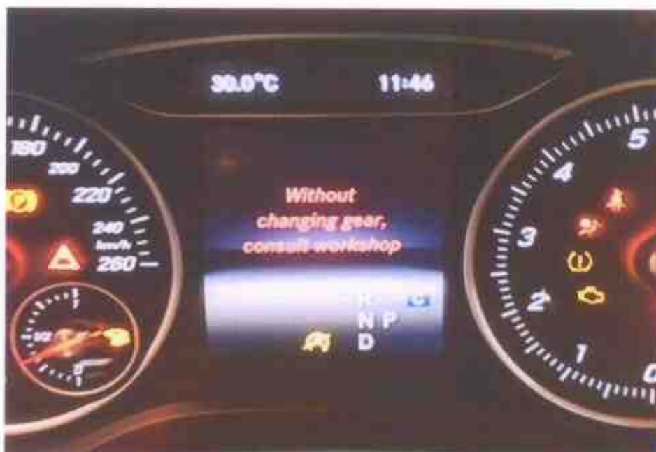
Photo 7 shows the warning message "without changing gear, consult workshop" that appeared on the instrument panel of the Insured Vehicle after the key was turned to half crank position. This would indicate a fault to the transmission of the Insured Vehicle.
