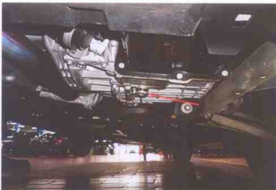
Photo 4 shows the drain plug (arrowed) for the transmission fluid of the Insured Vehicle. The drain plug was observed to be not fully secured/tightened.
