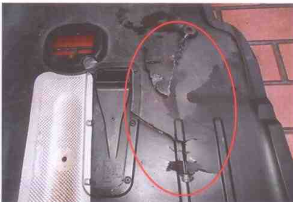
Photo 2 shows the torn second engine undercover of the Insured Vehicle. The second engine undercover was found to be torn at a single area (circled). The nature of the tear corresponds to a cut that was caused by a sharp edge object.
