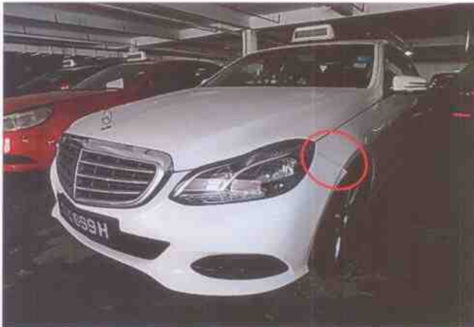
Photo 1 shows the general left view of the front portion of the Taxi at the time of the Pre- Repair Survey conducted by LKK Auto Consultants Pte. Ltd. which was taken 2 days after the accident. The damages to the Taxi were observed to be confined to the left front portion, particularly to its front bumper and left front tyre fender (circled).
