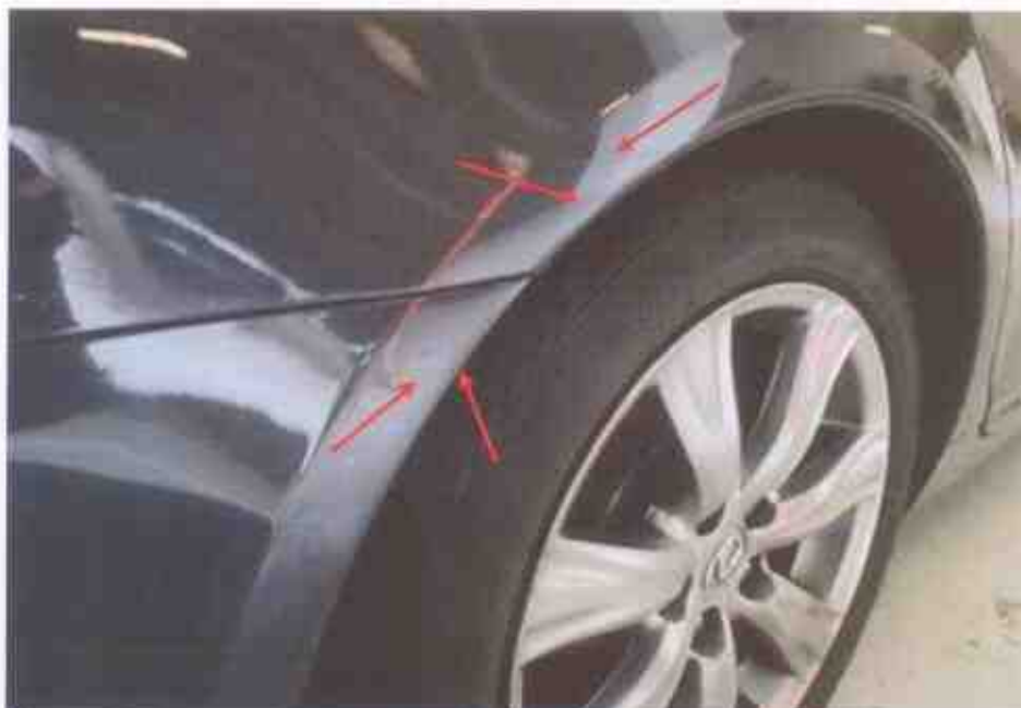
Photo 14 shows a close up view of the paint graze marks on the right rear tyre fender (red arrows).
