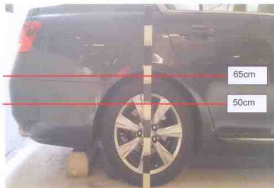
Photo 18 shows the height measurement being conducted on the right rear portion of the Lexus. The body part within the height range of 50cm to 65cm above ground was the edges of the right rear wheel rim as well as the right rear tyre fender where the graze marks were found.
