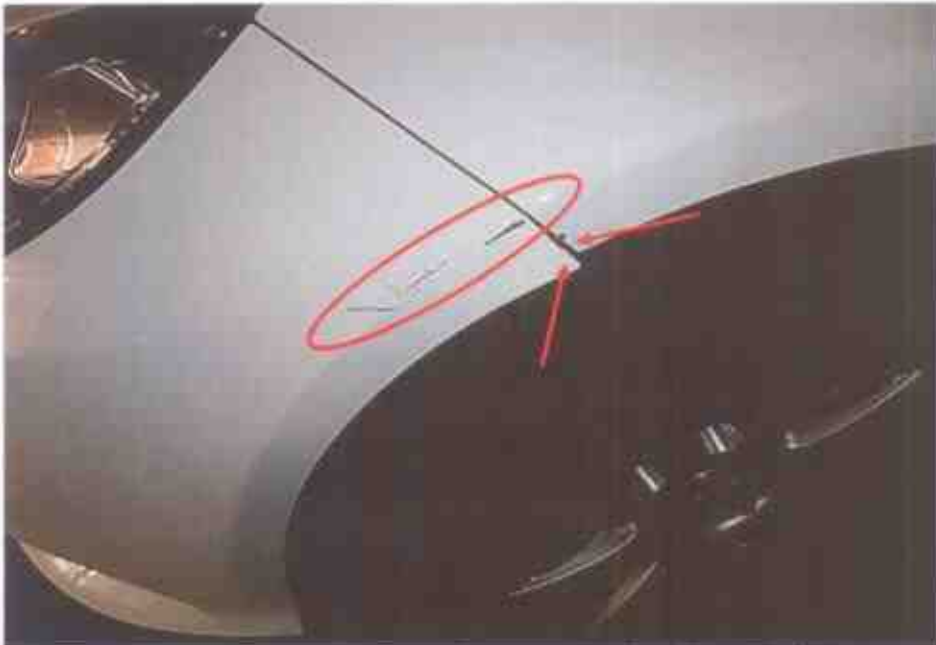
Photo 2 shows a closer view of the left front portion of the Taxi. The front bumper was dislodged at the left corner edge (arrowed). Paint graze marks were also found on the left portion of the front bumper as well as on the left front tyre fender (circled).
