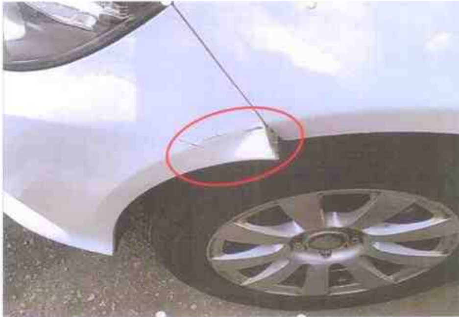
Photo 15 shows a close up view of the damages sustained to the left front portion of the Taxi post- accident (circled). Upon closer examination of these photos, the damages seem to be consistent with the photos taken during the accident reporting as well as the Pre- Repair Survey.
