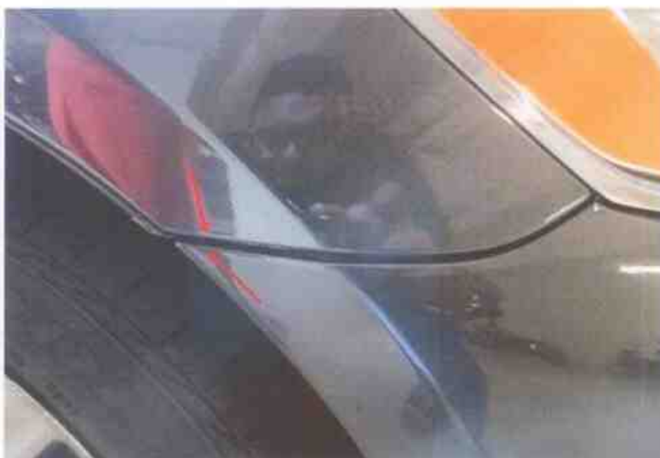
Photo 7 shows the misalignment of the Lexus's front bumper at the right corner edge (arrowed).
