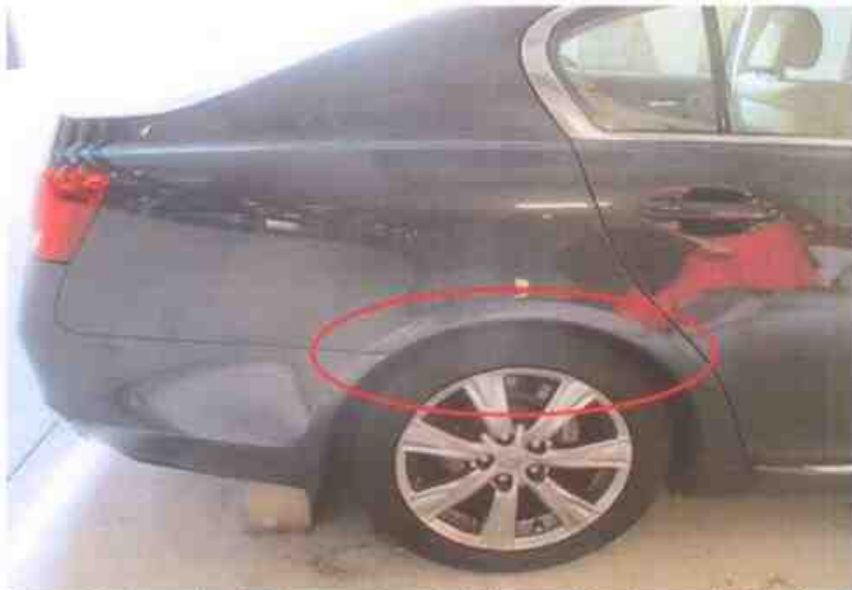
Photo 12 shows the right rear portion of the Lexus. We observed several paint graze marks on the right rear tyre fender as well as relatively minor marks of grazing nature around the edges of the right rear wheel rim (circled).
