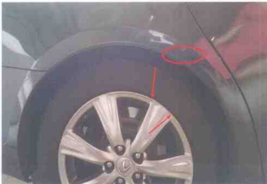
Photo 13 shows a close up view of the paint graze marks on the right rear tyre fender (circled) as well as relatively minor marks of grazing nature around the edges of the right rear wheel rim (red arrows).
