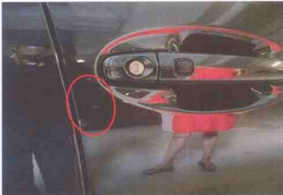
Photo 10 shows the paint graze marks found near the handle of the driver door of the Lexus (circled).
