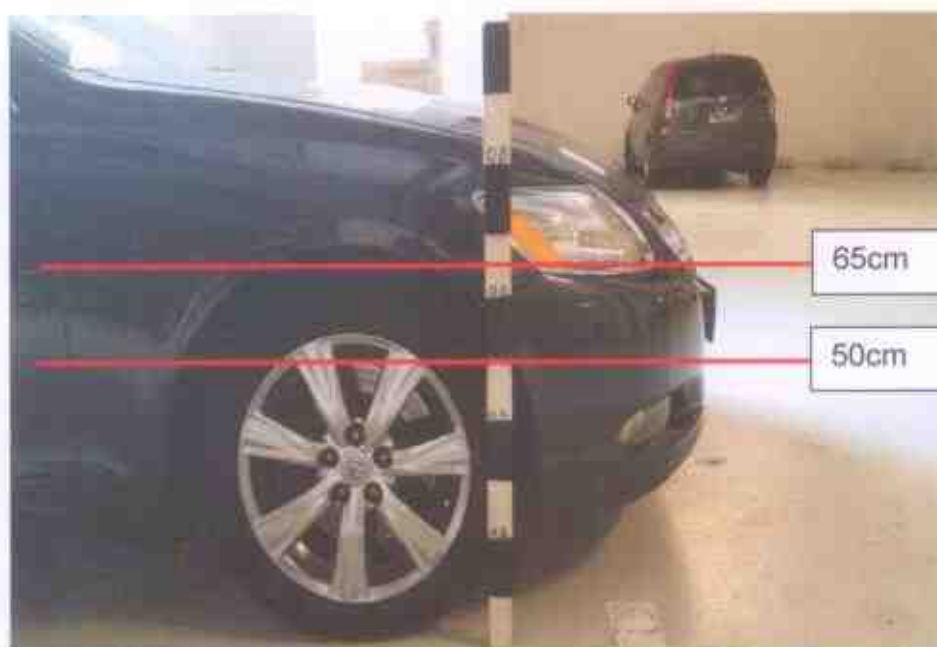
Photo 17 shows the height measurement being conducted on the right front portion of the Lexus. The body part within the height range of 50cm to 65cm above ground was the edges of the right front wheel rim where the graze marks were found.
