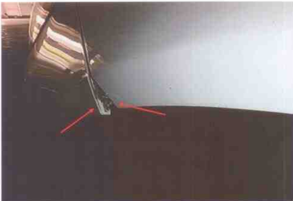
Photo 3 shows a close up view of the dislodgement of the Taxi's front bumper at the left corner edge (arrowed).
