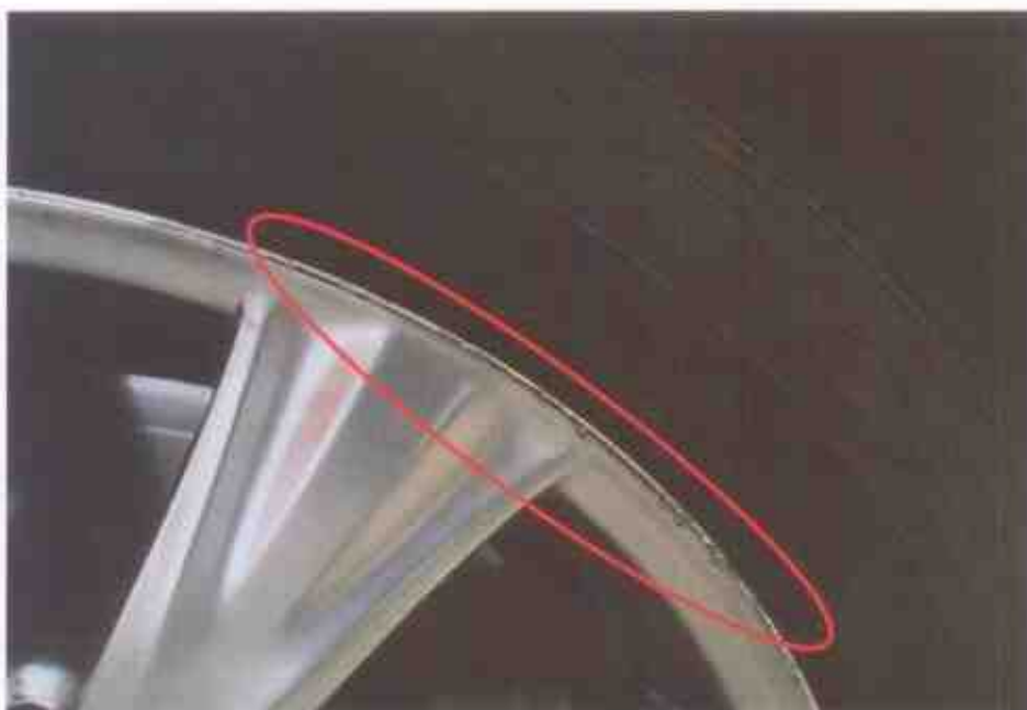
Photo 9 shows a close up view of the relatively minor marks of grazing nature observed around the edges of the right front wheel rim of the Lexus (circled).
