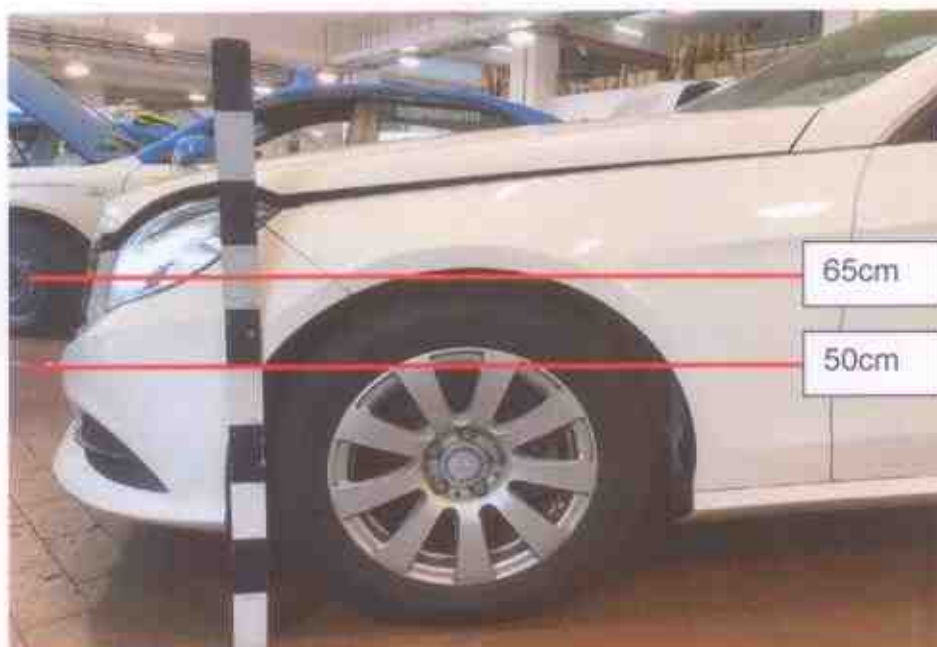
Photo 16 shows the height measurement being conducted on the left front portion of the Taxi (using a similar make and model). The paint graze marks and the dislodgement of the front bumper on the left front portion of the Taxi were measured to be between the height ranges of 50cm to 65cm above ground level.
