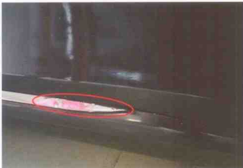
Photo 11 shows a close up view of the dent found on the driver door body chrome trim (circled).
