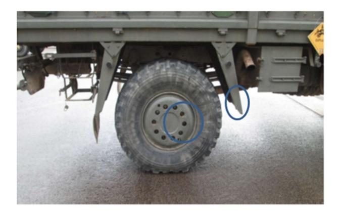
Close View of Impact Point to MID 20504: Insignificant scratches to right rear tyre guard and rims
