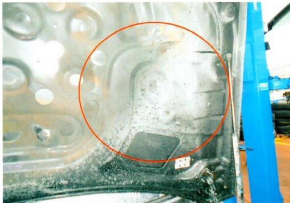
Photo 5 shows the burn pattern and whitish burn marks (circled) that were found on the underside of the front bonnet of the Insured Vehicle. Such whitish burn marks are a result of exposure to prolong heat intensity, which may indicate where the fire had started. Rust would also begin to develop on these areas soon after the fire.
