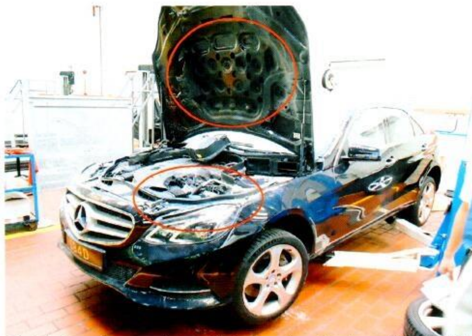
Photo 1 shows the general view of the front portion of the Insured Vehicle at the time of our inspection. The fire damage to the Insured Vehicle was confined to its front bonnet, at the centre area; engine parts were amongst the body parts that were found to have been affected as a result of the fire.
