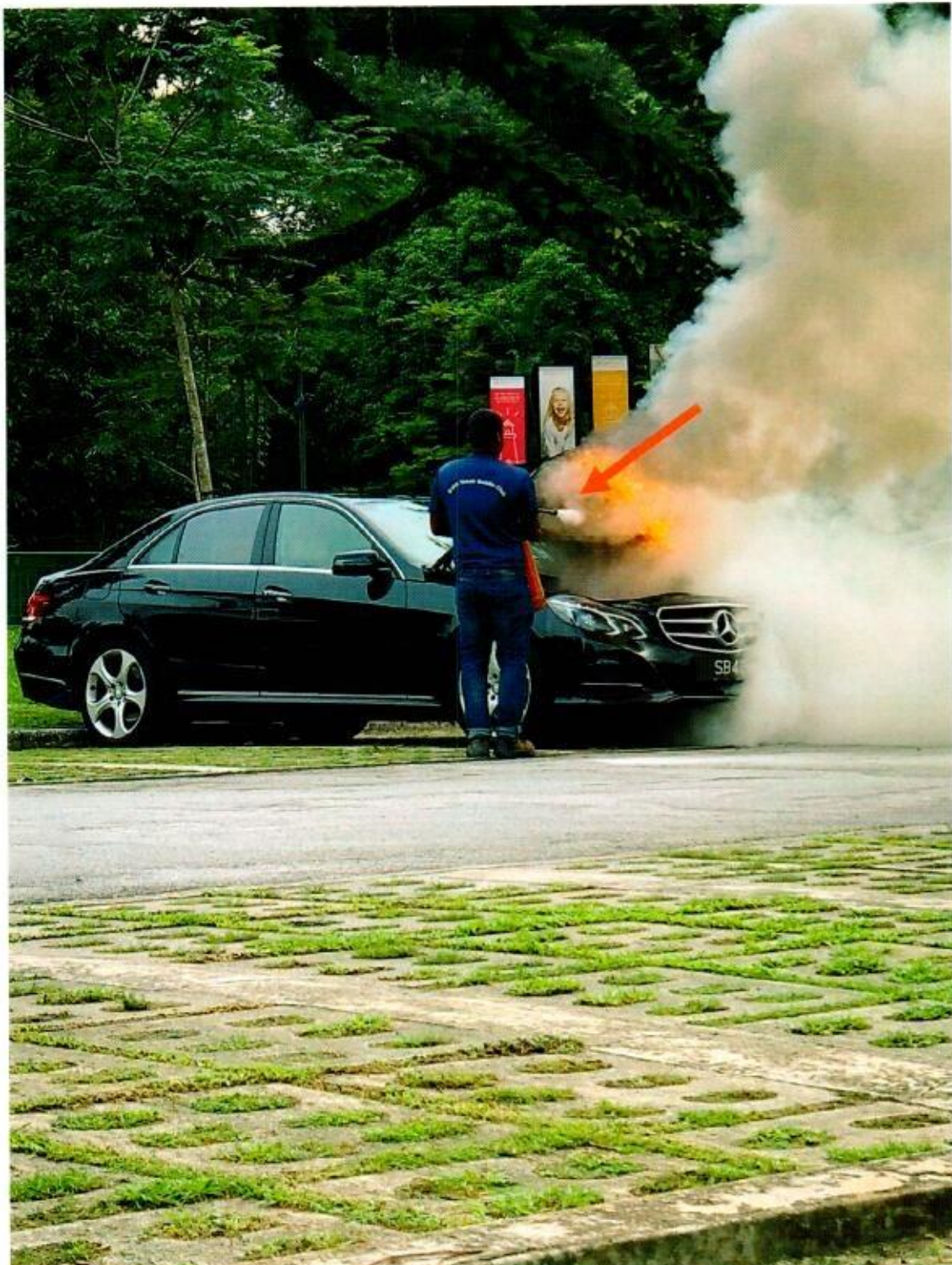
Photo 14 shows the Insured Vehicle at the incident scene while the club staff extinguishing the fire (arrowed). There appears to be no abnormal foreign material(s) and/or object(s) found on the ground in the immediate area where the Insured Vehicle was parked. In general, the information that could be gathered from these photographs had corresponded to the events that were related to us by Mr Mark Shaw & Ms Tiara.
