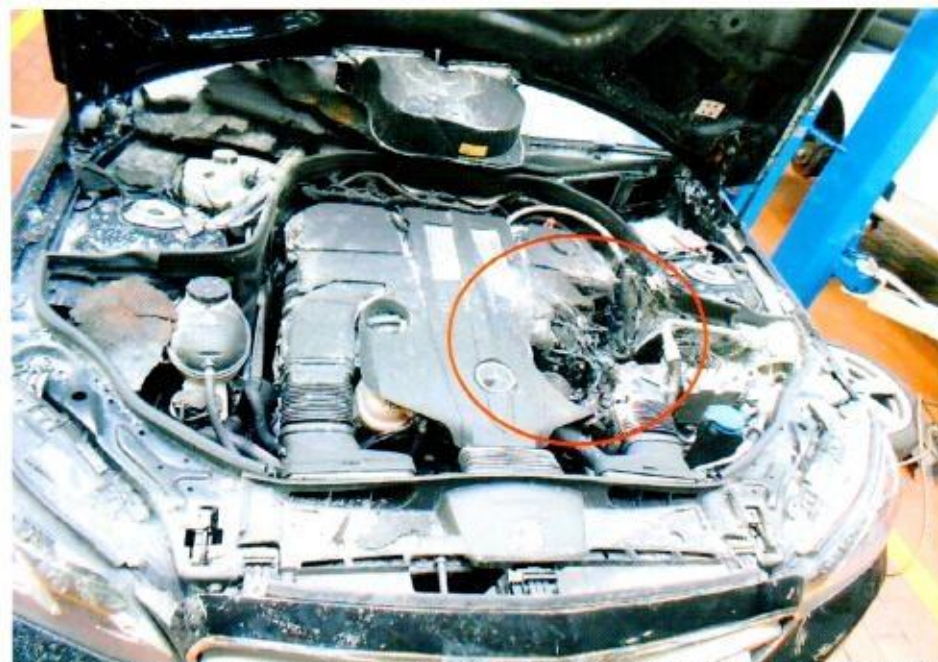
Photo 2 shows the general view of the front centre portion of the Insured Vehicle at the time of our inspection. The fire damage to the Insured Vehicle was confined to its front bonnet, at the centre area; engine parts were amongst the body parts that were found to have been affected as a result of the fire.
