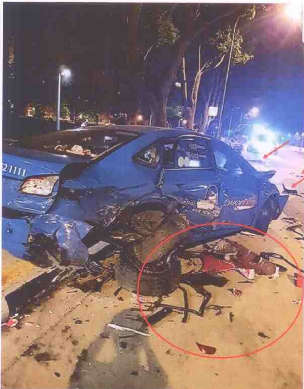
Photo 5 shows the accident scene after the accident. Vehicular debris could be seen lying mainly within the bus bay, on the right side of SHC 8317Z. This had included broken body parts (circled) from SLM 10K. Upon closer examination of the photograph, I had also observed some vehicular debris (arrowed) lying on the extreme left lane after the location where SHC 8317Z had stopped.
