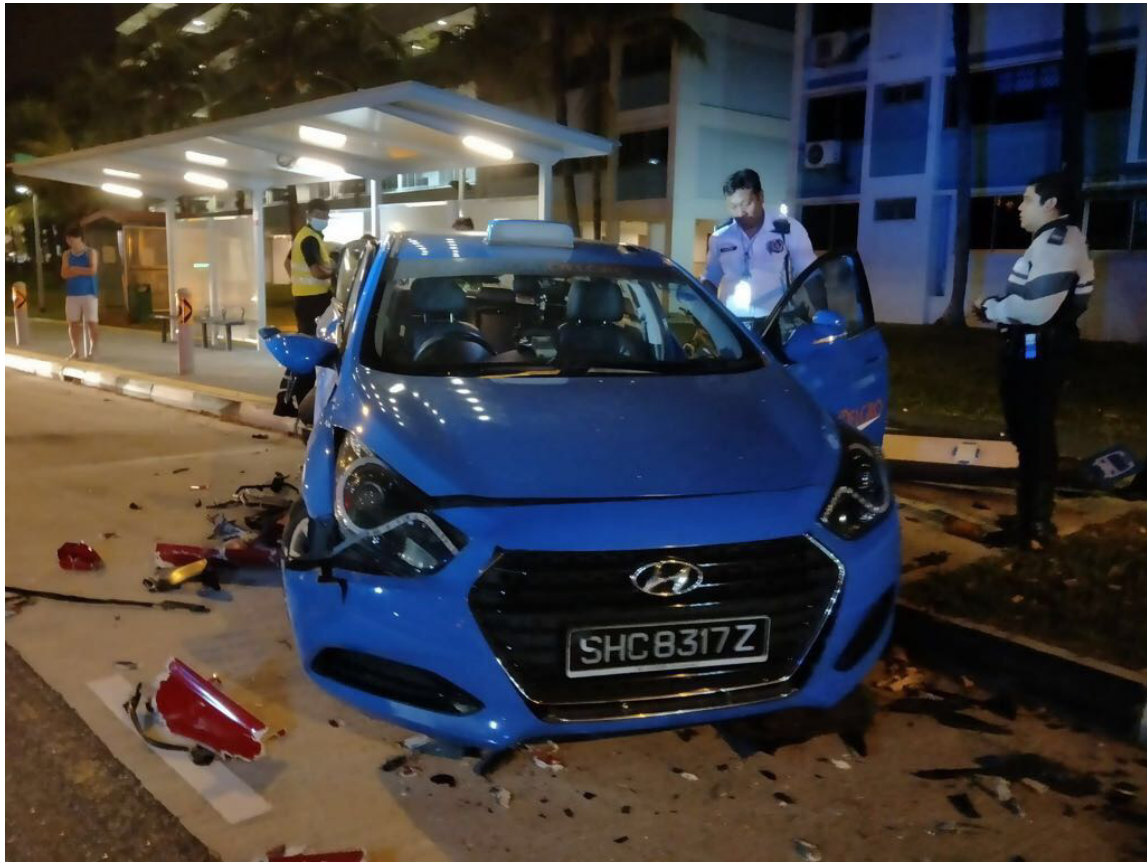
Photo 1 shows a general view of the frontal portion of SHC 8317Z after the accident. It was observed to have come to a complete rest with its entire body within the bus bay. It was stopped in a slanted position approximately 40° towards the right of the direction of traffic flow.
