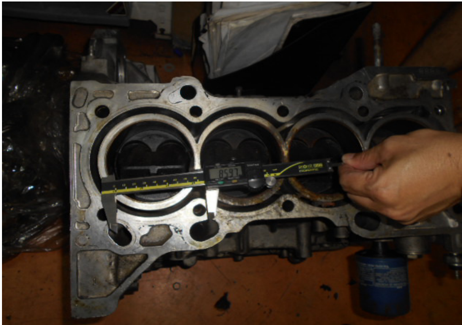
Photo 5 shows measurement being carried out to the bore of cylinder 1 of the Honda engine. The bore and stroke measurements of the Honda engine were carried out using a digital Vernier Caliper, which was calibrated prior to the start of measurements.
