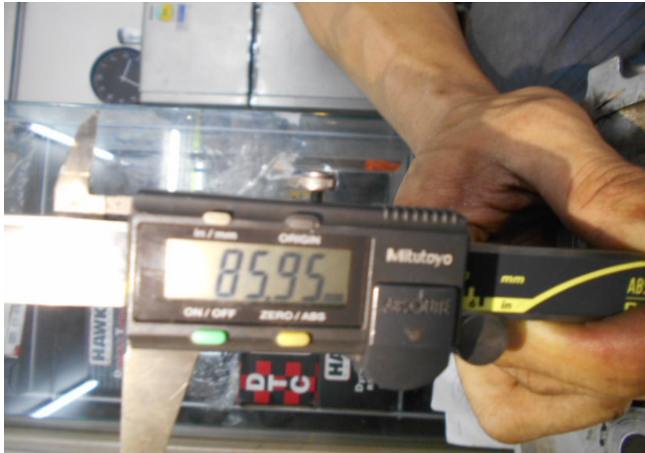
Photo 19 shows the stroke measurement of cylinder 4, which was recorded to be 85.95mm.
