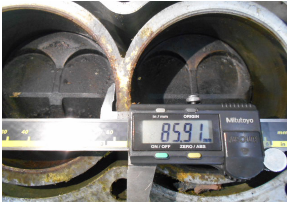
Photo 11 shows the bore measurement of cylinder 2, which was recorded to be 85.91mm.
