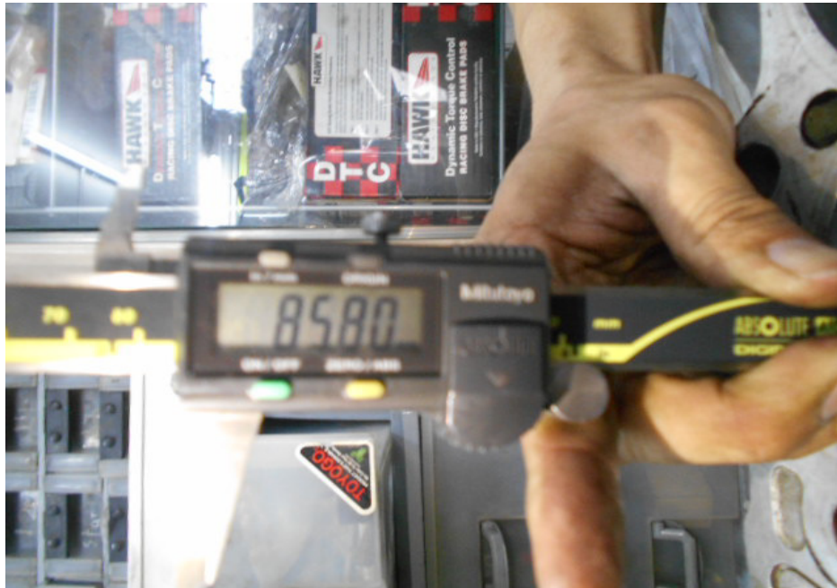
Photo 9 shows the stroke measurement of cylinder 1, which was recorded to be 85.80mm.
