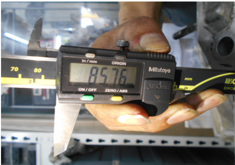
Photo 16 shows the stroke measurement of cylinder 3, which was recorded to be 85.76mm.
