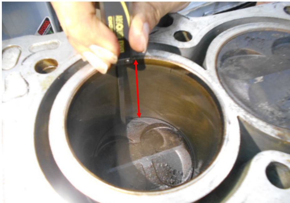
Photo 8 shows measurement being carried out to the stroke of cylinder 1 of the Honda engine. The bore and stroke measurements of the Honda engine were carried out using a digital Vernier Caliper.
