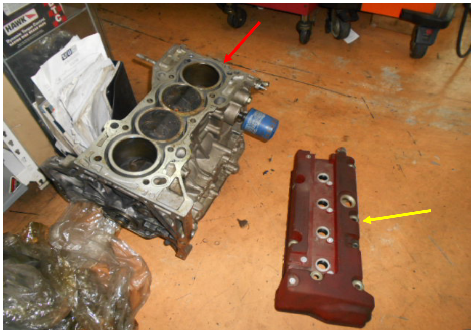
Photo 4 shows the top block (yellow arrow) of the Honda engine separated from its bottom block (red arrow). This was to enable me to carry out measurements of its cylinders, in particular the bore and stroke measurements of each cylinder, which typically can be used to determine the engine displacement or more commonly referred to as engine cc.
