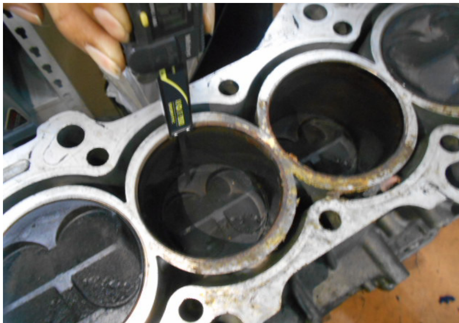
Photo 12 shows measurement of the stroke for cylinder 2 of the Honda engine that I had inspected.
