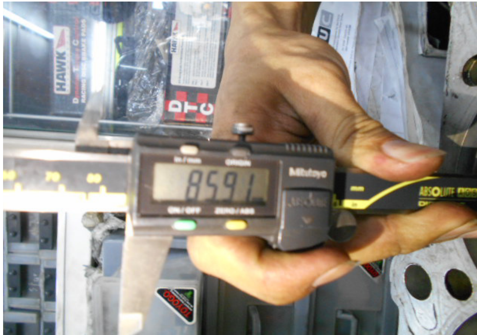
Photo 13 shows the stroke measurement of cylinder 2, which was recorded to be 85.91mm.
