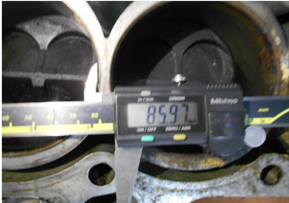
Photo 7 shows the bore measurement of cylinder 1, which was recorded to be 85.97mm.
