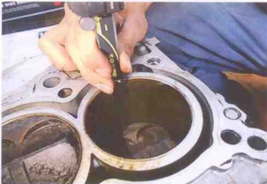
Photo 18 shows measurement being carried out to the stroke of cylinder 4 of the Honda engine. The bore and stroke measurements of the Honda engine were carried out using a digital Vernier Caliper, which was calibrated prior to the start of measurements.
