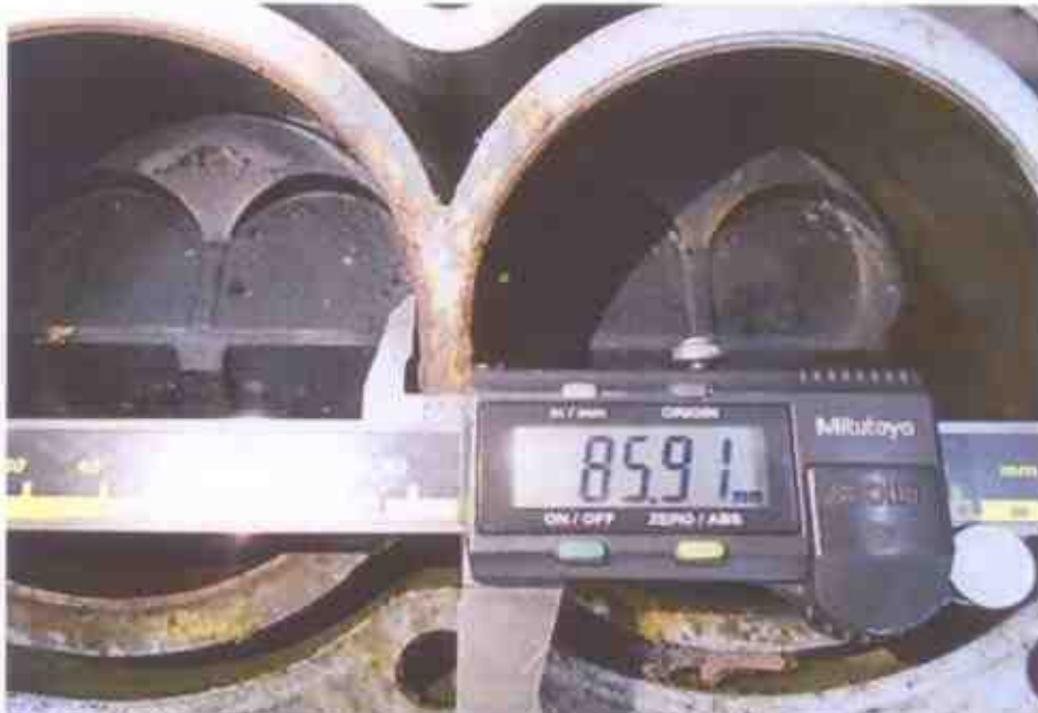
Photo 11 shows the bore measurement of cylinder 2, which was recorded to be 85.91mm.
