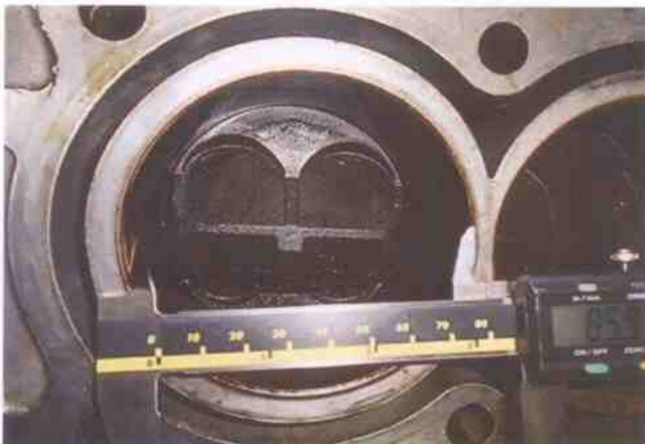
Photo 10 shows measurement being carried out to the bore of cylinder 2 of the Honda engine. The bore and stroke measurements of the Honda engine were carried out using a digital Vernier Caliper, which was calibrated prior to the start of measurements.
