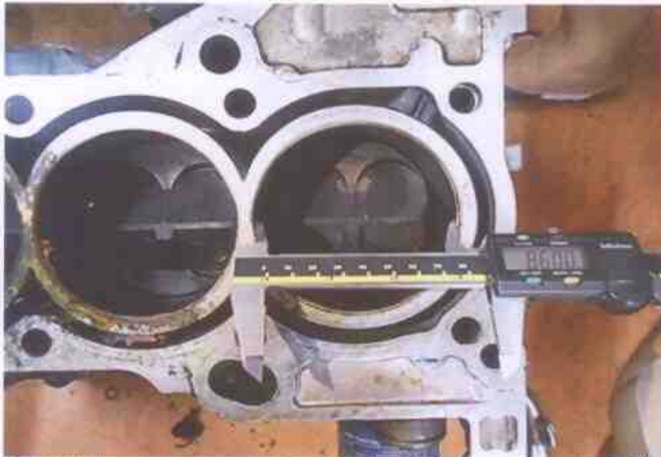
Photo 17 shows measurement being carried out to the bore of cylinder 4 of the Honda engine. The bore and stroke measurements of the Honda engine were carried out using a digital Vernier Caliper. The bore measurement of cylinder 4 was recorded to be 86.00mm.
