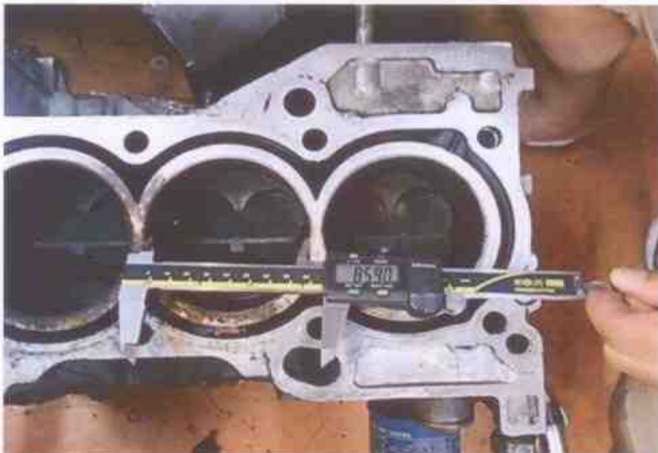
Photo 14 shows measurement being carried out to the bore of cylinder 3 of the Honda engine. The bore and stroke measurements of the Honda engine were carried out using a digital Vernier Caliper. The bore measurement of cylinder 3 was recorded to be 85.90mm.
