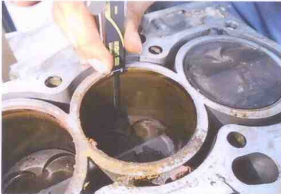
Photo 15 shows measurement of the stroke for cylinder 3 of the Honda engine that I had inspected.
