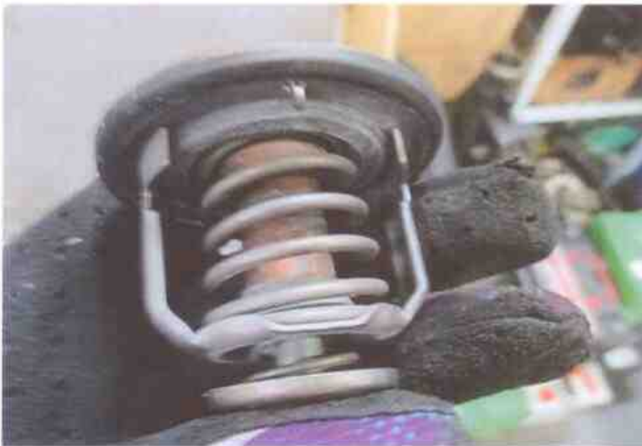
Photo 12 shows a close up view of the Insured Vehicle's thermostat which was observed to be partially burnt and/or melted.
