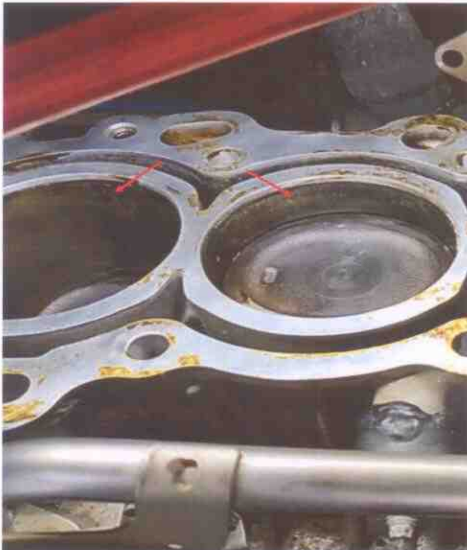
Photo 8 shows the scoring marks observed on the cylinder walls of the engine block (arrowed). Causation of such scoring marks is due to the pistons which are made of aluminium heating up faster than the engine block. Due to the overheating of the engine, the pistons will expand radically as they get hot, which is not the case for the cylinders of the engine block. The pistons will bind against the cylinder walls thus badly scoring those walls.
