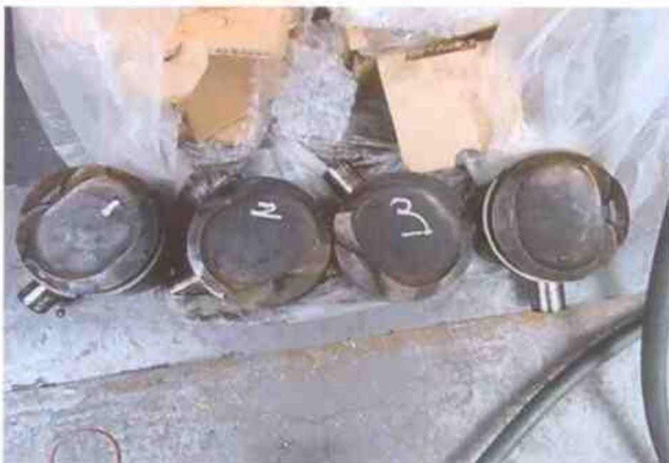
Photo 5 shows the pistons of the Insured Vehicle which were observed to be severely burnt
