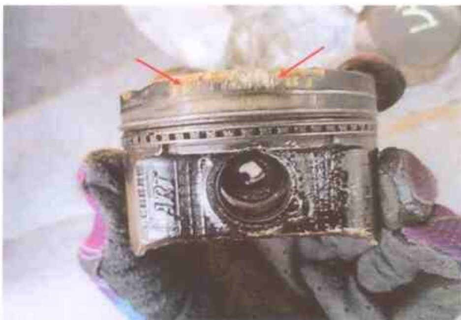
Photo 7 shows the scoring marks observed on the sides of 1 of the severely burnt pistons (arrowed). Causation of such scoring marks is due to the pistons which are made of aluminium heating up faster than the engine block. Due to the overheating of the engine, the pistons will expand radically as they get hot, which is not the case for the cylinders of the engine block. The pistons will bind against the cylinder walls thus badly scoring those walls, burning and cracking the pistons as well as the piston rings.
