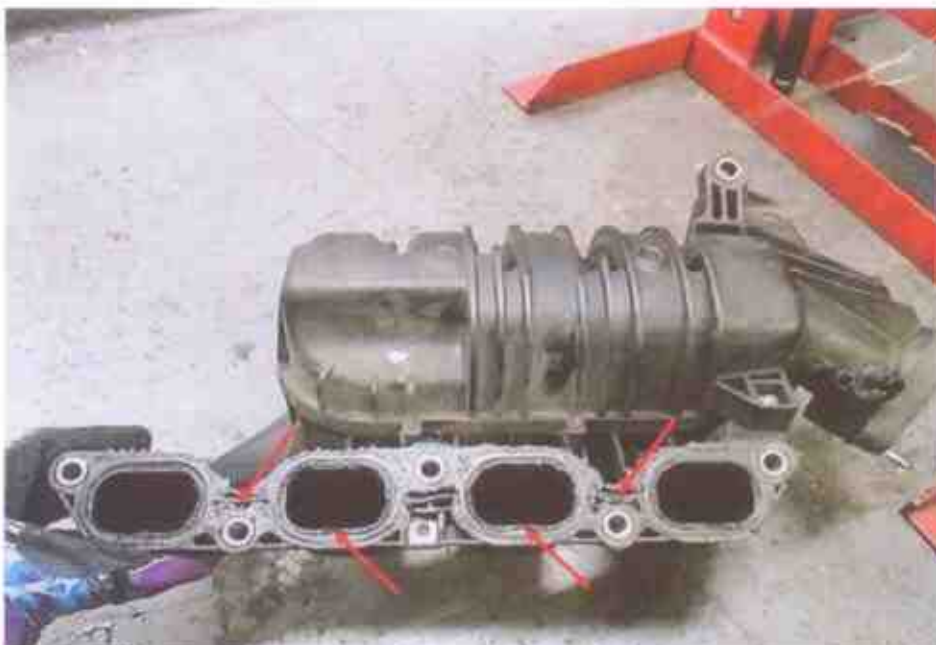
Photo 3 shows the engine inlet manifold of the Insured Vehicle which was observed to be partially burnt and/or melted (arrowed).
