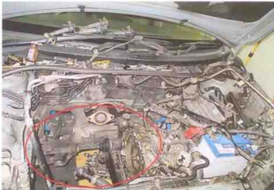
Photo 2 shows the general view of the engine compartment of the Insured Vehicle at the time of our inspection. We observed that the engine had been dismantled from the engine bay and dismantled. The various components of the Insured Vehicle's cooling system had also been removed from the front portion of the engine compartment (circled).
