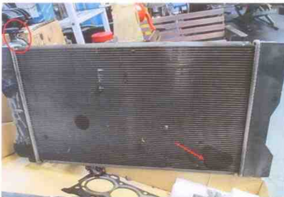
Photo 9 shows the radiator of the Insured Vehicle which was observed to be partially burnt and/or melted (arrowed) and the broken radiator outlet joint (circled).
