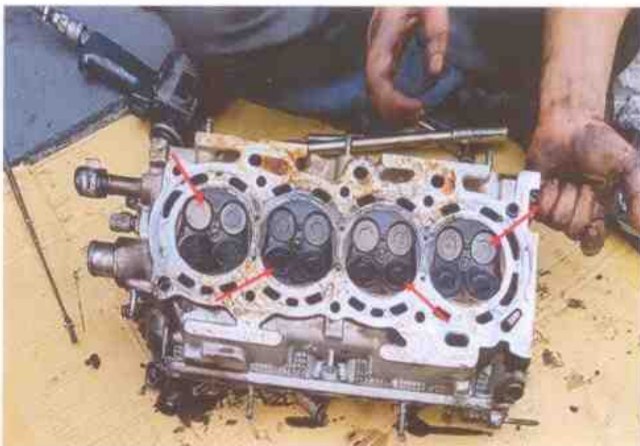
Photo 4 shows the engine valves and engine valve seals of the Insured Vehicle which were observed to be partially burnt and/or melted (arrowed).
