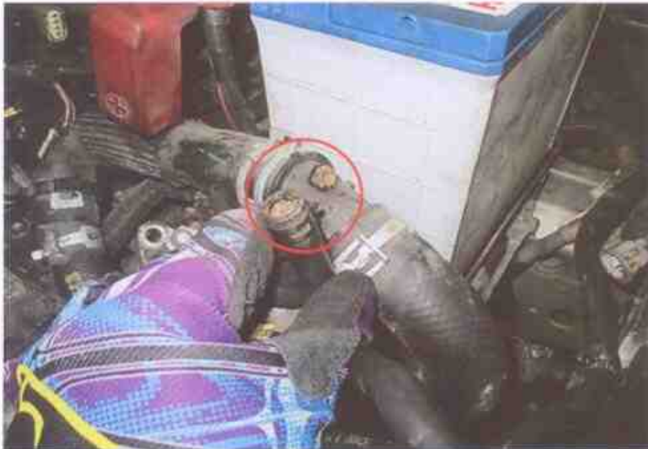
Photo 13 shows the broken radiator hose caused by overheating of the Insured Vehicle (circled).
