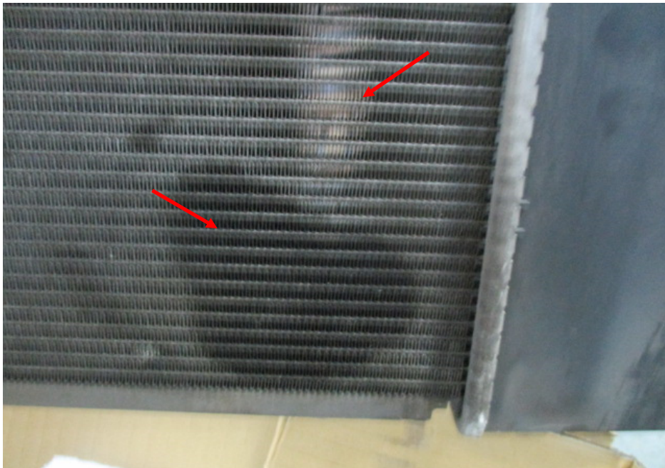
Photo 10 shows a close up view of the radiator of the Insured Vehicle which was observed to be partially burnt and/or melted (arrowed).
