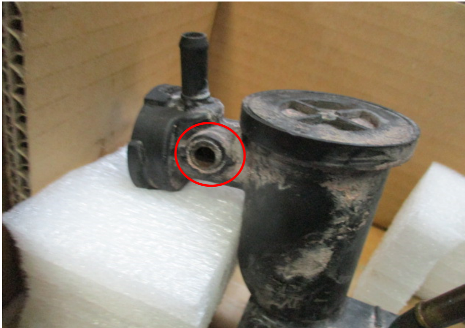
Photo 11 shows a close up view of the broken radiator outlet joint (circled).
