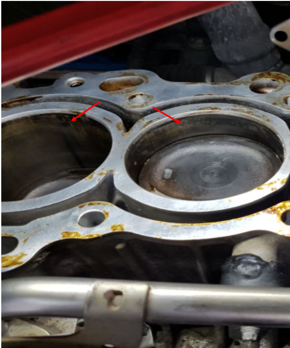
Photo 8 shows the scoring marks observed on the cylinder walls of the engine block (arrowed). Causation of such scoring marks is due to the pistons which are made of aluminium heating up faster than the engine block. Due to the overheating of the engine, the pistons will expand radically as they get hot, which is not the case for the cylinders of the engine block. The pistons will bind against the cylinder walls thus badly scoring those walls.
