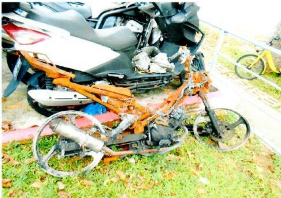
Photo 2 shows the right portion view of the Insured Vehicle at the time of our inspection. The Insured Vehicle was noted to have sustained fire damages that severely effected on the entire parts of the Insured Vehicle.
