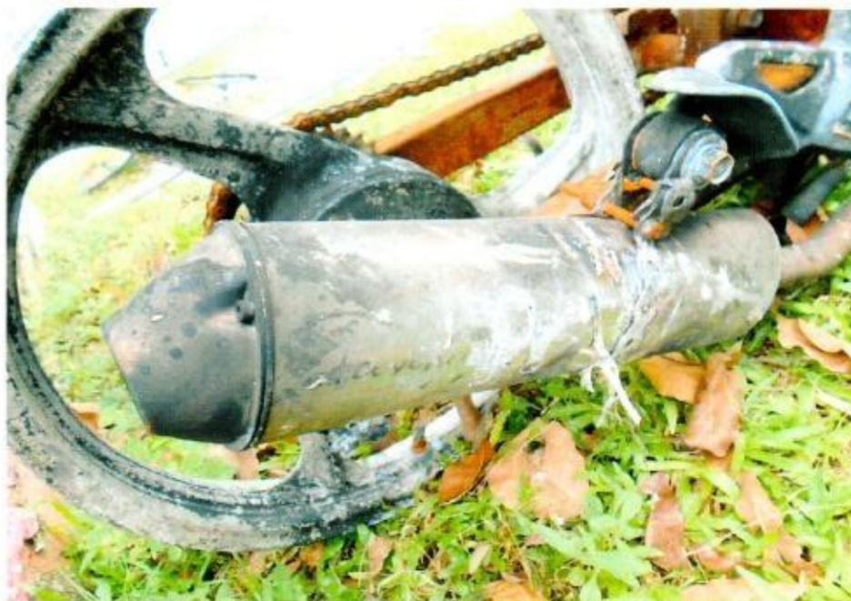
Photo 8 shows the after-market exhaust pipe. It was believe from manufacturer called 'LeoVince'. It was said to be an approved LTA after-market exhaust pipe.
