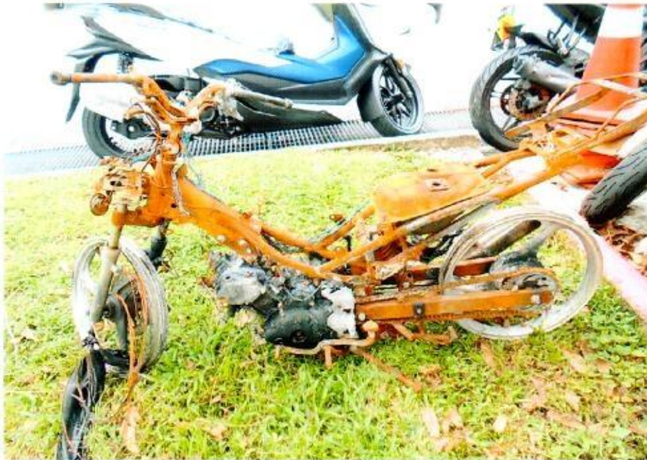
Photo 1 shows the left portion view of the Insured Vehicle at the time of our inspection. The Insured Vehicle was noted to have sustained fire damages that severely effected on the entire parts of the Insured Vehicle.
