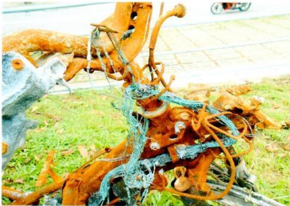
Photo 6 shows the front portion of the Insured Vehicle at the time of our inspection. Wirings were noted to have greenish residual likely due to an electrical short circuit.
