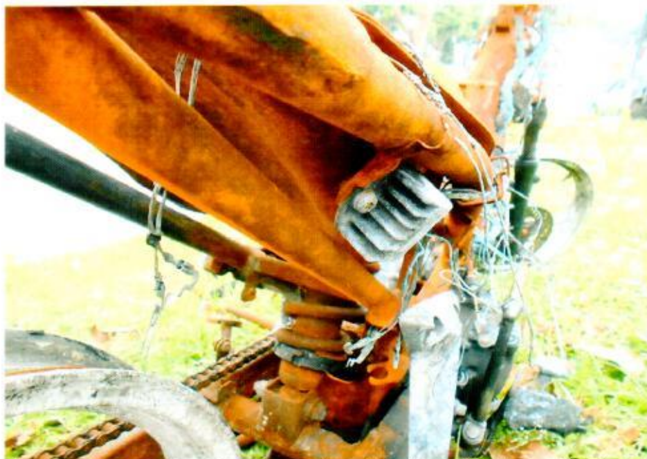
Photo 7 shows the view from rear portion of the Insured Vehicle at the time of our inspection. Stretches of wires were noted to have greenish residual likely due to an electrical short circuit.
