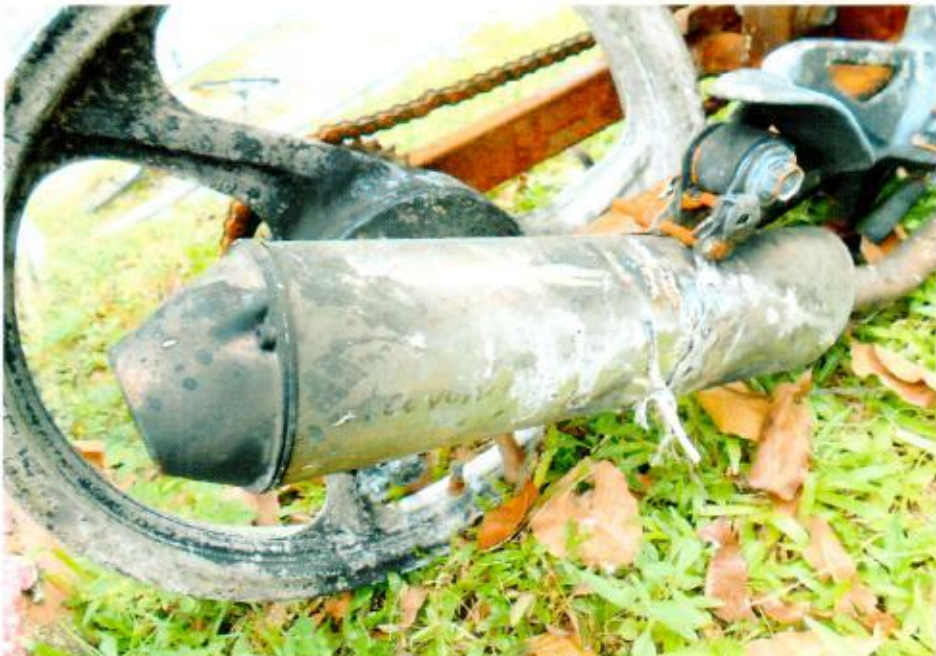
Photo 4 shows the after-market exhaust pipe. It was believe from manufacture called 'LeoVince'. It was said to be an approved LTA after-market exhaust pipe.
