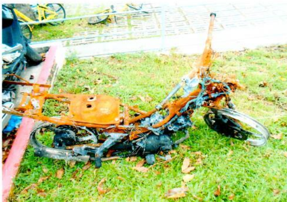
Photo 5 shows rust would normally start to develop around these areas soon after a fire as prolonged exposure to high heat intensity usually causes steel/metal material body parts to be exposed to natural environmental condition. The rust that had developed on the Insured Vehicle is an indication that it had sustained exposure to prolonged high heat intensity.
