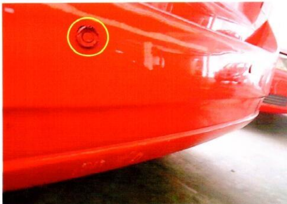
Photo 7 shows the left reverse sensor which was dislodged as a result of the rear bumper being pushed inwards (circled).
