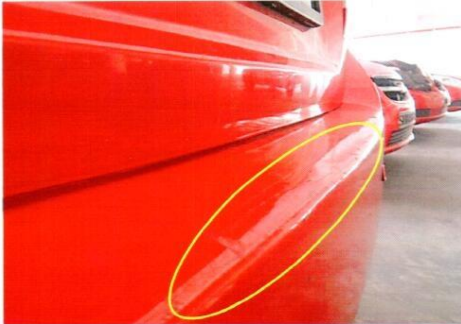
Photo 5 shows the paint cracks on the top portion of the rear bumper of the Taxi (circled).
