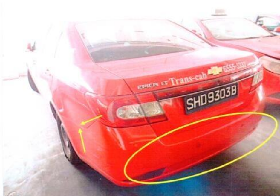
Photo 3 shows a left view of the rear portion of the Taxi at the time of the Pre-Repair Survey conducted by LKK Auto Consultants Pte. Ltd. taken 5 days after the accident. The damages were concentrated at the lower left portion and the top portion of the rear bumper (circled). We did not observe any obvious misalignment at the left corner edges of the rear bumper (arrowed).
