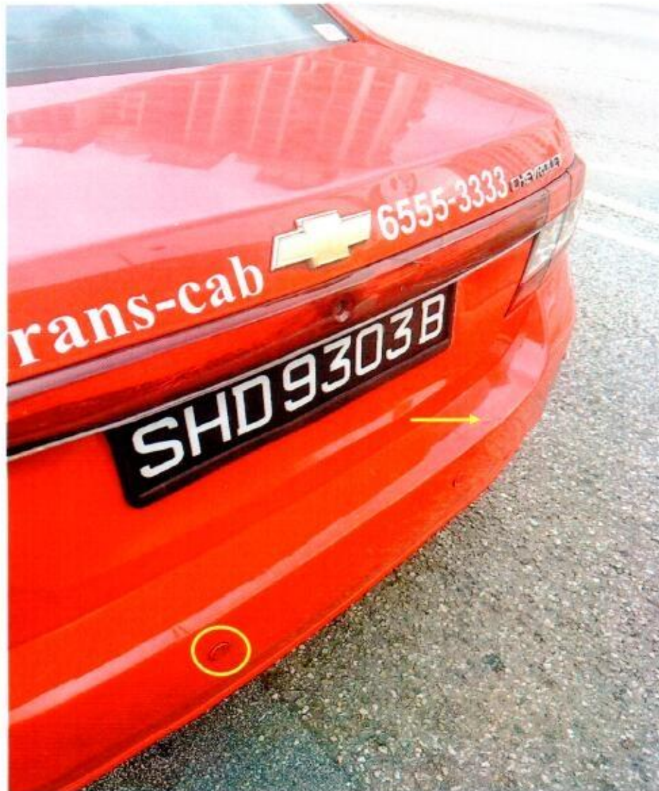
Photo 21 shows the rear portion of the Taxi post-accident. We observed the same paint cracks on the top portion of the Taxi's rear bumper (arrowed) as well as the dislodged left reverse sensor (circled).
