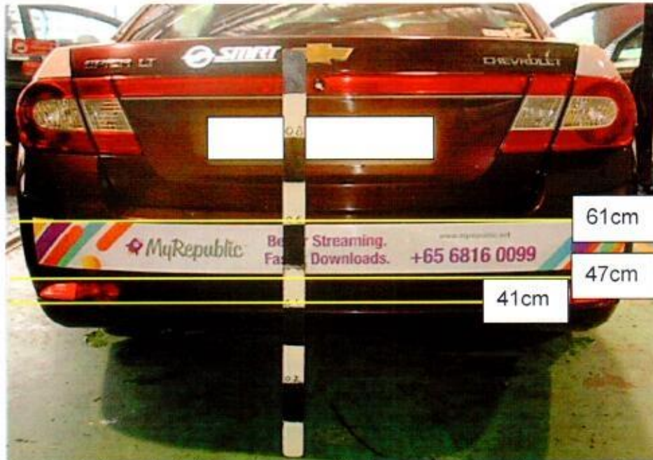
Photo 23 shows the height measurement being conducted on the rear portion of the Taxi (using a similar make and model). The height range above ground level of the Taxi's left reflector lamp where the vertical crack was found was measured to be approximately between 41cm to 47cm. The height above ground level of the top portion of the Taxi's rear bumper at the area where the paint cracks were found was measured to be approximately 61cm.
