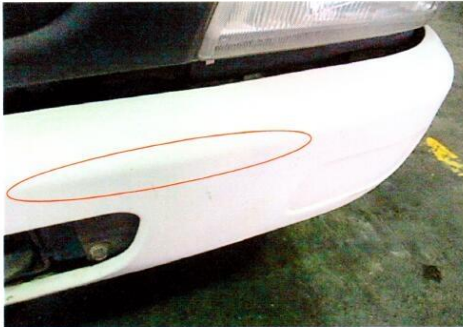
Photo 14 shows horizontal paint graze marks observed on the left portion of the Lorry's front bumper (circled).
