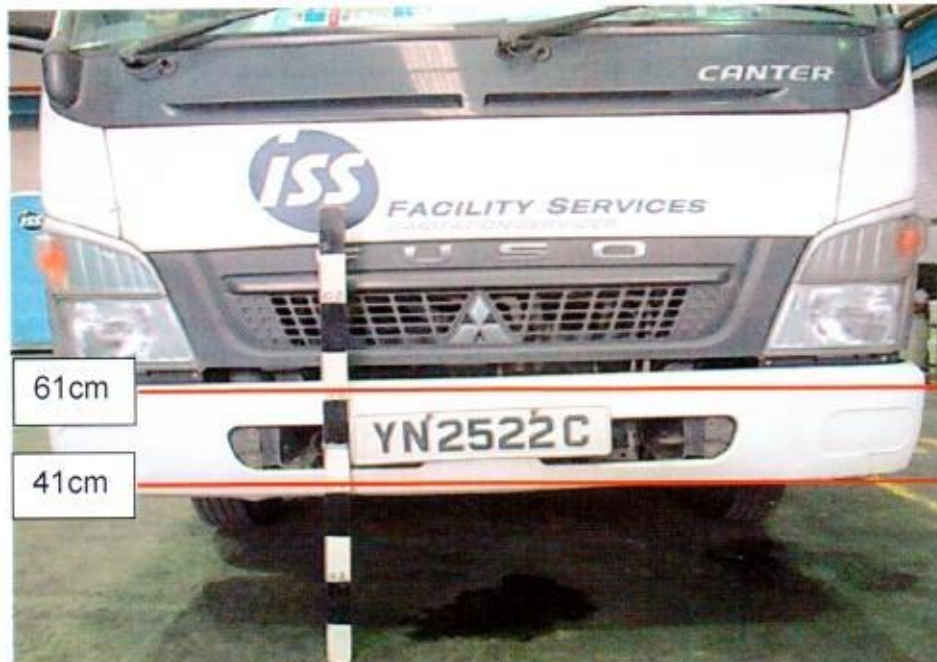
Photo 24 shows the height measurement being conducted on the front portion of the Lorry. The vertical dent found on the lower left portion of the Lorry's front bumper is within the 41cm to 47cm height range. The bodypart at 61cm above ground level was the left upper portion of the Lorry's front bumper which corresponded to the height of the red paint transfer marks found on the Lorry as well as the height of the paint cracks found on the top portion of the Taxi's rear bumper.
