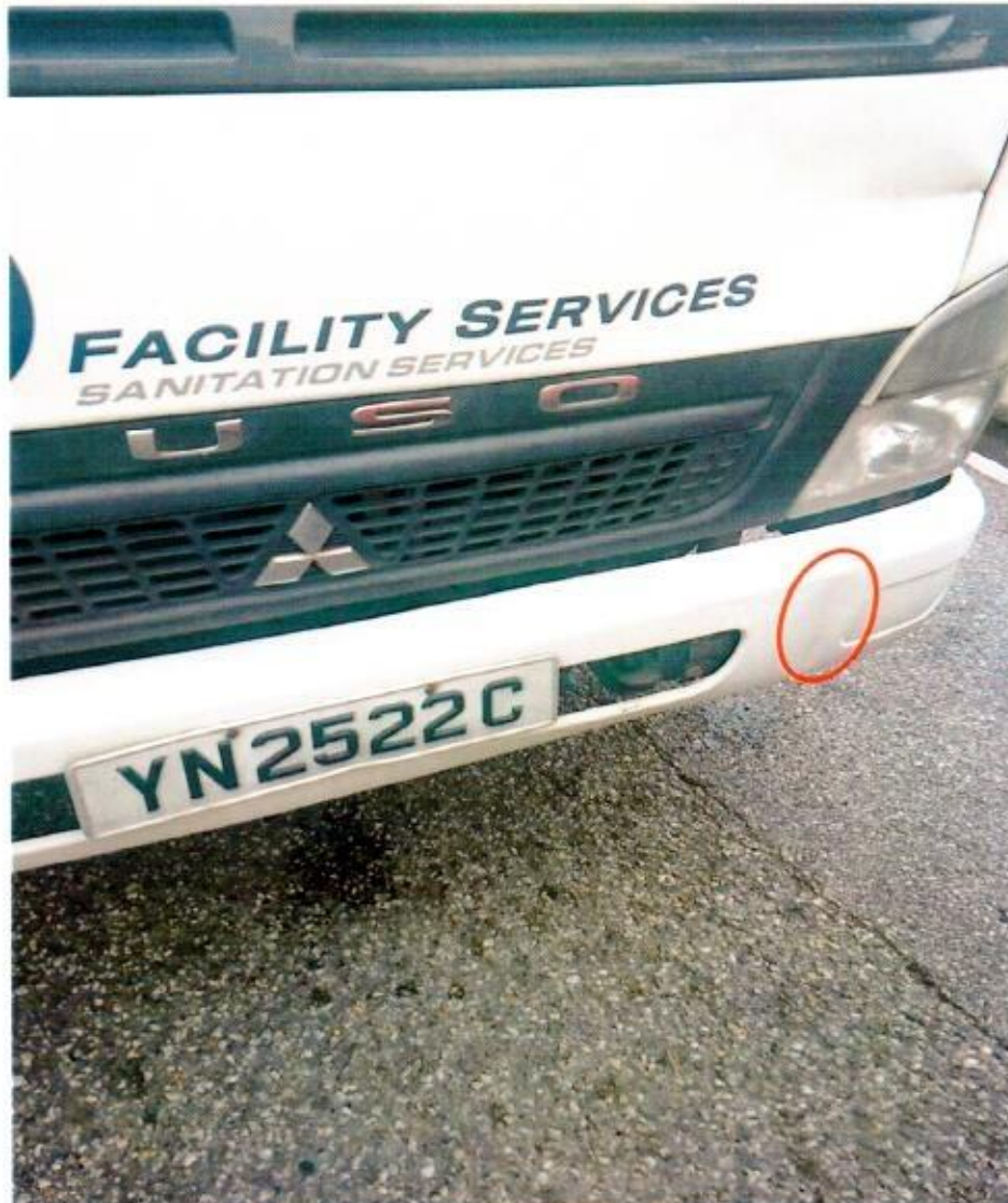
Photo 22 shows the front portion of the Lorry post-accident. We observed the same vertical dent on the lower left portion of the Lorry's front bumper (circled).
