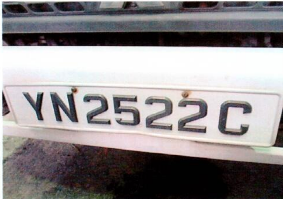
Photo 11 shows the Lorry's front number plate which was observed to be distorted.
