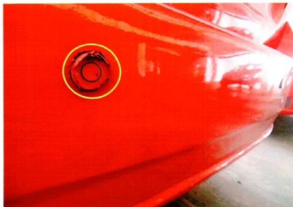
Photo 8 shows a close up view of the left reverse sensor which was dislodged as a result of the rear bumper being pushed inwards (circled).
