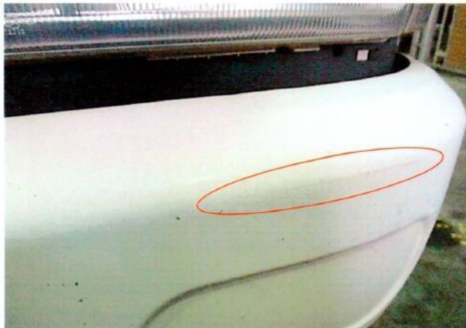
Photo 17 shows upon closer examination of the left portion of the Lorry's front bumper, we found faint red paint transfer marks (circled).
