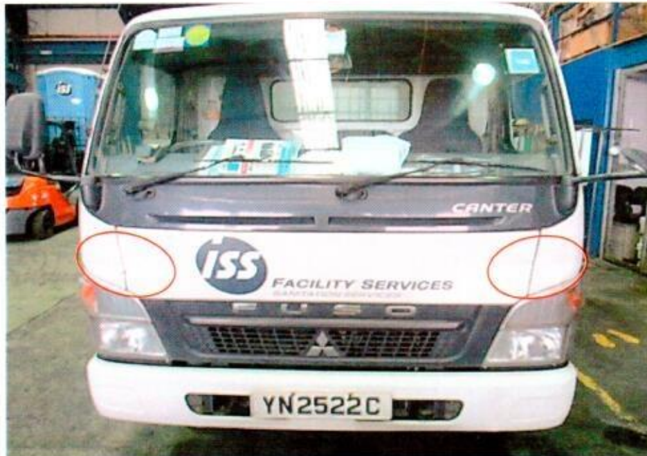
Photo 10 shows the general view of the front portion of the Lorry at the time of our physical inspection. We observed that the Lorry had sustained numerous damages on its front portion (circled) as a result of past accidents as mentioned by Mr Yew who was present during our physical inspection.
