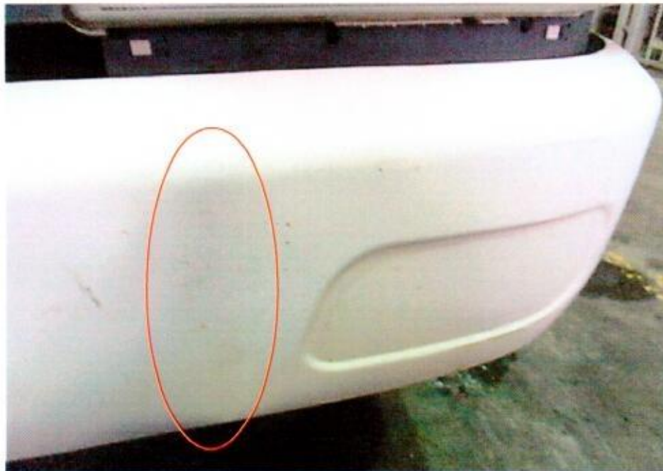
Photo 16 shows a closer view of the vertical dent found on the lower left portion of the Lorry's front bumper (circled).
