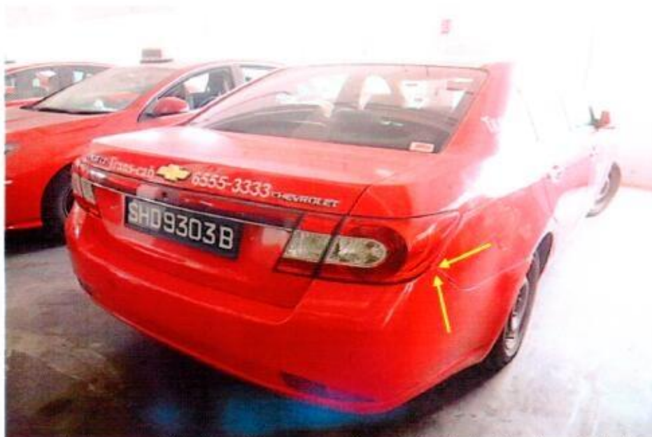
Photo 4 shows a right view of the rear portion of the Taxi at the time of the Pre-Repair Survey conducted by LKK Auto Consultants Pte. Ltd. taken 5 days after the accident. We did not observe any obvious misalignment at the right corner edges of the rear bumper (arrowed).
