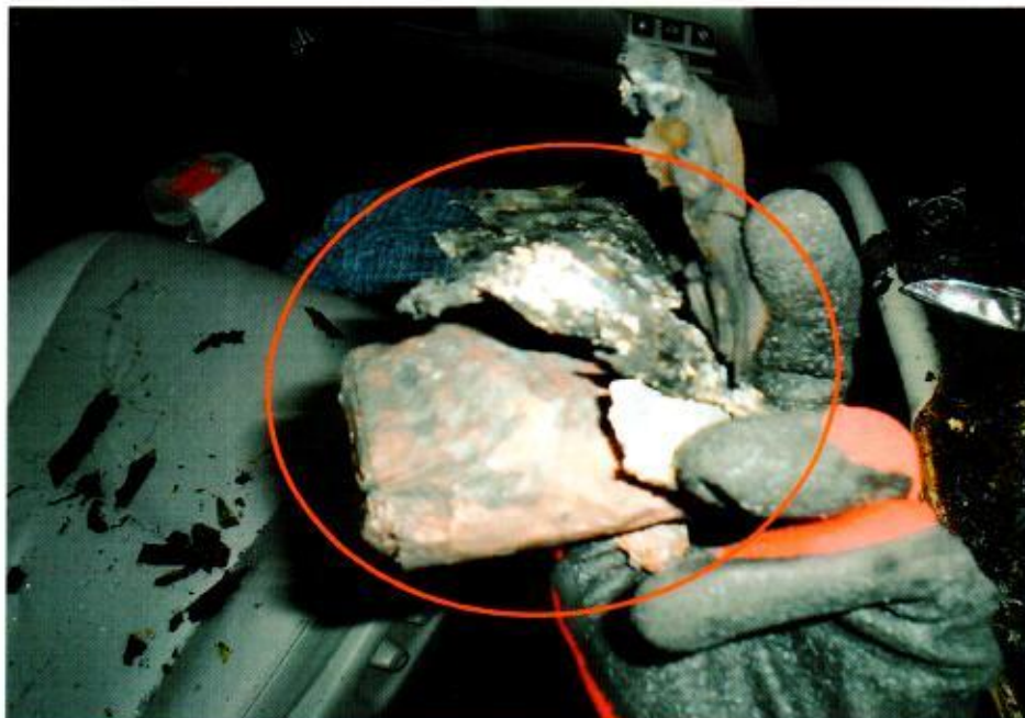
Photo 15 shows a closer view of the burnt 'Power Bank'. It was taken from the driver's interior door compartment.
