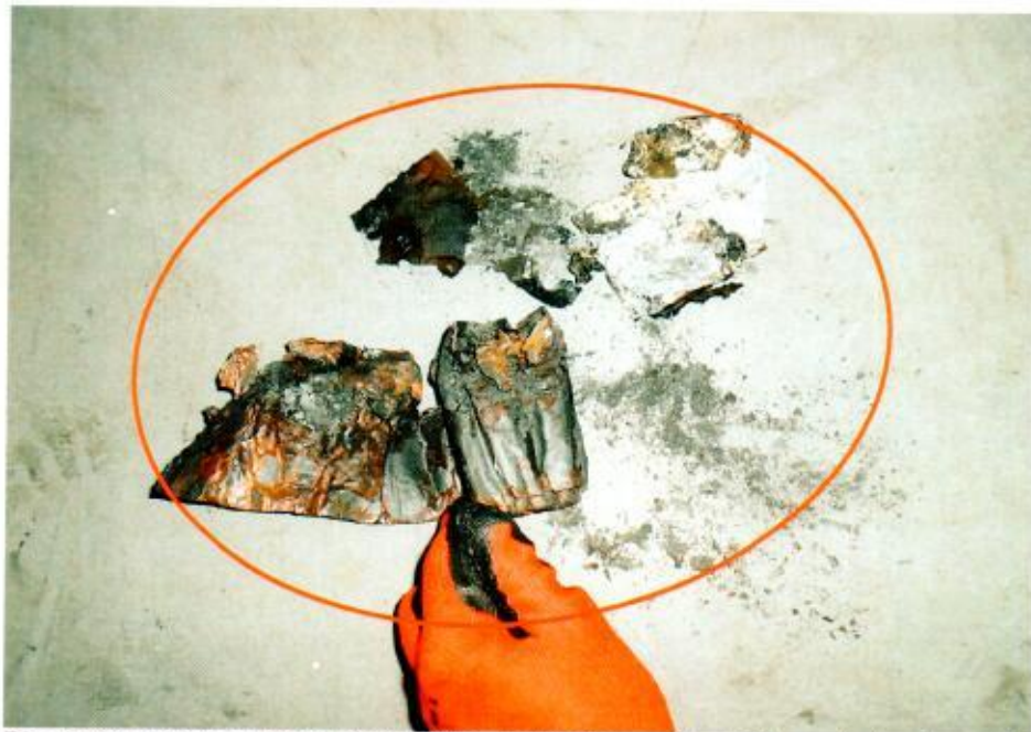
Photo 16 shows a closer view of the burnt 'Power Bank'. It was taken from the driver's interior door compartment.
