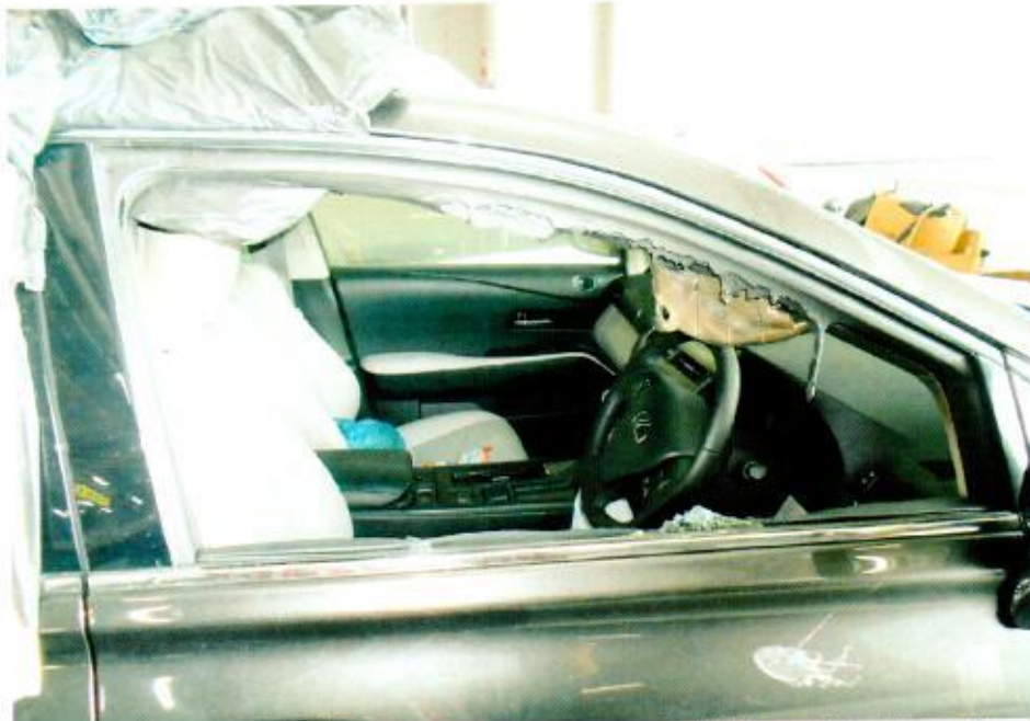
Photo 5 shows the driver's side of the Insured Vehicle at the time of our inspection. Its driver's side window was observed to be shattered due to the fire incident.
