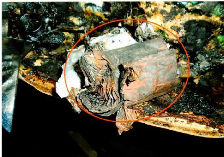
Photo 13 shows a closer view of the burnt 'Power Bank'. It was taken from the driver's interior door compartment.
