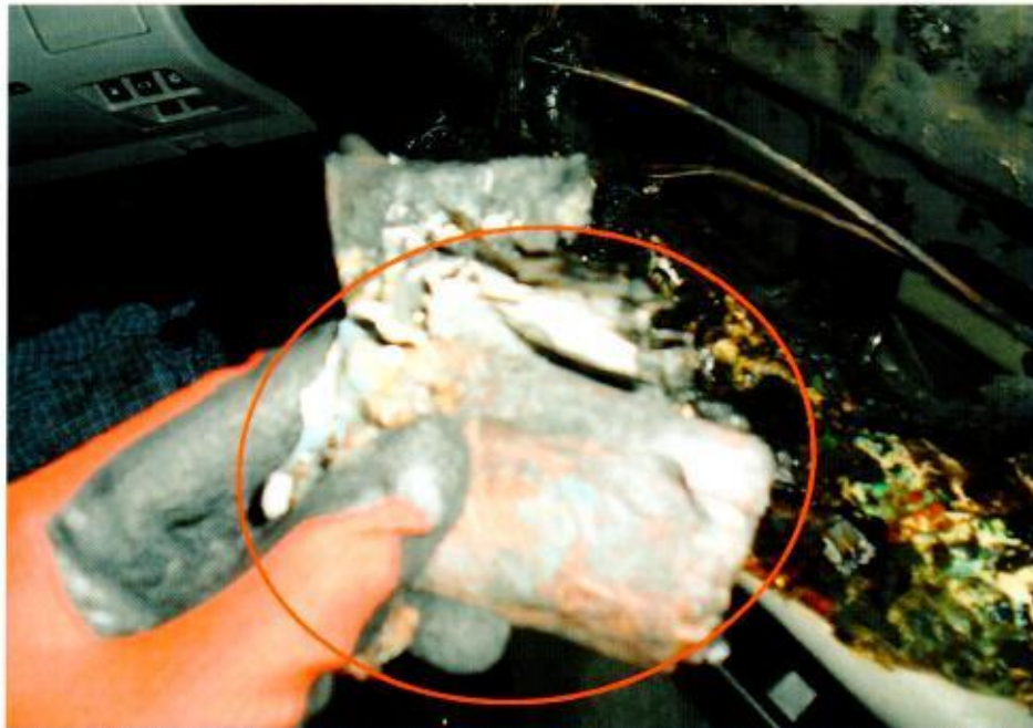
Photo 14 shows a closer view of the burnt 'Power Bank'. It was taken from the driver's interior door compartment.
