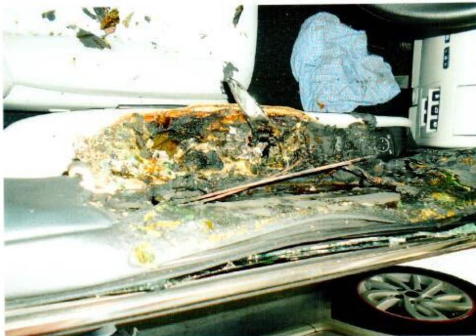
Photo 6 shows a closer view of the driver's interior door portion of the Insured Vehicle at the time of our inspection (top view). It was observed to be significantly burnt and/or melted as a result of the fire.
