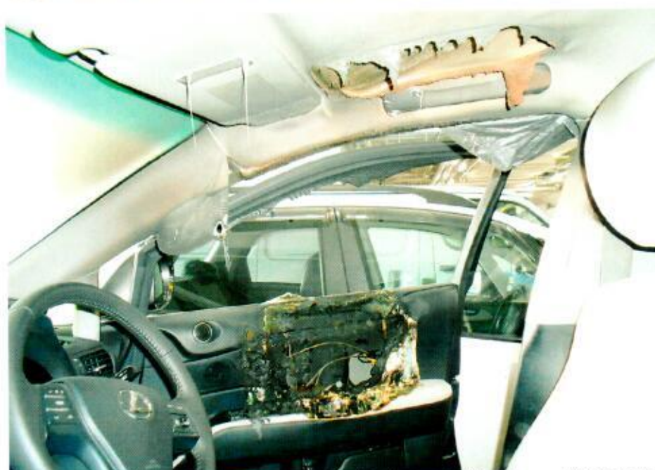
Photo 10 shows the general view of the driver's seat of the Insured Vehicle (as viewed from the front passenger's seat) at the time of our inspection. The affected area was observed only around the driver's seat area.
