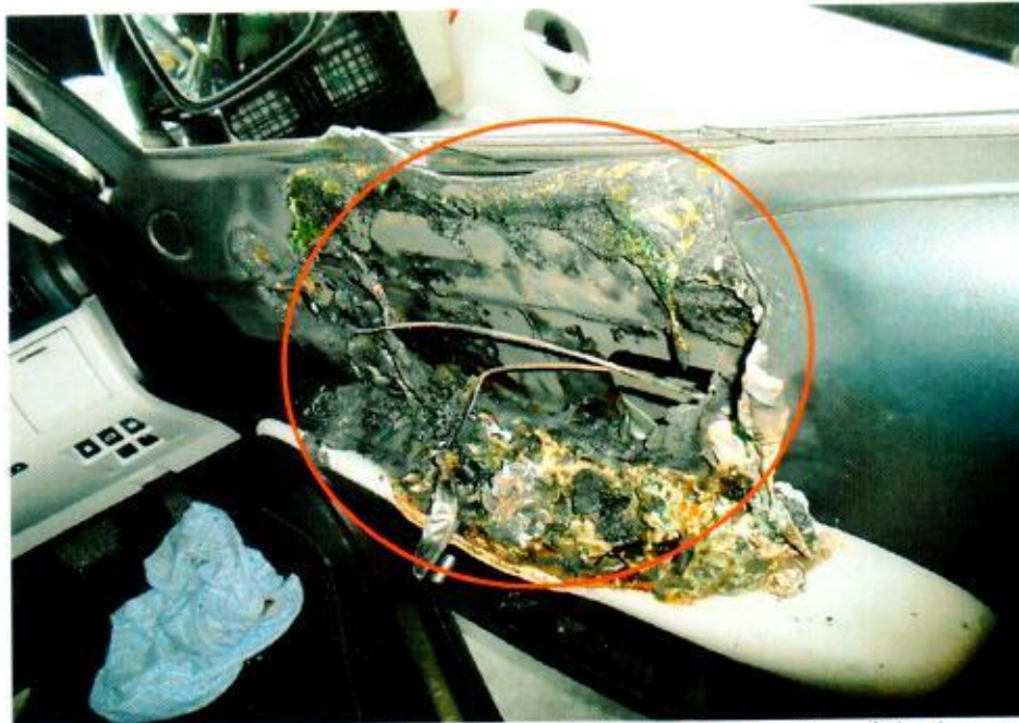
Photo 12 shows a closer view of the driver's interior door portion of the Insured Vehicle at the time of our inspection. It was observed to be significantly burnt and/or melted as a result of the fire.
