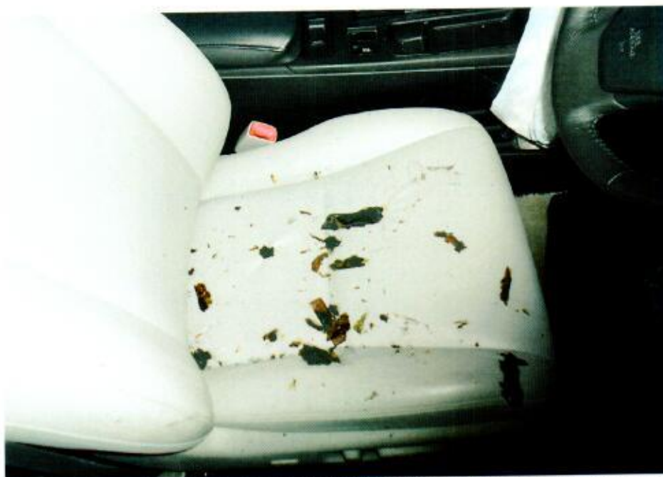
Photo 9 shows the charred rubber substance fell onto the Insured Vehicle seat. The debris was from the burnt materials from the driver's door portion.
