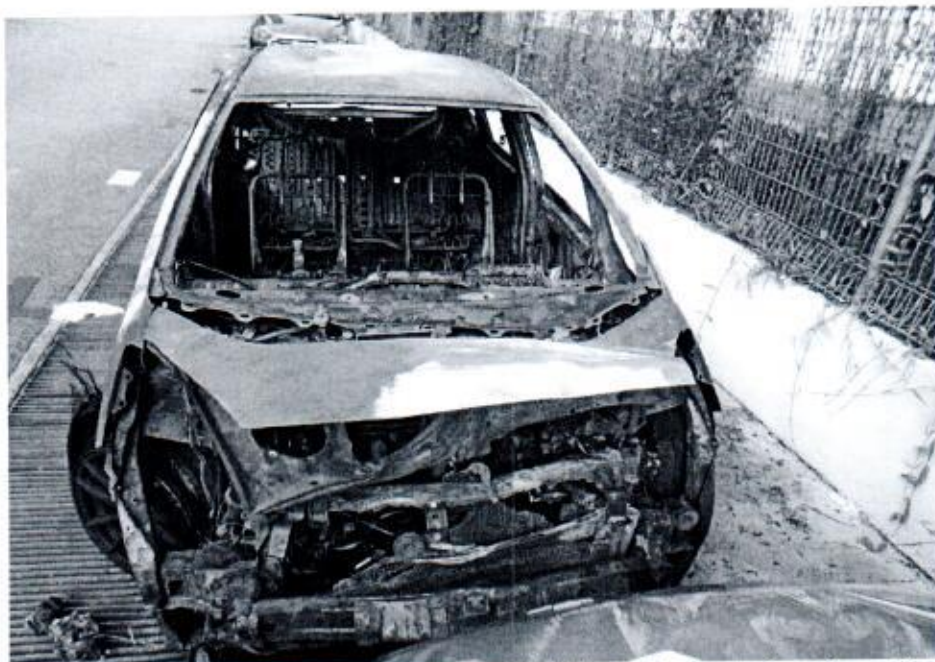
Photo 1 shows the front view of the Insured Vehicle at the time of our inspection. The Insured Vehicle was noted to have sustained fire damages that severely effected on the entire parts of the Insured Vehicle.
