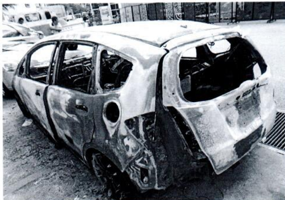
Photo 4 shows the rear left side of the Insured Vehicle at the time of our inspection. The Insured Vehicle was noted to have sustained fire damages that severely effected on the entire parts of the Insured Vehicle.
