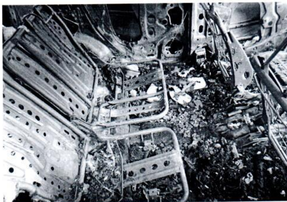
Photo 2 shows the interior view of the Insured vehicle, it was observed to have sustained with severe burnt damages due to the fire.
