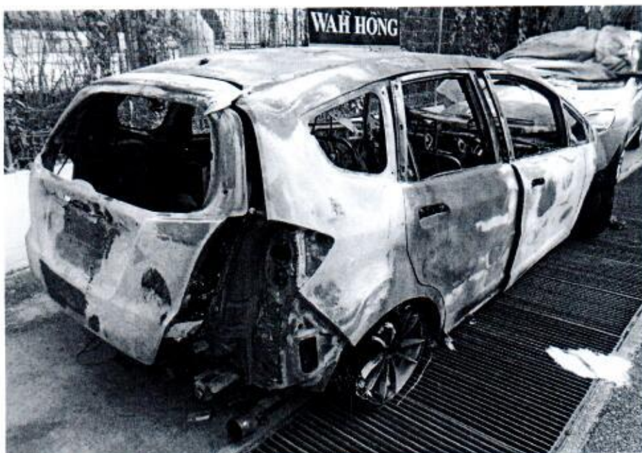
Photo 3 shows the rear right side of the Insured Vehicle at the time of our inspection. The Insured Vehicle was noted to have sustained fire damages that severely effected on the entire parts of the Insured Vehicle.
