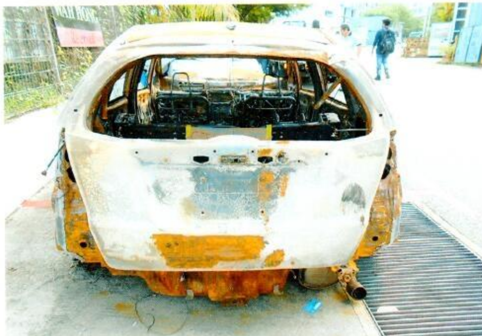
Photo 7 shows the whitish burn marks are a result of exposure to prolonged heat intensity. Rust would normally start to develop around these areas soon after a fire as prolonged exposure to high heat intensity usually causes steel/metal material body parts to be exposed to natural environmental condition. The rust that had developed on the Insured Vehicle is an indication that it had sustained exposure to prolonged high heat intensity.
